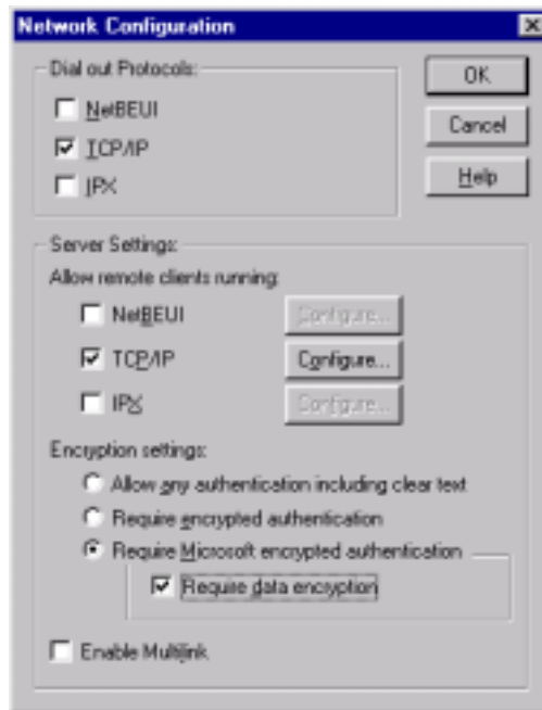
Figure 18 Windows NT Server RAS Network Configuration
