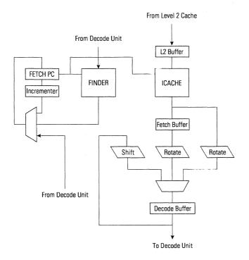
Figure 2: Instruction Fetch Unit Simplified Block Diagram
