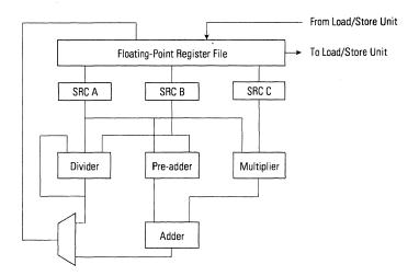
Figure 5: Floating-Point Execution Unit Block Diagram
