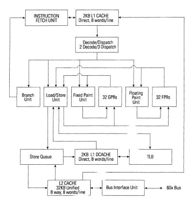
Figure 1: Data Path Simplified Block Diagram
