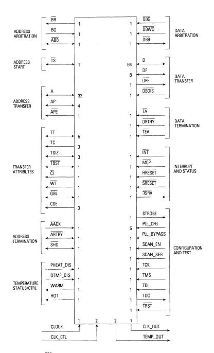
Figure 24: X<sup>704</sup> Bus Interface Signals
