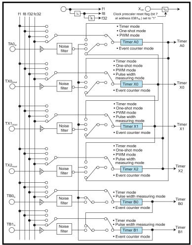
Figure 2—M16C/20 offers a competitive array of timers—far more than the typical 8-bit MCU—six channels, six pins, and a bunch of modes. Notice the flexible triggering options, including the chip's dual clocks (Xin and XCin).
