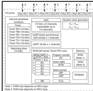
Figure 1—Bits shmitz! It's the copious memory (up to 48 KB of ROM or flash memory and 2 KB of RAM) and functional peripherals onboard, not the 16-bit ALU, that makes the M16C/20 such a good fit for mainstream embedded designs.
