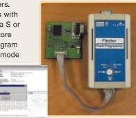
Supported MCUs : 16-bit M16C/80 Series 16-bit M16C/60 Series 16-bit M16C/20 Series 8-bit 740 Family 38000 Series
