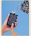
•Supports serial programming mode (Standard serial I/O mode) •Ultra small (card size) Approx.55(W) x 85(H) x 17(D)mm •Ultra light Approx.55g
