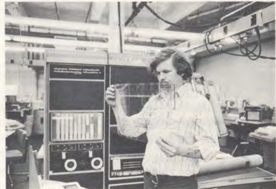
Gems Group Leader Al Brown examines a printed circuit board layout. This film was produced by the plotter and is the end result of the GEMS effort.
