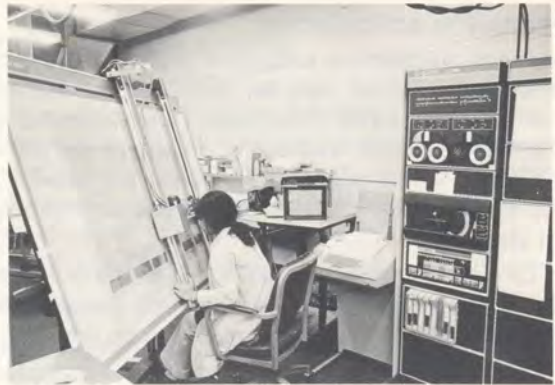
Dora Bacener logs the X/Y axis of components on a GEMS digitizer interfaced with a PDP-8/e.
