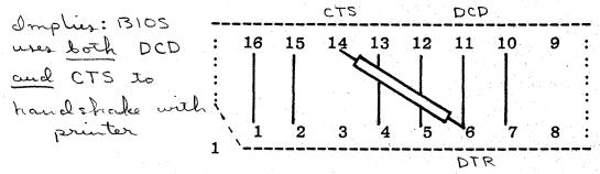
The DNB option on the TI 810 must be enabled by setting the panel switches to:
