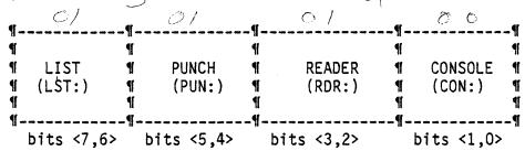
Whenever a reference to a logical device is made for I/O, the BIOS first looks at the appropriate bit field in the IOBYTE, and then uses one of the four physical devices service routines. The IOBYTE can be either examined or modified via the STAT command.
