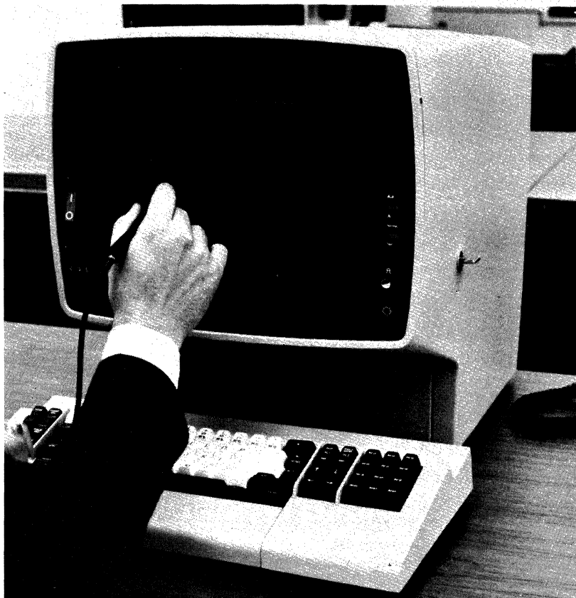
Figure 4-2. When using the selector light-pen, correct positioning of the tip of the pen is important.
