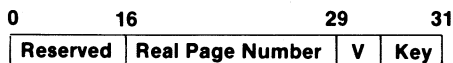
Figure 11-33. TLB Real Page Number, Valid, and Key Bits (One of Sixteen Per TLB)
