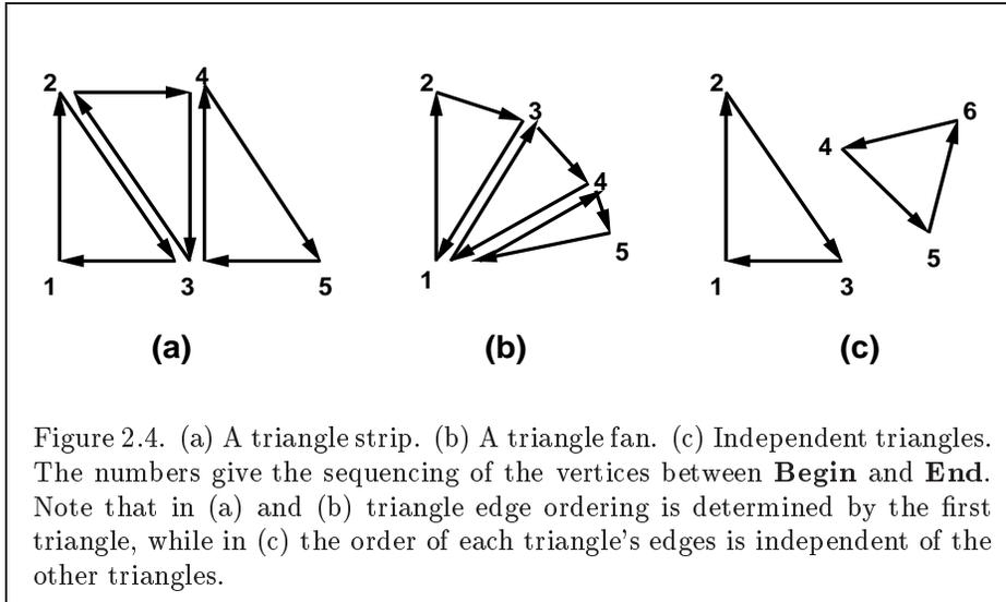
exception: each vertex after the first always replaces vertex B of the two stored vertices. The vertices of a triangle fan are enclosed between **Begin** and **End** when the value of the argument to **Begin** is **TRIANGLE\_FAN**.
