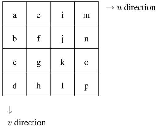
Table C.10: Pixel layout for an COMPRESSED\_RGB8\_ETC2 compressed block.
