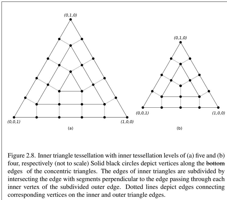
Figure 2.8. Inner triangle tessellation with inner tessellation levels of (a) five and (b) four, respectively (not to scale) Solid black circles depict vertices along the bottom edges of the concentric triangles. The edges of inner triangles are subdivided by intersecting the edge with segments perpendicular to the edge passing through each inner vertex of the subdivided outer edge. Dotted lines depict edges connecting corresponding vertices on the inner and outer triangle edges.
