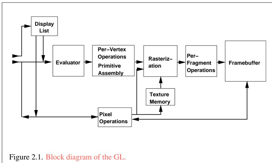
Figure 2.1. Block diagram of the GL.
