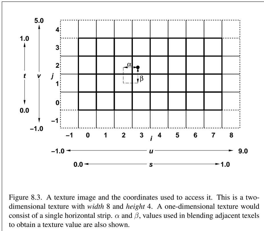
Figure 8.3. A texture image and the coordinates used to access it. This is a two-dimensional texture with *width* 8 and *height* 4. A one-dimensional texture would consist of a single horizontal strip.  $\alpha$  and  $\beta$ , values used in blending adjacent texels to obtain a texture value are also shown.
