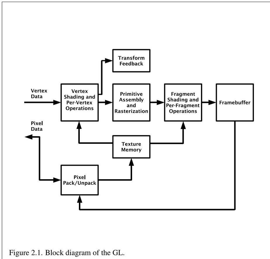
Figure 2.1. Block diagram of the GL.
