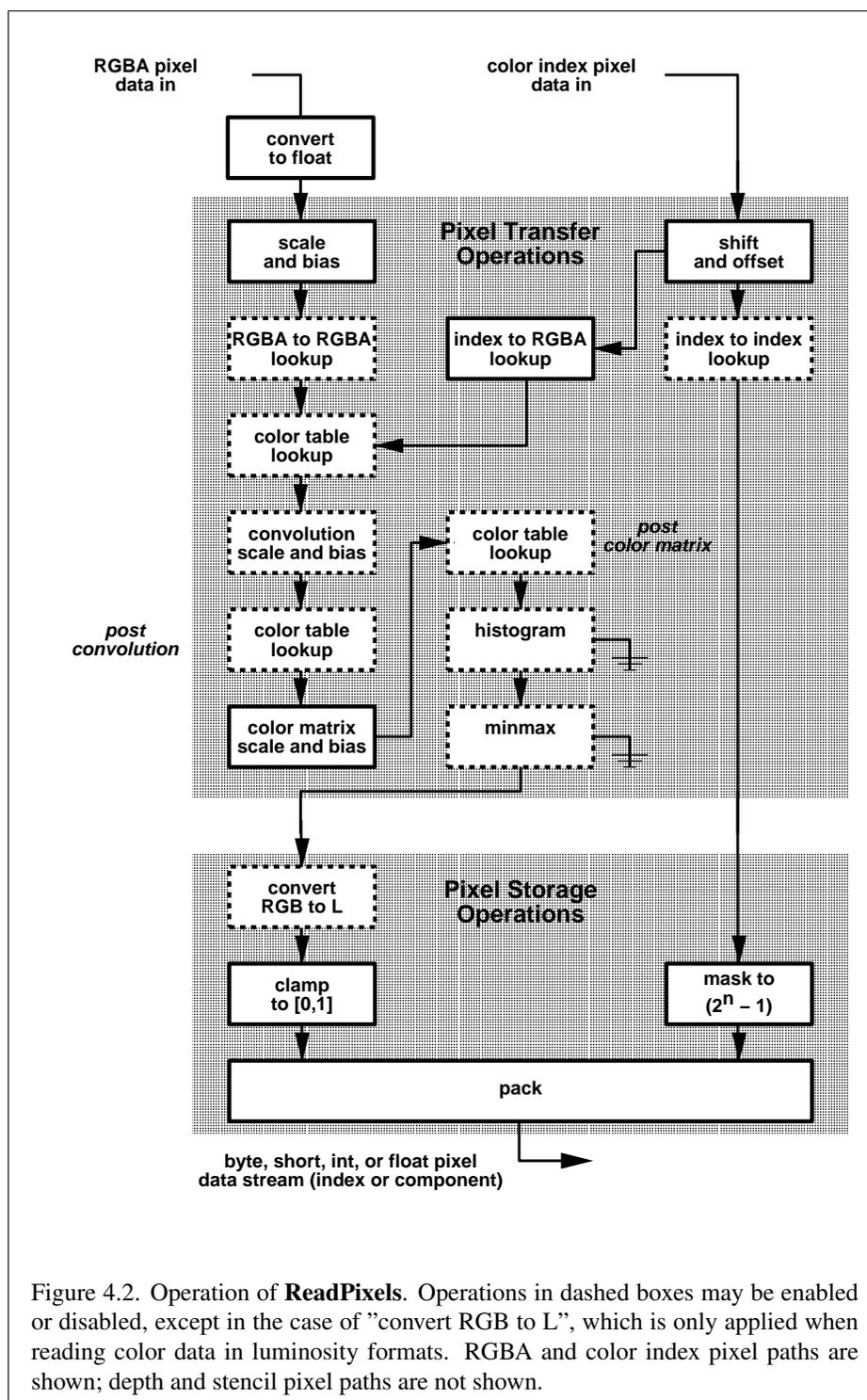
Figure 4.2. Operation of **ReadPixels**. Operations in dashed boxes may be enabled or disabled, except in the case of "convert RGB to L", which is only applied when reading color data in luminosity formats. RGBA and color index pixel paths are shown; depth and stencil pixel paths are not shown.
