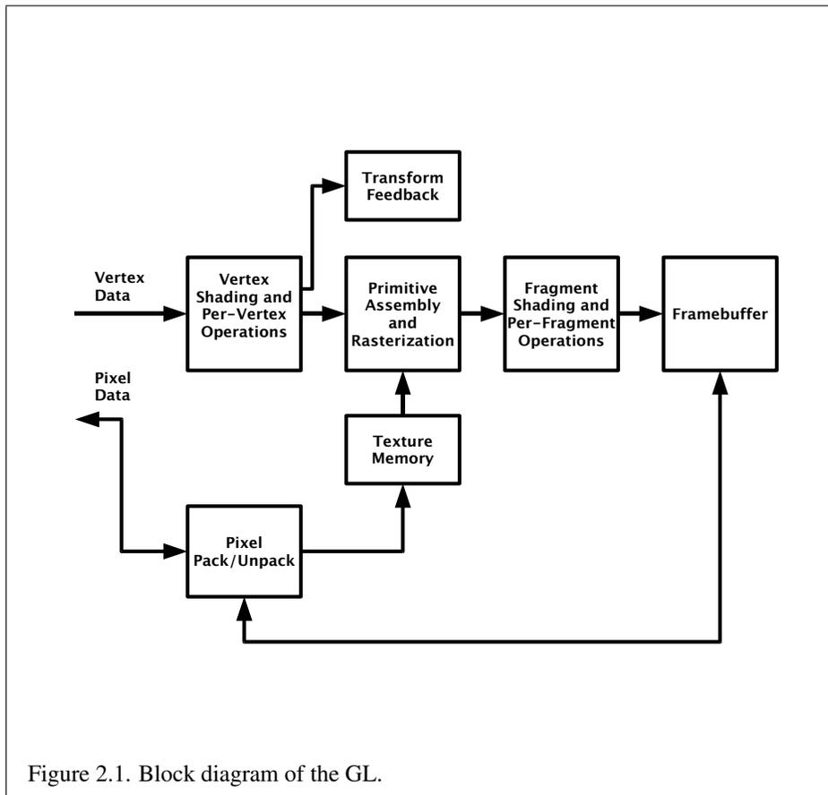
Figure 2.1. Block diagram of the GL.
