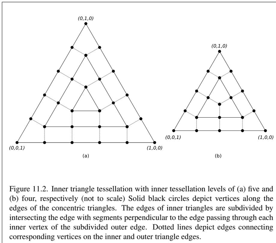
After all triangles are generated, each vertex in the subdivided triangle is assigned a barycentric  $(u, v, w)$  coordinate based on its location relative to the three vertices of the outer triangle.
