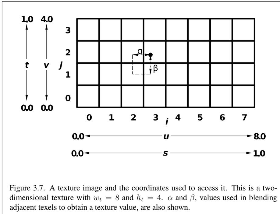
Figure 3.7. A texture image and the coordinates used to access it. This is a two-dimensional texture with  $w_t = 8$  and  $h_t = 4$ .  $\alpha$  and  $\beta$ , values used in blending adjacent texels to obtain a texture value, are also shown.
