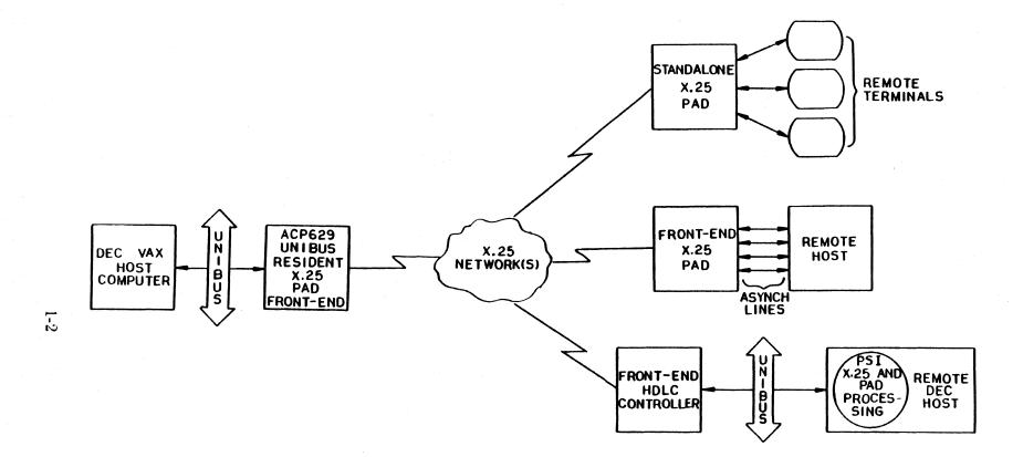
Figure 1-1. Typical X.25 Component PAD Configurations
