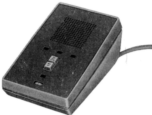
B. 2B TRANSMITTER-RECEIVER (THREE-PATH)
