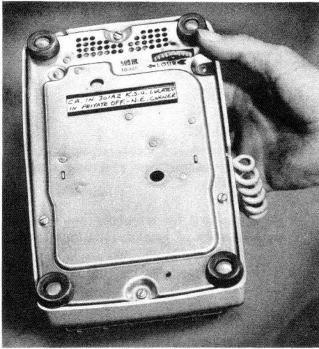
Fig. 3—Marking Equipment Location Using Form E-5826
