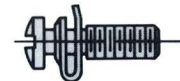
Male Screw Retainer (packaged 2 per kit) Material: Screw — Cadmium plated Steel Retainer Clip — Aluminum plated Steel Kit Part Number: 205980-1
