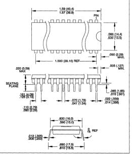
**40P6**, 40-Lead, 0.600" Wide, Plastic Dual-In-Line Dimensions in Inches and (Millimeters)
