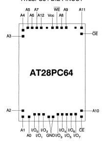
DIE SIZE: 146 X 217 mils CONNECT SUBSTRATE TO GROUND
