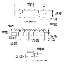
24D3, 24-Lead, 0.300" Wide, Non-Windowed Cerdip Dual-In-Line
