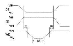
$t_S = t_H = 1 \mu sec (min.)$  $t_W = 10 msec (min.)$
