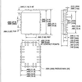
28KW, 28-Lead, Windowed, J-Leaded Chip Carrier Dimensions in Inches and (Millimeters)
