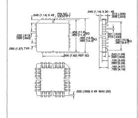
32J, 32-Lead Plastic J-Lead Chip Carrier Dimensions in Inches and (Millimeters) JEDEC OUTLINE MO-052 AE
