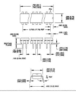
24P3, 24-Lead, 0.300" Wide, Plastic Dual-In-Line Dimensions in Inches and (Millimeters)
