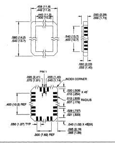
**44L**, 44-Pad, Non-Windowed, Ceramic Leadless Chip Carrier Dimensions in Inches and (Millimeters)
