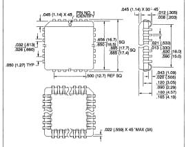
**68J**, 68-Lead Plastic J-Lead Chip Carrier Dimensions in Inches and (Millimeters)
