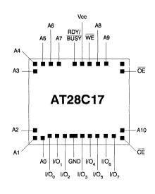
DIE SIZE: 137 X 117 mils CONNECT SUBSTRATE TO GROUND
