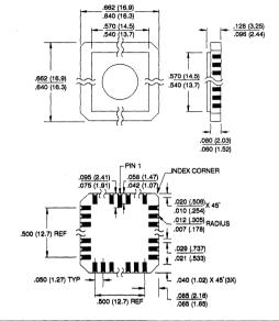
32M, 32-Lead, Non-Windowed, 32D6 Compatible, Ceramic Module Dimensions in Inches and (Millimeters)
