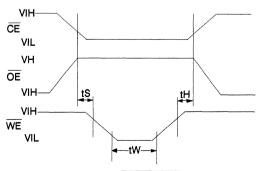
$t_S = t_H = 1\mu sec (min.)$   $t_W = 10 msec (min.)$  $V_H = 12 \pm 0.5 V$
