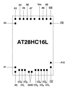
DIE SIZE: 118 X 144 mils CONNECT SUBSTRATE TO GROUND
