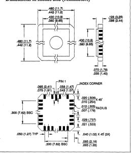
32LW, 32-Pad, Windowed, Ceramic Leadless Chip Carrier Dimensions in Inches and (Millimeters)
