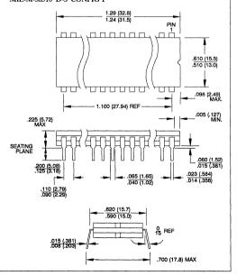
28D6, 28-Lead, 0.600" Wide, Non-Windowed, Cerdip Dimensions in Inches and (Millimeters)
