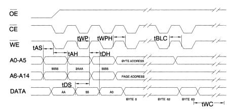
Notes: A6 through A14 must specify the page address during each high to low transition of WE (or CE) after the software code has been entered.
