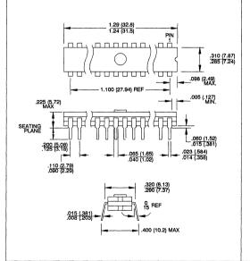
**24DW6**, 24-Lead, 0.600" Wide, Windowed, Cerdip Dimensions in Inches and (Millimeters)
