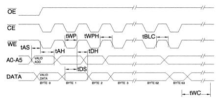
Note: A6 through A14 must specify the page address during each high to low transition of WE (or CE).
