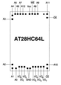
DIE SIZE: 146 X 217 mils CONNECT SUBSTRATE TO GROUND
