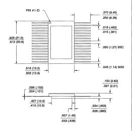
**24FW**, 24-Lead, Windowed, Brazed Flat Package Dimensions in Inches and (Millimeters)
