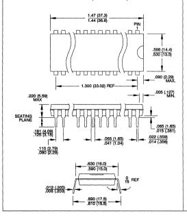
32P6, 32-Lead, 0.600" Wide, Plastic Dual-In-Line Dimensions in Inches and (Millimeters)
