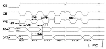
Note: A7 through A16 must specify the page address during each high to low transition of  $\overline{WE}$  (or  $\overline{CE}$ ).  $\overline{OE}$  must be high only when  $\overline{WE}$  and  $\overline{CE}$  are both low.
