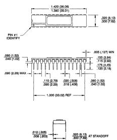
32B, 32-Lead, 0.600" Wide, Side Braze Ceramic Dual-In-Line Dimensions in Inches and (Millimeters) MIL-M-38510 CONFIG 3
