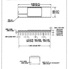
24C, 24-Lead, Non-Windowed, Cerpack Dimensions in Inches and (Millimeters) MIL-M-38510 F-6 CONFIG 1 JEDEC OUTLINE MO-019 AA
