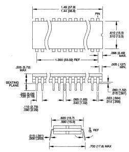
32D6, 32-Lead, 0.600" Wide, Non-Windowed, Cerdip Dimensions in Inches and (Millimeters)
