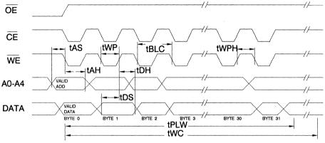
Note: A5 through A12 must specify the page address during each high to low transition of  $\overline{WE}$  (or  $\overline{CE}$ ).
