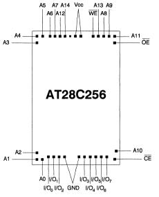
DIE SIZE: 224 X 323 mils CONNECT SUBSTRATE TO GROUND
