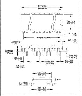
**28R**, 28-Lead, 0.330" Wide, Plastic Gull Wing SOIC Dimensions in Inches and (Millimeters)
