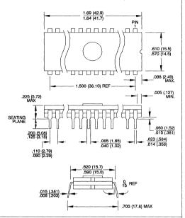
40DW6, 40-Lead, 0.600" Wide, Windowed, Cerdip Dimensions in Inches and (Millimeters)
