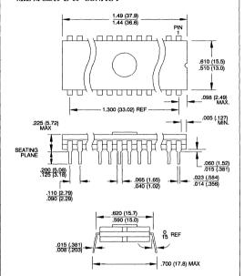
**32DW6**, 32-Lead, 0.600" Wide, Windowed, Cerdip Dimensions in Inches and (Millimeters)
