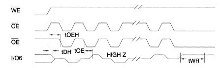
Notes: 1. Toggling either  $\overline{OE}$  or  $\overline{CE}$  or both  $\overline{OE}$  and  $\overline{CE}$  will operate toggle bit.
