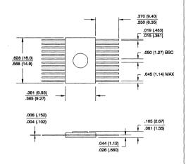
16D3, 16-Lead, 0.300" Wide, Non-Windowed, Cerdip Dimensions in Inches and (Millimeters)
