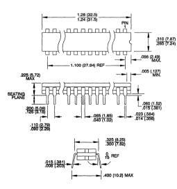
**24D6**, 24-Lead, 0.600" Wide, Non-Windowed, Cerdip Dimensions in Inches and (Millimeters) MIL-M-38510 D-3 CONFIG 1
