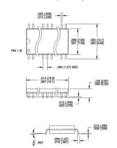
**24S**, 24-Lead, 0.300" Wide, Plastic Gull Wing SOIC Dimensions in Inches and (Millimeters)
