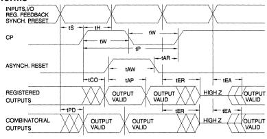
Note: 1. Timing measurement reference is 1.5V. Input AC driving levels are 0.0V and 3.0V, unless otherwise specified.
