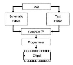
Note: 1. Examples of compilers are ABEL™, CUPL™, and LOG/iC. Each of these products contains modules which allow simulation of your design. They also minimize your logic equations, which gives you flexibility in describing your design.
