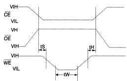
$t_S = t_H = 1\mu \sec (min.)$   $t_W = 10 \text{msec (min.)}$  $V_H = 12 \pm 0.5 \text{V}$
