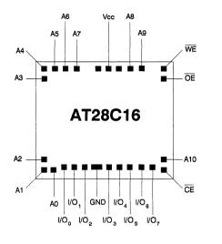
DIE SIZE: 137 X 117 mils CONNECT SUBSTRATE TO GROUND
