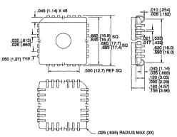
**68KW**, 68-Lead, Windowed, J-Leaded Chip Carrier Dimensions in Inches and (Millimeters)
