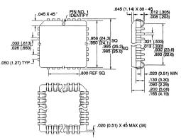
**32K**, 32-Lead, Non-Windowed, J-Leaded Chip Carrier Dimensions in Inches and (Millimeters)
