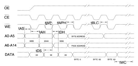
Notes: A6 through A16 must specify the page address during each high to low transition of WE (or CE) after the software code has been entered.
