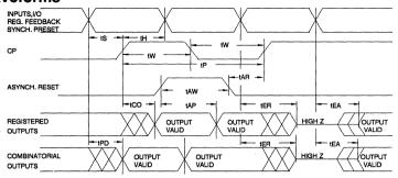
Note: 1. Timing measurement reference is 1.5V. Input AC driving levels are 0.0V and 3.0V, unless otherwise specified.
