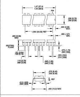
24P6, 24-Lead, 0.600" Wide, Plastic Dual-In-Line Dimensions in Inches and (Millimeters)
