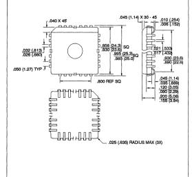
**28L**, 28-Pad, Non-Windowed, Ceramic Leadless Chip Carrier
