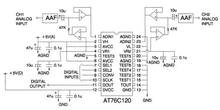
Notes: AVCC, AGND, +5V (A)— analog supply DVCC, GND, +5V (D)— digital supply
