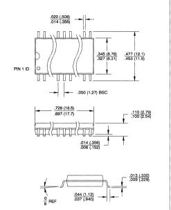
16S, 16-Lead, 0.300" Wide, Plastic Gull Wing SOIC Dimensions in Inches and (Millimeters)
