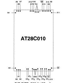
DIE SIZE: 356 X 429 mils CONNECT SUBSTRATE TO GROUND
