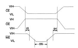
$t_S = t_H = 5\mu sec (min.)$  $t_W = 10 msec (min.)$
