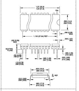
**28P6**, 28-Lead, 0.600" Wide, Plastic Dual-In-Line Dimensions in Inches and (Millimeters)
