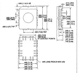
44KW, 44-Lead, Windowed, J-Leaded Chip Carrier Dimensions in Inches and (Millimeters)
