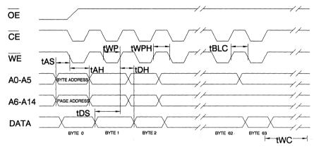
Notes: A6 through A14 must specify the page address during each high to low transition of  $\overline{WE}$  (or  $\overline{CE}$ ).
