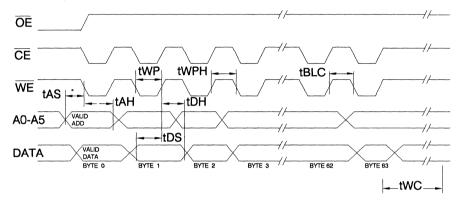
A6 through A16 must specify the page address during each high to low transition of  $\overline{WE}$  (or  $\overline{CE}$ ).  $\overline{OE}$  must be high only when  $\overline{WE}$  and  $\overline{CE}$  are both low. Note:
