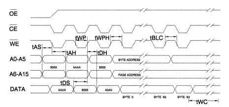
Notes: A6 through A15 must specify the page address during each high to low transition of WE (or CE) after the software code has been entered.
