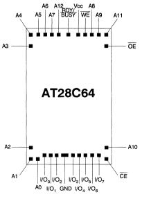
DIE SIZE: 133 X 207 mils CONNECT SUBSTRATE TO GROUND
