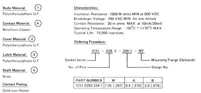
Figure 1. Unmodified Yamaichi SOIC socket.
