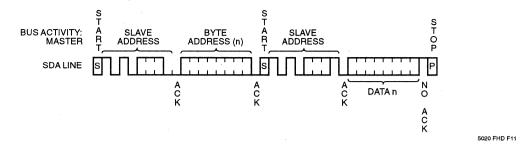
Figure 10. Sequential Read Timing
