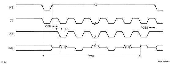
(11) Beginning and ending state of I/O6 is indeterminate.
