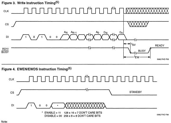
(5) The ORG pin is used to configure the device for x8 or x16 operation. When x8 organization is selected, AN = A7 and DN = D7. When x16 organization is selected, AN = A6 and DN = D15.
