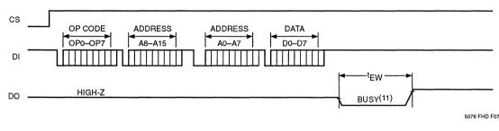
Figure 5. Program/Erase Timing (x16 Format)
