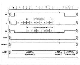
Figure 3. Temporary Change in Output
