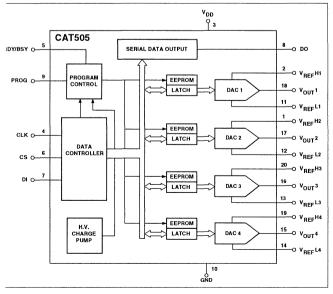
The CAT505 offers 4 independently programmable DACs each having its own reference inputs and each capable of rail to rail output swing. Output settings, stored non-volatile EEPROM memory, are not lost when the device is powered down and are automatically reinstated when power is returned. Each output can be dithered to test new output values without effecting the stored settings and stored settings can be read back without disturbing the DAC's output.
