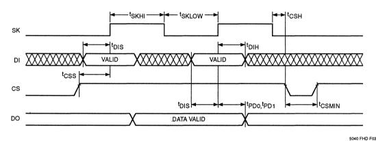
Figure 1. Sychronous Data Timing
