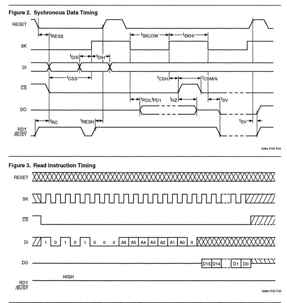
16 bit data field is also required following the 8 bit address field.
