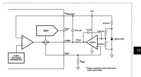
Figure 4a. External Voltage Reference, Single Supply
