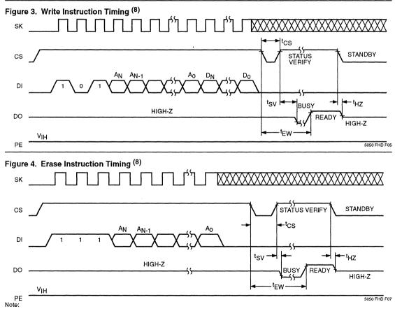
(8) The ORG pin is used to configure the device for x8 or x16 operation. When x8 organization is selected, AN = A10 and DN = D7. When x16 organization is selected, AN = A9 and DN = D15.
