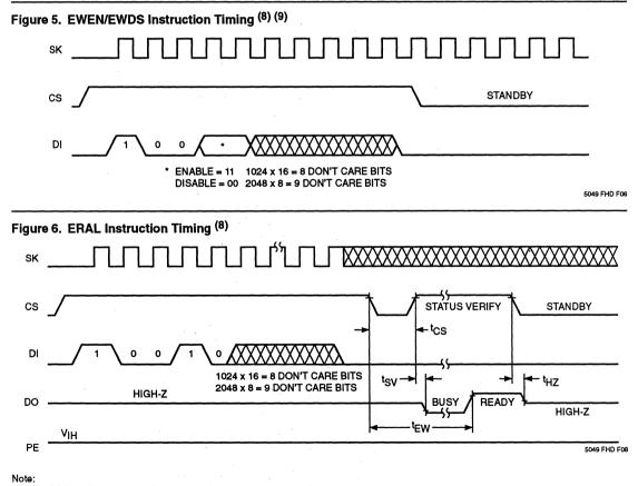
(8) The ORG pin is used to configure the device for x8 or x16 operation.
