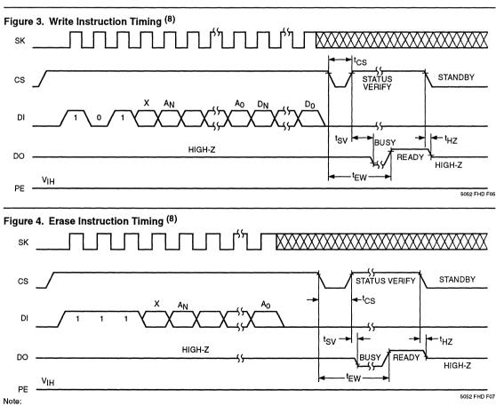
(8) The ORG pin is used to configure the device for x8 or x16 operation. When x8 organization is selected, AN = A9 and DN = D7. When x16 organization is selected, AN = A8 and DN = D15.
