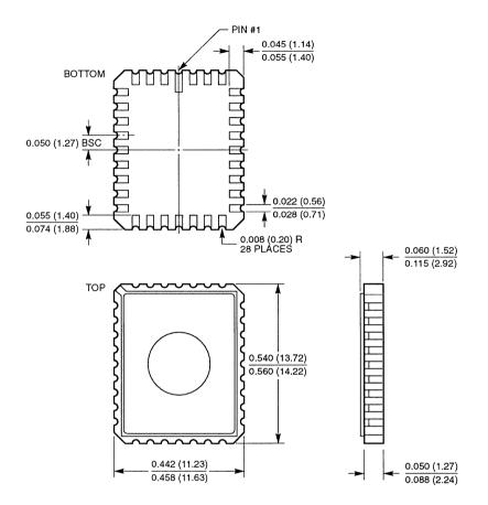
ote: All linear dimensions are in inches and parenthetically in millimeters.
