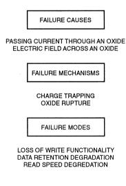
specification or serial E<sup>2</sup>PROMs of low density. Err correction is not practical for charge trapping induce failures. A low failure rate during the useful life region achieved by proper design, processing, and screenin
