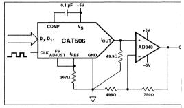
Figure 2. Buffer Voltage Output 0 to +2.5V
