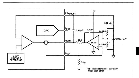
Figure 4a. External Voltage Reference, Single Supply
