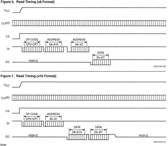
(8) Clock = 4.9152 MHz for the CAT33C804A or 3.579545 MHz for the CAT33C804B.
