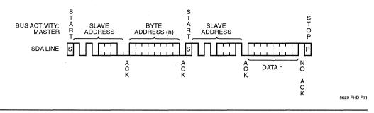
Figure 10. Sequential Read Timing
