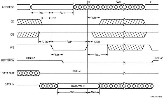
falling edge of  $\overline{WE}$  or  $\overline{CE}$ , whichever occurs last. Data, conversely, is latched on the rising edge of  $\overline{WE}$  or  $\overline{CE}$ . whichever occurs first. Once initiated, a byte write cycle automatically erases the addressed byte and the new data is written within 10 ms.
