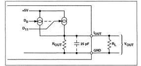
Figure 1. DAC Output Equivalent Circuit
