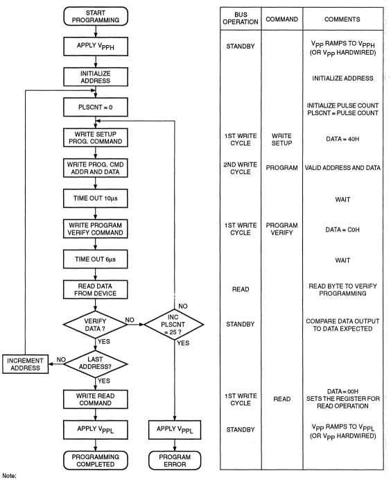
(16) The algorithm MUST BE FOLLOWED to ensure proper and reliable operation of the device.
