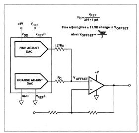
Coarse-Fine Offset Control by Averaging DAC Outputs for Single Power Supply Systems
