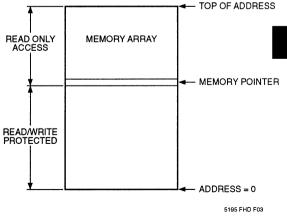
In addition, to allow for reading multiple words from the memory and minimize the overhead of repeated Read instructions, a Read Sequential (RSEQ) instruction allows you to specify a starting location and then continuously shift out data to the end of the array.
