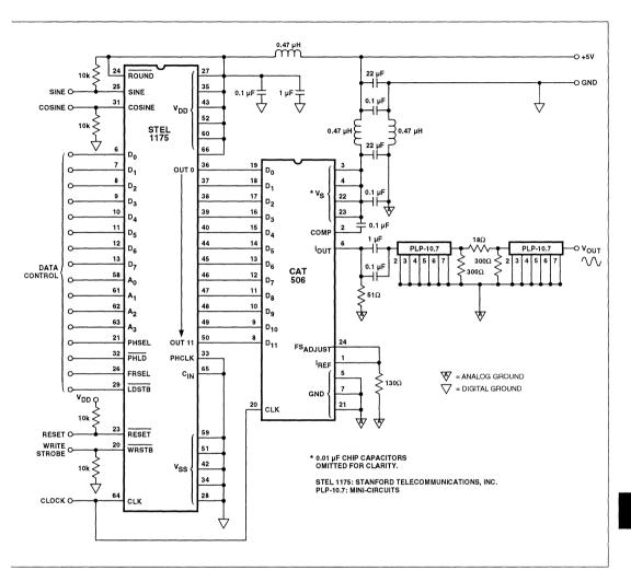
Figure 6. Direct Digital Synthesis (DDS) Using the CAT506
