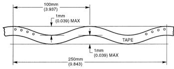
ALLOWABLE CAMBER TO BE 1mm/100mm NONACCUMULATIVE OVER 250mm
