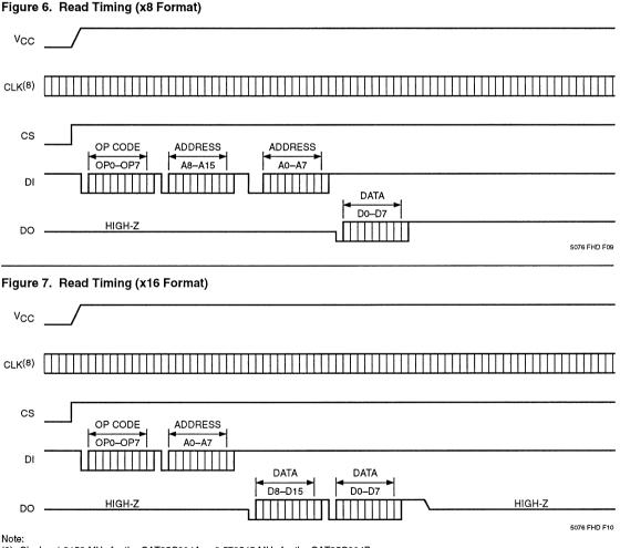
(8) Clock = 4.9152 MHz for the CAT35C804A or 3.579545 MHz for the CAT35C804B.
