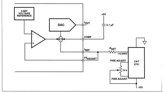
Figure 4b. External Voltage Reference, Dual Supply
