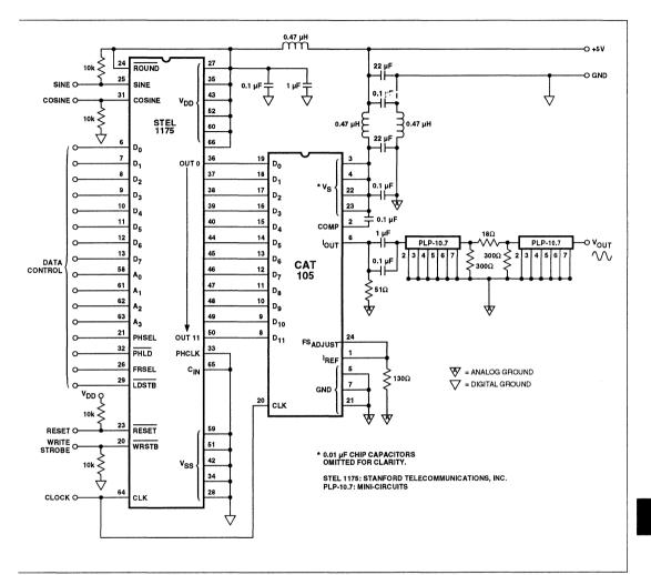
Figure 6. Direct Digital Synthesis (DDS) Using the CAT105
