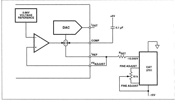
Figure 4b. External Voltage Reference, Dual Supply
