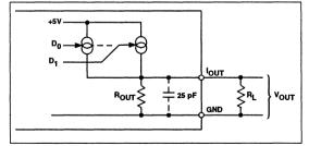
Figure 1. DAC Output Equivalent Circuit
