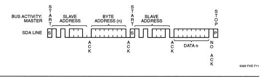
Figure 10. Sequential Read Timing
