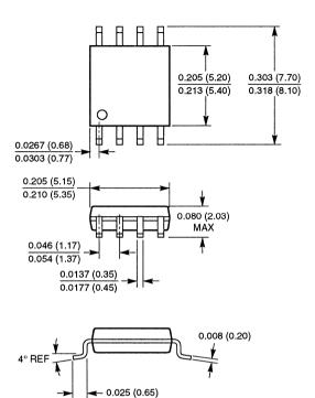
Note: 1. All linear dimensions are in inches and parenthetically in millimeters.
