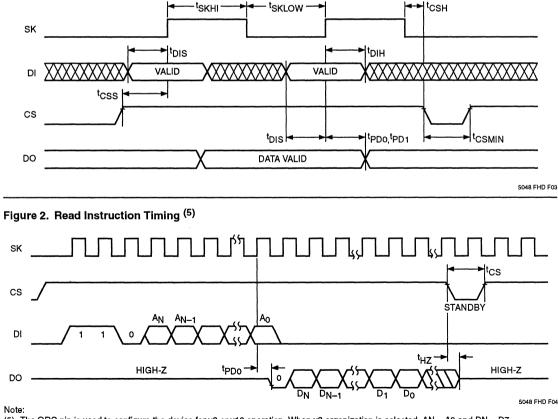
(5) The ORG pin is used to configure the device for x8 or x16 operation. When x8 organization is selected, AN = A8 and DN = D7. When x16 organization is selected, AN = A7 and DN = D15. At power-down, when  $V_{CC}$  falls below a threshold of approximately 3.5V, the data protection circuitry inhibits the erase and write instructions and a write disable (EWDS) is executed internally.
