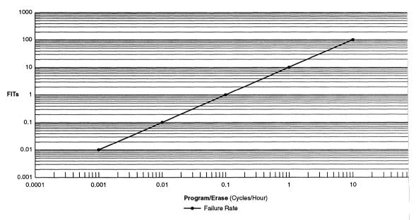
Figure 2. Endurance Cycles to Time Conversion Nomograph
