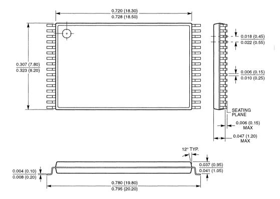
Note: 1. All linear dimensions are in inches and parenthetically in millimeters.
