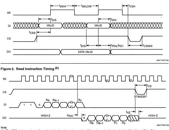
(6) The ORG pin is used to configure the device for x8 or x16 operation. When x8 organization is selected, AN = A8 and DN = D7. When x16 organization is selected, AN = A7 and DN = D15. At power-down, when  $V_{CC}$  falls below a threshold of approximately 2.4V, the data protection circuitry inhibits the erase and write instructions and a write disable (EWDS) is executed internally.
