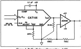
Figure 2. Buffer Voltage Output 0 to +2.5V
