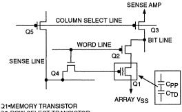
Q2•ROW SELECT TRANSISTOR Q3•COLUMN SELECT TRANSISTOR Q4•BYTE SELECT TRANSISTOR Q5•SENSE SELECT TRANSISTOR
