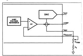
Figure 3. FSADJUST Equivalent Circuit
