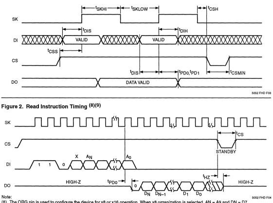
(8) The ORG pin is used to configure the device for x8 or x16 operation. When x8 organization is selected, AN = A9 and DN = D7. When x16 organization is selected, AN = A8 and DN = D15.
