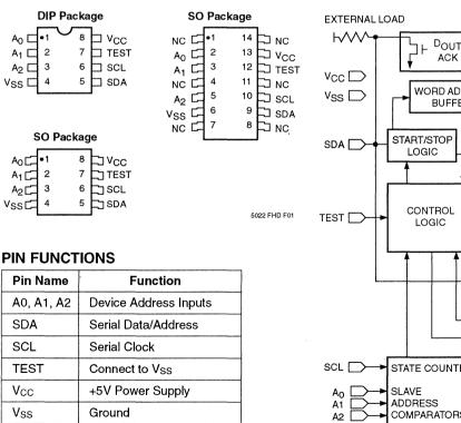
features a 16 byte page write buffer. The device operates via the  $l^2$ C bus serial interface and is available in 8 pin DIP, 8 pin SO and 14 pin SO packages.
