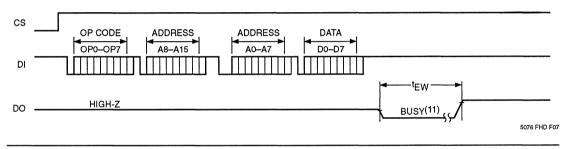
Figure 5. Program/Erase Timing (x16 Format)
