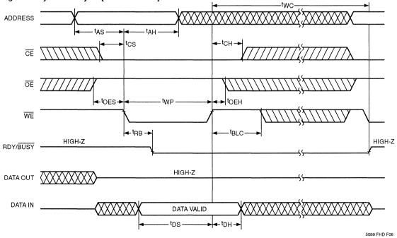
falling edge of  $\overline{WE}$  or  $\overline{CE}$ , whichever occurs last. Data, conversely, is latched on the rising edge of  $\overline{WE}$  or  $\overline{CE}$ , whichever occurs first. Once initiated, a byte write cycle automatically erases the addressed byte and the new data is written within 5 ms.
