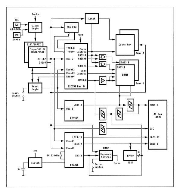
Figure 1-1. MK82310-PI-Super System Block Diagram
