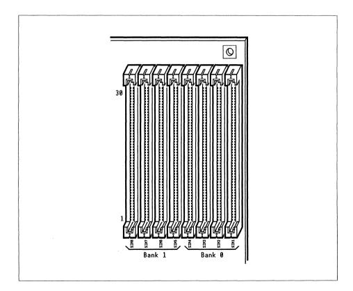
SIMMs 1-4 are configured as bank 0. SIMMs 5-8 are configured as bank 1. The same type of memory must be placed placed in each bank if interleaving of banks is to be used. When only one bank is populated, bank 0 should be used. The MK82310-PI-Super board can be configured for different amounts of memory. Table 3-10 shows the possible memory configurations.
