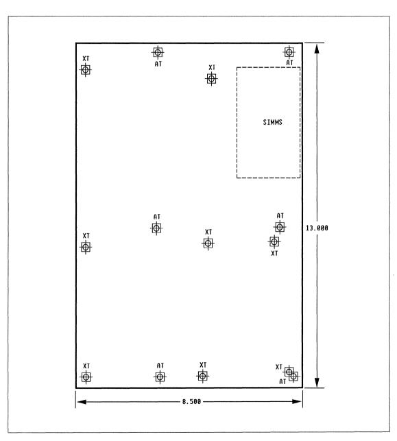
Figure 3-4. MK82310-PI-Super Board Mounting Holes
