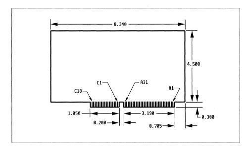
AT slot 5 on the MK82310-PI-Super board accommodates XT adapter boards with PCB depths below the 8-bit I/O connector. XT cards can have depths up to 0.5 inch below the 8-bit I/O connector. Note that AT slot 5 can be optionally populated with an 8-bit or 16-bit I/O connector. The MK82310-PI-Super is shipped with AT slot 5 configured as an 8-bit slot. Figure 3-8 shows the XT deep slot adapter board dimensions.
