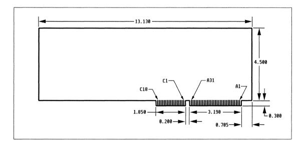
Figure 3-6. AT Adapter Board, Full-Length
