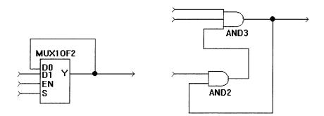
Figure 5-21 Examples of combinatorial loops (feedback)
