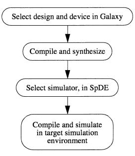
Figure 8-2 Simulation design flow for FPGAs
