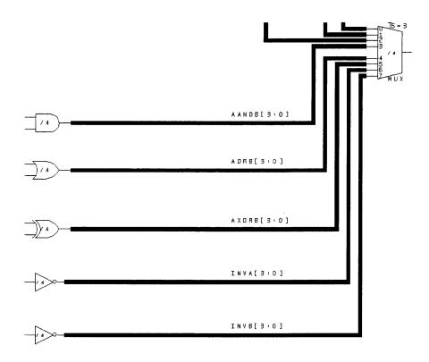
Figure 3-54 Connecting the mux to AND, OR, XOR, and inverters
