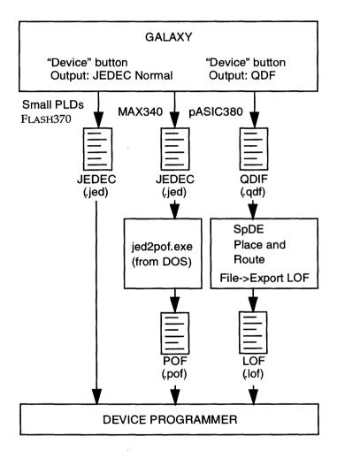
Figure 10-1 Design flow for device programming
