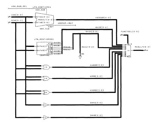
Figure 3-51 Final circuit of PLD design
