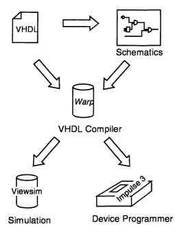
Figure 7-1 Warp3 design flow
