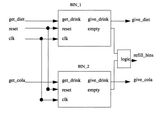
Figure 3-7 Block Diagram for refill.vhd
