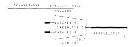
Figure 3-57 Connecting the Add-sub component
