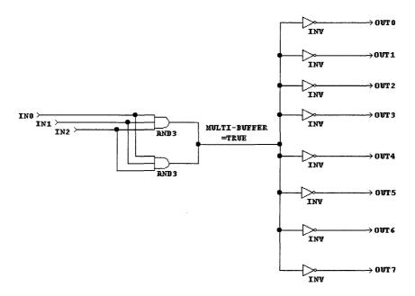
Figure 5-26 Double buffering example
