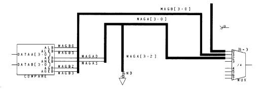
Figure 3-53 Connection the comparators to the mux
