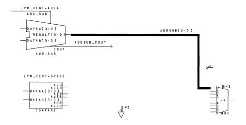
Figure 3-52 Connecting the mux to the comparator
