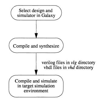
Figure 8-1 Simulation design flow for PLDs and CPLDs
