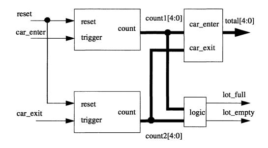
Figure 3-29 Block Diagrm for total.vhd
