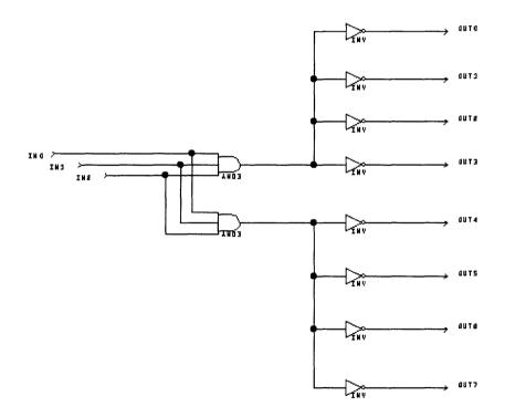
Figure 5-29 Circuit demonstrating paralleling
