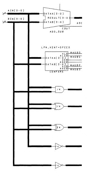
Figure 3-55 Connecting the A and B input buses
