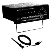
caused by cable resistance. A front panel LED overload lamp lights if the output exceeds 25 mA and current limiting occurs at 70 mA output. The output circuit can accept up to  $\pm 25$  mA source or sink current at rated accuracy. The rear connector also includes a low-Z output of the +10 Volt reference source with 5 mA maximum drive for external reference tracking. Wideband output noise is 25 microvolts, pk max.
