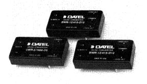
Industry standard packaging (2" x 1" x 0.375") coupled with across the board pin-out compatibility with other suppliers makes DATEL's 10 Watt UWR/BWR Series of dc-to-dc power converters ideal as drop-in replacements for larger, less reliable converters from other manufacturers.
