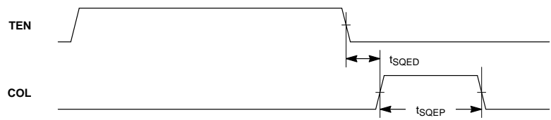
Figure 34. Mode 4 COL/CI Output Timing
