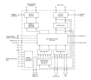
Figure 2. 3002 Block Diagram
