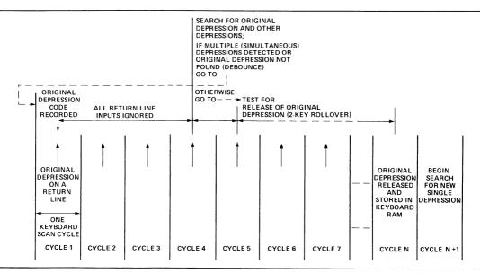
Figure 3. Keyboard Debounce and 2-Key Rollover Timing.
