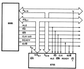
\*USE CE FOR FIRST 8755 IN SYSTEM, AND CE FOR OTHERS. BY CONNECTING CE OF EACH 8755 CHIP TO EACH OF A<sub>11</sub> THROUGH A<sub>15</sub>, THE MINIMUM SYSTEM CAN USE 5-8755's (10K BYTES) WITHOUT REQUIRING CE DECODER.
