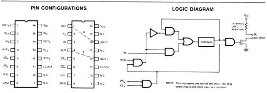
DASH LINES INDICATE NECESSARY EXTERNAL PRINTED CIRCUIT BOARD CONNECTIONS FOR PROPER OPERATION OF THE 2405.
