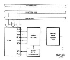
Asynchronous Interface to Telephone Lines
