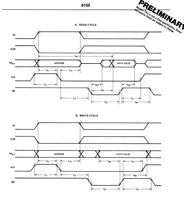
FIGURE 7. 8155 READ/WRITE TIMING DIAGRAM.
