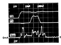
Figure 1. I<sub>DD</sub> transient current during shift cycles.
