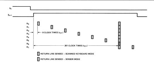
Figure 13. Return Line Timing for Scanned Keyboard and Sensor Mode.
