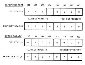
In this example, the In-Service FF corresponding to line 4 (the highest priority FF set) was reset and line 4 became the lowest priority, while all the other priorities rotated correspondingly.
