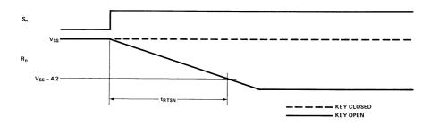
Figure 15. Detailed Timing - Sensor Mode.
