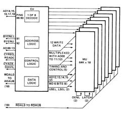
in-1600 Series Block Diagram (Word Length Less Than 9-Bits) in-1600 Series Block Diagram (Word Length More Than 9-Bits)
