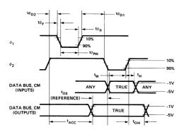
Figure 2. Timing Detail.
