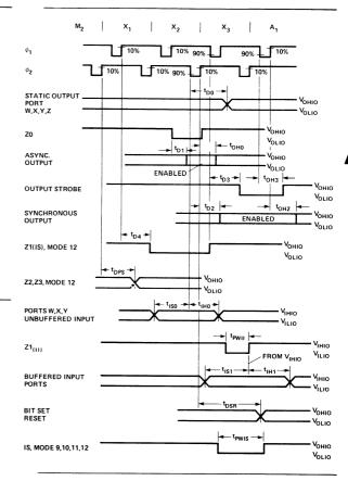
Figure 11. 4265 I/O Timing Diagram.
