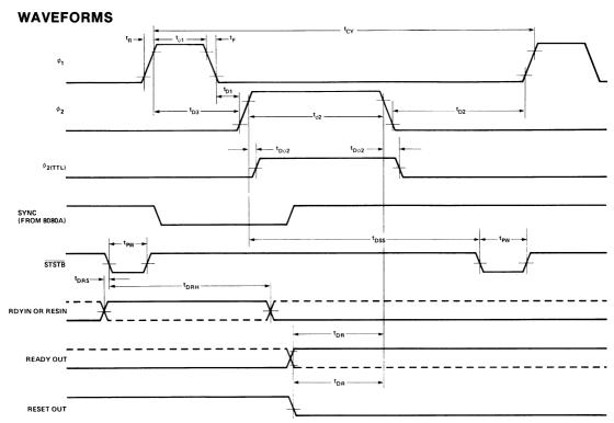
VOLTAGE MEASUREMENT POINTS:  $\phi_1$ ,  $\phi_2$  Logic "0" = 1.0V, Logic "1" = 7.0V. READY, RESET Logic "0" = 0.8V, Logic "1" = 3.0V. All other signals measured at 1.5V.
