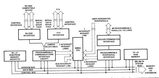
1. Interrupts originating from the Programmable Communications Interface and Programmable Peripheral Interface are jumper selectable.
