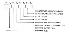
Based on the status of the Status Register, the CPU may Read the Tx Reg, Rx Reg, or Result Register, if more information is needed.
