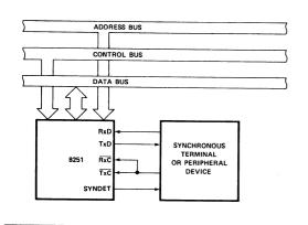
Synchronous Interface to Terminal or Peripheral Device
