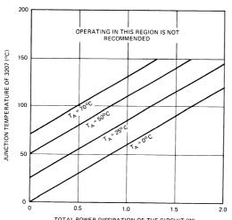
TOTAL POWER DISSIPATION OF THE CIRCUIT (W) TOTAL POWER = D.C. POWER + POWER CONSUMED IN CHARGING AND DISCHARGING LOAD CAPACITANCE.
