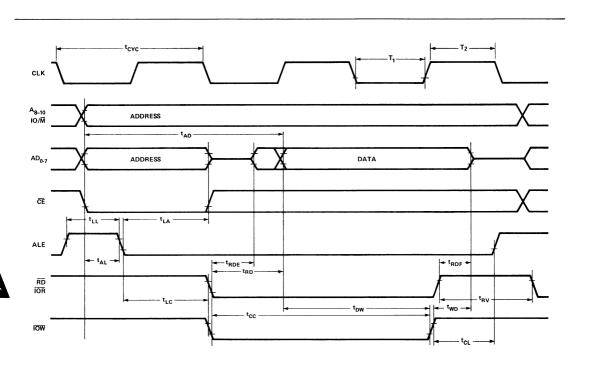
FIGURE 5. ROM READ AND I/O READ AND WRITE.
