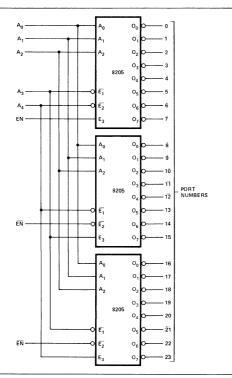
ray of 8205s can be used to create a simple interface to a 24K memory system.
