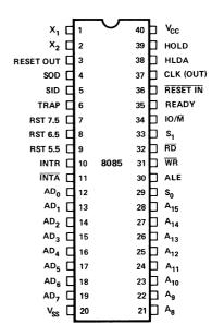
Figure 1. 8085 PINOUT DIAGRAM
