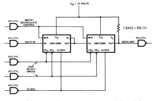
NOTE (1): The 2401/2405 is directly compatible device to device. An external 1.5K $\Omega$  ± 5% load resistor is recommended for driving one TTL load with the 2401/2405 output.
