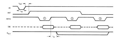
Note: Interrupt acknowledge INTA sequence must remain "HIGH" (at least) until leading edge of first INTA.
