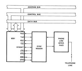
Synchronous Interface to Telephone Lines
