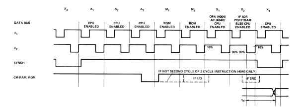
Figure 1. Timing Diagram.
