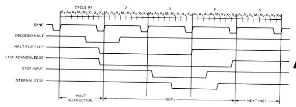
Figure 4. Halt Timing (Exit Using Stop Input).
