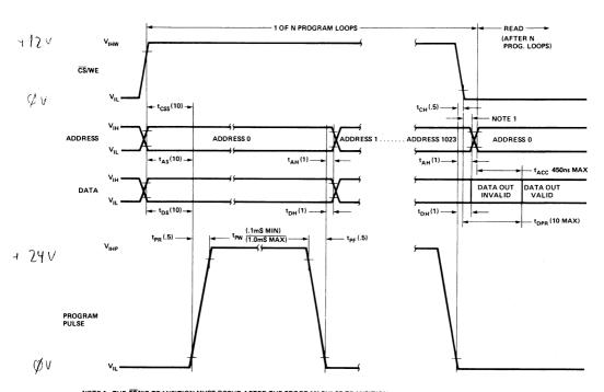
NOTE 1. THE CS/ME TRANSITION MUST OCCUR AFTER THE PROGRAM PULSE TRANSITION AND BEFORE THE ADDRESS TRANSITION. NOTE 2. NUMBERS IN ( ) INDICATE MINIMUM TIMING IN  $\mu$ S UNLESS OTHERWISE SPECIFIED.
