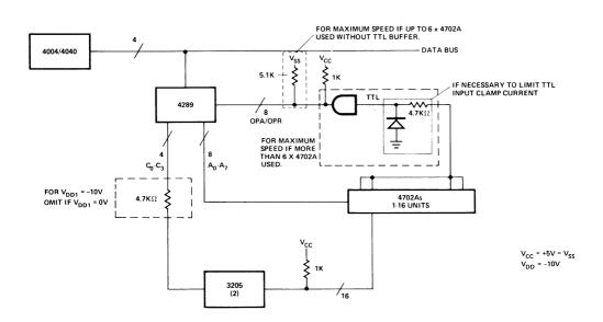
Figure 4. 4289 and 4702A Block Diagram.
