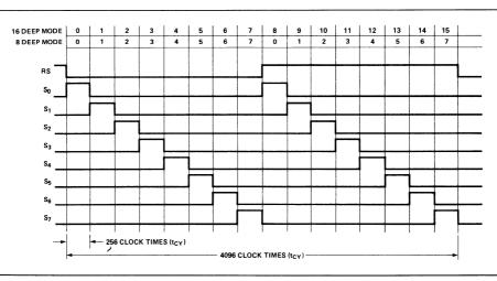
Figure 11. Individually Scanned Display Mode Timing After Execution of 0 or 16 WRM Instruction (or 8 WRMs for 8 Nibbles Deep Mode).
