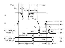
Figure 10. Timing Detail.
