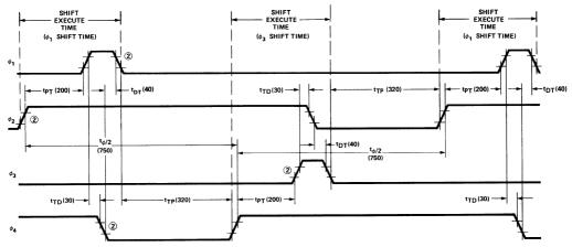
Note: 2. +2.0V and  $V_{DD}$ -2.0V are the reference low and high level respectively for measuring the timing of  $\phi_1$ ,  $\phi_2$ ,  $\phi_3$  and  $\phi_4$ .
