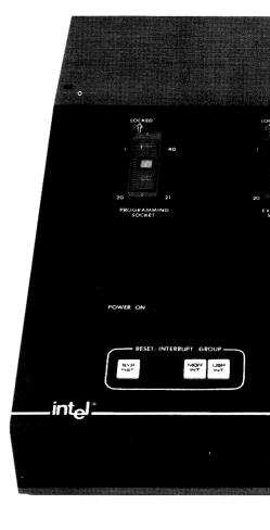
PROMPT 48's **COMMANDS** are grouped and color-coded to simplify access to the 8748's separate program and data memory. You can EXAMINE and MODIFY registers, data memory or program memory.
