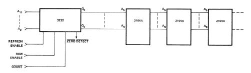
Figure 1. Typical Connection of 3232 and 2104 Memories.
