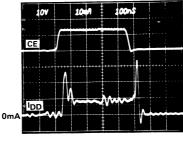
Figure 2.  $I_{\mbox{DD}}$  transient current during I/O cycles.
