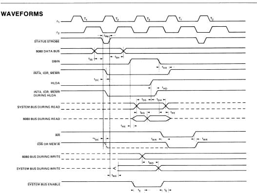
VOLTAGE MEASUREMENT POINTS: D<sub>0</sub>-D<sub>7</sub> (when outputs) Logic "0" = 0.8V, Logic "1" = 3.0V. All other signals measured at 1.5V.
