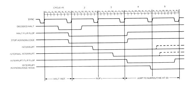
Figure 6. Halt Timing (Exit Using Interrupt).
