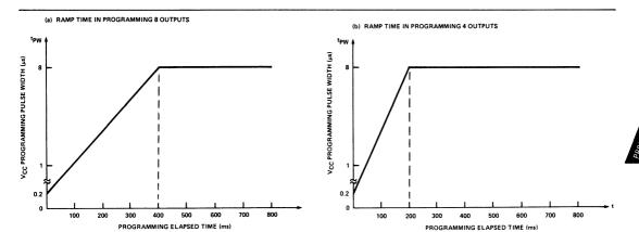
Figure 3. VCC Pulse Width vs. Programming Time.
