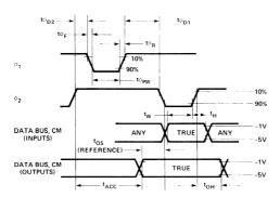
Figure 2. Timing Detail.
