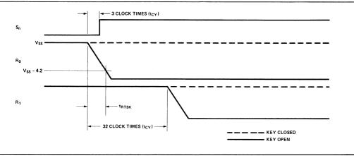
Figure 14. Detailed Timing - Scanned Keyboard Mode.
