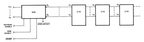
Figure 1. Typical Connection of 3242 and 2116 Memories.
