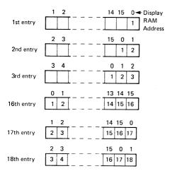
Note that now the display position and register address do not correspond. Consequently, entering a character to an arbitrary position in the Auto Increment mode may have unexpected results. Entry starting at Display RAM address 0 with sequential entry is recommended.
