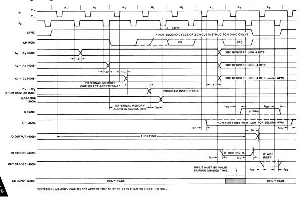
Figure 1. 4008 and 4009 Timing Diagram.
