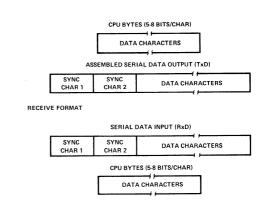
Synchronous Mode, Transmission Format
