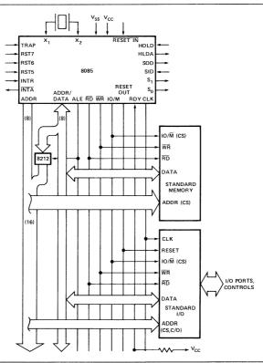
FIGURE 8. MCS-85™ MINIMUM SYSTEM (USING STANDARD MEMORIES)
