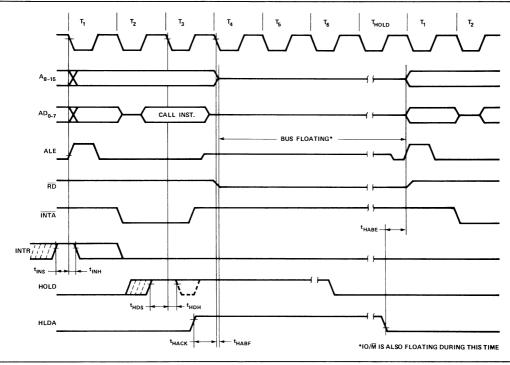
FIGURE 5. 8085 INTERRUPT AND HOLD TIMING
