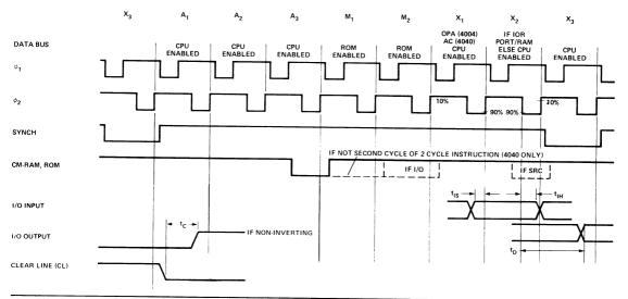
Figure 1. Timing Diagram
