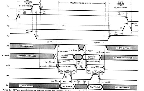
Notes: 2. +2.0V and  $V_{DD}$ -2.0V are the reference low and high level respectively for measuring the timing of  $\phi_1 \dots \phi_4$ , CE, CS, WE, and addresses.
