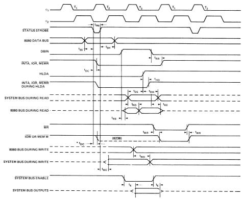
VOLTAGE MEASUREMENT POINTS:  $D_0$ - $D_7$  (when outputs) Logic "0" = 0.8V, Logic "1" = 3.0V. All other signals measured at 1.5V.
