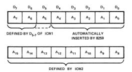
A0-4 are automatically inserted by the 8259, while A15-6 are programmed by ICW1 and ICW2. When interval = 8, A5 is fixed by the 8259. If interval = 4, A5 is programmed in ICW1. Thus, the interrupt service routines can be located anywhere in the memory space. The 8 byte interval will maintain compatibility with current 8080 RESTART instruction software, while the 4 byte interval is best for compact jump table.
