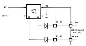
NOTE THAT ISOLATION DIODES MUST BE PLACED IN THE SCAN LINES AS SHOWN IF THE SCAN LINES ARE ALSO USED TO STROBE A DISPLAY. IF THE KEYBOARD USED HAS A DIODE AT EACH KEY, THEN THE SCAN LINE ISOLATION DIODES ARE NOT REQUIRED.
