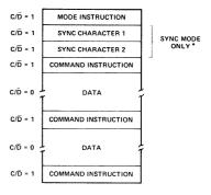
\*The second SYNC character is skipped if MODE instruction has programmed the 8251 to single character Internal SYNC Mode. Both SYNC characters are skipped if MODE instruction has programmed the 8251 to ASYNC mode.
