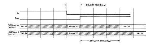
Figure 12. Individually Scanned Display Mode.
