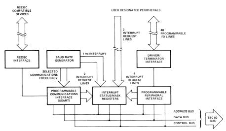
NOTES: INTERRUPTS ORIGINATING FROM THE PROGRAMMABLE COMMUNICATIONS INTERFACE AND PROGRAMMABLE PERIPHERAL INTERFACE ARE JUMPER-SELECTABLE.
