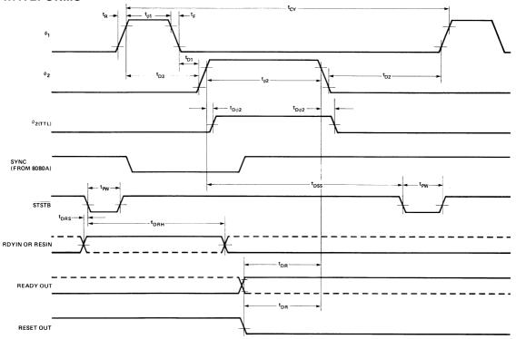
VOLTAGE MEASUREMENT POINTS:  $\phi_1$ ,  $\phi_2$  Logic "0" = 1.0V, Logic "1" = 8.0V. All other signals measured at 1.5V.
