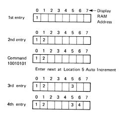
In the Right Entry mode, Auto Incrementing and non Incrementing have the same effect as in the Left Entry except if the address sequence is interrupted:
