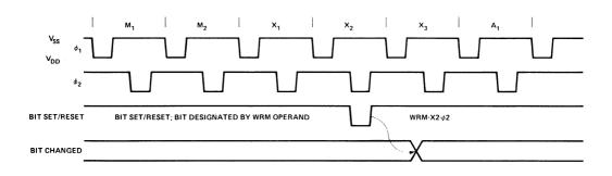
Figure 8. Bit Set/Reset Operation Timing.
