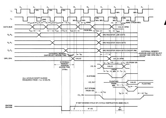
Figure 7. MCS-40 Timing Diagram for 4289.
