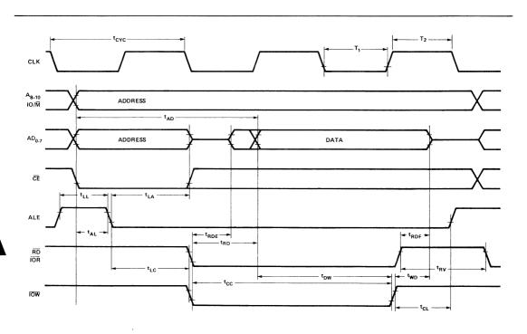
FIGURE 4. PROM READ AND I/O WRITE TIMING.
