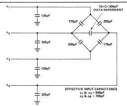
Figure 2. 2416 Equivalent Capacitance Circuit. (Maximum values shown.)
