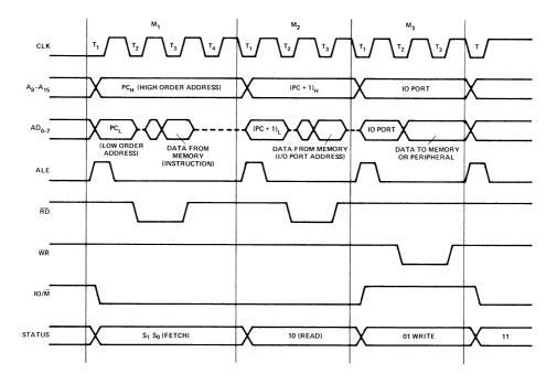
FIGURE 2. 8085 BASIC SYSTEM TIMING.
