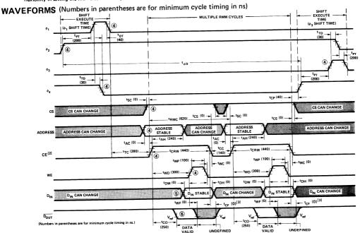
Notes: 2. When CE is off, the 2416 output level is determined by the external output termination.
