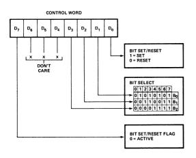
When Port C is being used as status/control for Port A or B, these bits can be set or reset by using the Bit Set/Reset operation just as if they were data output ports.
