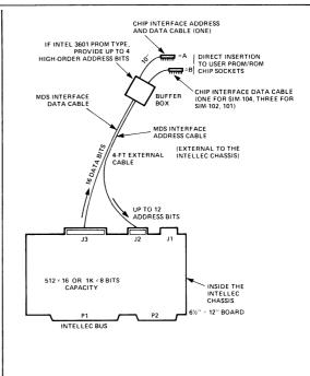
Fig. 1. Data Flow of ROM-SIM Module
