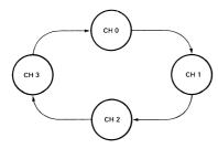
If the ROTATING PRIORITY bit is not set (set to a zero), each DMA channel has a fixed priority. In the fixed priority mode, Channel 0 has the highest priority and Channel 3 has the lowest priority. If the ROTATING PRIORITY bit is set to a one, the priority of each channel changes after each DMA cycle (not each DMA request). Each channel moves up to the next highest priority assignment, while the channel which has just been serviced moves to the lowest priority assignment:
