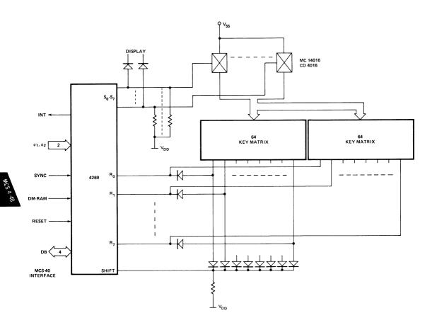
Figure 7. 128 Scanned Input Keys.
