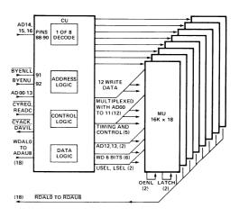
in-40 Series Block Diagram (Word Length Less Than 9-Bits) in-40 Series Block Diagram (Word Length More Than 9-Bits)
