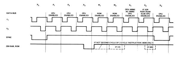
Figure 9. Timing Diagram.
