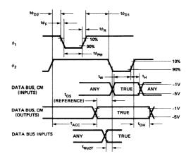
Figure 3. Timing Detail.
