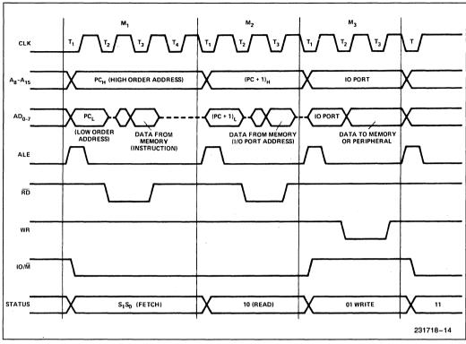
Figure 10. 8085AH Basic System Timing
