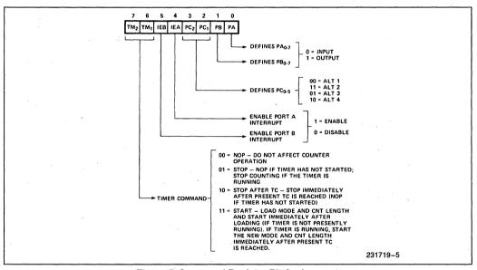
Figure 5. Command Register Bit Assignment
