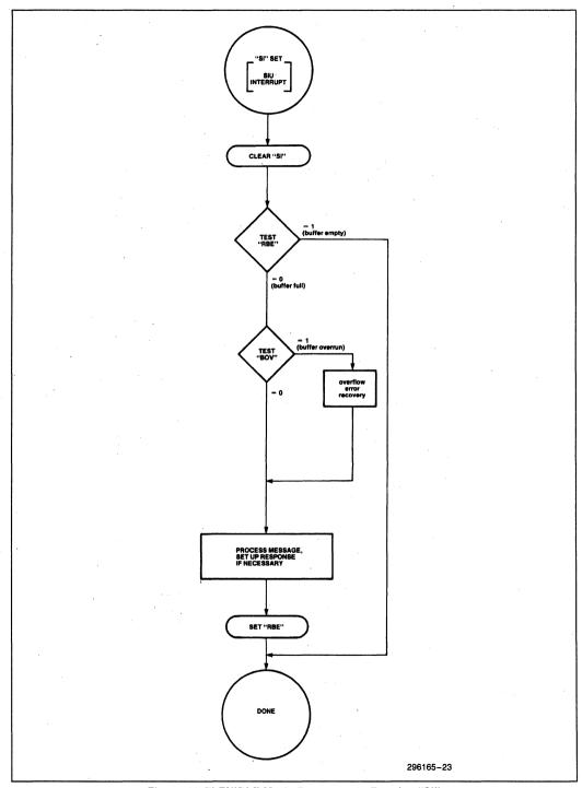
Figure 11. FLEXIBLE Mode Response to Receive "SI"
