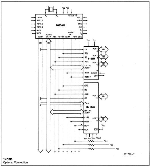
Figure 7. 8085AH Minimum System (Standard I/O Technique)
