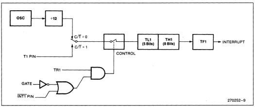
Figure 7. Timer/Counter 1 Mode 0: 13-Bit Counter
