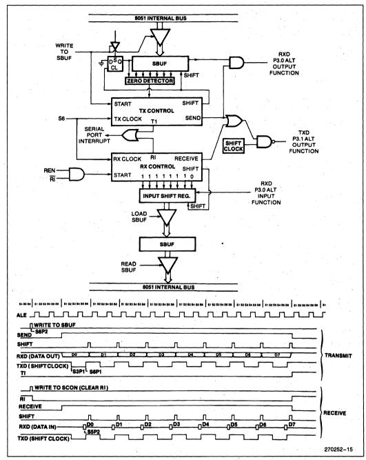
Figure 17. Serial Port Mode 0
