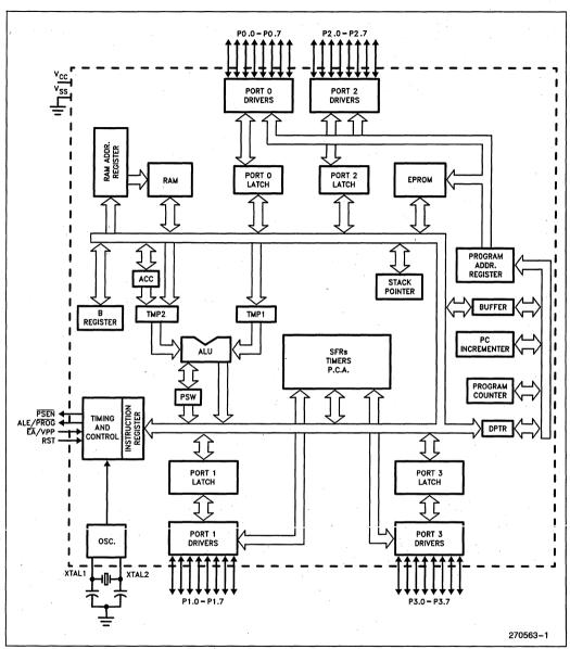
Figure 1. 87C51FB Block Diagram
