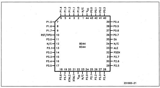
Figure 3B. PLCC Pin Configuration
