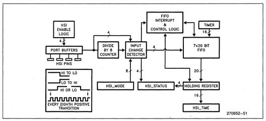
Figure 27. High Speed Input Unit
