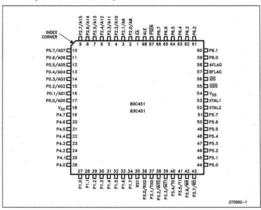
Figure 1. Pin Connections (PLCC)
