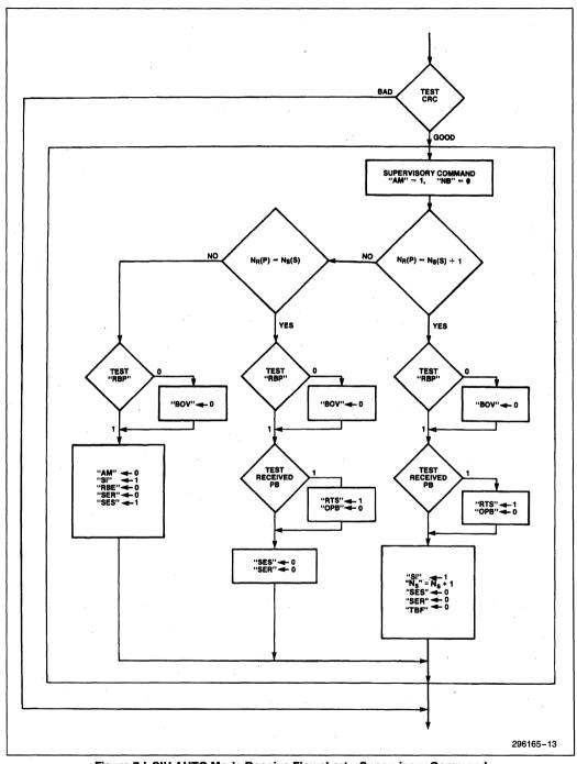
Figure 7d. SIU AUTO Mode Receive Flowchart—Supervisory Command
