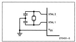
Figure 3. Using the On-Chip Oscillator
