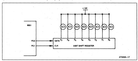
Figure 17. Output Expansion Using Serial Port
