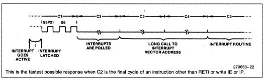
Figure 25. Interrupt Response Timing Diagram
