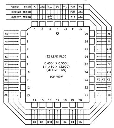
Figure 3. PLCC Lead Configuration
