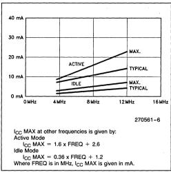
Figure 6. I<sub>CC</sub> vs Frequency. Valid only within frequency specifications of the device under test.
