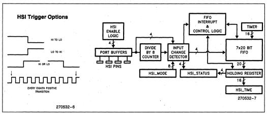
Figure 7. High Speed Input Unit
