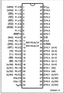
Figure 2.5A. DIP Pin Out
