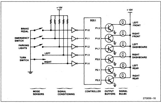
Figure 16. Microcomputer Turn-Signal Connections
