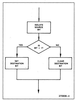
Figure 8. Bit Transfer Instruction Operation
