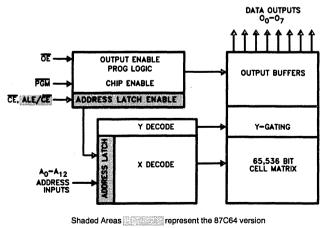
Figure 1. Block Diagram
