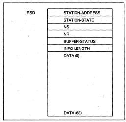
Figure 16. Remote Station Database Structure
