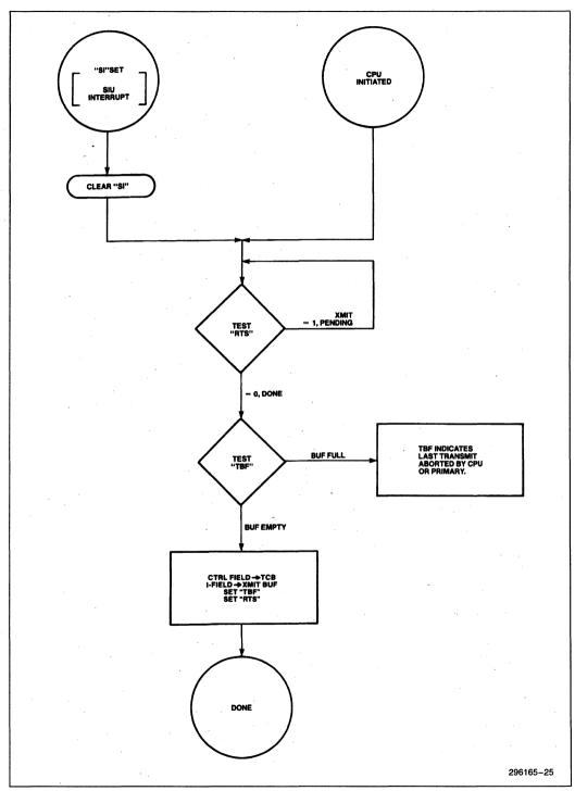
Figure 13. FLEXIBLE Mode Response to Transmit "SI"
