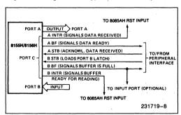
Figure 9. Example: Command Register = 00111001
