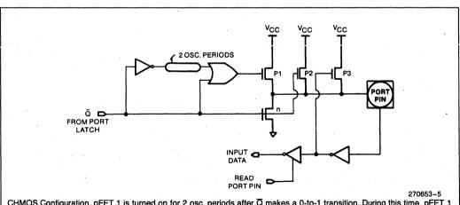
CHMOS Configuration. pFET 1 is turned on for 2 osc. periods after  $\overline{Q}$  makes a 0-to-1 transition. During this time, pFET 1 also turns on pFET 3 through the inverter to form a latch which holds the 1. pFET 2 is also on. Port 2 is similar except that it holds the strong pullup on while emitting 1s that are address bits. (See text, "Accessing External Memory".)
