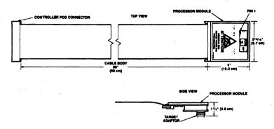
Figure 1: Processor Module Dimensions
