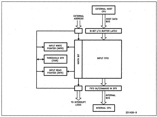
Figure 5. Input FIFO Channel Functional Block Diagram
