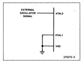
Figure 4. External Drive Configuration
