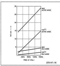
Figure 5. I<sub>CC</sub> vs. FREQ. Valid only within frequency specifications of the device under test.
