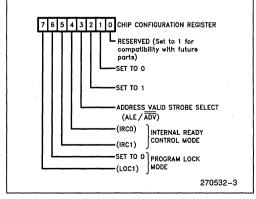
Figure 4. Chip Configuration Register
