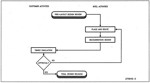
Figure 4. Layout and Verification Phase Flowchart
