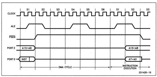
Figure 11. DMA Transfer from Internal Memory to Internal Memory
