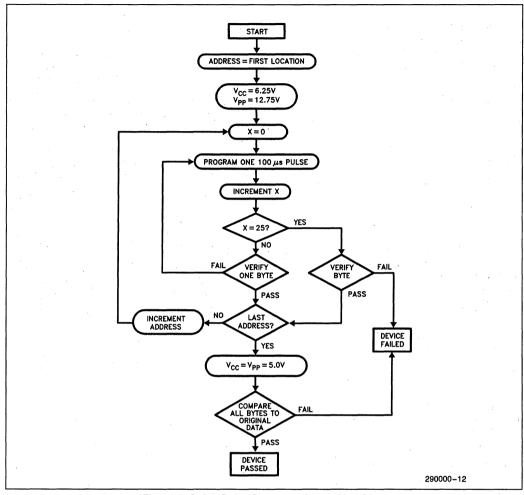
Figure 5. Quick-Pulse Programming™ Algorithm
