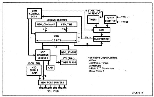
Figure 8. High Speed Output Unit
