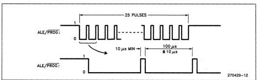
Figure 6. PROG Waveforms
