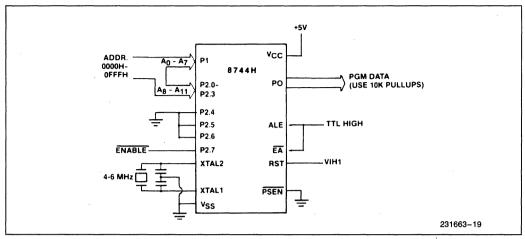
Figure 10. Program Verification Configuration
