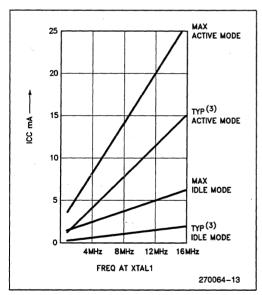
Figure 5. I<sub>CC</sub> vs. Frequency. Valid only within frequency specifications of the device under test.
