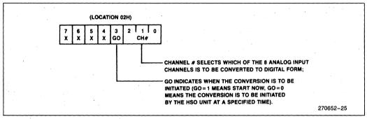
Figure 33. A/D Command Register
