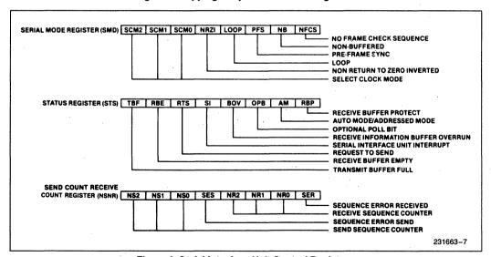
Figure 6. Serial Interface Unit Control Registers
