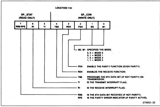
Figure 40. Serial Port Control/Status Register
