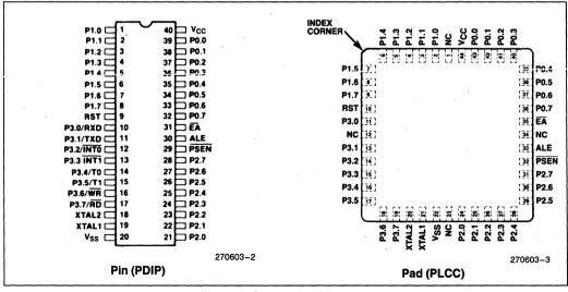
**Figure 2. Connection Diagrams**
