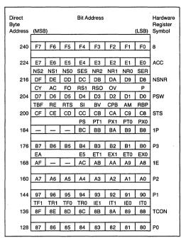
Figure 7. Special Function Register Bit Address
