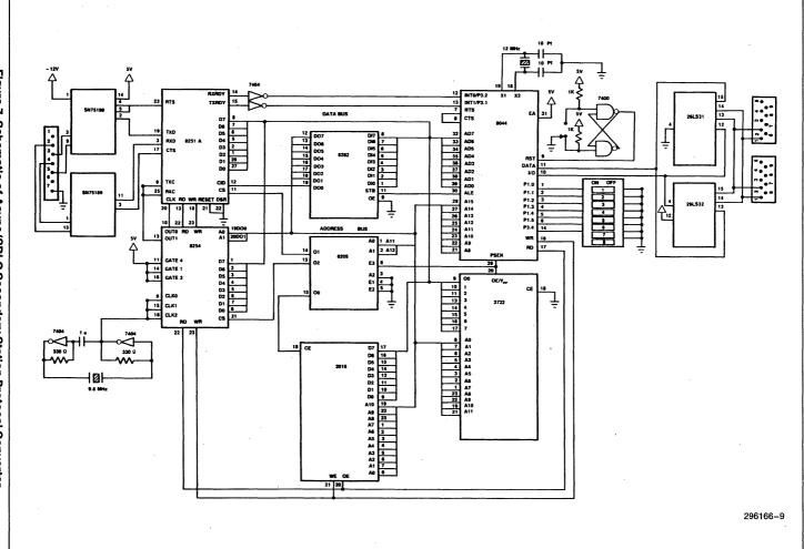
Figure 7. Schematic of Async/SDLC Secondary Station Protocol Converter
