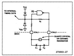
Figure 30. Using the CHMOS On-Chip Oscillator
