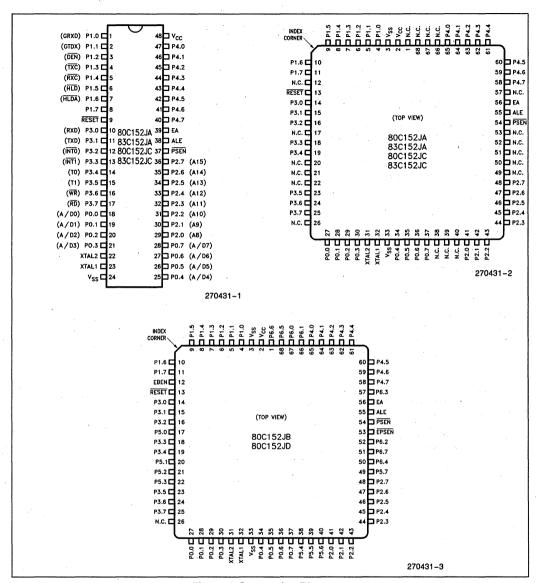
Figure 1. Connection Diagrams
