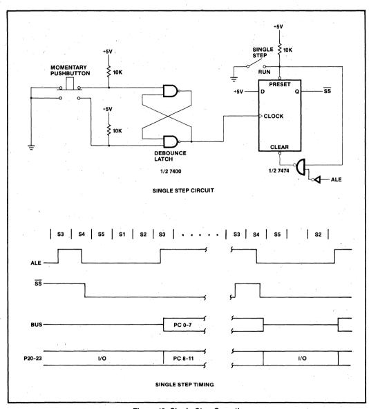
Figure 13. Single Step Operation
