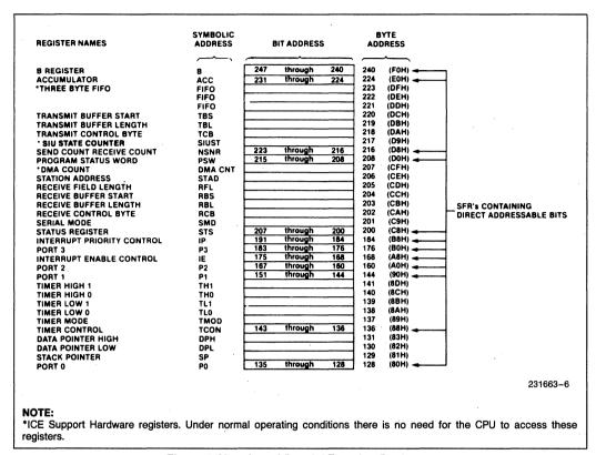
Figure 5. Mapping of Special Function Registers
