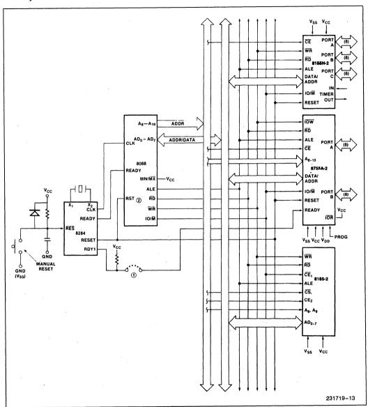
Figure 13b. 8088 Five Chip System Configuration
