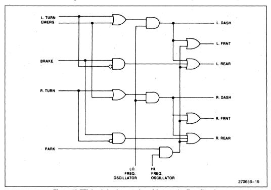
Figure 15. TTL Logic Implementation of Automotive Turn Signals
