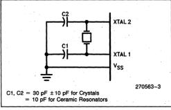
Figure 3. Oscillator Connections
