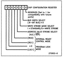
Figure 10. Chip Configuration Register
