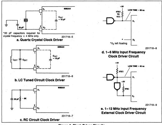
**Figure 5. Clock Driver Circuits**
