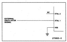
Figure 4. External Drive Configuration
