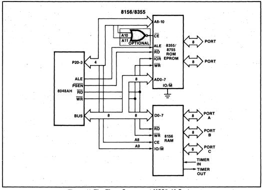
Figure 11. The Three-Component MCS®-48 System
