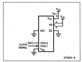
Figure 7. I<sub>CC</sub> Test Condition, Idle Mode. All other pins are disconnected.
