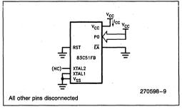
Figure 8.  $I_{CC}$  Test Condition, Power Down Mode.  $V_{CC} = 2.0V$  to 5.5V.
