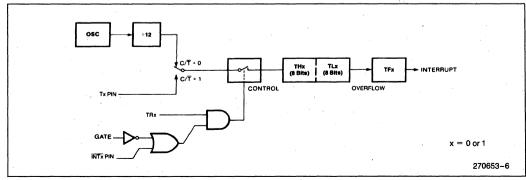
Figure 8. Timer/Counter 0 or 1 in Mode 0: 13-Bit Counter
