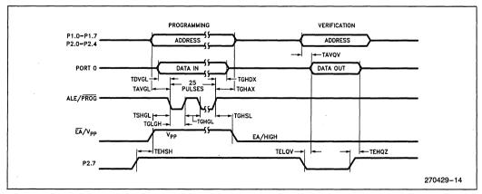
**EPROM Programming and Verification Waveforms**
