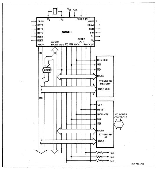
Figure 9. 8085 System (Using Standard Memories)
