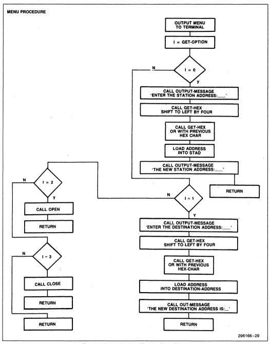
Figure 27. Application Module Flow Chart
