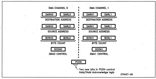
Figure 4.1. DMA Registers
