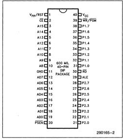
Figure 2. 40-Pin Dip Package
