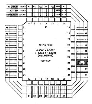
Figure 3. PLCC(N) Lead Configuration
