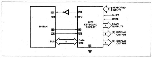
Figure 8. Keyboard/Display Interface
