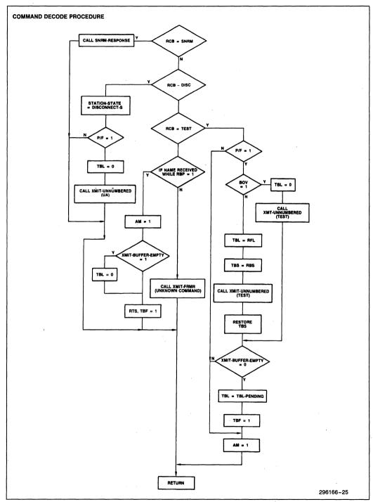
Figure 23. Secondary Station Driver Flow Chart
