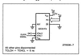
Figure 7. I<sub>CC</sub> Test Condition Idle Mode
