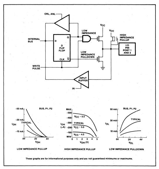
Figure 4. "Quasi-bidirectional" Port Structure
