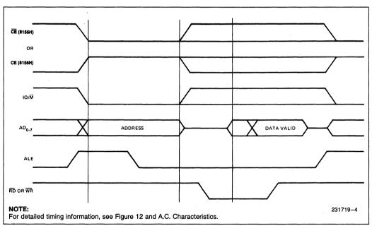
Figure 4. 8155H/8156H On-Board Memory Read/Write Cycle
