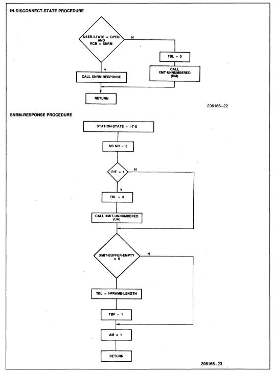
Figure 21. Secondary Station Driver Flow Chart
