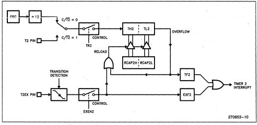
Figure 13. Timer 2 Auto Reload Mode (DCEN = 0)
