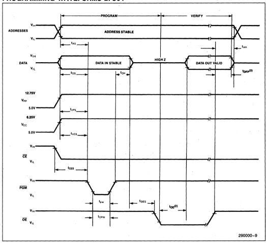
The Input Timing Reference Level is 0.8V for V<sub>IL</sub> and 2V for a V<sub>IH</sub>.
