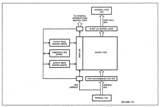
Figure 6. Output FIFO Channel Functional Block Diagram
