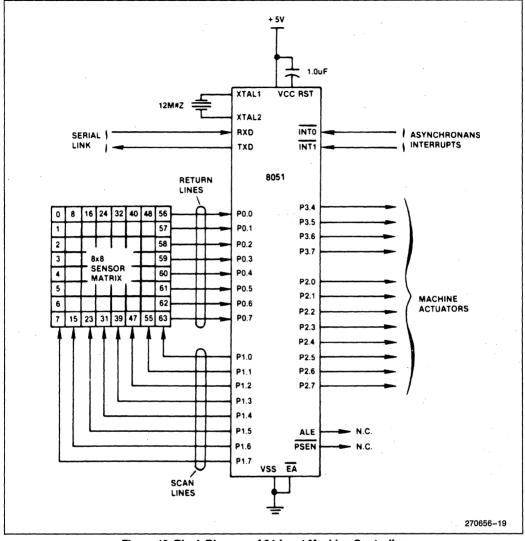
Figure 19. Block Diagram of 64-input Machine Controller
