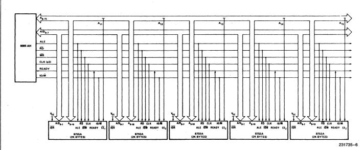
NOTE: Use  $\overline{\text{CE}_1}$  for the first 8755A in the system, and  $\text{CE}_2$  for the other 8755A's. Permits up to 5-8755A's in a system without CE decoder.
