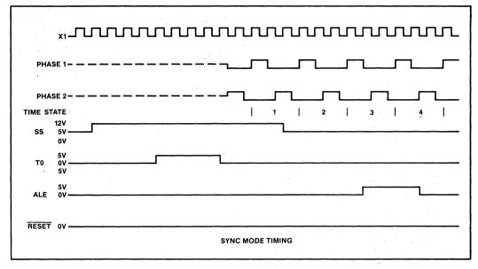
Figure 15. Sync Mode Timing
