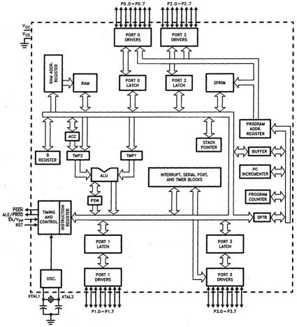
Figure 1. 8751BH Block Diagram
