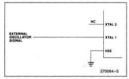
Figure 4. External Drive Configuration
