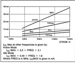
Figure 5. I<sub>CC</sub> vs Frequency
