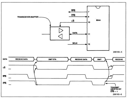
Figure 3. Serial Interface Timing—Clocked Mode
