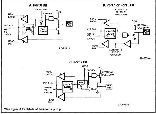
Figure 2. 8XC51FA/FB Port Bit Latches and I/O Buffers
