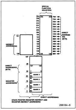
Figure 10. Addressing Operands in Internal Data Memory
