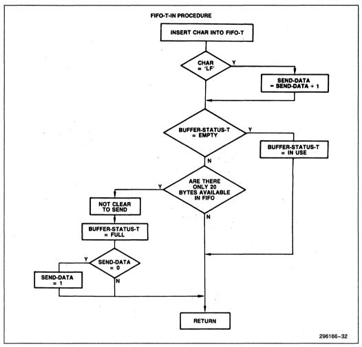
Figure 30. Application Module Flow Chart
