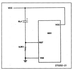
Figure 26. Power on Reset Circuit
