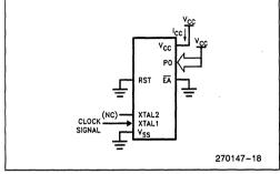
Figure 7. I<sub>CC</sub> Test Condition, Idle Mode. All other pins are disconnected.
