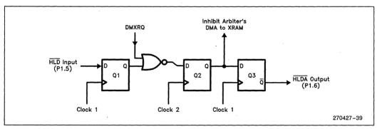
Figure 4.8. Internal Logic of the Arbiter
