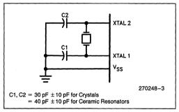
Figure 3. Oscillator Connections
