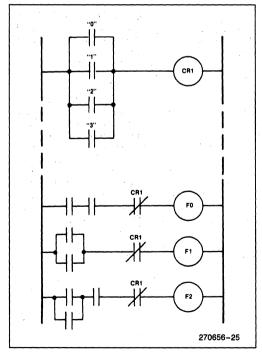
Figure 22. Ladder Diagram for Output Override Circuitry
