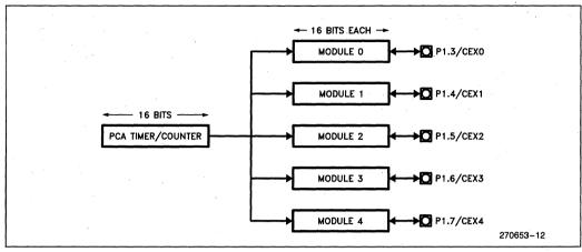
Figure 15. Programmable Counter Array
