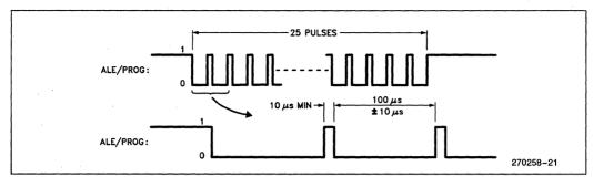
Figure 11. PROG Waveforms
