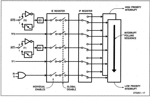
Figure 19. 8051 Interrupt Control System
