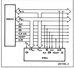
Figure 3. 8755A in 8085AH System (Memory-Mapped I/O)
