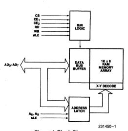
Figure 1. Block Diagram
