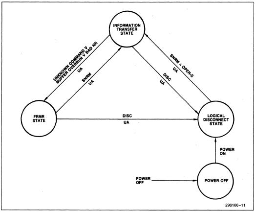
Figure 9. State Diagram of Secondary Station
