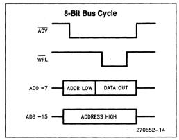
Figure 15. Write Strobe with Address Valid Strobe
