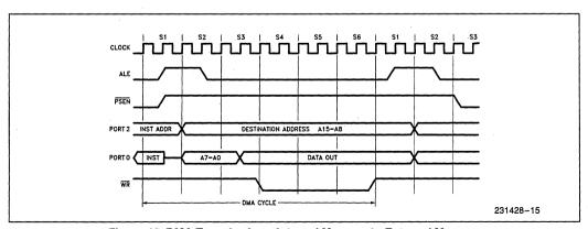
Figure 10. DMA Transfer from Internal Memory to External Memory
