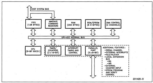
Figure 4. UPI-452 Functional Block Diagram
