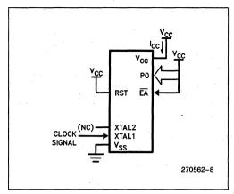
Figure 7. I<sub>CC</sub> Test Condition, Active Mode.
