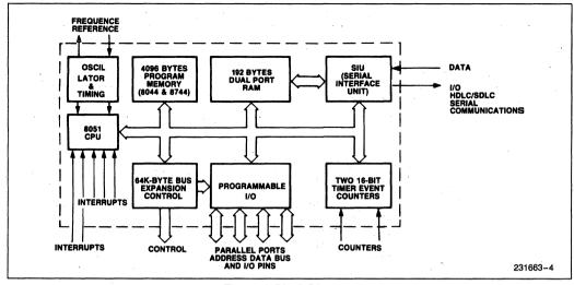
Figure 4. Block Diagram
