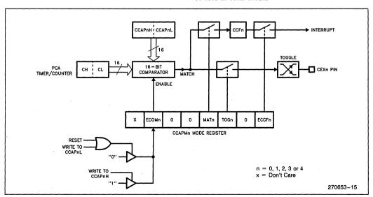
Figure 18. PCA 16-Bit Comparator Mode: Software Timer and High Speed Output
