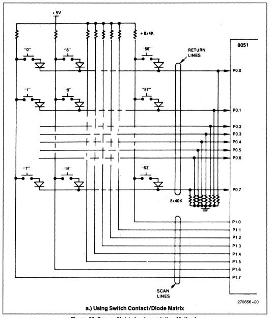
Figure 20. Sensor Matrix Implementation Methods
