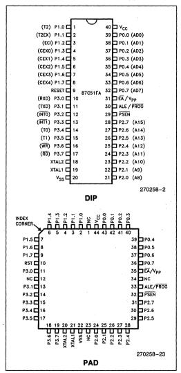
Figure 2. Pin Connections
