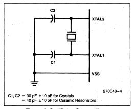
**Figure 3. Oscillator Connections**
