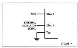
Figure 4. External Clock Drive Configuration
