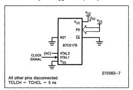
Figure 7. I<sub>CC</sub> Test Condition Idle Mode
