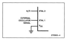
Figure 4. External Clock Drive Configuration
