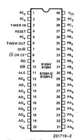
Figure 2. Pin Configuration
