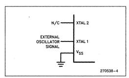
Figure 4. External Clock Drive Configuration
