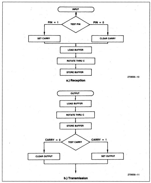
Figure 12. Serial I/O Algorithms
