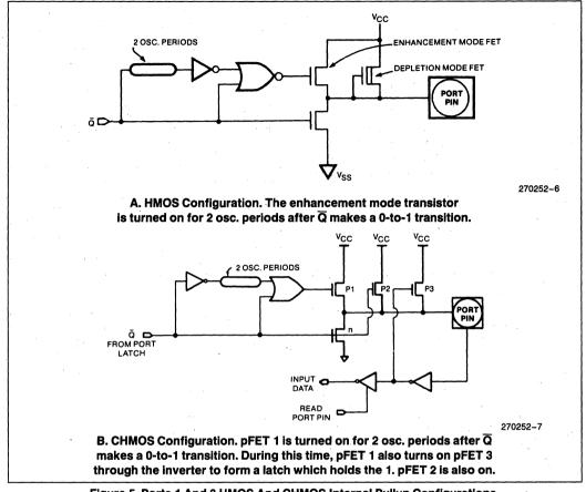
Figure 5. Ports 1 And 3 HMOS And CHMOS Internal Pullup Configurations.
