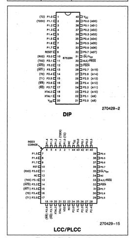
Figure 2. Pin Connections
