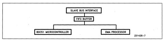
Figure 3. UPI-452 Conceptual Block Diagram
