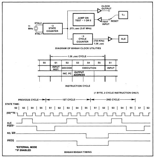
Figure 10. MCS®-48 Timing Generation and Cycle Timing
