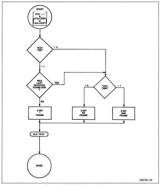
Figure 8. SIU AUTO Mode Transmit Flowchart
