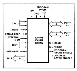
Figure 16. 8048AH and 8049AH Logic Symbol
