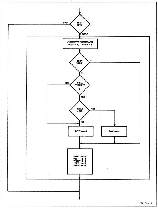
Figure 7b. SIU AUTO Mode Receive Flowchart—Unknown Command
