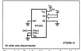
Figure 8. I<sub>CC</sub> Test Condition, Power Down Mode.  $V_{CC} = 2.0V \text{ to 5.5V}.$
