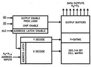
Figure 1. Block Diagram
