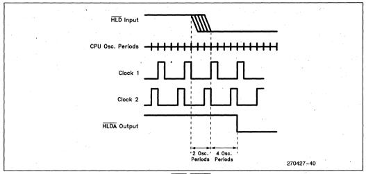
Figure 4.9. Minimum HLD/HLDA Response Time
