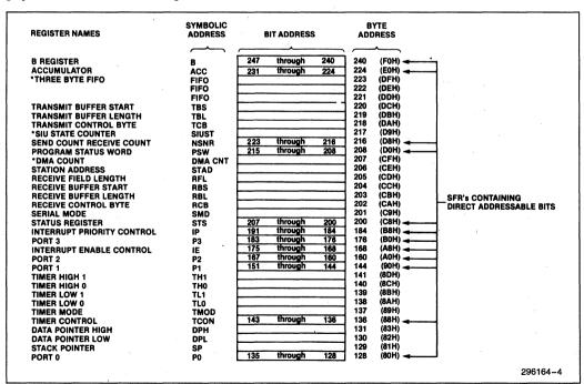
Figure 6. Mapping of Special Function Registers
