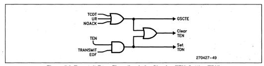
Figure 5.2. Transmit Error Flags (Logic for Clearing TEN, Setting TDN)
