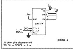
Figure 6. I<sub>CC</sub> Test Condition, Active Mode
