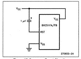
Figure 27. Power on Reset Circuitry
