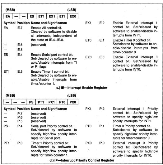
Figure 7. Peripheral Configuration Registers (Continued)
