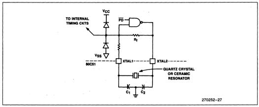
Figure 34. Using the CHMOS On-Chip Oscillator
