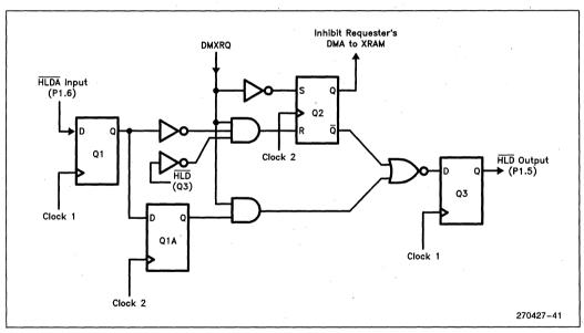
Figure 4.10. Internal Logic of the Requester (Clock 1 and Clock 2 are Shown in Figure 4.9)
