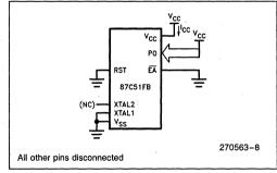
Figure 8.  $I_{CC}$  Test Condition, Power Down Mode.  $V_{CC}=2.0V$  to 5.5V.
