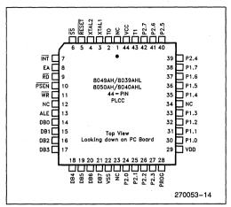
Figure 3. Pin Configuration
