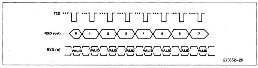
Figure 37. Serial Port Mode 0 Timing
