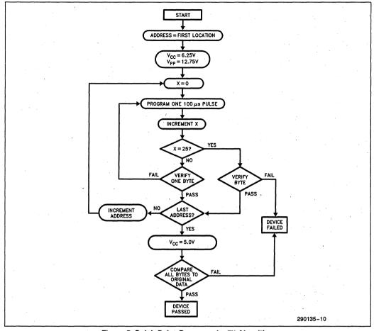
Figure 5. Quick-Pulse Programming™ Algorithm
