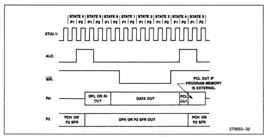
Figure 7. External Data Memory Write Cycle
