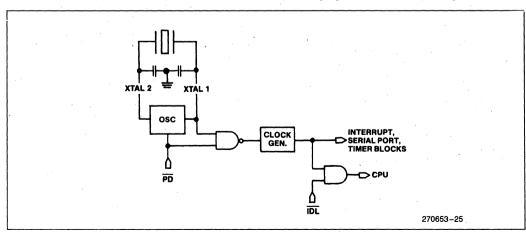
Figure 28. Idle and Power Down Hardware
