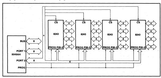
Figure 9. Low Cost I/O Expansion
