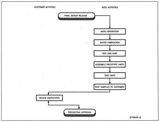
Figure 5. Manufacturing Phase Flowchart
