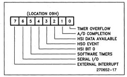
Figure 24. Interrupt Pending Register
