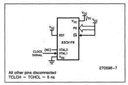
Figure 6. I<sub>CC</sub> Test Condition, Active Mode
