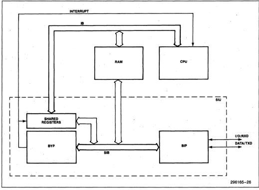
Figure 14. The Bit and Byte Processors
