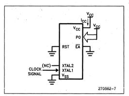
Figure 8. I<sub>CC</sub> Test Condition, Idle Mode. All other pins are disconnected.
