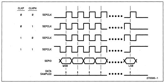
Figure 5. SEP Clock Waveforms
