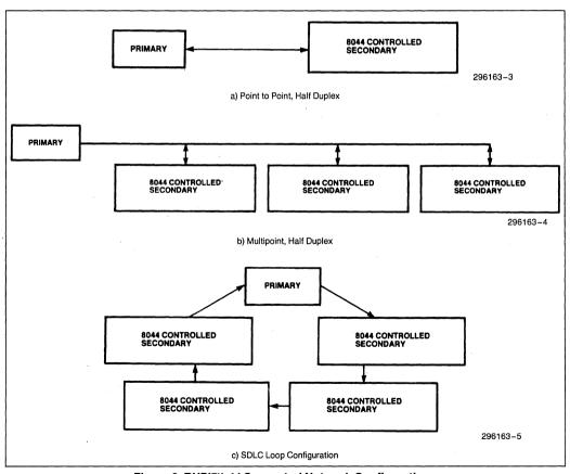
Figure 3. RUPI™-44 Supported Network Configurations
