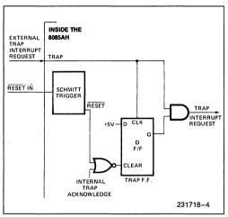
Figure 4. TRAP and RESET In Circuit
