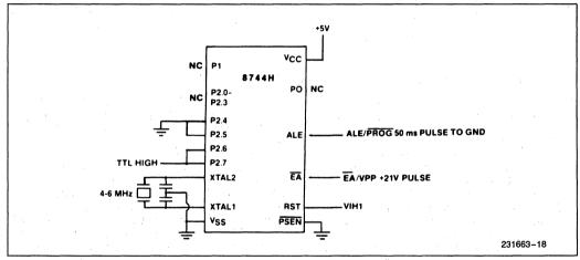
Figure 9. Security Bit Programming Configuration
