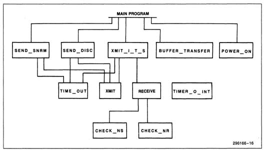
Figure 17. Block Diagram of Primary Station Software Structure
