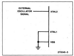
**Figure 4. External Drive Configuration**
