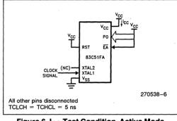
Figure 6. I<sub>CC</sub> Test Condition, Active Mode
