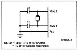
Figure 3. Oscillator Connections
