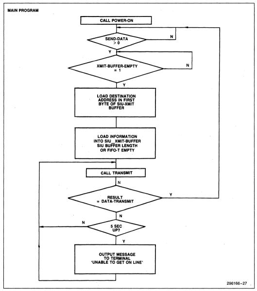
Figure 25. Application Module Flow Chart
