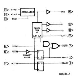
Figure 1. Block Diagram
