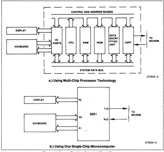
Figure 11. Secure Banking Terminal Block Diagram
