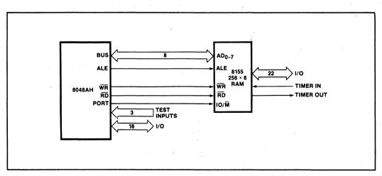
Figure 6. 8048AH Interface to 256 x 8 Standard Memories
