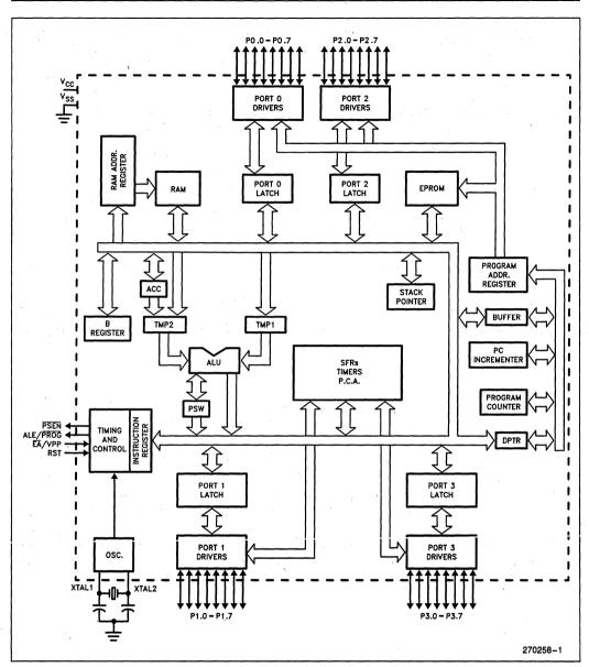
Figure 1. 87C51FA Block Diagram
