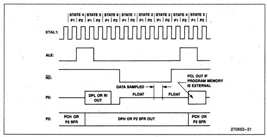
Figure 6. External Data Memory Read Cycle
