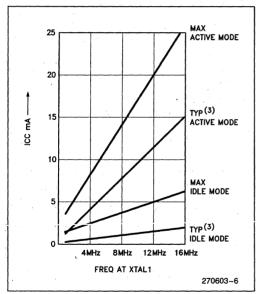
Figure 5. I<sub>CC</sub> vs. Frequency.
