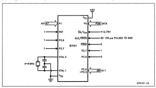
Figure 10. Programming Configuration
