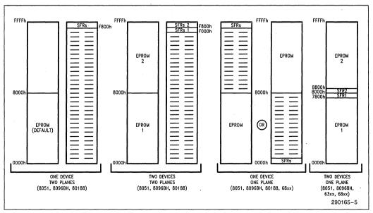
Figure 5. A Few Possible Memory Plane Configurations
