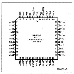
Figure 3. 44-Lead PLCC Package
