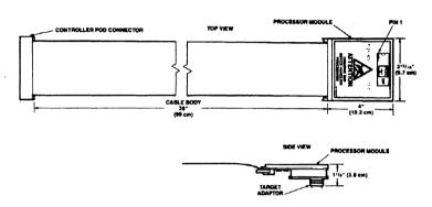
Figure 1: Processor Module Dimensions
