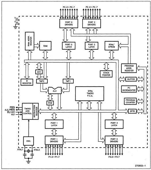
Figure 1. 8XC51FA/FB Functional Block Diagram
