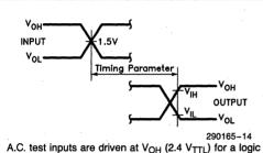
A.C. test inputs are driven at V $_{OH}$  (2.4 V $_{TTL}$ ) for a logic "1" and V $_{OL}$  (0.45 V $_{TTL}$ ) for a logic "0". Input timing begins at 1.5V. Output timing ends at V $_{IH}$  (2.0 V $_{TTL}$ ) and V $_{IL}$
