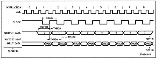
**Shift Register Mode Timing Waveforms**
