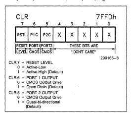
Figure 8. Control Level Register (CLR)
