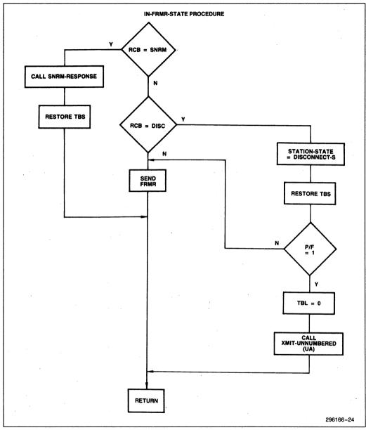
Figure 22. Secondary Station Driver Flow Chart
