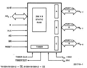
Figure 1. Block Diagram
