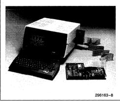
Figure 6. RUPI-44 iPDS Personal Development System, EMV-44 Buffer Box, and EMV-44 Module Plugged into a User Prototype Board
