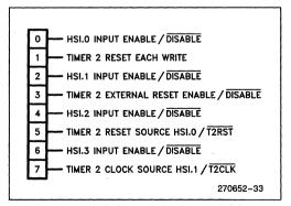
Figure 44. I/O Control Register 0 (IOC0)
