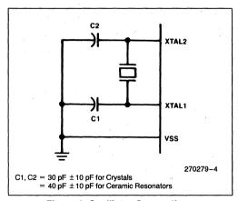
**Figure 3. Oscillator Connections**
