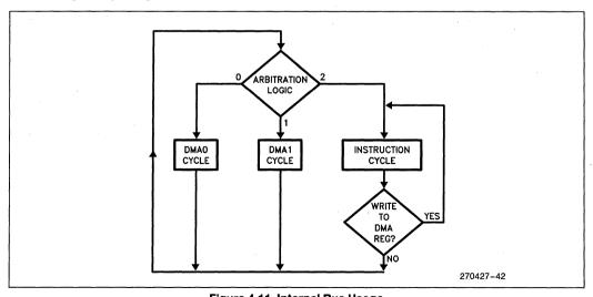
Figure 4.11. Internal Bus Usage
