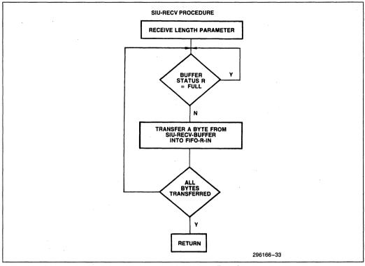
Figure 31. Application Module Flow Chart
