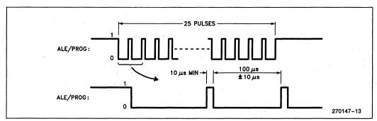
Figure 11. PROG Waveforms
