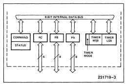
Figure 3. 8155H/8156H Internal Registers
