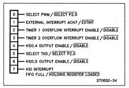
Figure 45. I/O Control Register 1 (IOC1)
