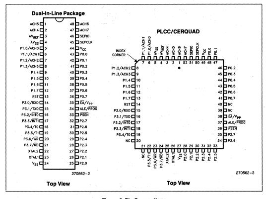
Figure 2. Pin Connections
