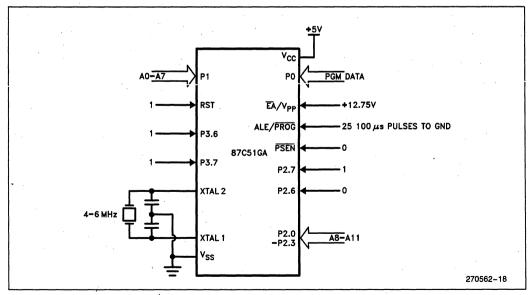
Figure 11. Programming Configuration
