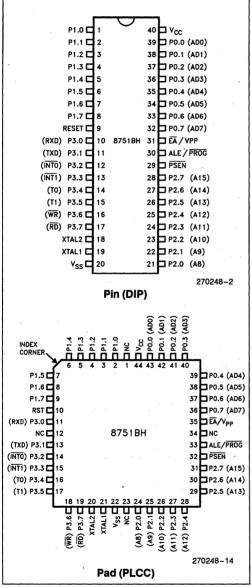
Figure 2. Pin Connections
