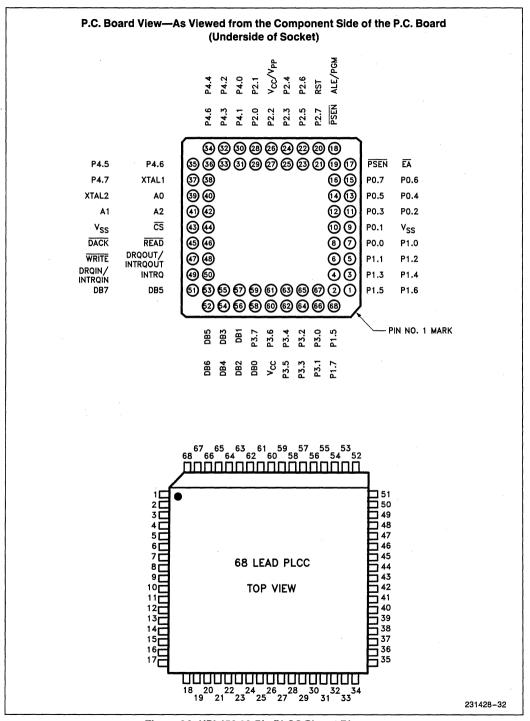
Figure 2A. UPI 452 68-Pin PLCC Pinout Diagram
