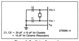
Figure 3. Oscillator Connections
