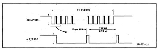
Figure 11. PROG Waveforms
