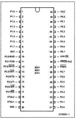
Figure 1. 8051 Family Pinout Diagram
