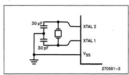
Figure 3. Using the On-Chip Oscillator
