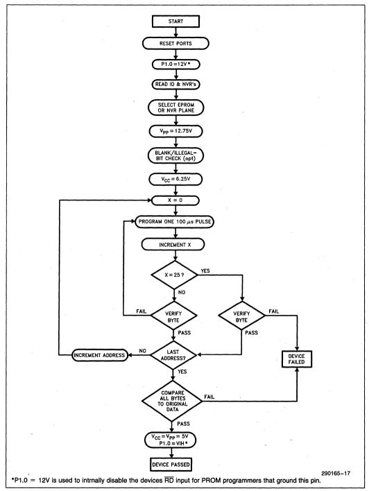
Figure 14. 87C75PF Quick-Pulse Programming<sup>TM</sup> Algorithm
