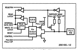
Figure 12. Port 2 Pin Diagram
