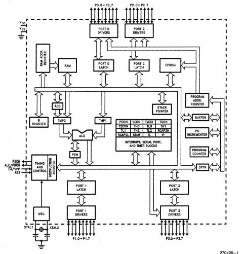
Figure 1. Block Diagram
