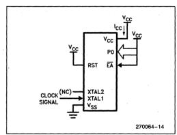
Figure 6. I<sub>CC</sub> Test Condition, Active Mode. All other pins are disconnected.
