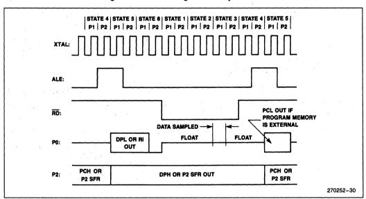
Figure 37. External Data Memory Read Cycle
