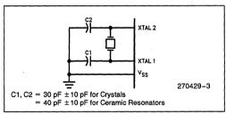
Figure 3. Oscillator Connections
