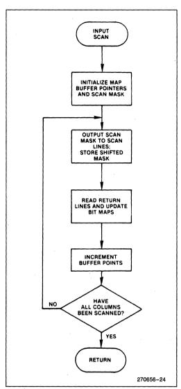
Figure 21. Flowchart for Reading in Sensor Matrix
