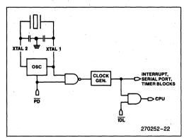
Figure 27. Idle and Power Down Hardware
