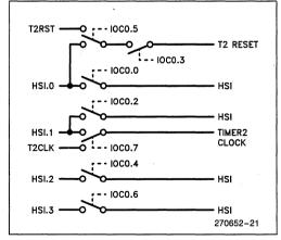
Figure 29. IOC0 Control of HSI Pin Functions
