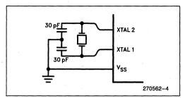
Figure 3. Using the On-Chip Oscillator
