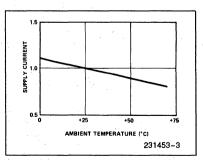
Typical Supply Current vs Temperature, Normalized  $\Delta I$  Supply/ $\Delta T_A = -0.45\%$ °C
