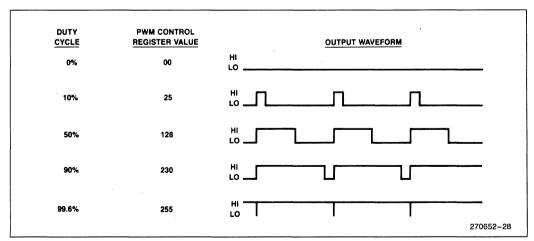
Figure 36. Typical PWM Outputs
