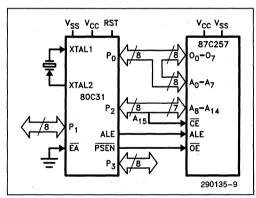
Figure 4. 80C31 with 87C257 System Configuration
