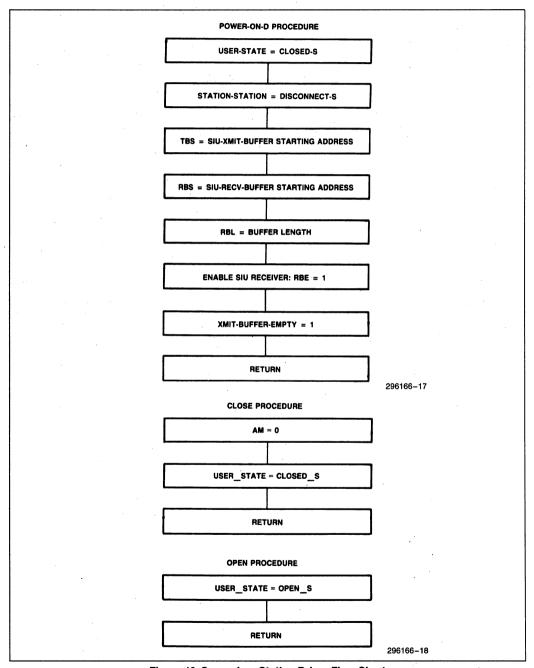
Figure 18. Secondary Station Driver Flow Chart
