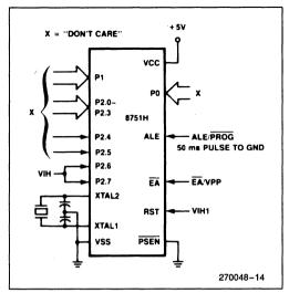
Figure 7. Programming the Security Bit
