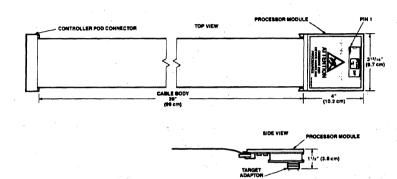
Figure 1. Processor Module Dimensions
