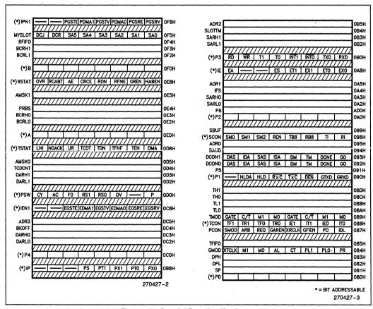
Figure 2.2. Special Function Registers
