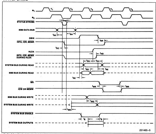
VOLTAGE MEASUREMENT POINTS:  $D_0-D_7$  (when outputs) Logic "0" = 0.8V, Logic "1" = 3.0V. All other signals measured at 1.5V.
