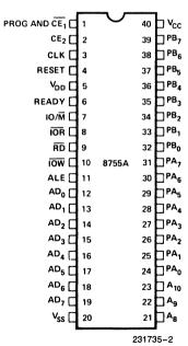
Figure 2. Pin Configuration
