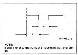
Figure 12. Asymmetrical Square-Wave Output Resulting from Count of 9
