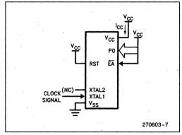
Figure 6. I<sub>CC</sub> Test Condition, Active Mode.
