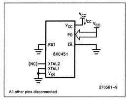
Figure 10. I<sub>CC</sub> Test Condition, Power Down Mode. All other pins are disconnected.
