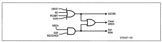
Figure 5.3. Receive Error Flag (Logic for Clearing GREN, setting RDN)
