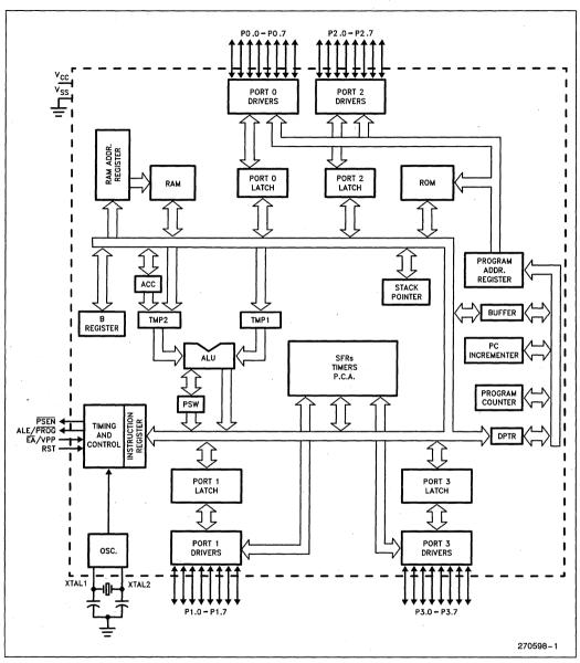
Figure 1. 83C51FB Block Diagram
