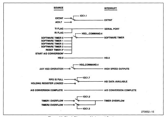
Figure 22. Block Diagram of Interrupt System
