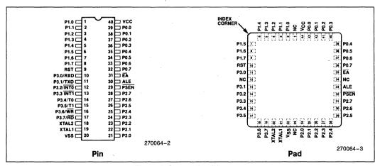
Figure 2. Connection Diagrams
