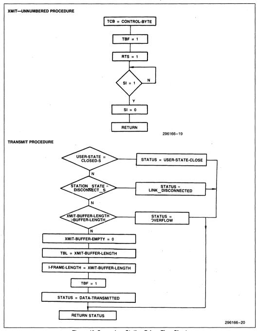
Figure 19. Secondary Station Driver Flow Chart
