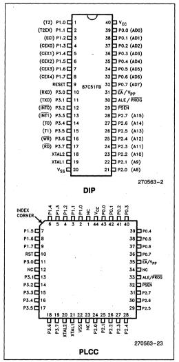
Figure 2. Pin Connections
