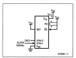
Figure 7. I<sub>CC</sub> Test Condition, Active Mode. All other pins are disconnected.
