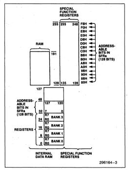
Figure 3. Internal Data Memory Address Space
