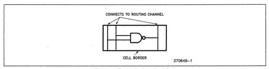
Figure 1. Example Standard Cell
