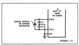
Figure 13. Using the On-Chip Oscillator
