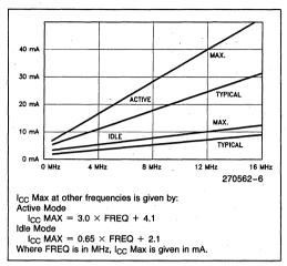
Figure 6. I<sub>CC</sub> vs Frequency valid only within frequency specifications of the device under test.
