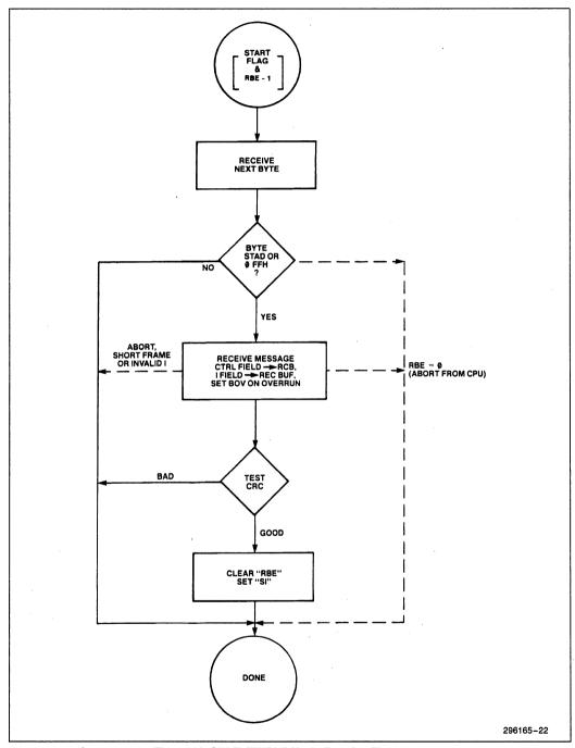
Figure 10. SIU FLEXIBLE Mode Receive Flowchart
