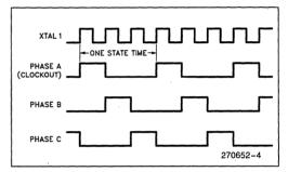
Figure 4. Internal Timings Relative to XTAL 1
