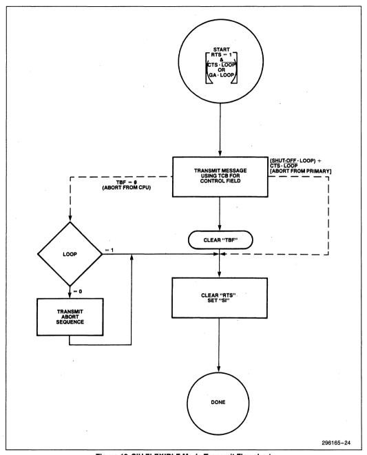
Figure 12. SIU FLEXIBLE Mode Transmit Flowchart
