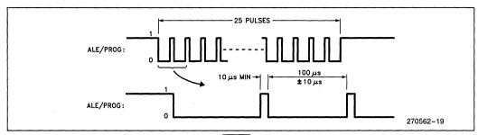
Figure 12. PROG Waveforms
