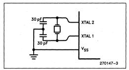
Figure 3. Using the On-Chip Oscillator
