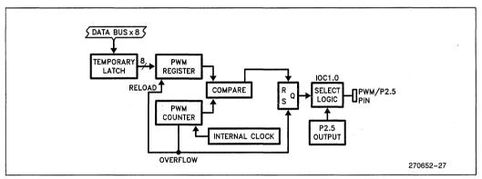
Figure 35. Pulse Width Modulated (D/A) Output
