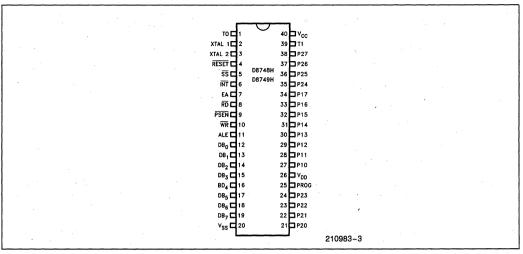
Figure 3. Pin Configuration
