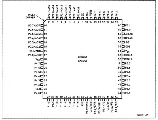
Figure 2. Pin Connections (PLCC)
