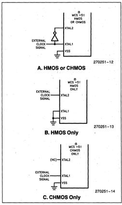
Figure 14. Using an External Clock
