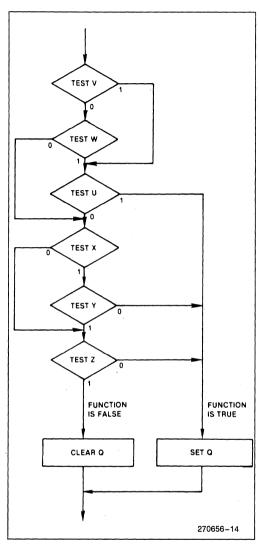
Figure 14. Flow Chart for Tree-Branching Algorithm
