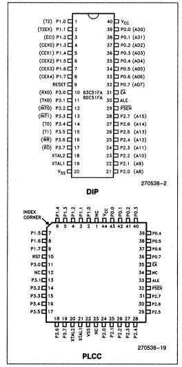
Figure 2. Pin Connections
