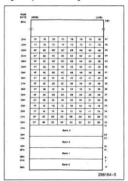
Figure 9. RAM Bit Address
