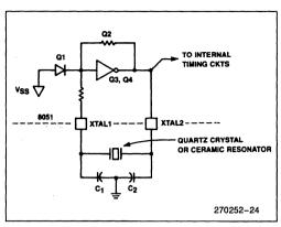
Figure 30. Using the HMOS On-Chip Oscillator
