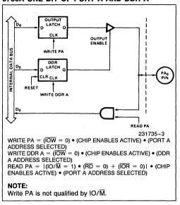
Note that hardware RESET or writing a zero to the DDR latch will cause the output latch's output buffer to be disabled, preventing the data in the Output Latch from being passed through to the pin. This is equivalent to putting the port in the input mode. Note also that the data can be written to the Output Latch even though the Output Buffer has been disabled. This enables a port to be initialized with a value prior to enabling the output.
