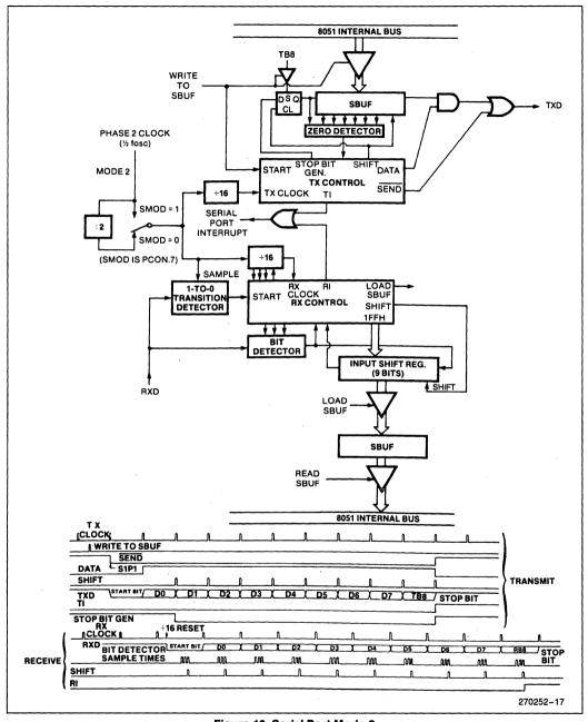
Figure 19. Serial Port Mode 2
