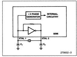
Figure 3. Block Diagram of Oscillator
