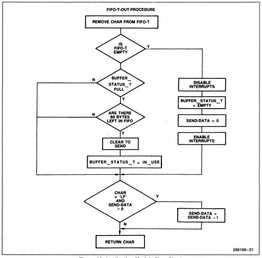
Figure 29. Application Module Flow Chart
