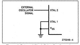
Figure 4. External Clock Drive Configuration
