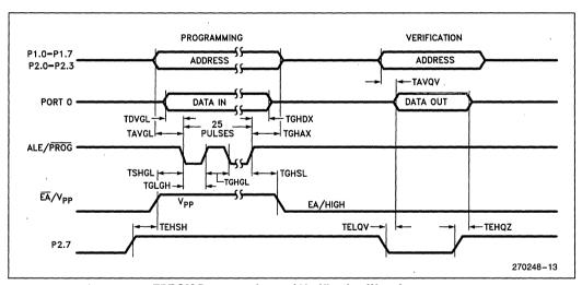
**EPROM Programming and Verification Waveforms**
