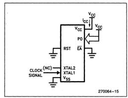
Figure 7. I<sub>CC</sub> Test Condition, Idle Mode. All other pins are disconnected.
