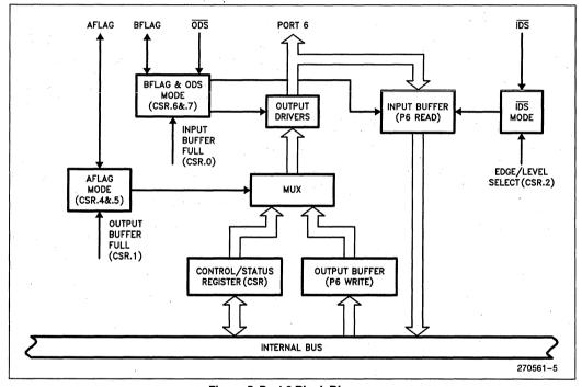
Figure 5. Port 6 Block Diagram
