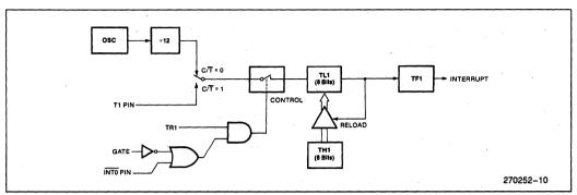
Figure 9. Timer/Counter 1 Mode 2: 8-Bit Auto-Reload
