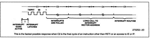
Figure 24. Interrupt Response Timing Diagram
