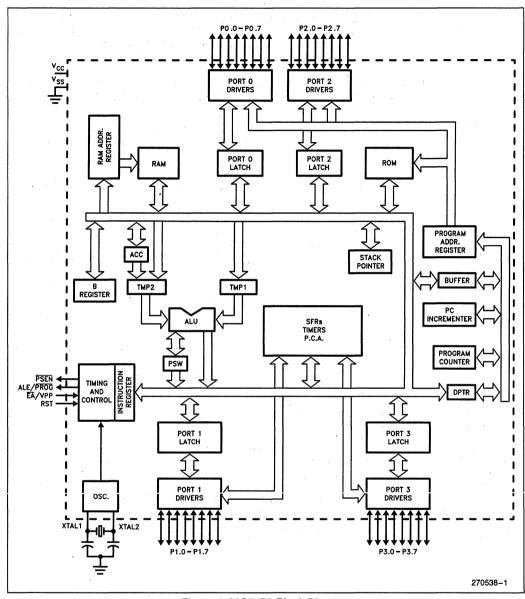
Figure 1. 83C51FA Block Diagram
