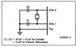
Figure 3. Oscillator Connections
