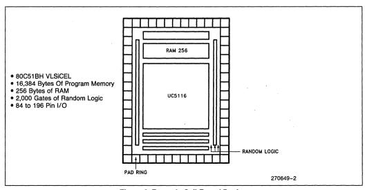
Figure 2. Example Cell-Based Design
