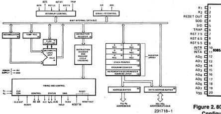
Figure 1. 8085AH CPU Functional Block Diagram
