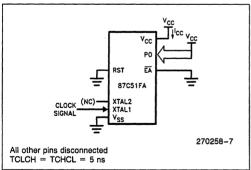
Figure 7. I<sub>CC</sub> Test Condition Idle Mode
