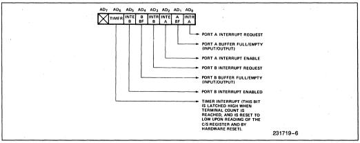
Figure 6. Status Register Bit Assignment
