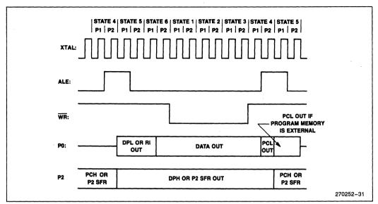
Figure 38. External Data Memory Write Cycle
