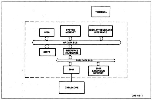
Figure 1. Block Diagram of 8088/8044 Interface Test
