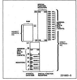
Figure 5. Internal Data Memory Address Space
