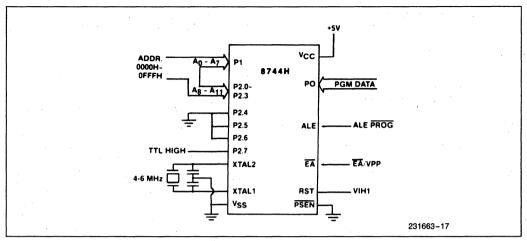
Figure 8. Programming Configuration
