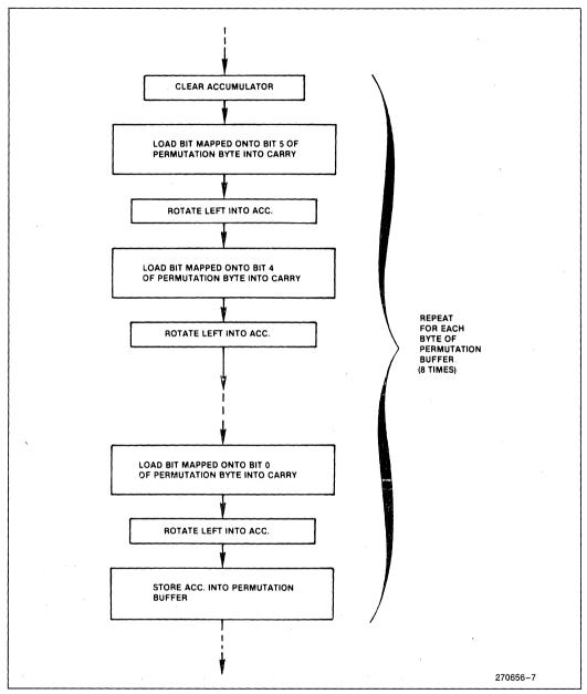
Figure 10b. DES Key Permutation with Boolean Processor
