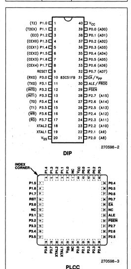
Figure 2. Connection Diagrams
