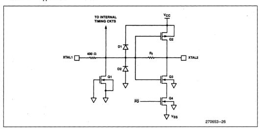
Figure 29. On-Chip Oscillator Circuitry
