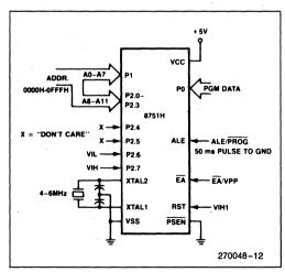
Figure 5. Programming Configuration
