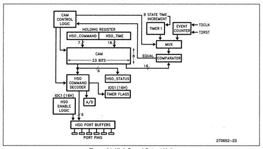
Figure 31. High Speed Output Unit
