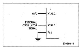
Figure 4. External Clock Drive Configuration
