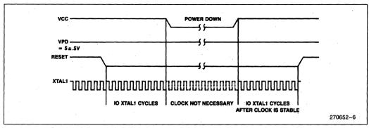
Figure 7. Power Down Timing
