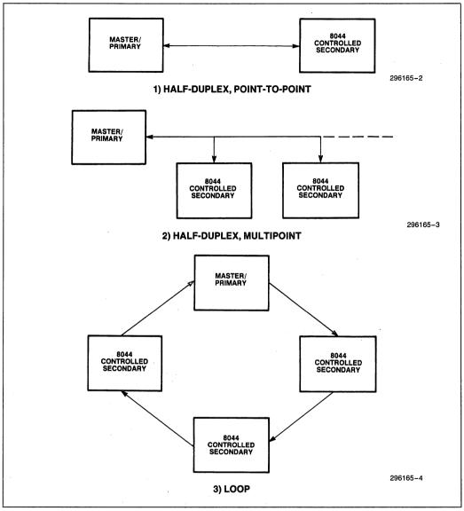
Figure 2. RUPI-44 Data Link Configurations
