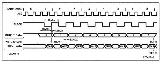
**Shift Register Mode Timing Waveforms**
