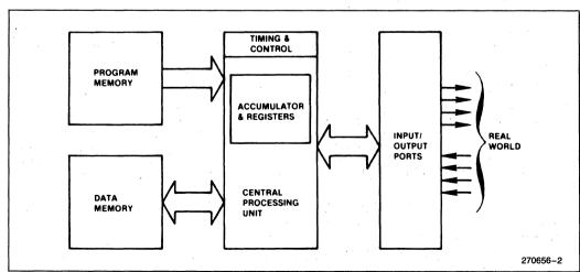
Figure 2. Block Diagram for Abstract Digital Computer
