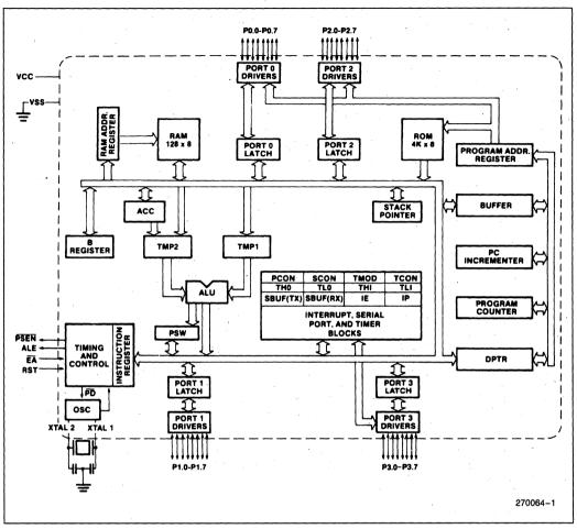
Figure 1. Block Diagram
