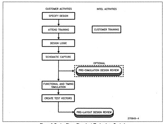
Figure 3. Design Phase Flowchart (Technology Center)
