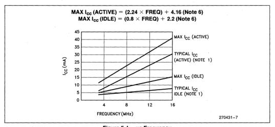
Figure 5. I<sub>CC</sub> vs Frequency
