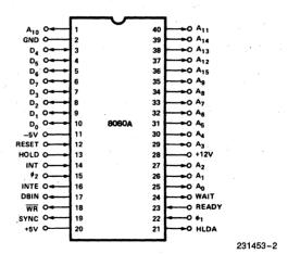
Figure 2. Pin Configuration
