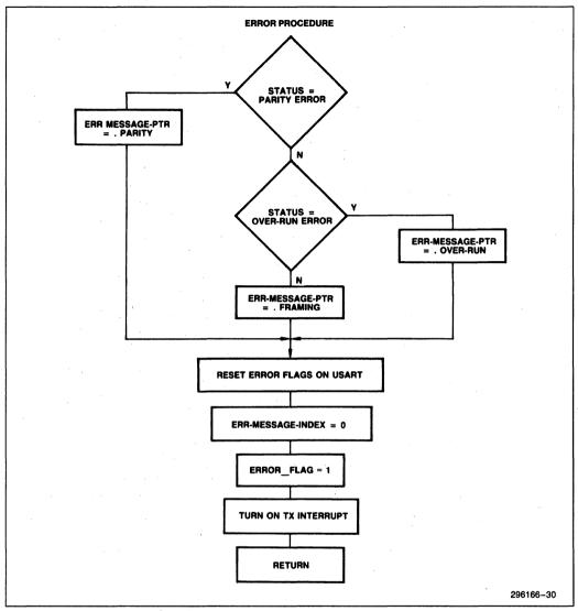
Figure 28. Application Module Flow Chart
