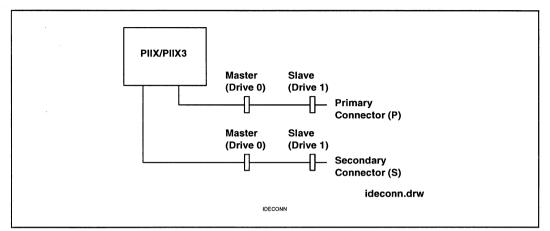
Figure 4. IDE Connector and Drive Nomenclature
