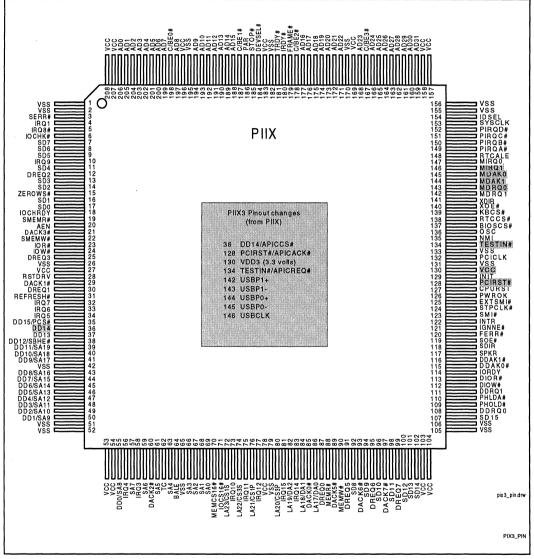
Figure 11. PIIX/PIIX3 Pin Assignment
