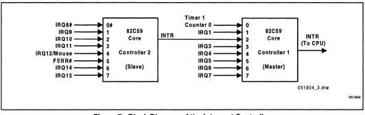
Figure 7. Block Diagram of the Interrupt Controller
