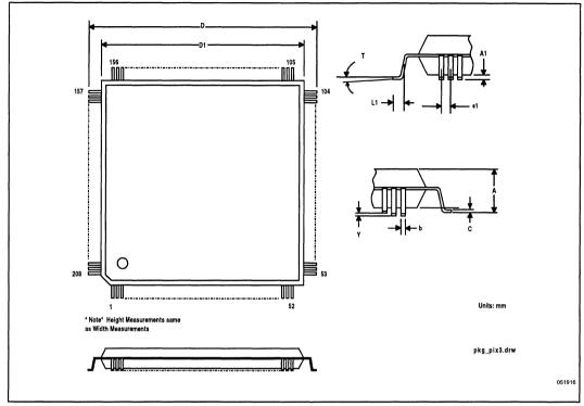
Figure 12. 208 Pin Quad Flat Pack (QFP) Dimensions
