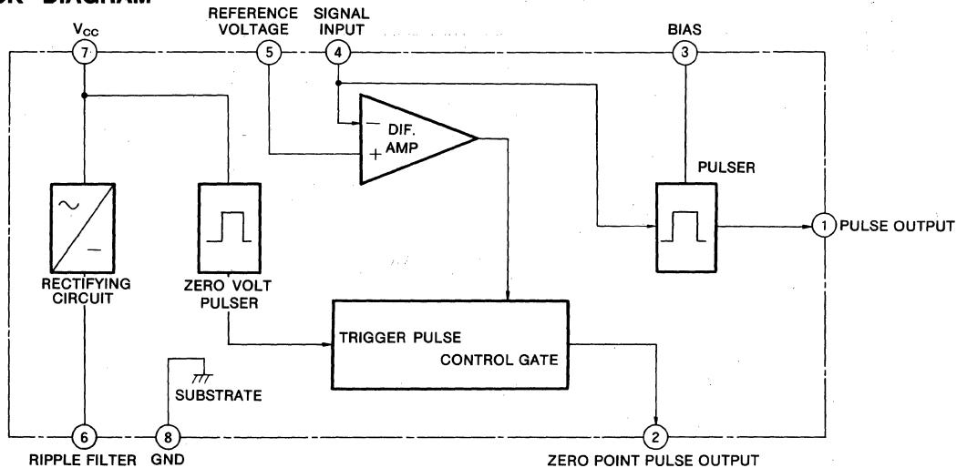
\* CAPACITOR MUST BE CONNECTED BETWEEN PIN 6 AND GND.
