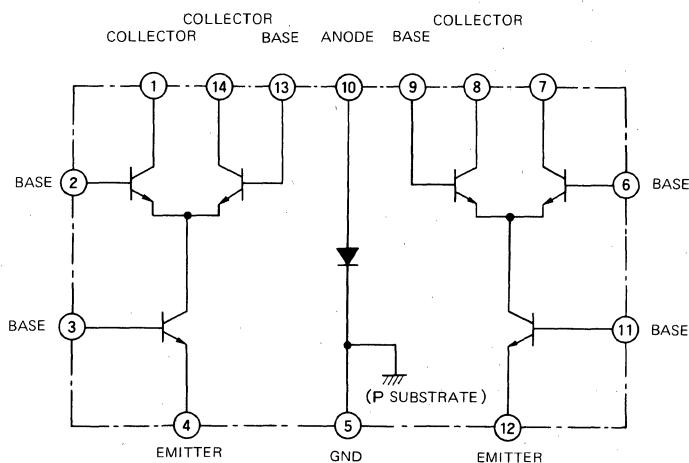
**DUAL DIFFERENTIAL AMPLIFIER****ABSOLUTE MAXIMUM RATINGS** ( $T_a=25^\circ\text{C}$ , unless otherwise noted)
