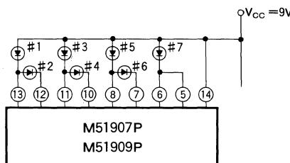
Connect similar to 1~3 according that a number of LED is odd or even. For example, in case of no use of #8 LED, connect similar to the case of no use of #2 LED.
