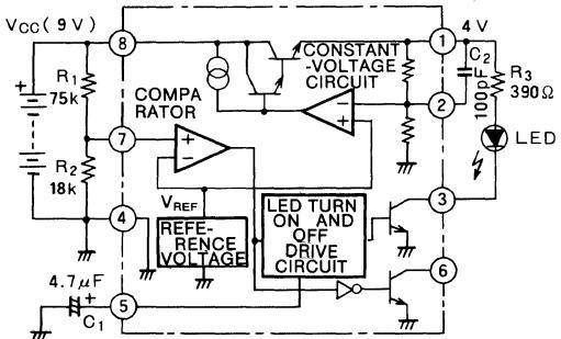
This is a battery reduced voltage checker which is set so that the LED starts turn ON and OFF when the voltage drops by 25% ( $V_{CC}=6.8V$ ) of the supply voltage ( $V_{CC}=9V, 1.5V \times 6$ ).  $C_1=4.7\mu F \rightarrow f=1.8Hz$
