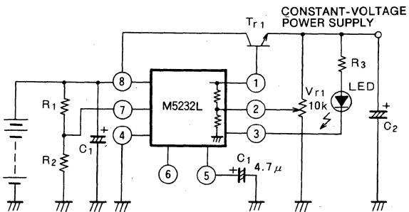
The current capacity of the built-in constant-voltage regulated power supply is approximately 20mA. However, by externally mounting transistor  $Tr_1$ , as shown in the figure on the left, it is possible to yield a constant-voltage regulated power supply with a high current capacity of 1A or more. The output voltage of the power supply can also be varied with variable resistor  $V_{r1}$ .
