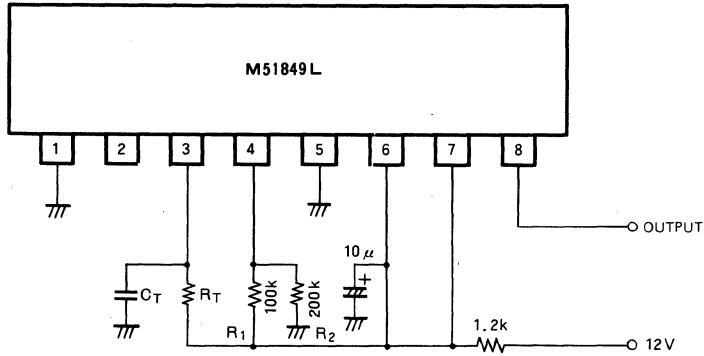
With the circuit connected as shown and it will trigger itself free run as a multivibrator.
