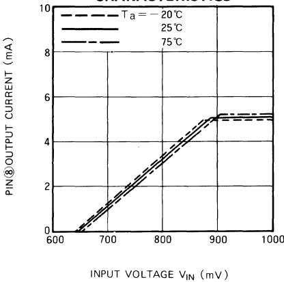
**PIN①OUTPUT CURRENT VS INPUT VOLTAGE TEMPERATURE CHARACTERISTICS**
