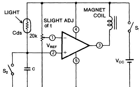
$$t = 0.7CR_{cds} \cdot \ln \frac{V_{CC}}{V_{CC}-V_{REF}}$$
