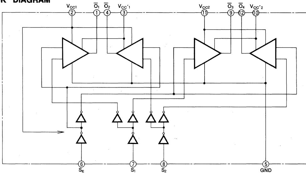
**DUAL BI-DIRECTIONAL MOTOR DRIVER****ABSOLUTE MAXIMUM RATINGS** ( $T_a=25^\circ\text{C}$ , unless otherwise noted)
