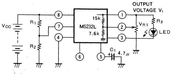
The M5232L has its output voltage  $V_1$  set by the built-in resistor, as shown in the figure, but this can be changed by connecting a semi-fixed resistor across GND and pins (1) and (2).
