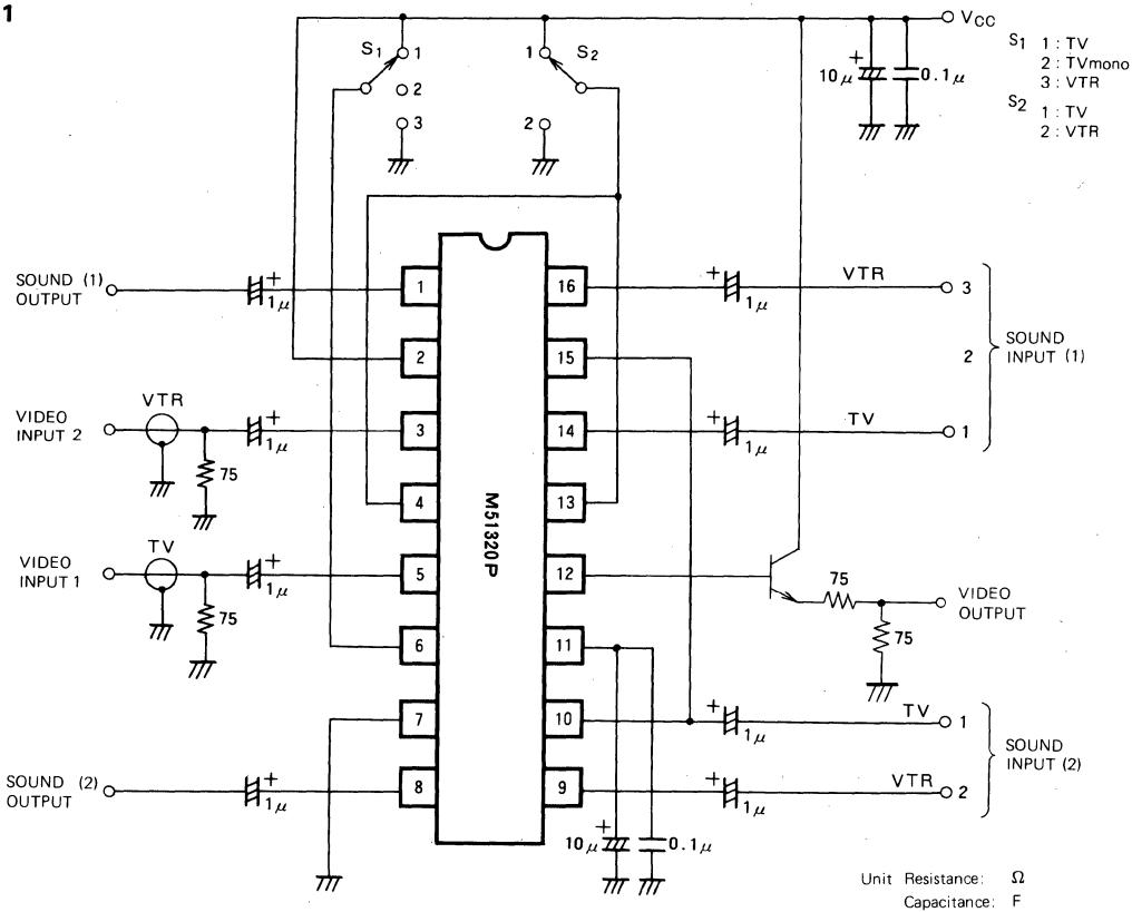
(Note) It is usually to use the external transistor to the video output shown in Fig. 1. When the supply voltage is below 9 volts, it is able to use the circuit shown in Fig. 2. In this circuit, the power dissipation is given by the following formula;
