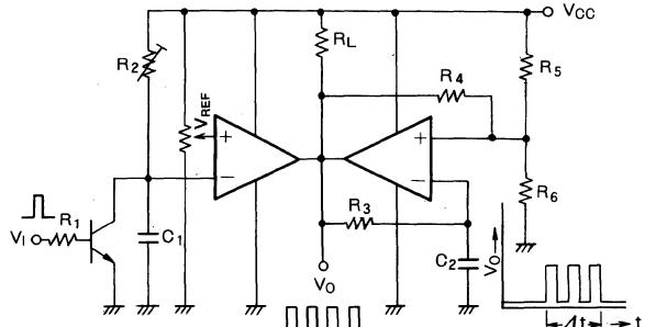
$$\Delta t = C_1 R_2 \cdot \ln \frac{V_{CC}}{V_{CC} - V_{REF}}$$
