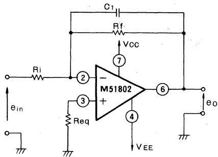
$$R_{req} = \frac{R_f \cdot R_i}{R_f + R_i} \quad e_o = \frac{1}{R_i C_1} \int e_{in} dt$$
