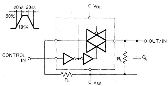
**QUADRUPLE BILATERAL SWITCH****TYPICAL PERFORMANCE CHARACTERISTICS****Analog switch "ON"
