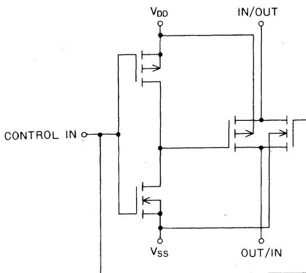
**LOGIC DIAGRAM (EACH SWITCH)**
