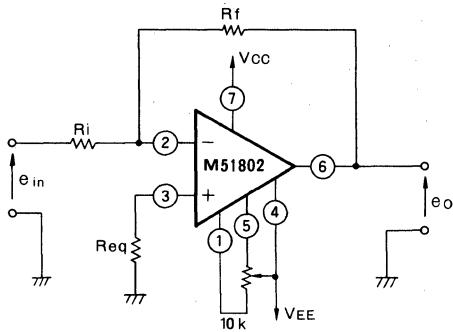
$$R_{req} = \frac{R_f \cdot R_i}{R_f + R_i} \quad A_{vo} = \frac{R_f}{R_i}$$
