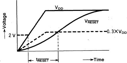
In case the power is on again after it is off and the voltage of RESET  $V_{RESET}$  is not perfectly down, the  $t_{RESET}$  must be also kept in over 1 msec, which was mentioned in the above diagram. When the prescribed condition is not satisfied, add the circuit illustrated below to the RESET and make the power-on reset function accurately. In this case, make sure to select an external capacitance to satisfy the  $V_{RESET} \geq 1 \text{ msec.}$
