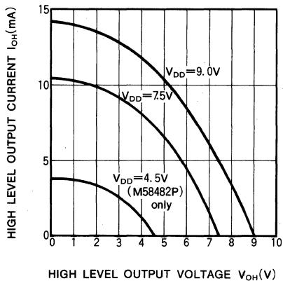
(2)  $I_{OH} - V_{OL}$  (OUT 1, OUT 2, OUT 3)
