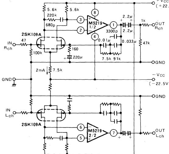
Left channel circuit constants are identical to those of right channel.
