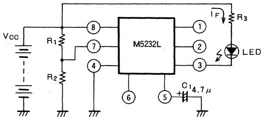
The output is not stabilized at  $V_{CC} < 5V$  since the output voltage at pin (1) of M5232L is not regulated at 4V. When an LED is connected directly from  $V_{CC}$  as shown in the figure on the left, it is possible to configure a battery checker of less than  $V_{CC} 5V$ . In this case, however, the  $I_F$  for the LED will fluctuate in accordance with the changes in  $V_{CC}$ .
