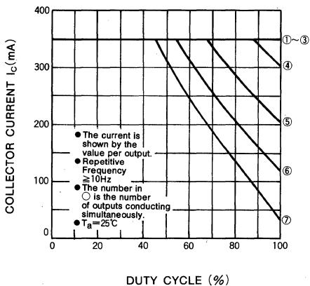
**ALLOWABLE COLLECTOR CURRENT AS A FUNCTION OF DUTY CYCLE**
