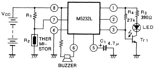
In nomal circumstances the LED is set off and the current dissipation is kept down. In abnormal circumstances, the LED turn ON and OFF. It is also possible to drive a relay or indicator using a buzzer at pin(6).
