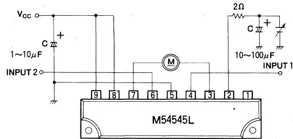
4) Motor speed control by the  $V_R$  and  $V_{CC'}$
