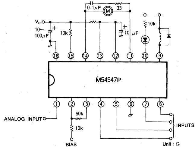
**BI-DIRECTIONAL MOTOR DRIVER WITH MOTOR SPEED CONTROL****DESCRIPTION**
