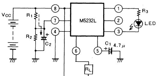
By connecting C<sub>2</sub> in parallel with R<sub>2</sub>, V<sub>CC</sub> is turned on, the charging current indicated by the dotted line in the figure is made to flow, and until the pin(7) voltage reaches :
