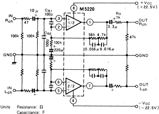
Left channel circuit constants are identical to those of right channel.
