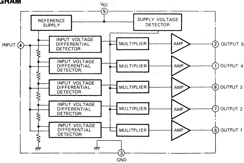
**LED LINEAR LEVEL INDICATOR****ABSOLUTE MAXIMUM RATINGS** ( $T_a=25^\circ\text{C}$ , unless otherwise noted)
