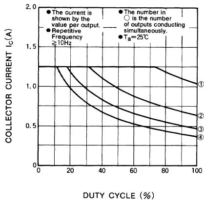
**ALLOWABLE COLLECTOR CURRENT AS A FUNCTION OF DUTY CYCLE**
