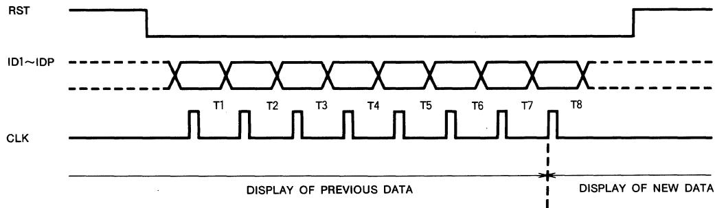
When LOAD is kept at "H", LOAD is automatically done at the 8th CLK input when RST="L". However, while RST="L", if there is a 9th CLK input, the 9th data will be loaded and displayed.
