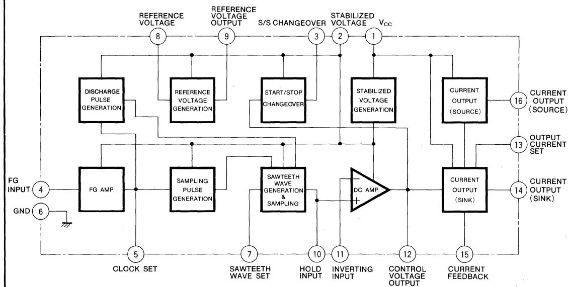
**FREQUENCY-VOLTAGE (F-V) CONVERTER****ABSOLUTE MAXIMUM RATING** ( $T_a=25^\circ\text{C}$ , unless otherwise noted)
