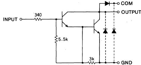
UNIT :  $\Omega$ **ABSOLUTE MAXIMUM RATINGS** ( $T_a = -20 \sim +75^\circ\text{C}$ , unless otherwise noted)
