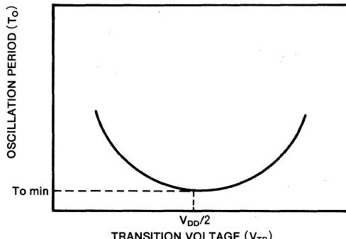
Fig. 2. Oscillation period ( $T_0$ ) VS Transition Voltage ( $V_{TR}$ )
