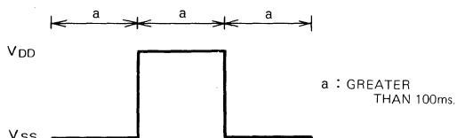
Fig. 3 L pin/M pin/PRESET pin input waveform
