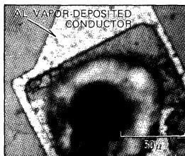
**Fig. 2 Example of corrosion of an aluminum vapor-deposited conductor (analyzed using a metallurgical microscope)**
