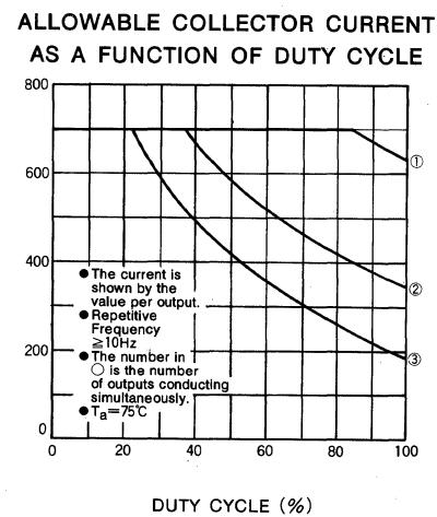
**6-UNIT 700mA TRANSISTOR ARRAY WITH CLAMP DIODE**
