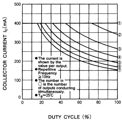
**ALLOWABLE COLLECTOR CURRENT AS A FUNCTION OF DUTY CYCLE**
