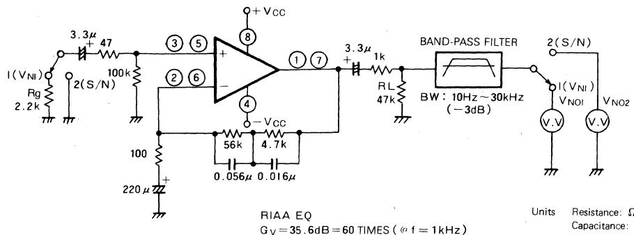
$$1. V_{NI} = V_{NO1} / 60 \text{ } (\mu\text{Vrms})$$
