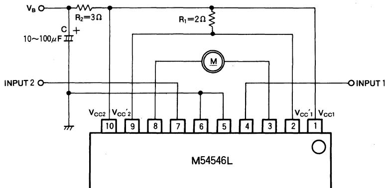
2) MOTOR SPEED CONTROL BY THE  $V_{CC'}$
