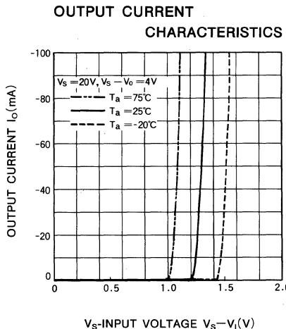
**7-UNIT 150mA SOURCE TYPE DARLINGTON TRANSISTOR ARRAY**
