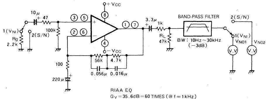
1.  $V_{NI} = V_{NO1}/60$  ( $\mu\text{VRms}$ )
