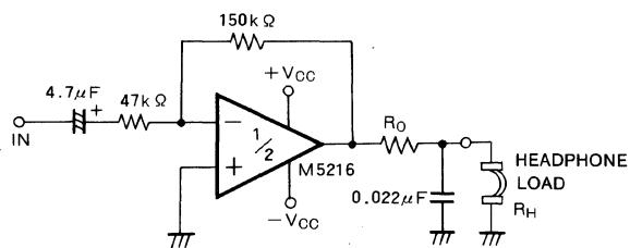
Note : For a single power supply system, the level of the (+) input pin should be shifted to  $V_{CC}/2$  potential and the output should be AC-coupled through a capacitor.
