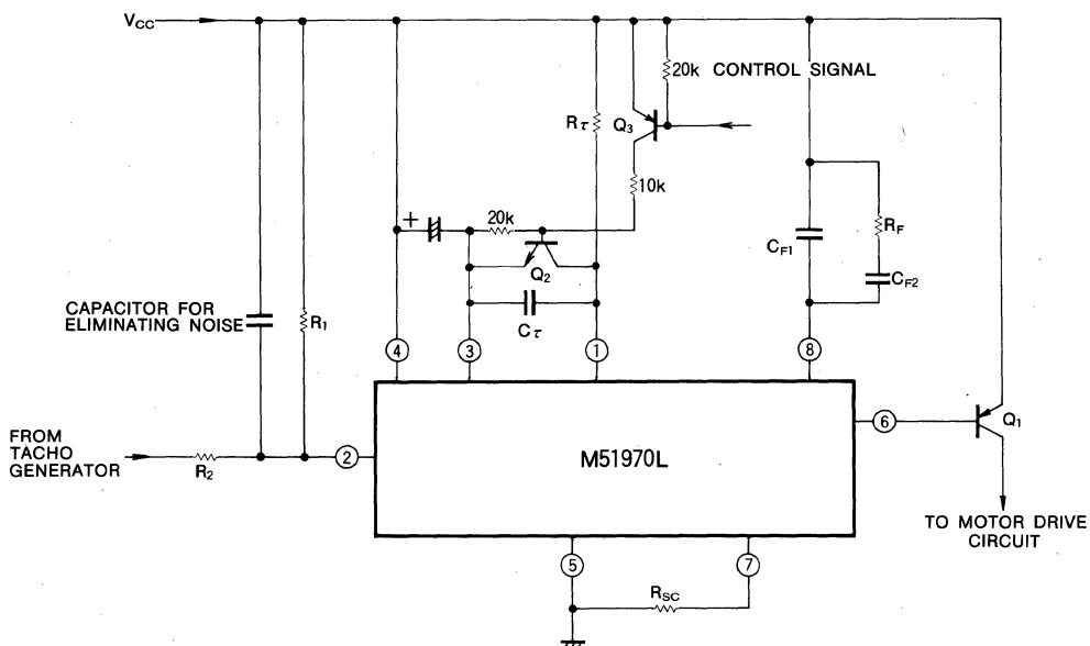
The motor is off when Q<sub>2</sub> and Q<sub>3</sub> are on.
