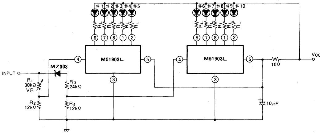
Note 1. Resistance  $R_1$  is selected so that the turn-on voltage for LED #6 is approximately 630mV higher than that of LED #5.
