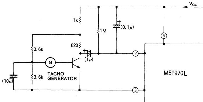
The above constants of capacitors are example in case  $F_C=500\text{Hz}$ .
