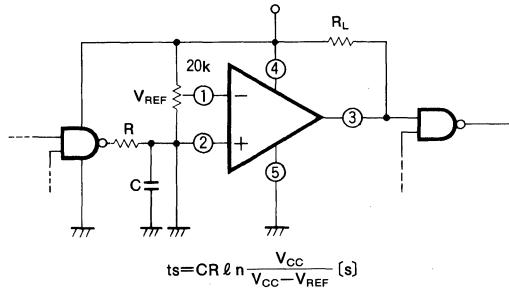
Window comparator (alarm circuit)
