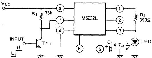
When the base of transistor Tr<sub>1</sub> is set low (normal), the pin(7) comparator input voltage is set high, pin (3) is set low and the LED is turned off.
