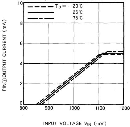
**PIN②OUTPUT CURRENT VS INPUT VOLTAGE TEMPERATURE CHARACTERISTICS**
