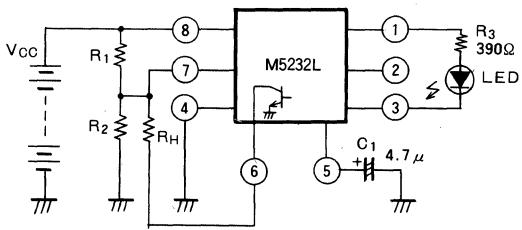
By connecting  $R_H$  across pins (6) and (7), as shown in the figure on the left, the turn ON and OFF start voltage is set at :
