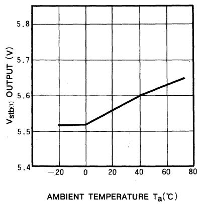
THRESHOLD VOLTAGE OF COMPARATOR 1
