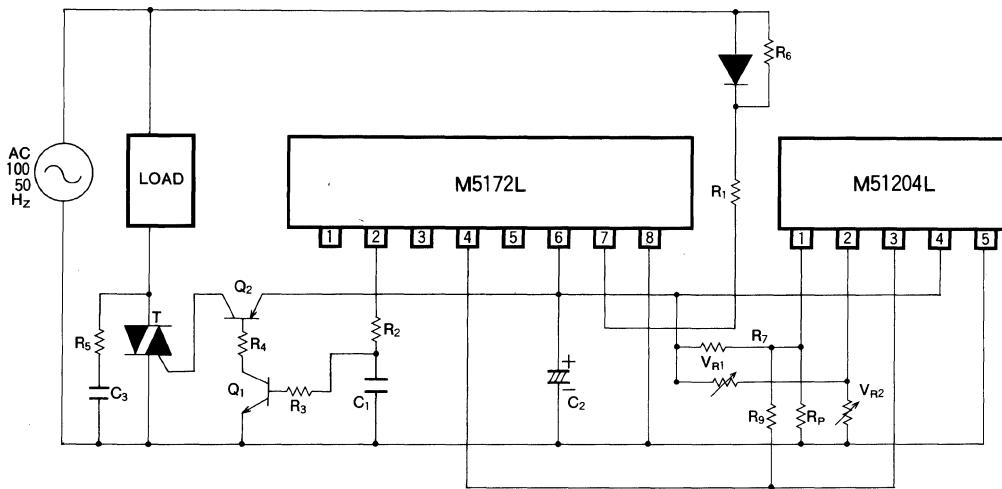
$R_1 = 6k\Omega(2W)$     $R_2 = 1k\Omega(\frac{1}{4}W)$     $R_3 = 10k\Omega(\frac{1}{4}W)$     $R_4 = 1k\Omega(\frac{1}{4}W)$
