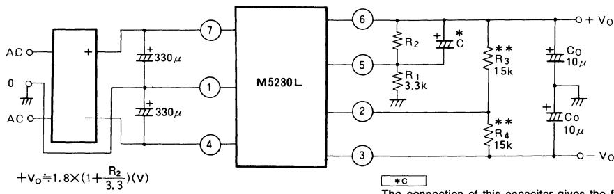
Note : When the input power supply lines become long, a  $0.1\mu F$  capacitor should be connected between input power supply pins ⑦ and ④ and ground.
