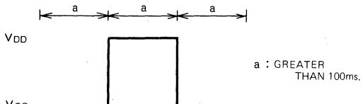
Fig. 2 MEMORY pin input waveform
