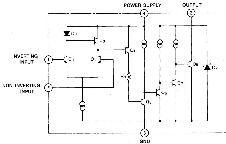
**VOLTAGE COMPARATOR****ABSOLUTE MAXIMUM RATINGS** ( $T_a=25^\circ\text{C}$ , unless otherwise noted)
