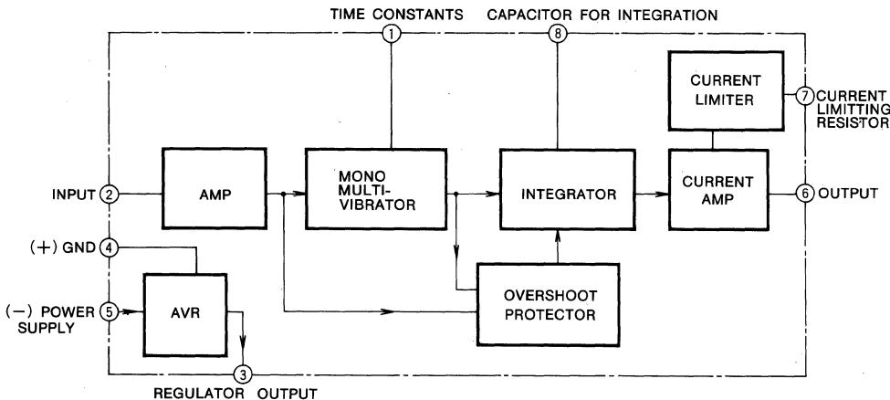
**SPEED CONTROL FOR DC MICRO MOTOR****ABSOLUTE MAXIMUM RATINGS** ( $T_a=25^\circ\text{C}$ , unless otherwise noted)
