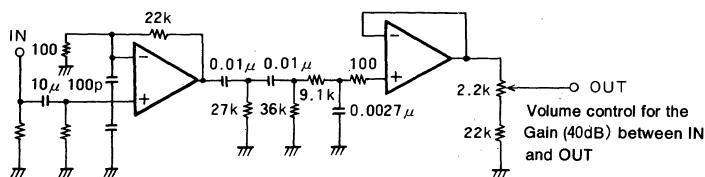
**DUAL CHANNEL ELECTRONIC ATT****TEST METHODS** ( $T_a=25^\circ\text{C}$ ,  $V_{CC}=12\text{V}$ ,  $f=1\text{kHz}$ , unless otherwise noted)
