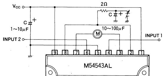
3) Motor speed control by the  $V_{CC}$
