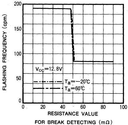
Note : 1. Flashing frequency characteristics was measured by changing the resistance value for break detecting instead of the lamp resistance used lamp; one 23W lamp
