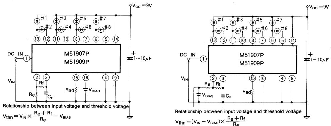
Relationship between input voltage and threshold voltage
