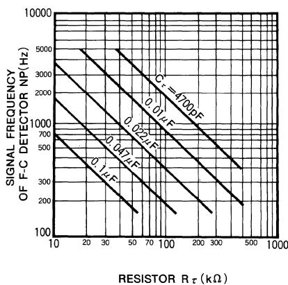
$R_\tau \cdot C_\tau$  determine the speed of motor
