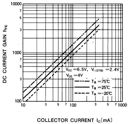
**7-UNIT 150mA TRANSISTOR ARRAY WITH CLAMP DIODE AND STROBE****DESCRIPTION**
