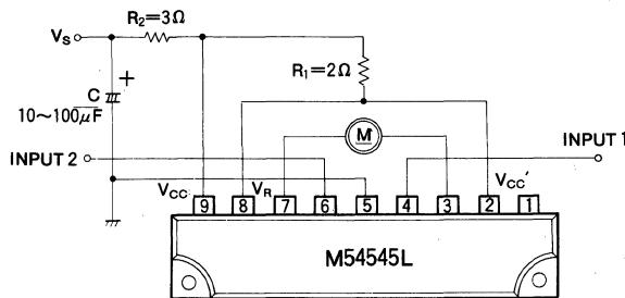
2) Motor speed control by the  $V_R$  and  $V_{CC}$
