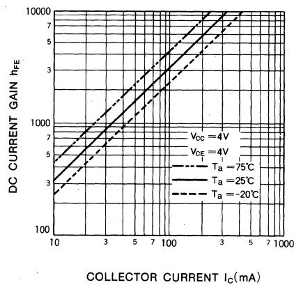
**4-UNIT 1.5A DARLINGTON TRANSISTOR ARRAY WITH CLAMP DIODE****DESCRIPTION**
