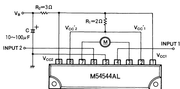
2) MOTOR SPEED CONTROL BY THE  $V_{CC}'$
