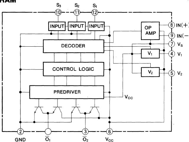
**BI-DIRECTIONAL MOTOR DRIVER WITH MOTOR SPEED CONTROL**
