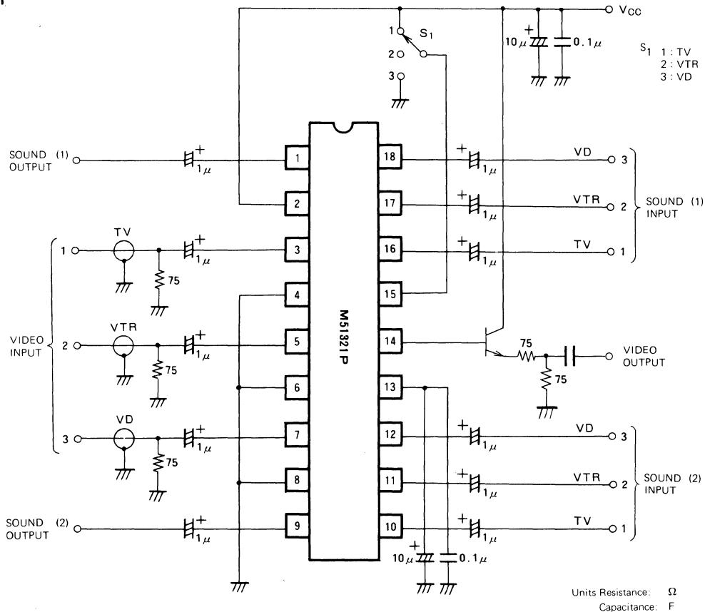
(Note) It is usually to use the external transistor to the video output shown in Fig. 1. When the supply voltage is below 9 volts, it is able to use the circuit shown in Fig. 2. In this circuit, the power dissipation is given by the following formula;
