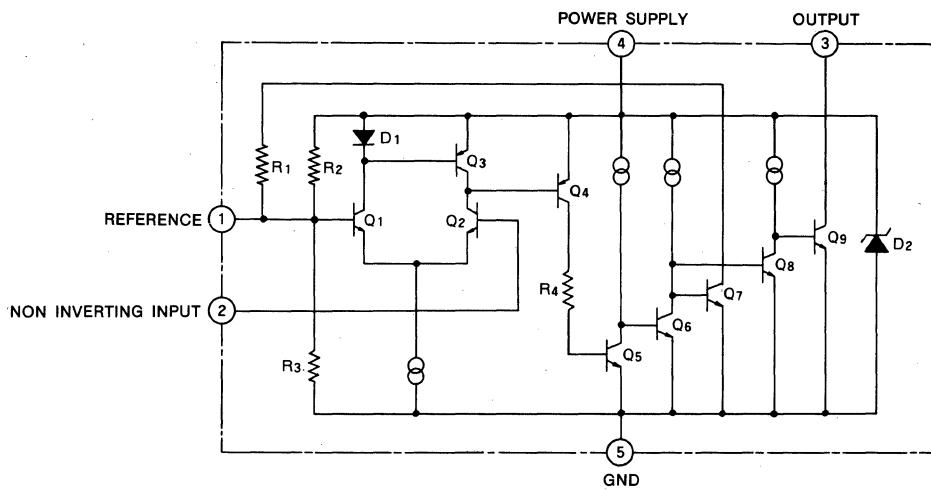
**VOLTAGE COMPARATOR****ABSOLUTE MAXIMUM RATINGS** ( $T_a=25^\circ\text{C}$ , unless otherwise noted)
