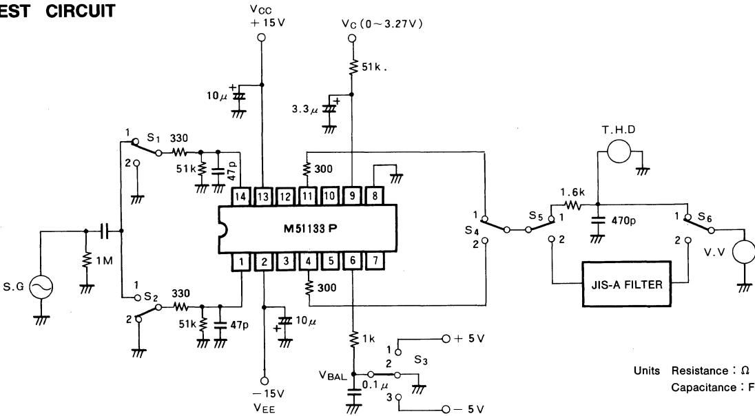
Note : Low-ripple-noise Power Supply recommended for  $V_{CC}$  and  $V_{EE}$ . (under  $2\mu$ Vrms)
