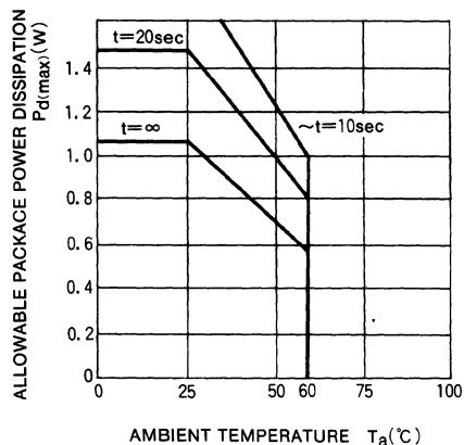
Note 1 : Mounted on an epoxy PC board with Cu cover on one side (5cm×5cm×0.8mm)
