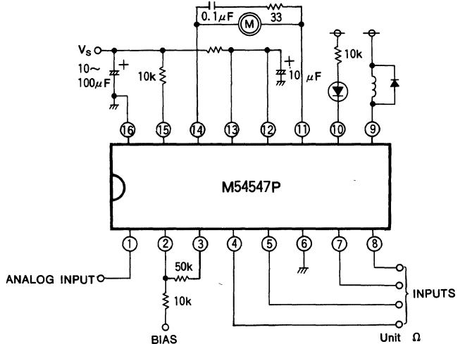
**BI-DIRECTIONAL MOTOR DRIVER WITH MOTOR SPEED CONTROL****DESCRIPTION**
