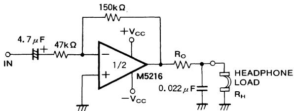
(Note) For a single power supply type, (+) input pin voltage level is shifted at  $V_{CC}/2$  and output must be used by AC connection by means of a capacitor
