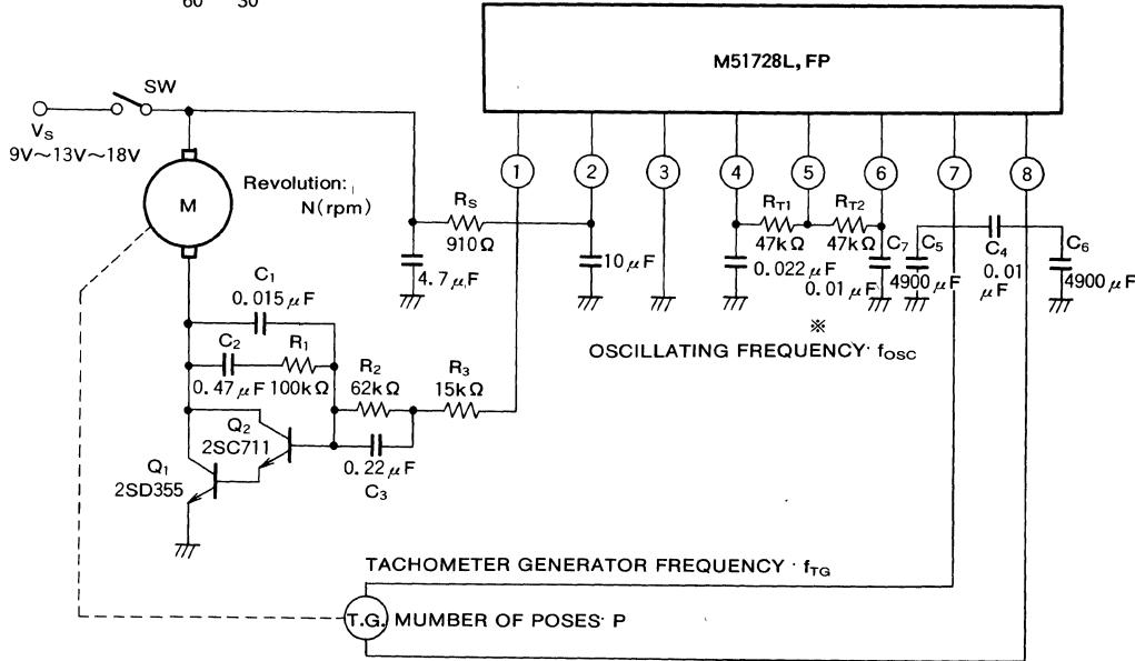
\* External signals of crystal oscillator can be input at Pin ⑥ as oscillating frequency. The input threshold value is as follows.
