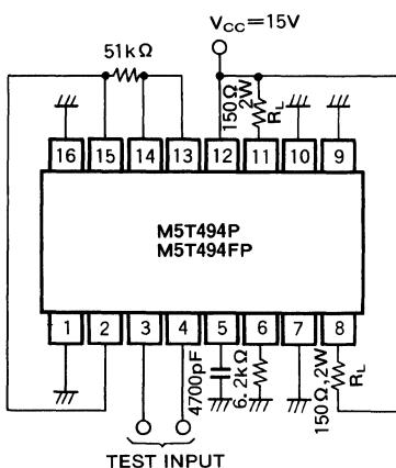
Note: Connect Pin ⑧ and Pin ⑪ to  $V_{CC}$  and connect Pin ⑨ and Pin ⑩ to GND via resistors  $R_L$  when emitter follower output is used.
