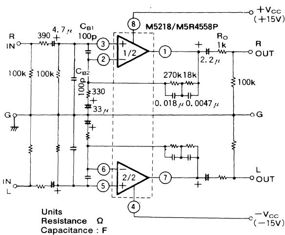
Left channel circuit constants are identical to those of right channel.
