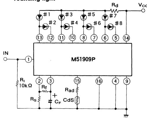
The LED current is determined by  $R_{\text{ad}} + R_{\text{cds}}$ .
