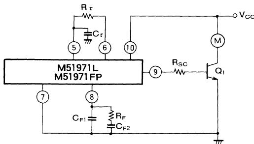
$$I_{9\max} = \frac{V_{9\max}}{R_{9\max} + R_{SC}} \quad V_{9\max} \approx 3.2V, \quad R_{9\max} \approx 100\Omega$$
