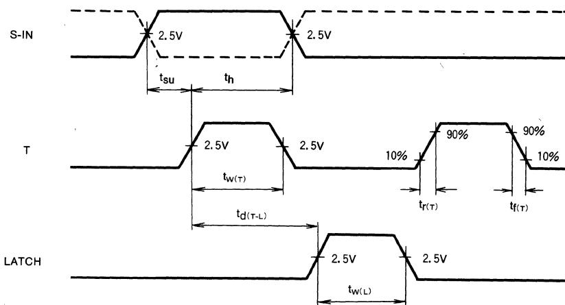
SWITCHING CHARACTERISTICS ( $T_a=+25^\circ\text{C}$ ,  $V_{cc}=5\text{V}$ )
