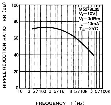
**(5V, 5.6V, 8V, 9V, 10V, 12V, 15V) 3-Terminal Fixed Positive Output Voltage Regulator (With Fold-Back Protection Circuit)**
