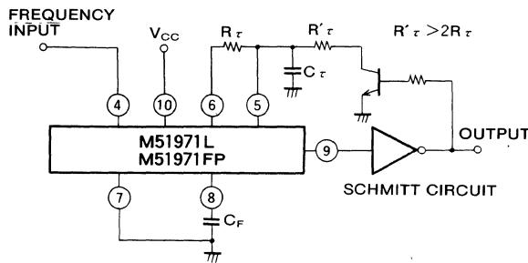
Note. The hysteresis of Schmitt circuit should be higher than repple voltage at Pin ⑧ (to prevent chattering)
