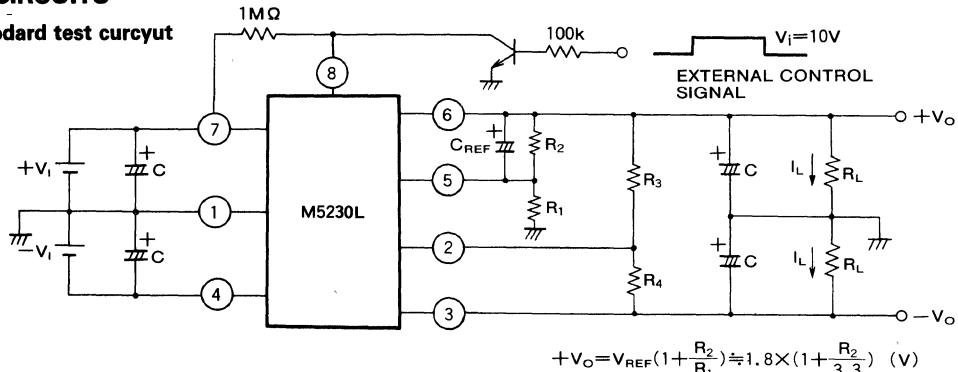
$$+V_o = V_{REF} \left(1 + \frac{R_2}{R_1}\right) \div 1.8 \times \left(1 + \frac{R_2}{3.3}\right) \text{ (V)}$$
