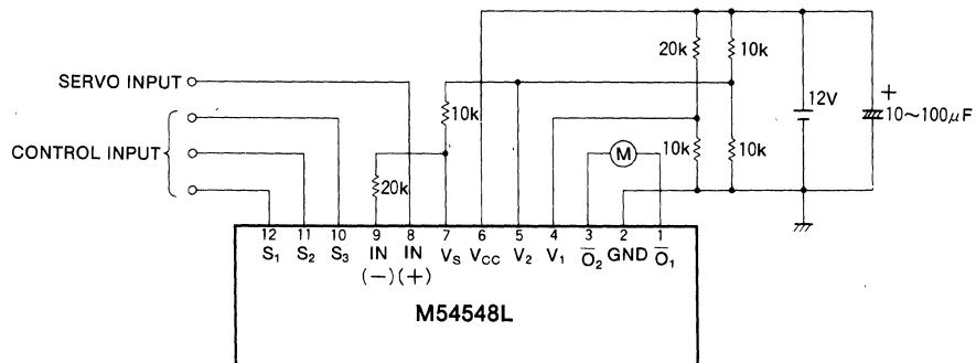
**BI-DIRECTIONAL MOTOR DRIVER WITH MOTOR SPEED CONTROL****DESCRIPTION**
