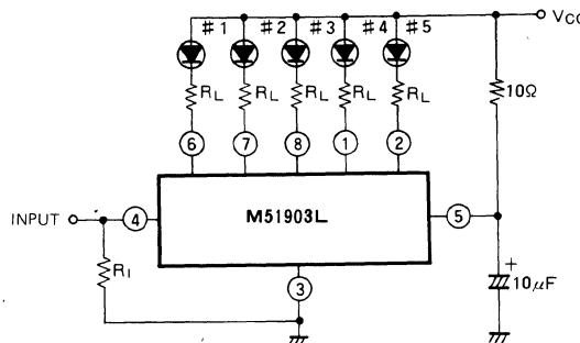
Note 1 The value of  $R_L$  is chosen to suit the LED devices to be used. The maximum LED current  $\approx (V_{CC} - \text{LED forward voltage drop} - 1.0)/R_L \leq 15\text{mA}$
