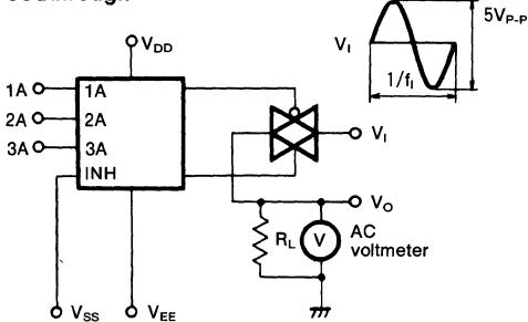
The feedthrough is taken as that frequency  $f_1$  at which, using a sine-wave input of  $2.5V_{P-P}$ ,  $20 \log_{10}(V_O/V_I) = -50dB$ . Refer to the function table for conditions of control input A.
