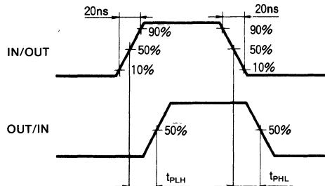
**5 "L-H" and "H-L" output propagation time (CONTROL IN-OUT/IN)**
