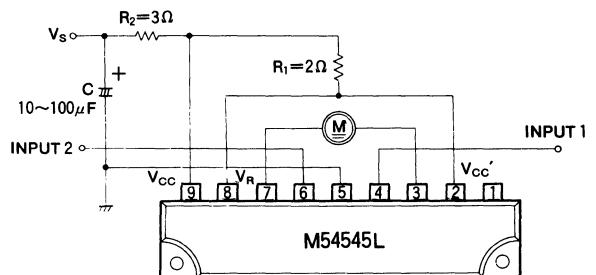
2) Motor speed control by the V<sub>R</sub> and V<sub>CC</sub>
