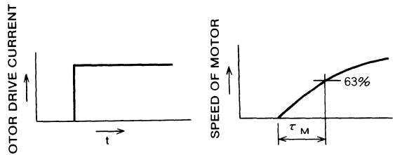
The method is to apply stepping current to halted motor and measure the time  $\tau_M$  when the speed of motor reaches 63% of the final speed and the  $\tau_M$  is obtained from the following equation.
