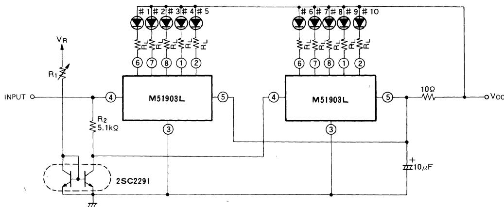
Note 1 Resistance  $R_1$  selected so that the turn-on voltage for LED #6 is approximately 210mV higher than that of LED #5
