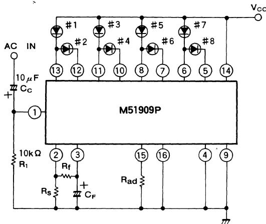
Rad: Resistance determining LED current
