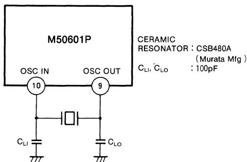
Fig. 1. Example Oscillator Circuit (using a ceramic resonator)
