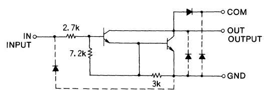
COM and GND are all common to 8 circuits.
