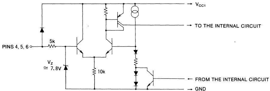
Apply  $3.5V - V_{CC}$  to the ON voltage ( $V_{IH}$ ) and  $0 - 1V$  to the OFF voltage ( $V_{IL}$ ) of the input.
