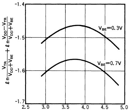
Fig. 2. Oscillation period ( $T_O$ ) VS Transition Voltage ( $V_{TR}$ )
