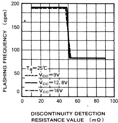
**FLASHING FREQUENCY CHARACTERISTICS ②**
