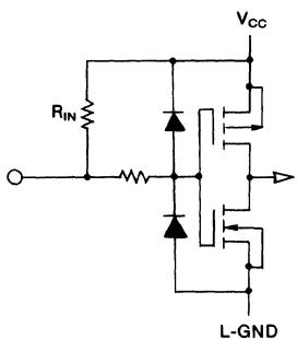
2 INPUT WITH PULL-DOWN RESISTOR
