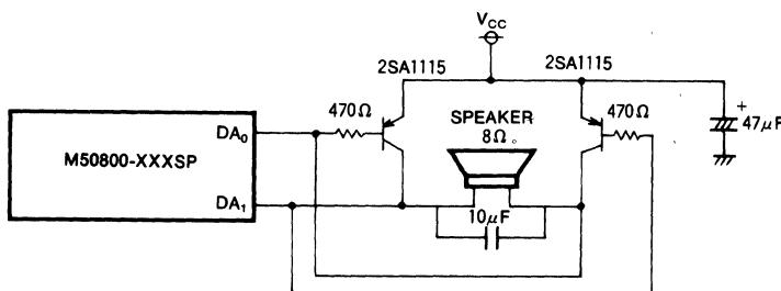
Maximum output power=500mW typ. ( $V_{CC}=5V$ )
