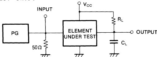
Input waveform is taken as  $t_r \leq 20\text{ns}$  and  $t_f \leq 20\text{ns}$
