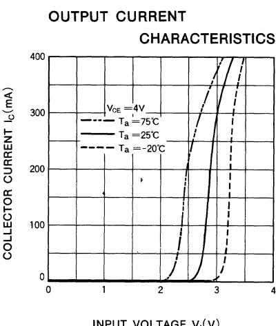
7-UNIT 400mA DARLINGTON TRANSISTOR ARRAY WITH CLAMP DIODE
