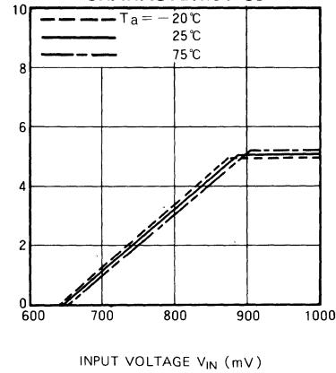
PIN①OUTPUT CURRENT VS INPUT VOLTAGE TEMPERATURE CHARACTERISTICS
