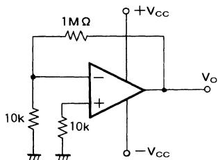
$$\bullet V_{IO} = \frac{V_O}{100} \quad (V_{CC} \pm 15V)$$
