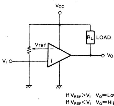
(2) Schmitt trigger circuit
