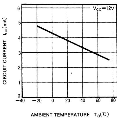
**INPUT CURRENT VS AMBIENT TEMPERATURE**
