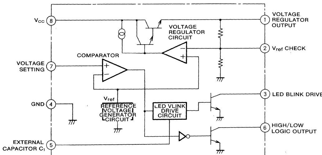
VOLTAGE DETECTOR/ON-OFF ALARM CIRCUIT
