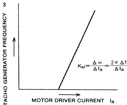
Plot the relationship between motor drive current and tacho generator frequency and obtain the inclination.
