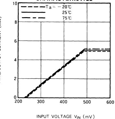
PIN⑦OUTPUT CURRENT VS INPUT VOLTAGE TEMPERATURE CHARACTERISTICS
