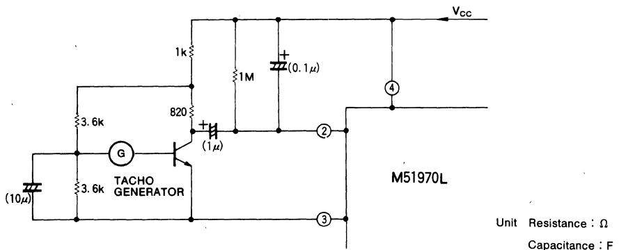
The above constants of capacitors are example in case  $F_G=500\text{Hz}$ .
