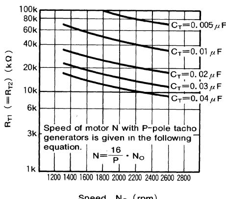
The fig. shows relationship between oscillator time constants ( $T_{T1}$ ,  $R_{T2}$ ,  $C_T$ ) and speed  $N_o$  of a motor with sixteen-pole tachometer generator. The limits in the above are obtained when  $R_{T1}=R_{T2}=47\text{k}\Omega$ ,  $C_T=0.01\mu\text{F}$ .
