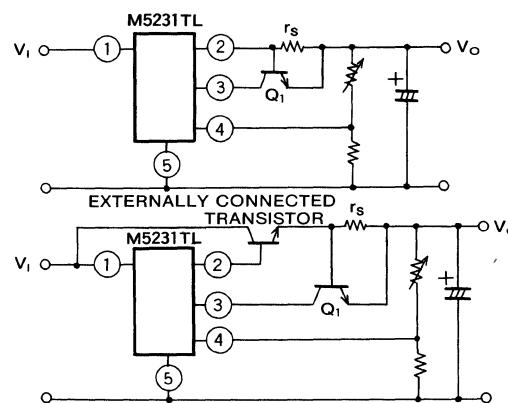
The control circuit consists of  $Q_1$  and  $r_s$ . If the control current is  $I_{SC}$ ,  $r_s$  is obtained from the equation below.
