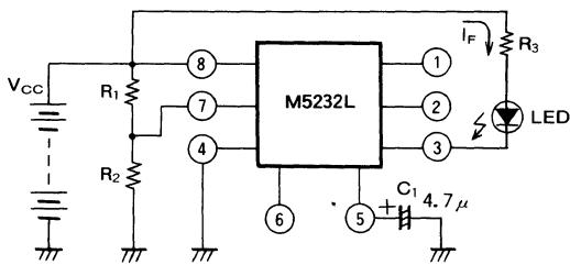
Since output Pin ① of the M5232L is regulated at 4V, the output is not stabilized at  $V_{CC}$  less than 5V.
