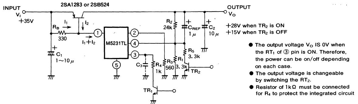
(Note) The load current can be over 1A by connection the external power TR.
