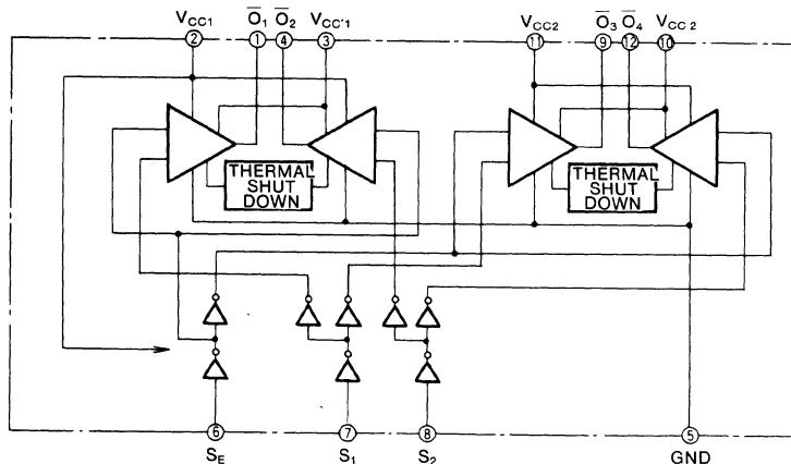
DUAL BI-DIRECTIONAL MOTOR DRIVER WITH THERMAL SHUT DOWN FUNCTION
