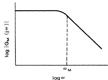
Simulated transfer function of the motor
