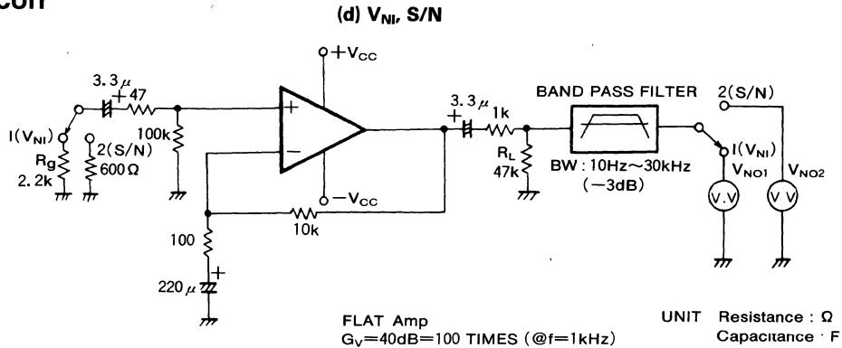
1.  $V_{NI} = V_{NO1}/100 (\mu\text{Vrms})$
