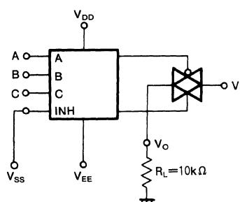
$$R_{ON}=10 \times \frac{(V_I-V_O)}{V_O} (\text{k}\Omega)$$
