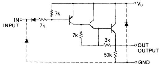
$V_s$  and GND are common to the 8 circuits.
