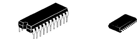
22-pin molded plastic DIP 24-pin molded plastic shrick
