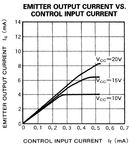
Note when collector output 2 system and emitter output 1 system are ON
