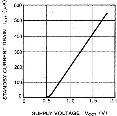
**OPERATING CURRENT DRAIN VS. SUPPLY VOLTAGE**
