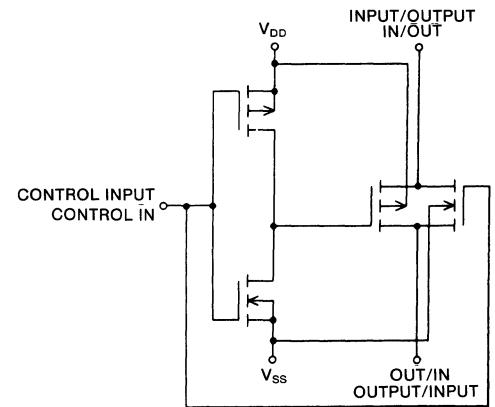
**LOGIC DIAGRAM (EACH SWITCH)**
