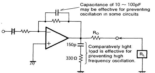
$R_o$  is recommended because it is effective for preventing capacitative load oscillation and controlling current when load is shorted.
