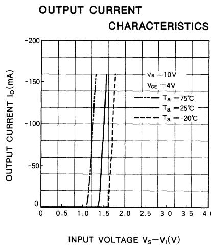
7-UNIT 150mA SOURCE TYPE DARLINGTON TRANSISTOR ARRAY
