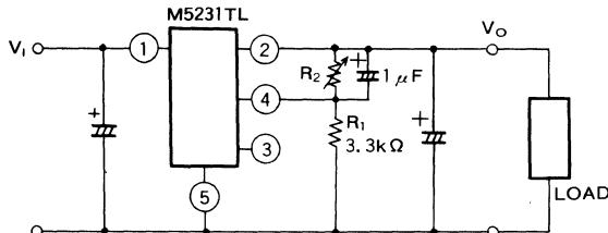
Output voltage ( $V_o$ ) can be set freely by externally connected resistors  $R_1$ ,  $R_2$  from the following equation.
