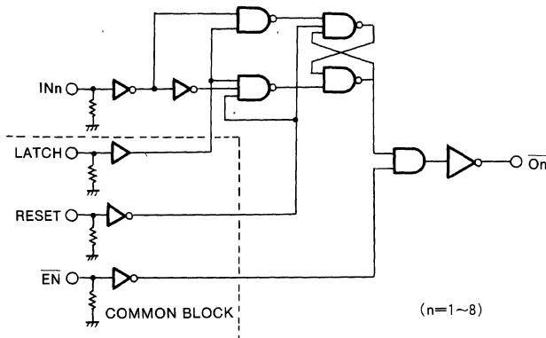
**INPUT/OUTPUT EQUIVALENT CIRCUIT SCHEMATICS**
