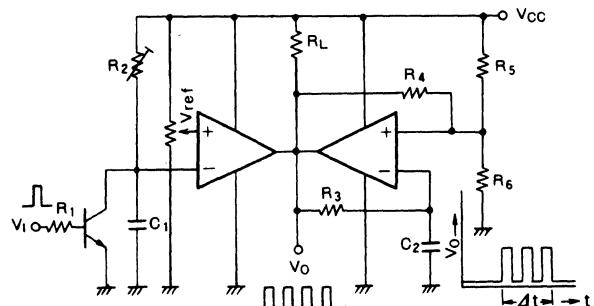
$$\Delta t = C_1 R_2 \cdot \ln \frac{V_{CC}}{V_{CC} - V_{ref}}$$
