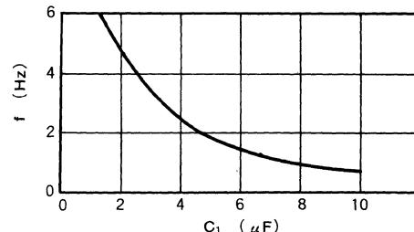
\* If capacitance  $C_1$  is even further reduced, oscillation will be possible up to a frequency of about 10 kHz
