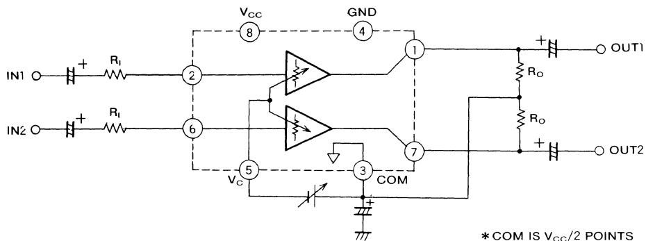
Note: 1.  $R_1$  is used to convert input voltage to current.
