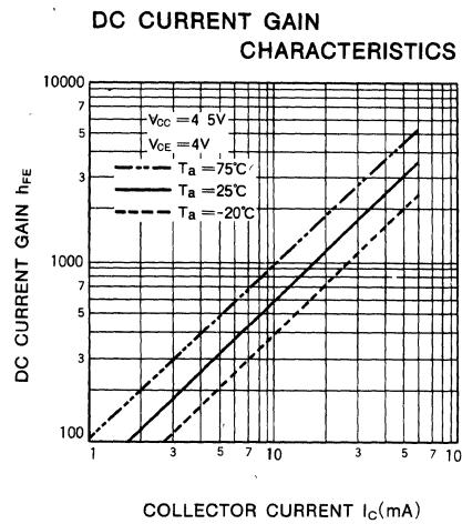
**7-UNIT 350mA TRANSISTOR ARRAY****DESCRIPTION**
