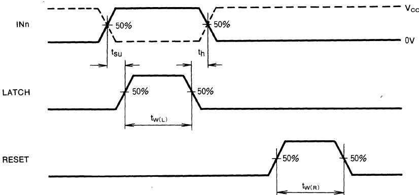
SWITCHING CHARACTERISTICS ( $T_a = +25^\circ\text{C}$ ,  $V_{cc} = 5\text{V}$ )
