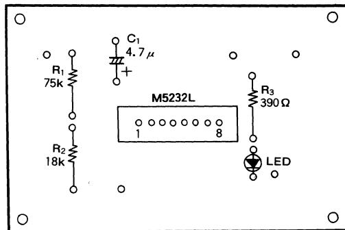
VOLTAGE DETECTOR/ON-OFF ALARM CIRCUIT
