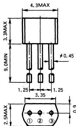
TYPE SOT-89L 3-PIN TRANSISTOR
