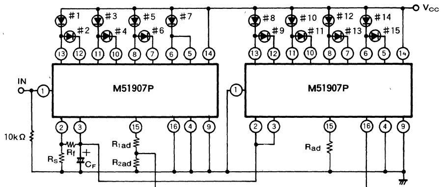
Note 1. To equalize the brightness levels of the M51907P and the M51909P, select  $R_{1ad}$  and  $R_{2ad}$  so that  $R_{ad} = R_{1ad} + R_{2ad}$ .
