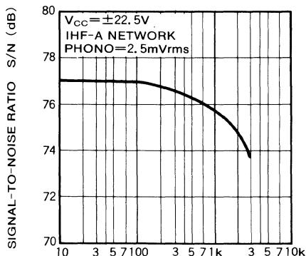
SIGNAL SOURCE RESISTANCE  $R_g$  (Ω)
