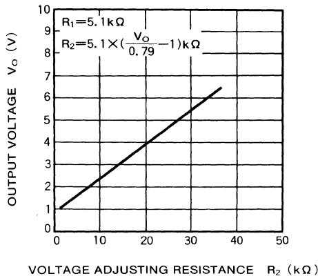
**3V,3-Terminal VARIABLE VOLTAGE OUTPUT REGULATOR (FOR DRIVER)**
