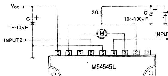
5) Motor speed control by the V<sub>R</sub>
