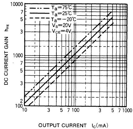
**8-UNIT 500mA SOURCE TYPE DARLINGTON TRANSISTOR ARRAY****DESCRIPTION**
