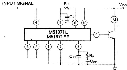
NOTE. The Pin ④ threshold voltage to GND is approximately 1.9V.
