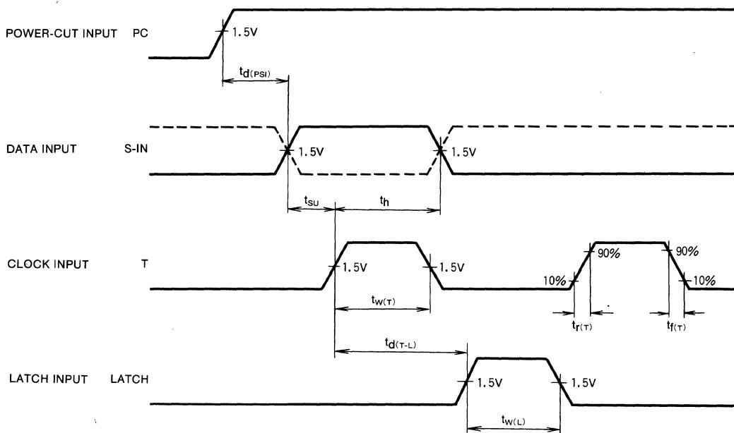
**9-BIT SERIAL-INPUT,LATCHED DRIVER****SWITCHING CHARACTERISTICS** ( $T_a=25^\circ\text{C}$ ,  $V_{CC}=5\text{V}$ )
