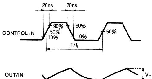
$f_{max}(C_{IN})$  is taken as that frequency  $f_i$  at which the output amplitude ( $V_o$ ) is 1/2 that at 1 kHz.
