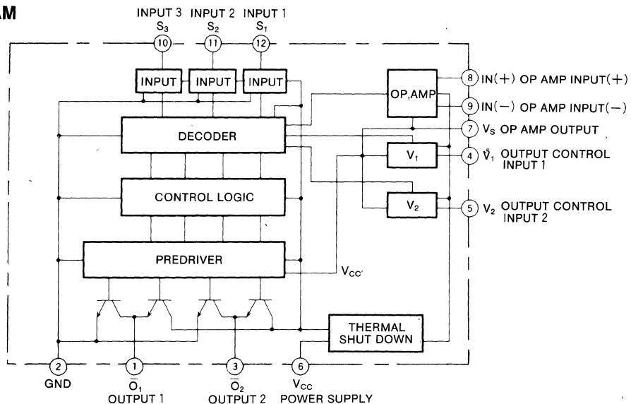
**BI-DIRECTIONAL MOTOR DRIVER WITH MOTOR SPEED CONTROL****ABSOLUTE MAXIMUM RATINGS** ( $T_a=25^\circ\text{C}$ , unless otherwise noted)
