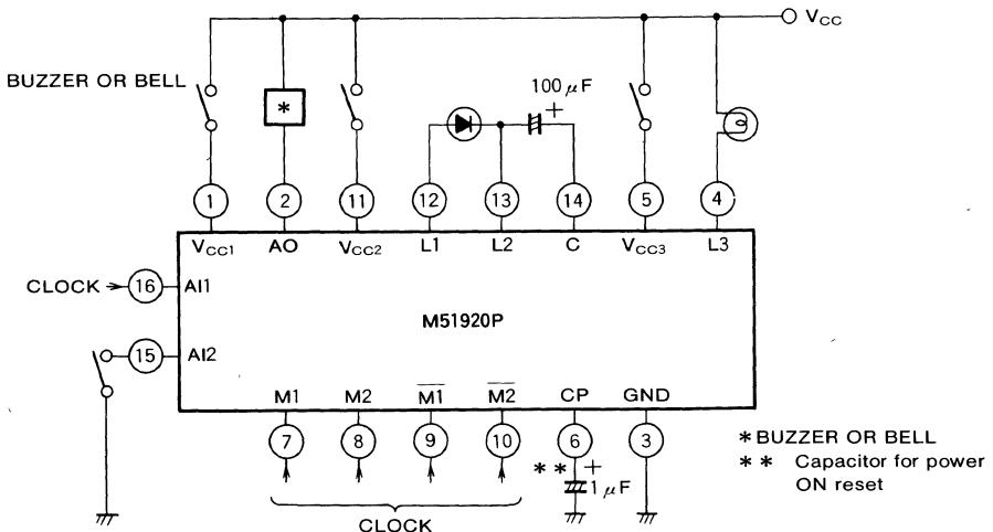
The power supply system is classified as follows:  $V_{CC1}$  for buzzer or bell,  $V_{CC2}$  for LED drive, and  $V_{CC3}$  for timer drive.
