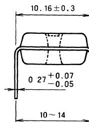
TYPE 32P4B 32-PIN MOLDED PLASTIC DIP (SHRINK)
