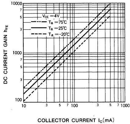
**7-UNIT 150mA DARLINGTON TRANSISTOR ARRAY WITH CLAMP DIODE****DESCRIPTION**
