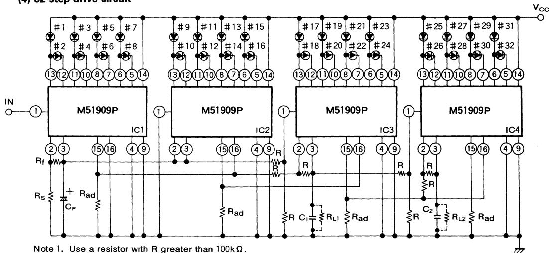
Note 1. Use a resistor with  $R$  greater than  $100\text{k}\Omega$ .
