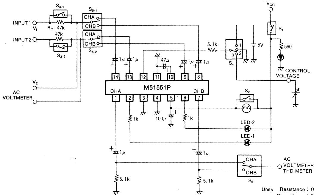
Note : When a dual polarity power supply is used, pin 3 is the  $V_{EE}$  pin (Ground pin 3 for signal polarity supply)
