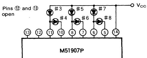
4. When any of LEDs #3 to #8 are not used:
