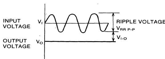
But the input voltage merely increases power dissipation if increased more than necessary, and should be set at the most suitable value.
