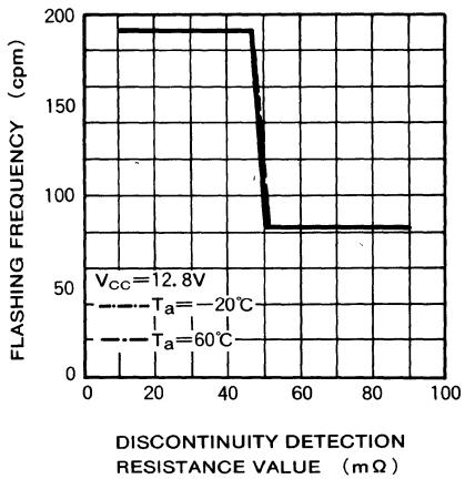
Note 1 For the flashing frequency characteristics the discontinuity detection resistance value has been measured instead of the lamp resistance value.
