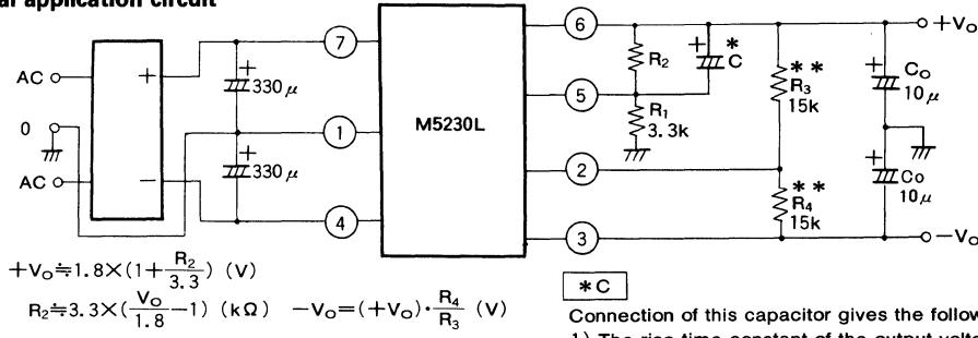
Note When the input power supply lines become long, a  $0.1\mu F$  capacitor should be connected between input power supply pins ⑦ and ④ and ground.
