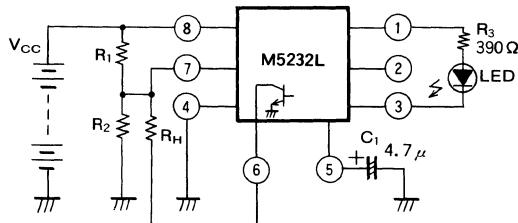
By connecting  $R_H$  across pins ⑥ and ⑦, as shown in the figure on the left, the on/off starting voltage is set at:
