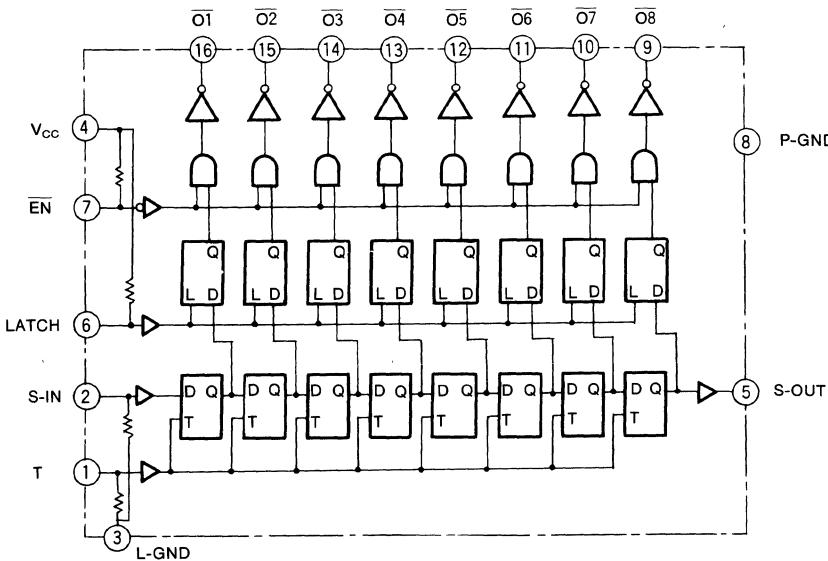
**BI-CMOS 8-BIT SERIAL-INPUT,LATCHED DRIVER**
