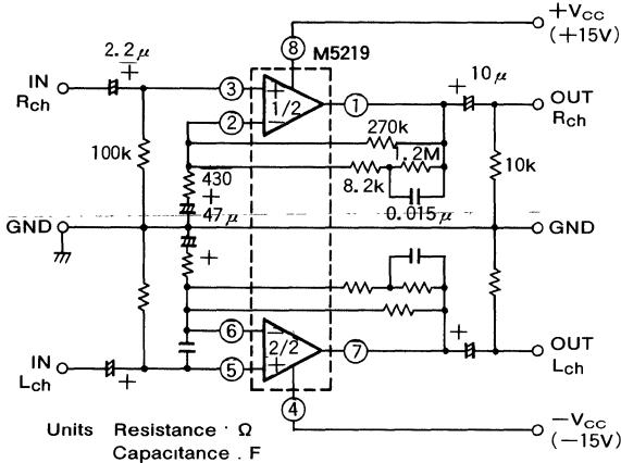
L<sub>ch</sub> circuit constants are identical to those of R<sub>ch</sub>
