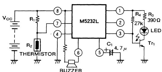
In normal circumstances, the LED is off and power dissipation is kept low. In abnormal circumstances, the LED blinks on and off. It is also possible to sound a buzzer or drive a relay using Pin 6.
