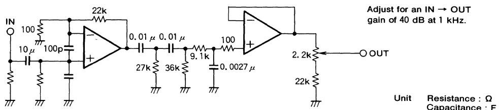
TEST METHODS ( $T_a=25^\circ\text{C}$ ,  $V_{CC}=12\text{V}$ ,  $f=1\text{kHz}$ , unless otherwise noted)
