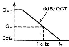
\* Measure frequency characteristics of voltage gain  $G_V$  when a feedback of  $100\%$  ( $1M\Omega$ ) is applied for DC and feedback is open ( $1000pF//470\mu F$ ) for AC. The  $f_T$  can be simply obtained by multiplying voltage gain of  $1kHz$  by frequency.
