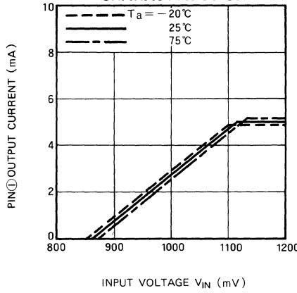
PIN②OUTPUT CURRENT VS INPUT VOLTAGE TEMPERATURE CHARACTERISTICS
