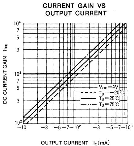
**8-UNIT 30mA PNP TRANSISTOR ARRAY****DESCRIPTION**
