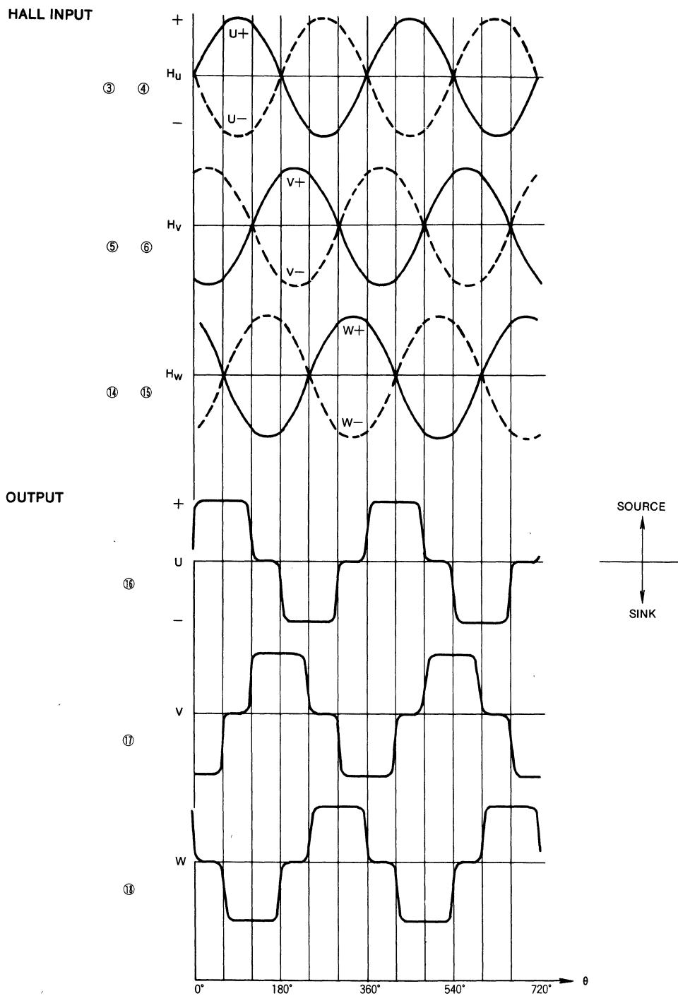
Note 1. The waveforms shown above are different from those at actual motor operation
