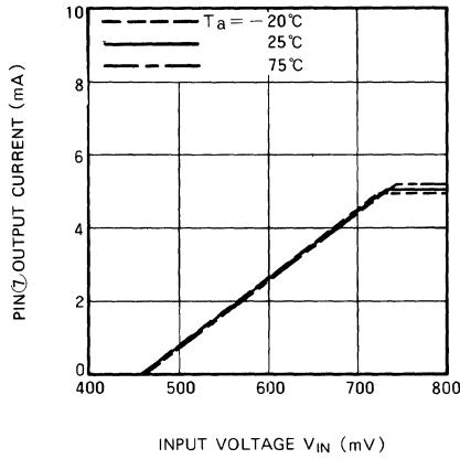
PIN⑧OUTPUT CURRENT VS INPUT VOLTAGE TEMPERATURE CHARACTERISTICS
