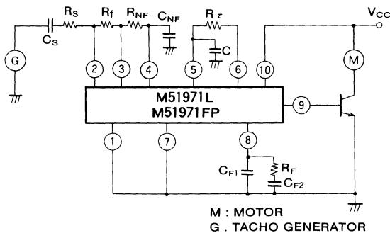
C<sub>S</sub> : Coupling capacitor for AC amplifier
