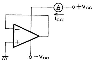
\* If output pin current is maintained at 0 and in quiescent state, the circuit needs not be a voltage follower as shown above.
