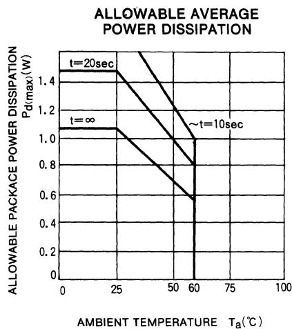
Note 1 : Mounted on an epoxy PC board with Cu cover on one side (5cm×5cm×0.8mm)
