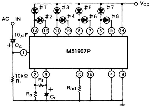
Rad: Resistance determining LED current
