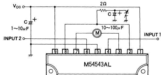
3) Motor speed control by the  $V_{CC}$
