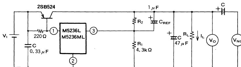
**(b) Ripple rejection test circuit**
