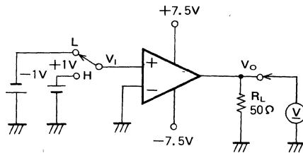
$$V_I \left\{ \begin{array}{l} H \text{ Isource} \\ L \text{ Isink} \end{array} \right.$$
