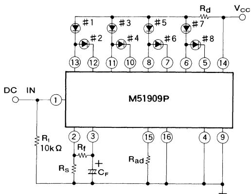
A realistic design involves taking the required output current (LED current:  $I_{LED}$ ) as the allowable maximum output current, and then determining the corresponding output terminal maximum voltage  $V_{O\ max}$  from the ALLOWABLE OUTPUT CURRENT VS. OUTPUT TERMINAL MAX VOLTAGE graph. Then if the maximum value for the supply voltage is  $V_{CC\ max}$ , the value of  $R_d$  has to be determined to satisfy the relation  $4 \cdot I_{LED} \cdot R_d > V_{CC\ max} - V_{O\ max}$ .
