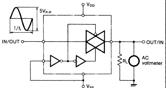
The feedthrough is taken as that frequency  $f_i$ , at which, using a sine-wave input of  $2.5V_{P-P}$ ,  $20 \log_{10}(V_o/V_i) = -50\text{dB}$ .
