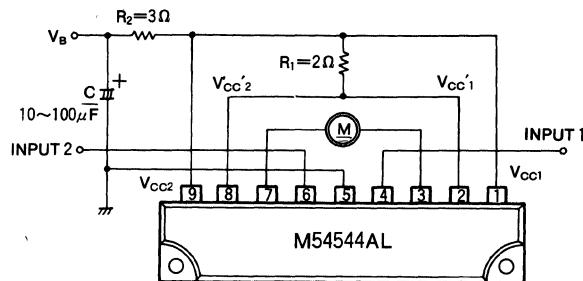
2) Motor speed control by the  $V_{CC}'$
