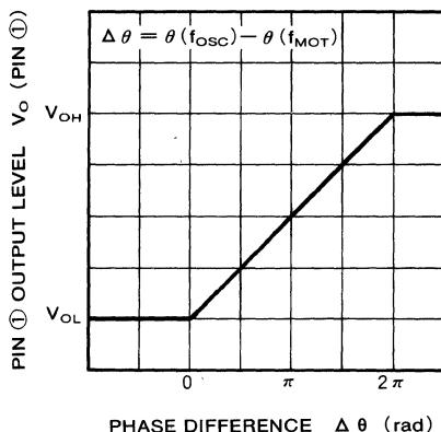
**OUTPUT CHARACTERISTICS OF WAVEFORM REFORM CIRCUIT (INTERNAL)**
