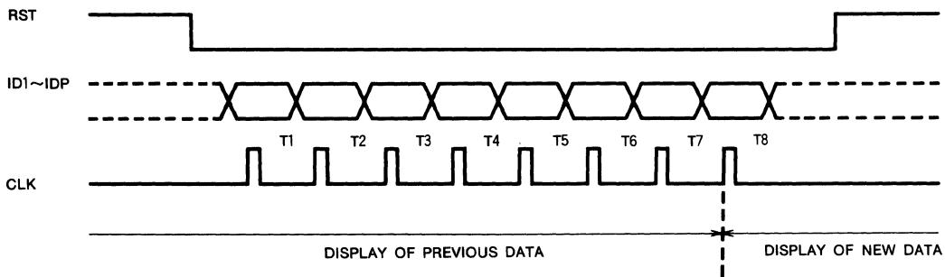
When LOAD is kept at " H ", LOAD is automatically done at the 8th CLK input when RST=" L ". However, while RST=" L ", if there is a 9th CLK input, the 9th data will be loaded and displayed
