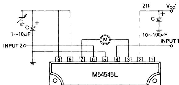
3) Motor speed control by the V<sub>CC'</sub>
