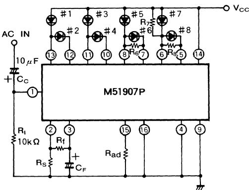
The currents flowing through each of the LEDs in the above circuit configuration are given by the following formulas.
