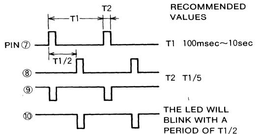
By applying a clock signal to pins ⑦ and ⑧, or ⑨ and ⑩, pin ④ will go "ON" for only a period of  $8 \cdot T_1$  from  $V_{CC3}$  ON; thereafter, pin ④ will be "OFF" until  $V_{CC3}$  is put on again.
