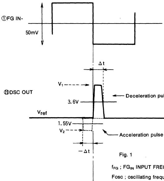
Measure acceleration or deceleration pulse at DOS<sub>OUT</sub> output, applying pulse (synchronous with Fosc) divided by Fosc to FG<sub>IN</sub>-in each mode.
