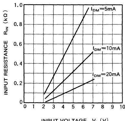
**Fig.2  $I_D - V_I$  CHARACTERISTICS IN APPLICATION EXAMPLE 2**
