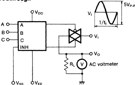
The feedthrough is taken as that frequency  $f_1$  at which, using a sine-wave input of  $2.5\text{V}_{\text{P-P}}$ ,  $20 \log_{10}(V_o/V_i) = -50\text{dB}$ . Refer to the function table for conditions of control inputs A, B, and C.
