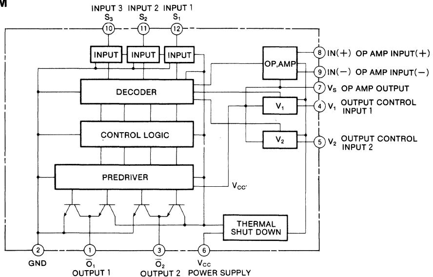
BI-DIRECTIONAL MOTOR DRIVER WITH MOTOR SPEED CONTROL
