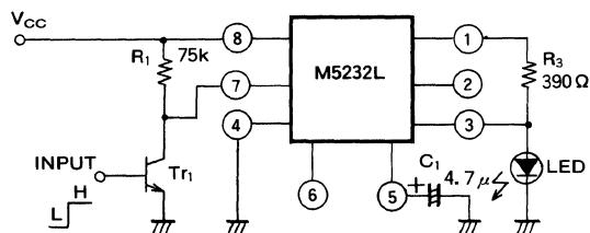
When the base of transistor  $Tr_1$  is set low (the normal condition), Pin 7 comparator voltage is set high, Pin 3 is set low, and the LED is switched off.
