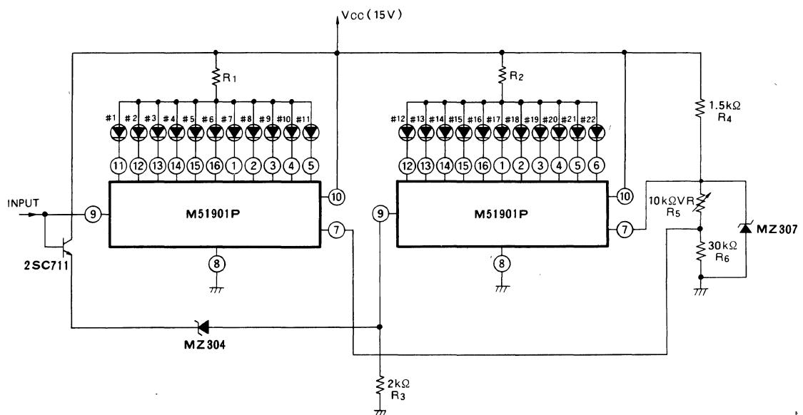
Note      R<sub>5</sub> is chosen such that the lower drive level limit for LED #12 is just 0.24V higher than higher drive level limit for LED #10
