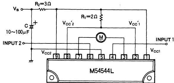
2) Motor speed control by the  $V_{CC'}$
