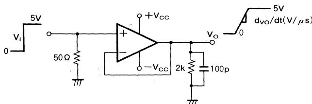
\* Measure high-speed capacity of DUT by reading on an oscilloscope and output pulse response (rising speed) by inputting pulse step in a voltage follower circuit of  $100\%$  feedback.
