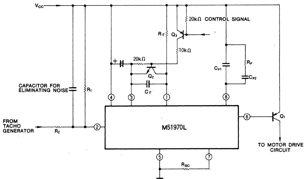
The motor is off when Q<sub>2</sub> and Q<sub>3</sub> are on.
