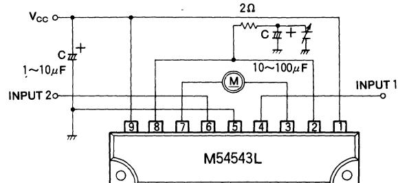
3) Motor speed control by the  $V_{CC}$
