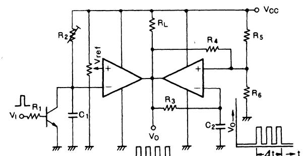
$$dt = C_1 R_2 \cdot \ln \frac{V_{cc}}{V_{cc} - V_{ref}}$$
