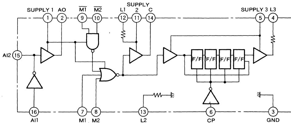
**LOW POWER SUPPLY VOLTAGE INDICATOR, WARNING DRIVER**
