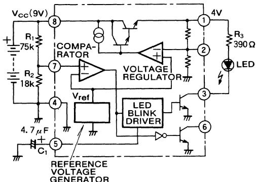
This low voltage checker for batteries is set to start the LED blinking when supply voltage  $V_{CC} = 9V$  (six 1.5V cells) is reduced by 25% (to 6.8V).
