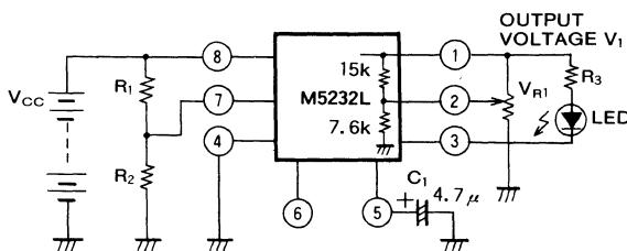
The output voltage  $V_1$  of the M5232L is set by the internal resistor as shown in the figure at left, but this can be changed by connecting a semi-fized resistor across GND and pins ① and ②.
