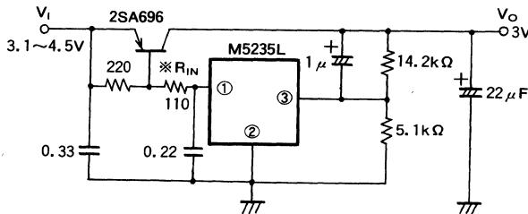
Note1. Resistors ranging from 180Ω to 200Ω should be inserted between the emitter and base of externally connected PNP transistors.
