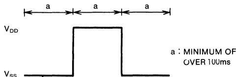
Fig. 3. Input Signal Waveform for the L, M, and PRESET Terminals
