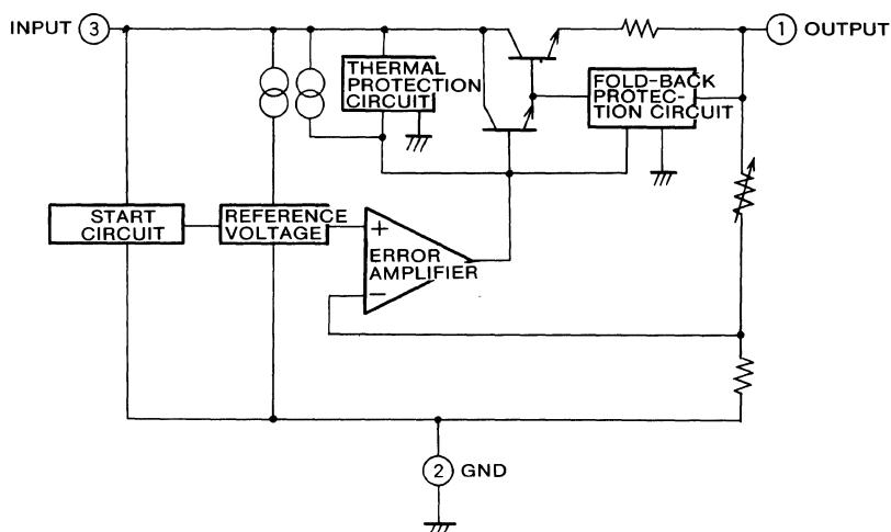
(5V, 5.6V, 8V, 9V, 10V, 12V, 15V) 3-Terminal Fixed Positive Output Voltage Regulator (With Fold-Back Protection Circuit)
