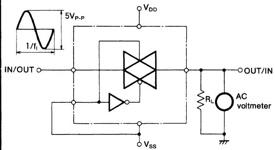
The feedthrough is taken as that frequency  $f_i$  at which, using a sine-wave input of 2.5V<sub>P-P</sub>,  $20 \log_{10}(V_o/V_i) = -50\text{dB}$ .
