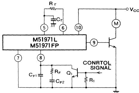
The motor is off when Q<sub>1</sub> is ON.
