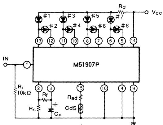
The LED current is determined by  $R_{ad} + R_{cds}$ .
