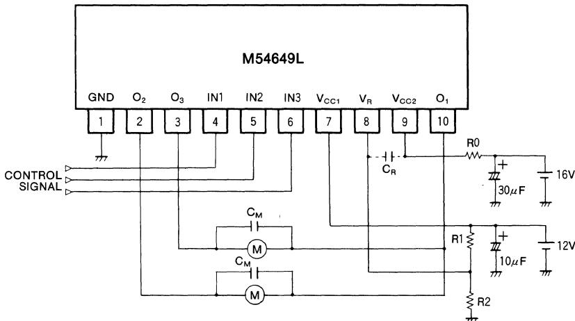
**CM** : Noise absorbing capacitor when the motor is driven should be less than  $0.1\mu F$ .
