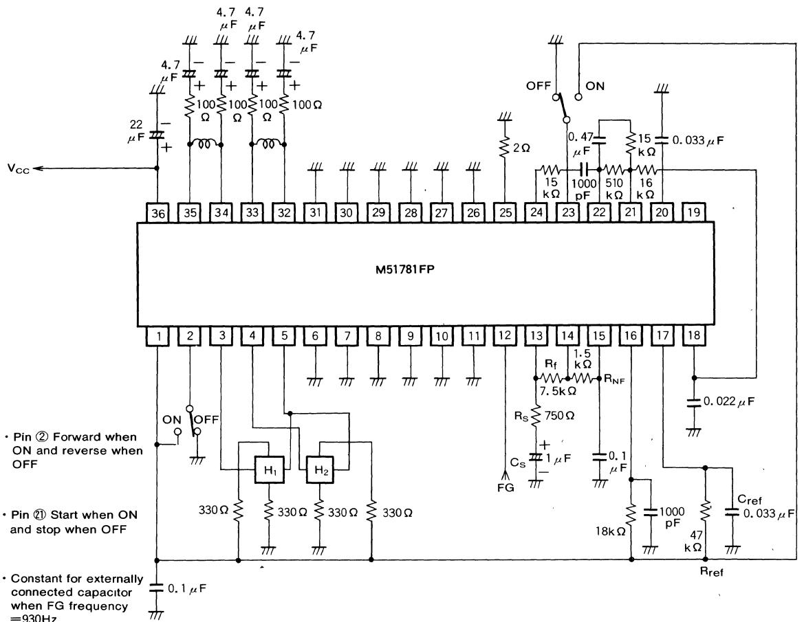
Note 1. The signal amplitude for the input tacho generator should be 1mV<sub>P-P</sub> or more.
