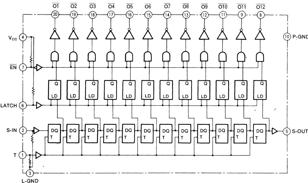
**BI-CMOS 12-BIT SERIAL-INPUT,LATCHED DRIVER**
