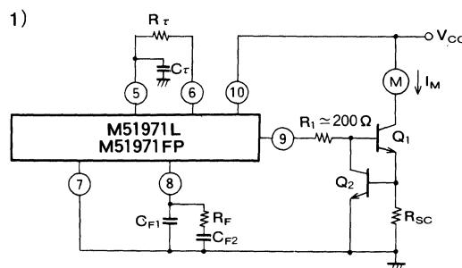
$$I_{M\max} = \frac{V_{BE2}}{R_{SC}} \approx \frac{0.7V}{R_{SC}}$$
