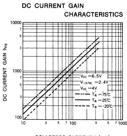
**6-UNIT 320mA TRANSISTOR ARRAY WITH CLAMP DIODE AND STROBE****DESCRIPTION**
