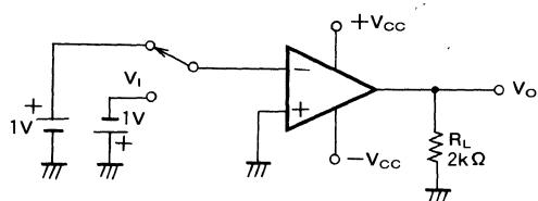
\* DUT is used in open status without feedback and output  $V_O$  is measured by applying  $+1V$  to an input. In this case, the output is saturated when an input is  $1V$  as open gain is high.
