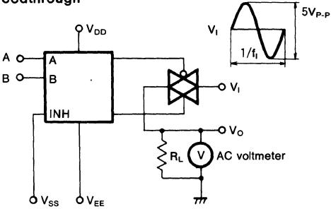
The feedthrough is taken as that frequency  $f_i$  at which, using a sine-wave input of  $2.5 \text{ V}_{\text{P-P}}$ ,  $20 \log_{10}(V_O/V_i) = -50 \text{ dB}$ . Refer to the function table for conditions of control inputs A and B.
