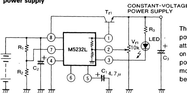
The current capacity of the built-in constant-voltage power supply is approximately 20mA. However, by attaching external transistor  $T_{R1}$  as shown in the figure on the left, it is possible to obtain a constant-voltage power supply with a large current capacity of 1A or more. The output voltage of the power supply can also be varied with variable resistor  $V_{R1}$ .
