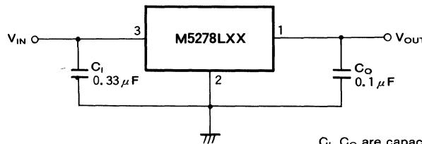
$C_I$ ,  $C_O$  are capacitors to prevent oscillation.
