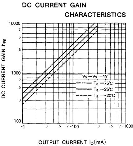
**7-UNIT 150mA SOURCE TYPE DARLINGTON TRANSISTOR ARRAY****DESCRIPTION**
