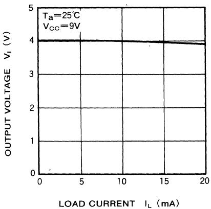
SATURATION VOLTAGE VS. LOAD CURRENT
