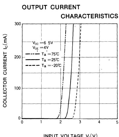
5-UNIT 320mA TRANSISTOR ARRAY WITH STROBE
