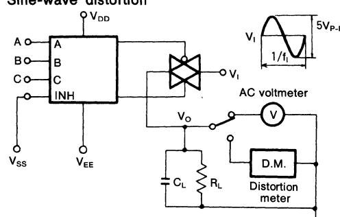
$f_{\text{max}}(\text{I/O})$  is taken as that frequency  $f_i$  at which, using a sine-wave input of  $2.5\text{V}_{\text{P-P}}$ ,  $20 \log_{10}(V_O/V_i) = -3\text{dB}$ . Refer to the function table for conditions of control inputs A, B, and C.
