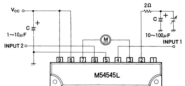
4) Motor speed control by the V<sub>R</sub> and V<sub>CC'</sub>
