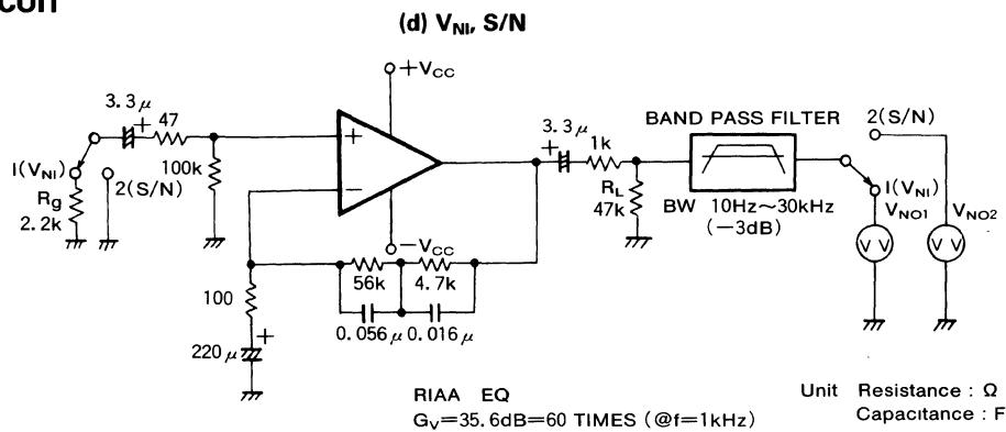
1.  $V_{NI} = V_{NO1}/60 (\mu\text{Vrms})$
