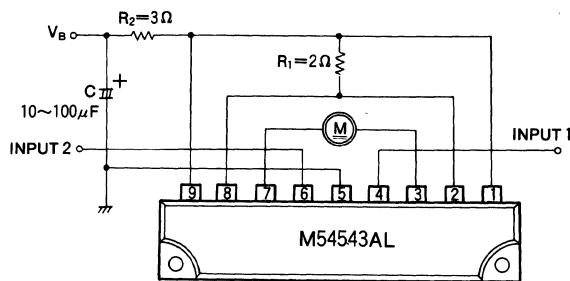
2) Motor speed control by the  $V_{CC'}$
