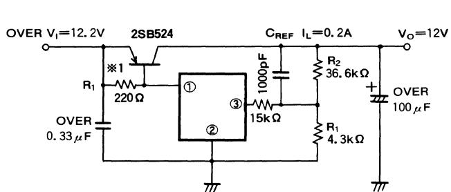
$$V_o = V_{REF} \times \left( 1 + \frac{R_2}{R_1} \right) V$$
