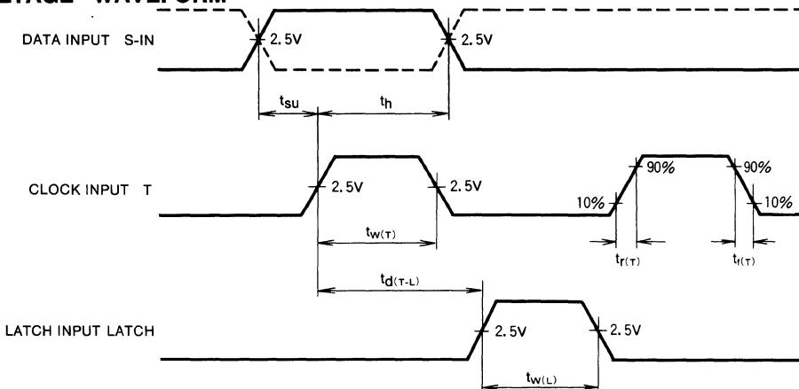
SWITCHING CHARACTERISTICS ( $T_a = +25^\circ\text{C}$ ,  $V_{cc} = 5\text{V}$ )
