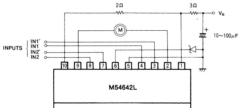
**BI-DIRECTIONAL MOTOR DRIVER WITH MOTOR SPEED CONTROL****DESCRIPTION**
