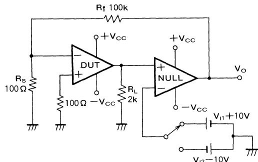
$$\bullet G_{VO} = 20 \log \frac{A_{vd}}{A_{vd} - \frac{R_s + R_f}{R_s} \times \frac{V_{O1} - V_{O2}}{V_{O1} - V_{O2}}} \\ = 10^3 \times \frac{20}{V_{O1} - V_{O2}} \\ = \frac{2 \times 10^4}{V_{O1} - V_{O2}}$$
