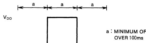
Fig. 2. Input Signal Waveform at the MEMORY Terminal
