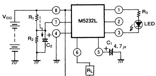
By connecting  $C_2$  in parallel with  $R_2$ ,  $V_{CC}$  is switched on, the charging current indicated by the dotted line in the figure flows, and the LED blinks on and off until the Pin 7 voltage reaches:
