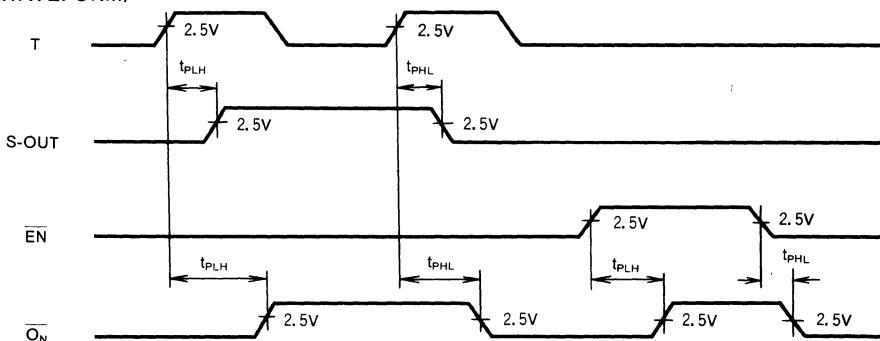
BI-CMOS 8-BIT SERIAL-INPUT,LATCHED DRIVER
