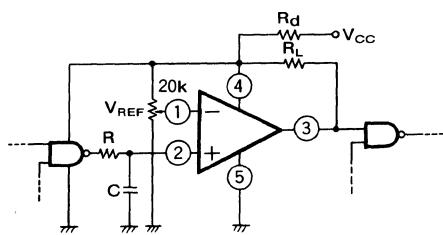
$$t_s = C R \ln \frac{V_{CC}}{V_{CC} - V_{REF}}$$
