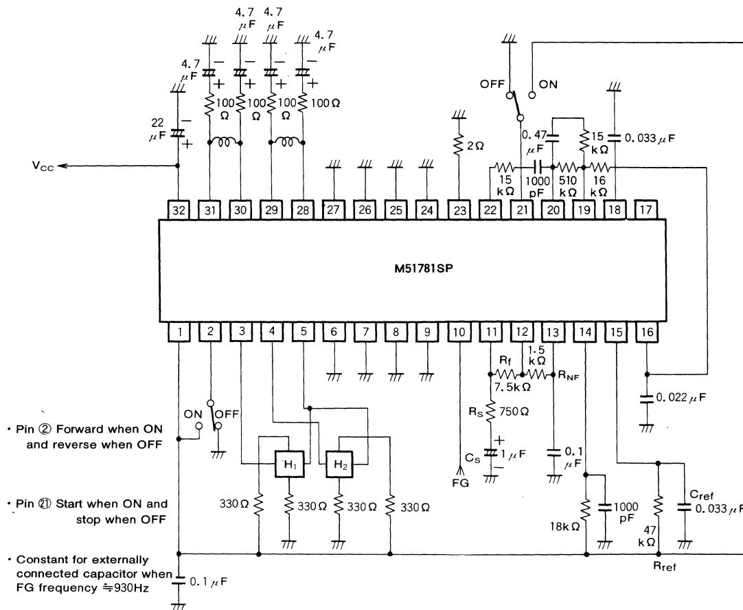
Note 1. The signal amplitude for the input tacho generator should be  $1\text{mV}_{\text{P-P}}$  or more.
