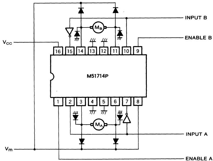
Note. A diode of small  $V_F$  is used between clamps. (For example, Schottky diode)
