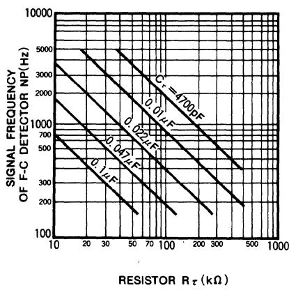
$R_\tau$ ,  $C_\tau$  determine the speed of motor
