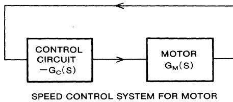
The speed control system for the motor is a negative feedback system, including control circuit and motor.
