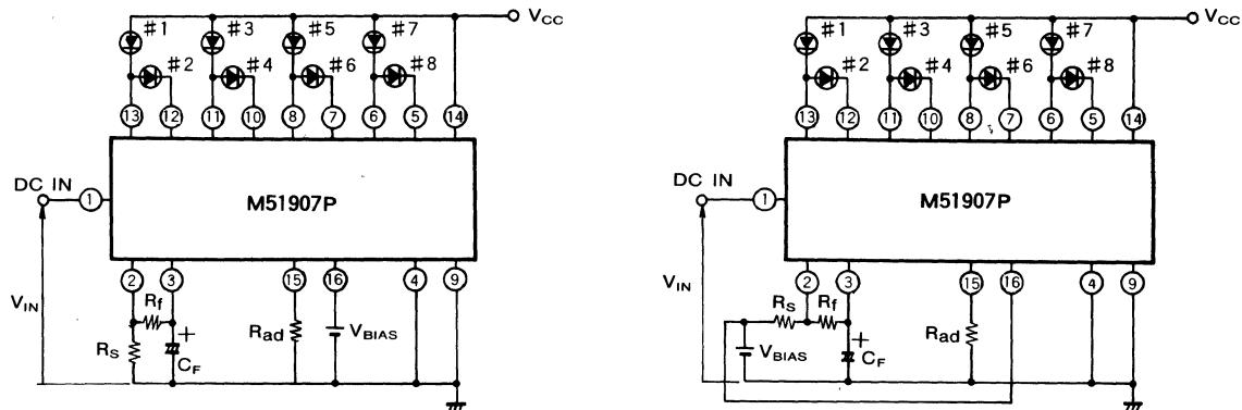
Display is given by the formula  $V_{IN} \times \frac{R_s + R_f}{R_s} - V_{BIAS}$
