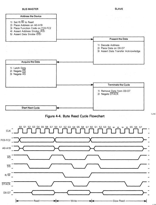
Figure 4-5. Read and Write Cycle Timing Diagram
