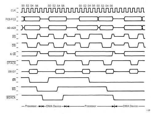
Figure 4-15. Bus Arbitration Timing for the 52-Pin Version
