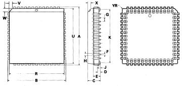
NOTES: 1. DIMENSIONS R AND U DO NOT INCLUDE MOLD FLASH. 2. DIMENSIONING AND TOLERANCING PER ANSI Y14.5M, 1982. 3. CONTROLLING DIMENSION: INCH
