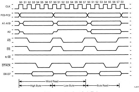
Figure 4-6. Word and Byte Read Cycle Timing
