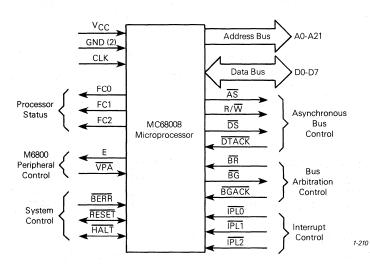
Figure 4-1. Input and Output Signals (Continued)
