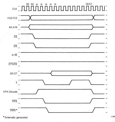
Figure 6-2. M6800 Cycle Timing
