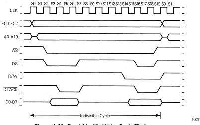
Figure 4-11. Read-Modify-Write Cycle Timing
