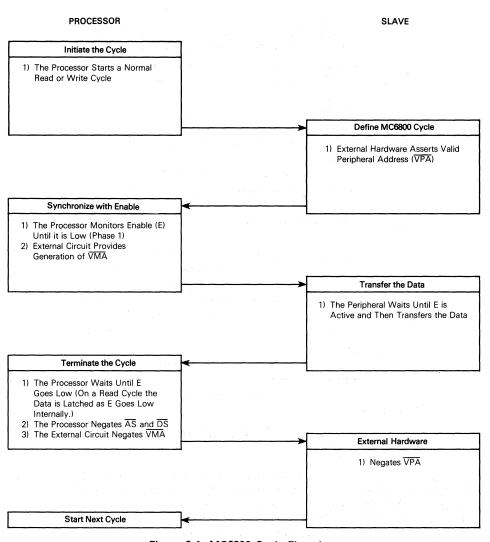
Figure 6-1. MC6800 Cycle Flowchart
