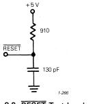
Figure 8-2. RESET Test Load
