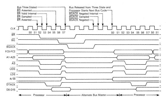
Figure 4-18. Bus Arbitration Timing Diagram-Processor Active
