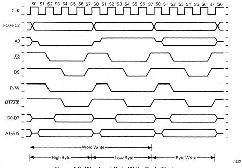
Figure 4-9. Word and Byte Write Cycle Timing
