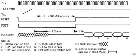
Figure 4-26. System Reset Timing Diagram
