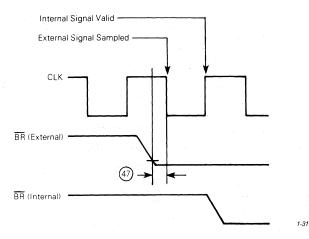
Figure 4-17. Timing Relationship of External Asynchronous Inputs to Internal Signals
