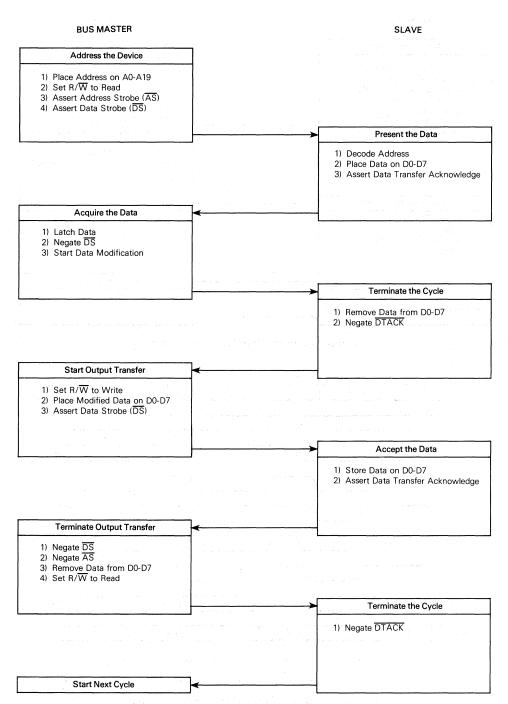
Figure 4-10. Read-Modify-Write Cycle Flowchart
