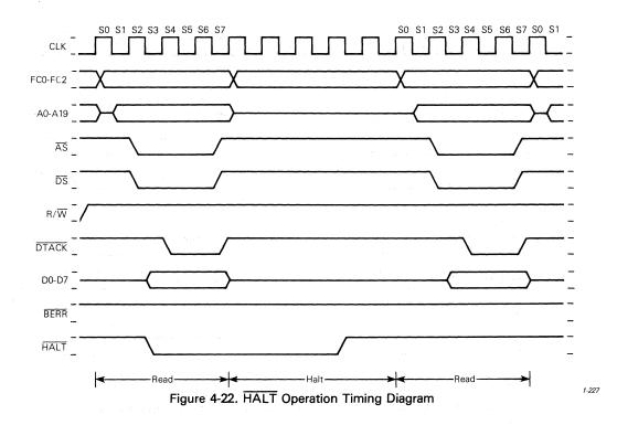
The single-step mode is derived from correctly timed transitions on the halt signal input. It forces the processor to execute a single bus cycle by entering the "run" mode until the processor starts a bus cycle then changing to the "halt" mode. Thus, the single-step mode allows the user to proceed through (and therefore debug) processor operations one bus cycle at a time.
