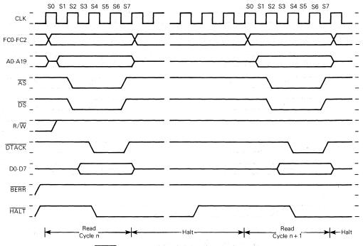
Figure 4-23. HALT Signal Single-Step Operation Timing Characteristics
