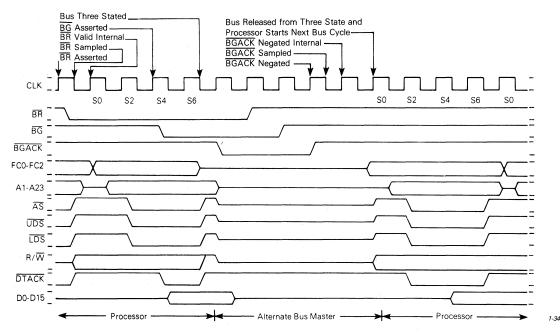
Figure 4-20. Bus Arbitration Timing Diagram—Special Case
