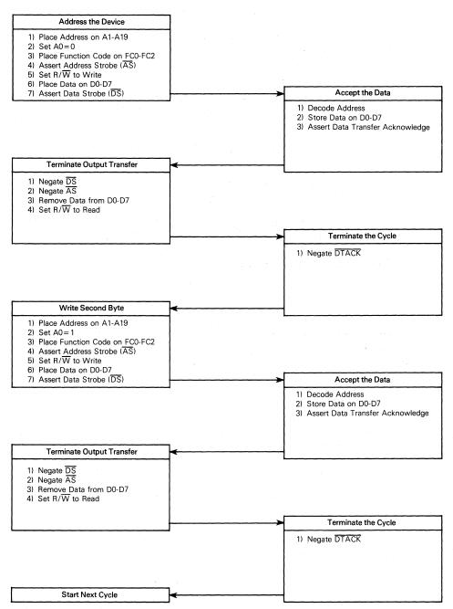
Figure 4-7. Word Write Cycle Flowchart
