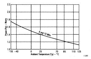
Figure 8-1. MC68008 Power Dissipation (PD) vs Ambient Temperature (TA)
