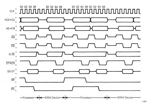
Figure 4-14. Bus Arbitration Timing for the 48-Pin Version
