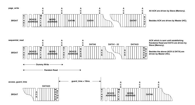
Figure 8-2. I<sup>2</sup>C Timing Chart
