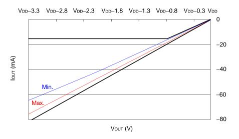
Figure 10-3. Full-speed Buffer Vol/lol Characteristics for High-speed Capable Transceiver
