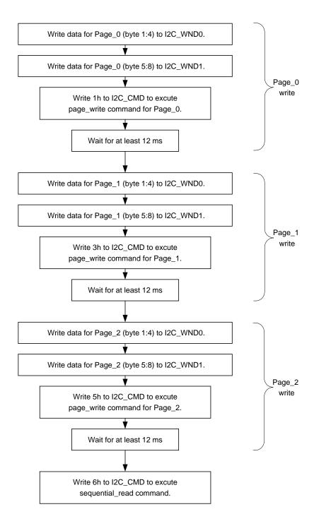
Figure 8-3. External Serial ROM Setting Flowchart
