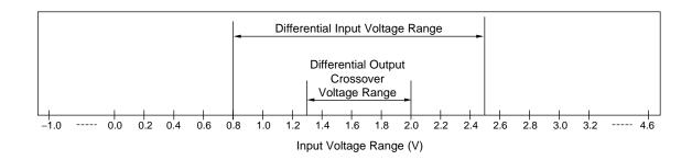
Figure 10-2. Full-speed Buffer Voн/loн Characteristics for High-speed Capable Transceiver
