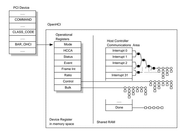
Figure 4-1. OpenHCI's PCI Configuration Space
