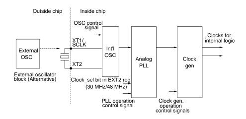
Figure 7-3.  $\mu$ PD720101's Clock System
