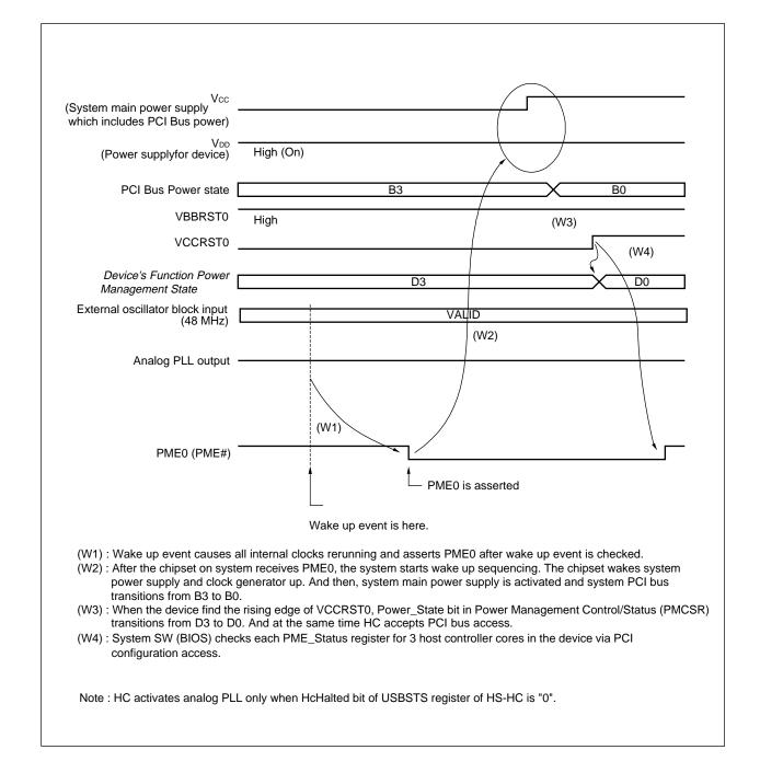
Figure 7-5. Clock Operation Diagram (Using 48-MHz Oscillator)
