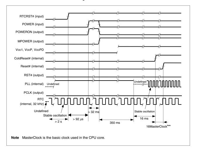
Figure 6-1. RTC Reset
