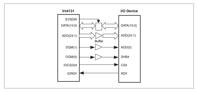
Figure 7-1. Connection with 16-Bit I/O Device Interface
