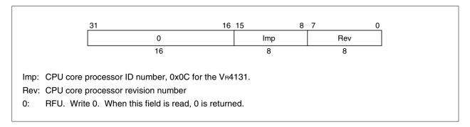
The processor revision number is stored as a value in the form y.x, where y is a major revision number in bits 7 to 4 and x is a minor revision number in bits 3 to 0.
