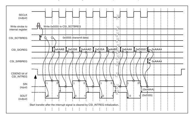
Figure 21-2. Single Transfer Mode (16-Bit Transfer)
