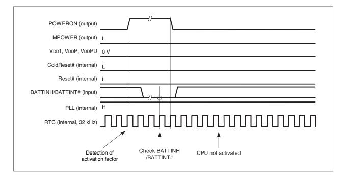
Figure 6-7. VR4131 Activation Sequence (When Not Activating)
