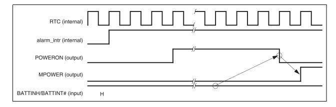
Figure 12-8. Activation via Elapsed Timer Interrupt (BATTINH/BATTINT# = 0)
