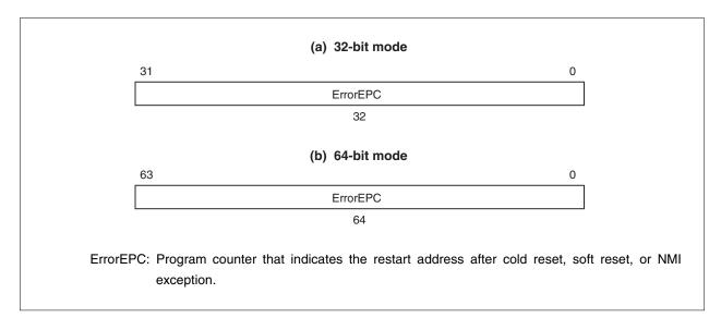
Figure 5-27. ErrorEPC Register Format (When MIPS16ISA Is Disabled)
