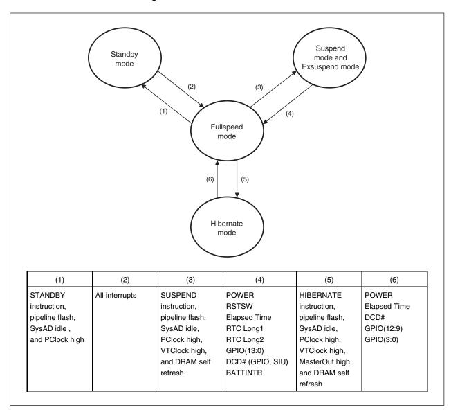
Figure 12-9. Power Mode State Transition
