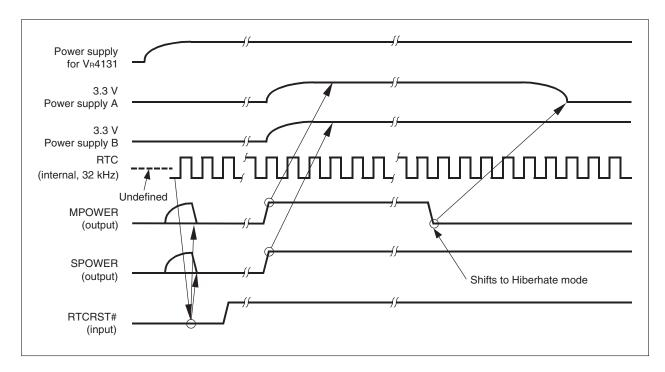
Figure 6-2. Power Supply Control Timing When Using SDRAM
