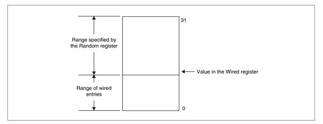
The Wired register is set to 0 upon cold reset. Writing this register also sets the Random register to the value of its upper limit (see **5.1.2 Random register (1)**). Figure 5-7 shows the format of the wired register.
