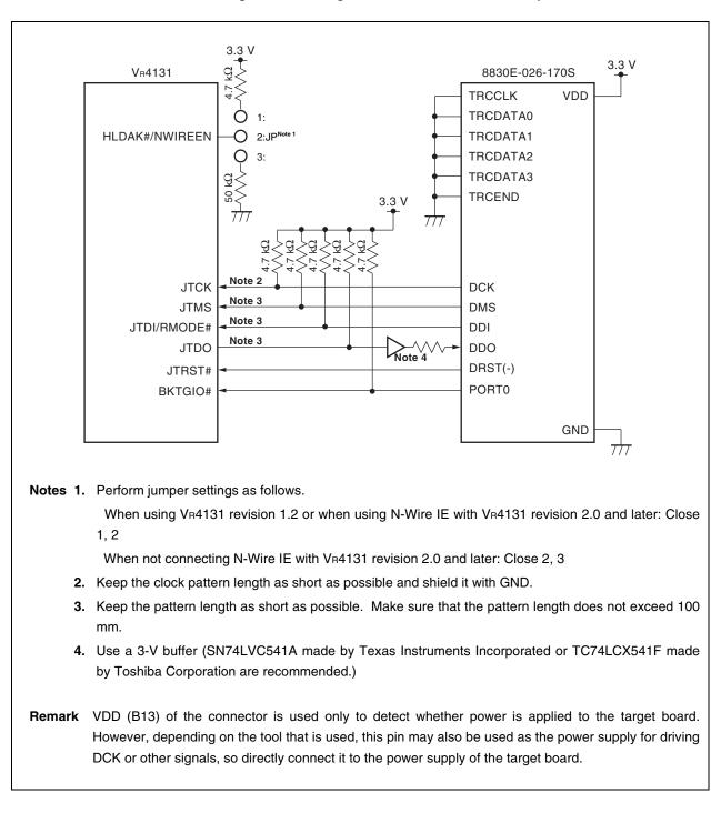
Figure A-1. Debug Tool Connection Circuit Example
