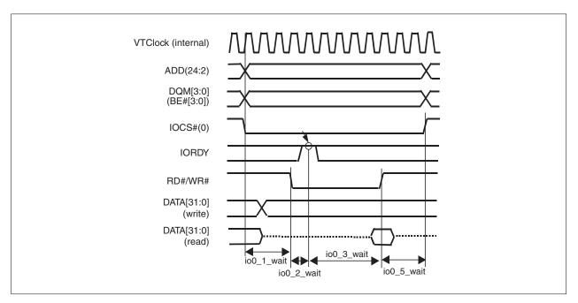
Figure 7-11. Setting Access Time by S/W for 4-Byte Access to I/O Space via 32-Bit Bus (io0\_1\_wait = 0010, io0\_2\_wait = 0010, io0\_3\_wait = 0010, io0\_5\_wait = 10, No Wait)
