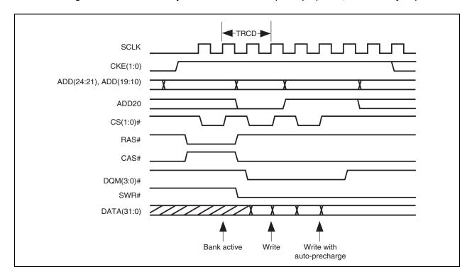
Figure 16-2. Block Write Cycle in 32-Bit Bus Mode (TRCD(2:0) = 010, CAS Latency = 2)
