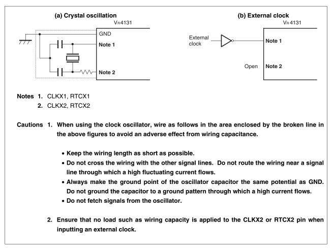
Figure 1-10. External Circuits of Clock Oscillator
