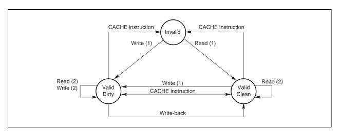
Figure 9-6. Data Cache State Diagram
