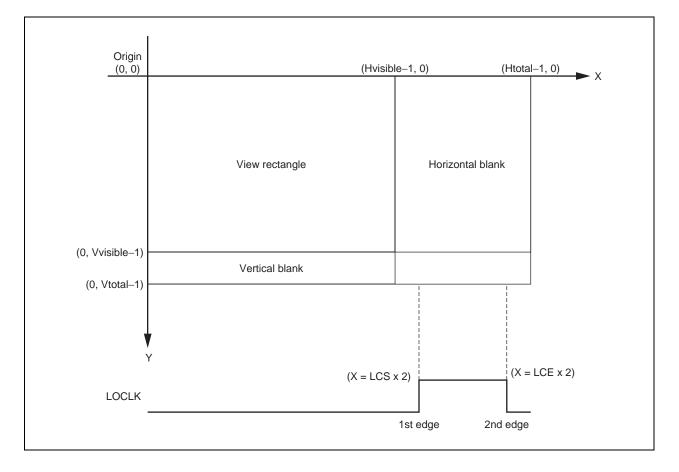
Figure 26-3. Position of Load Clock, LOCLK
