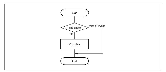
Figure 9-16. Data Check Flow on Hit\_Invalidate Operations
