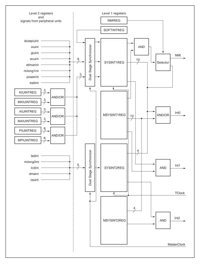
Figure 14-1. Peripheral Logic Block Assignment for Interrupt Registers
