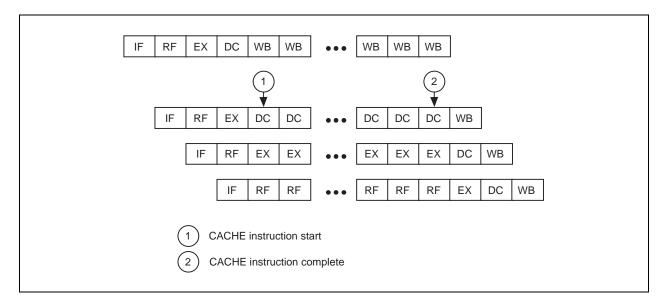
When the CACHE instruction enters the DC pipe-stage, the pipeline stalls while the CACHE instruction is executed. The pipeline begins running again when the CACHE instruction is completed, allowing the instruction fetch to proceed.
