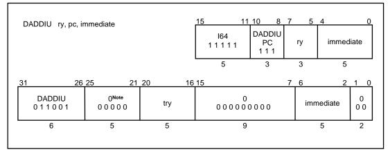
**Note** Zeros are shown in the field of bits 21 to 25 as placeholders. The 32-bit PC-relative instruction format shown above is provided here only to make the description complete; it is not a valid 32-bit MIPS instruction. Please see Chapter 4 for a complete definition of the semantics of the MIPS16 PC-relative instructions.
