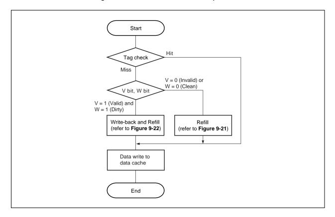
Figure 9-10. Data Check Flow on Store Operations
