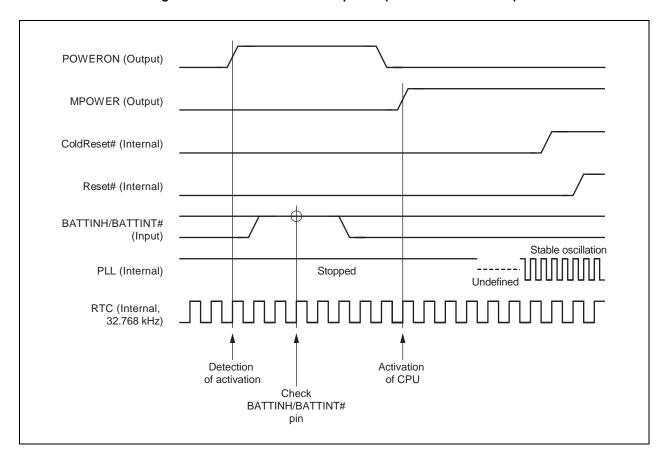
Figure 8-6. VR4181 Activation Sequence (when activation is OK)
