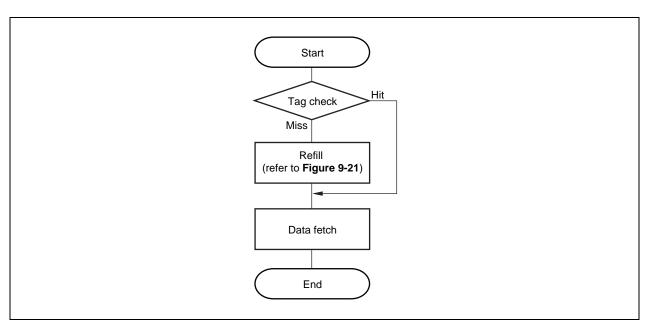
Figure 9-8. Data Check Flow on Instruction Fetch
