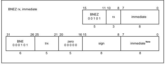
**Note** In MIPS16 mode, the branch offset is interpreted as halfword aligned. This is unlike 32-bit MIPS mode which interprets the offset value as word aligned. The 32-bit branch instruction format shown above is provided here only to make the description complete; it is not a valid 32-bit MIPS instruction. Please see Chapter 3 and Chapter 27 for a complete definition of the semantics of the MIPS16 branch instructions.
