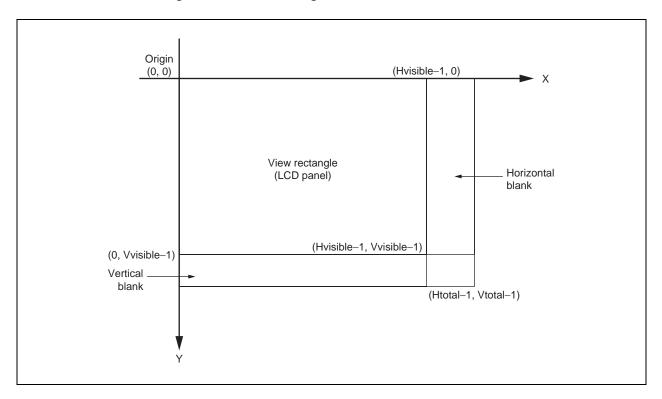
Figure 26-2. View Rectangle and Horizontal/Vertical Blank
