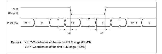
The polarity of FLM is programmable by FLMPOL bit. XS and XE are discussed in timing diagrams.
