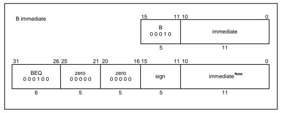
**Note** In MIPS16 mode, the branch offset is interpreted as halfword aligned. This is unlike 32-bit MIPS mode which interprets the offset value as word aligned. The 32-bit branch instruction format shown above is provided here only to make the description complete; it is not a valid 32-bit MIPS instruction. Please see Chapter 3 and Chapter 27 for a complete definition of the semantics of the MIPS16 branch instructions.
