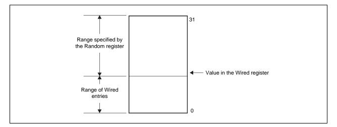
The Wired register is set to 0 upon Cold Reset. Writing this register also sets the Random register to the value of its upper bound (see **6.5.2 Random register (1)**). Figure 6-16 shows the format of the Wired register.
