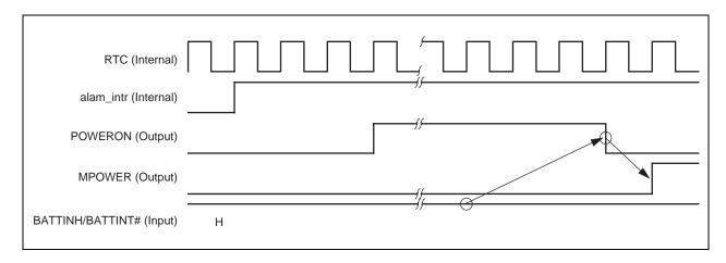
Figure 15-10. Activation via Alarm Interrupt (BATTINH = H)
