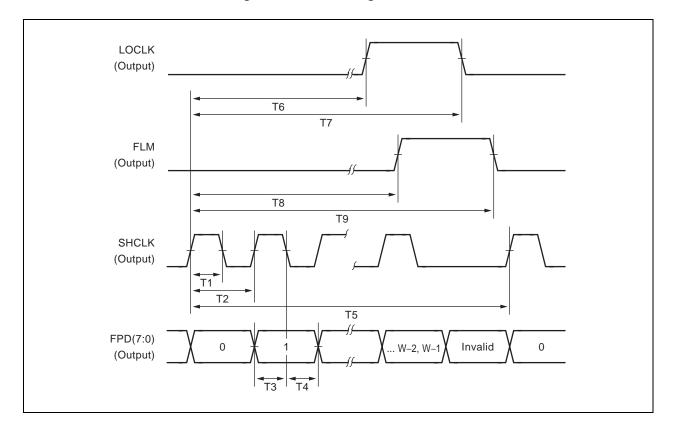
Figure 26-9. LCD Timing Parameters
