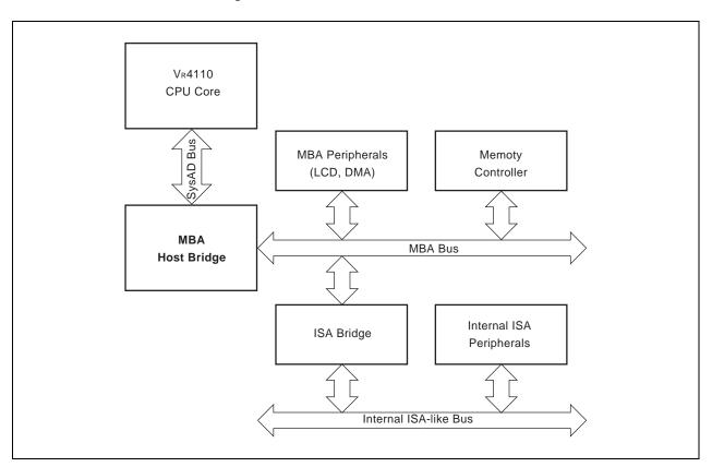
Figure 11-1. VR4181 Internal Bus Structure
