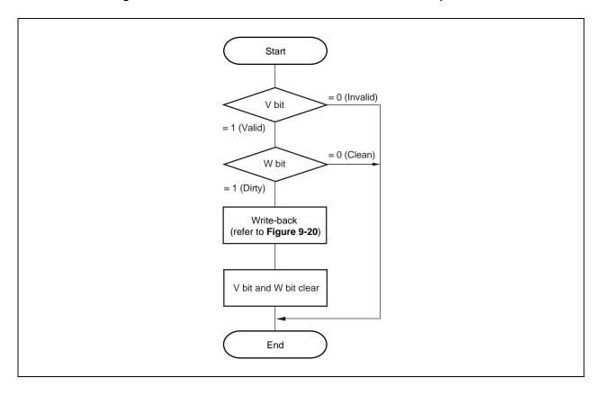
Figure 9-12. Data Check Flow on Index\_Writeback\_Invalidate Operations
