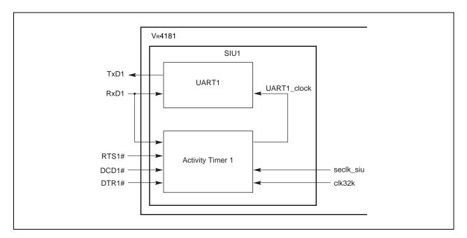
Figure 24-1. SIU1 Block Diagram
