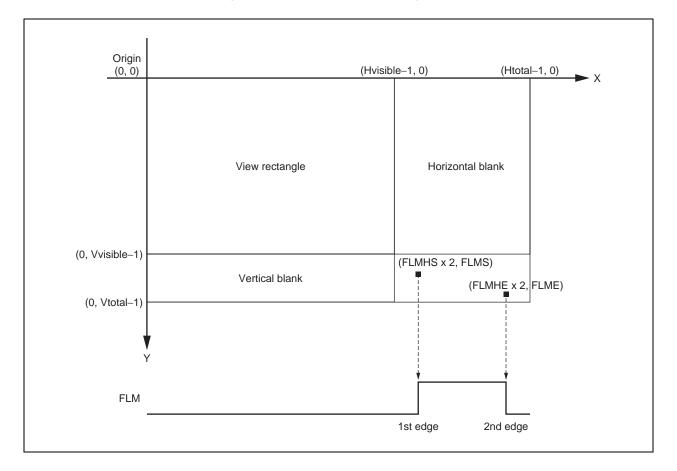
Figure 26-4. Position of Frame Edge, FLM
