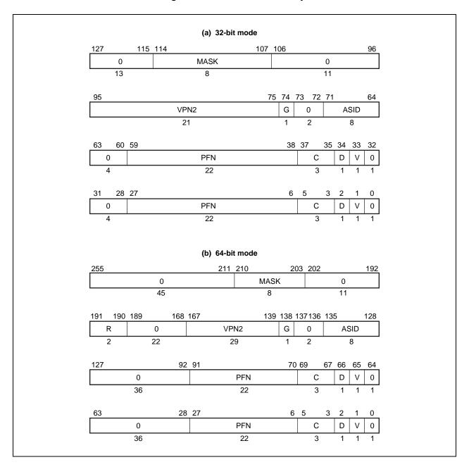
Figure 6-10. Format of a TLB Entry
