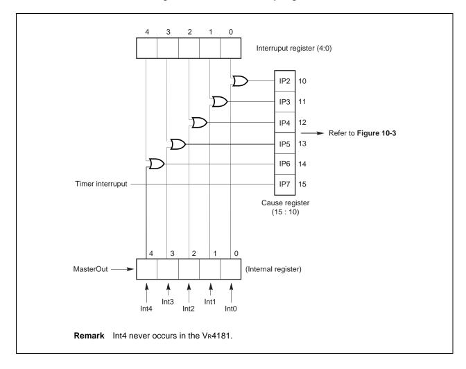
Figure 10-2. Hardware Interrupt Signals
