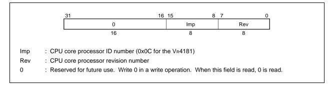
The low-order byte (bits 7:0) of the PRId register is interpreted as a revision number, and the high-order byte (bits 15:8) is interpreted as an implementation number. The processor revision number is stored as a value in the form y.x, where y is a major revision number in bits 7 to 4 and x is a minor revision number in bits 3 to 0.
