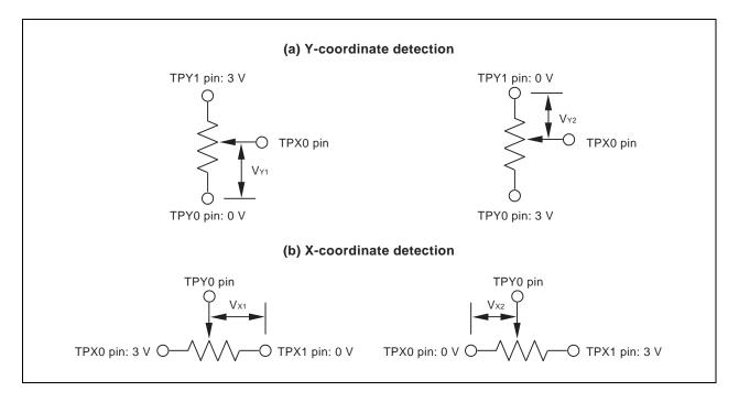
Figure 19-2. Coordinate Detection Equivalent Circuits
