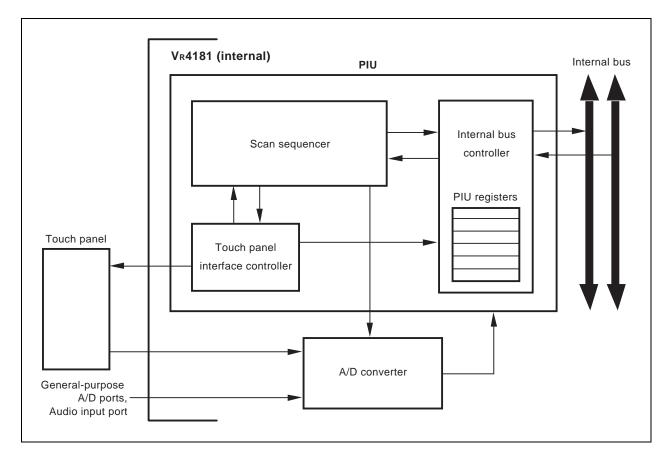
The PIU includes three blocks: an internal bus controller, a scan sequencer, and a touch panel interface controller.
