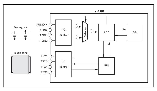
Figure 19-1. PIU Peripheral Block Diagram
