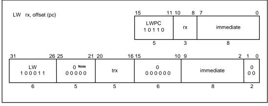
**Note** Zeros are shown in the field of bits 21 to 25 as placeholders. The 32-bit PC-relative instruction format shown above is provided here only to make the description complete; it is not a valid 32-bit MIPS instruction. Please see Chapter 4 for a complete definition of the semantics of the MIPS16 PC-relative instructions.
