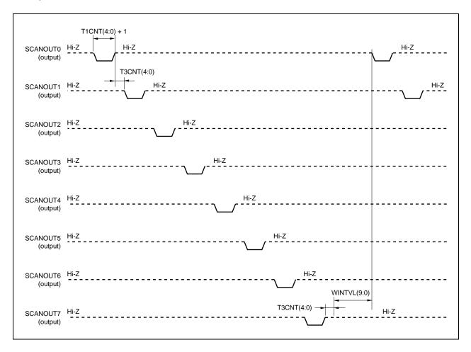
T1CNT(4:0) specifies the keyboard settling time and is expressed in 32.768 kHz clock cycles. Following activation of one of the SCANOUT(7:0) pins, the KIU will wait until the T1CNT(4:0) time before reading return data from the SCANIN(7:0) pins. The actual SCANOUT pins will be driven as low for (T1CNT(4:0) + 1) 32.768kHz clock cycles.
