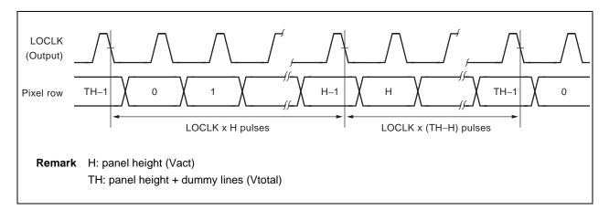
Remark Dummy lines are inserted when needed. For example, some panels can display only 240 lines, but has 242 line cycles. Load clock can be deactivated for the dummy lines (see DummyL bit description in 26.4.6).
