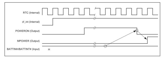
Figure 15-4. Activation via CompactFlash Interrupt Request (BATTINH = H)
