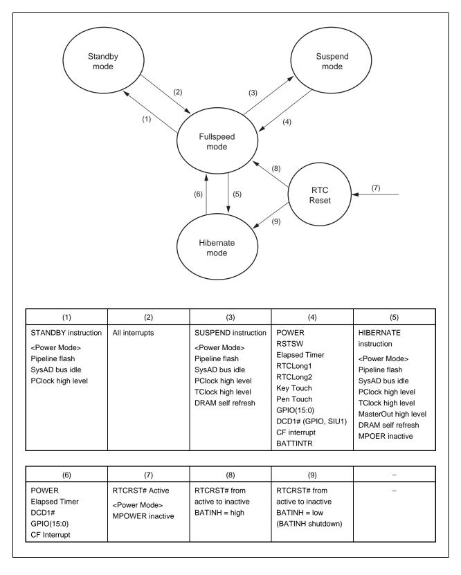
Figure 15-12. Transition of VR4181 Operating Mode (Power Mode)
