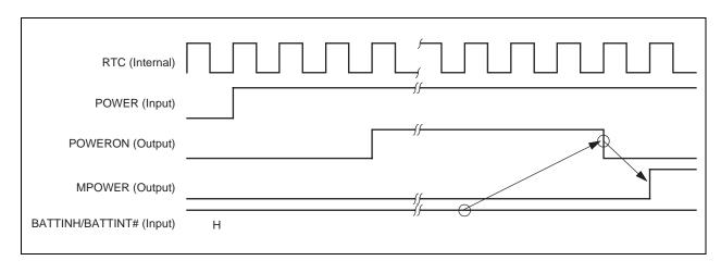
Figure 15-2. Activation via Power Switch Interrupt Request (BATTINH = H)
