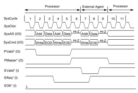
Figure 13-15 Processor Write Requests Followed by External Write Request
