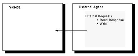
Figure 12-4 External Requests to Processor
