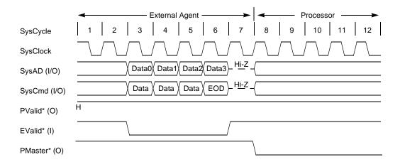
Figure 13-20 Block Read Response in Slave State
