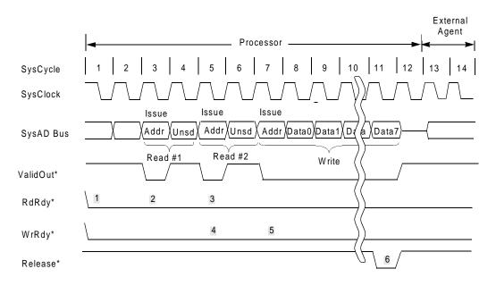
Figure 11-16 Multiple-Split-Read Cycles with Two Reads Split by One Write
