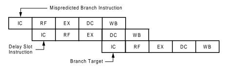
Figure 3-3 CPU Pipeline Branch Delay
