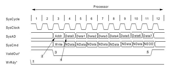
Figure 11-7 Processor Block Write Request
