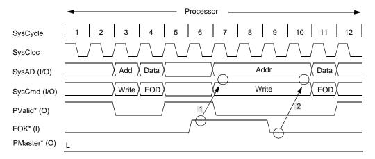
Figure 13-10 Delayed Second Processor Write Request
