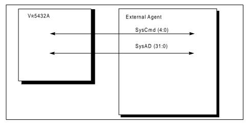
Figure 9-2 System Interface Buses in R43K Mode
