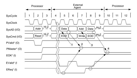
Figure 13-21 External Write Request Following Read Request
