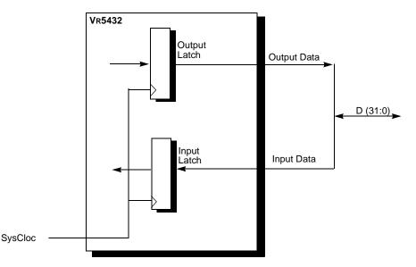
Figure 13-3 System Interface Register-to-Register Operation
