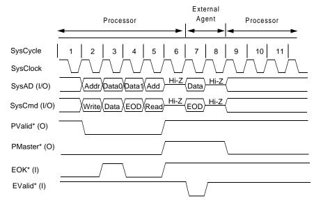
Figure 13-13 Processor Write Request Followed by Processor Read Request
