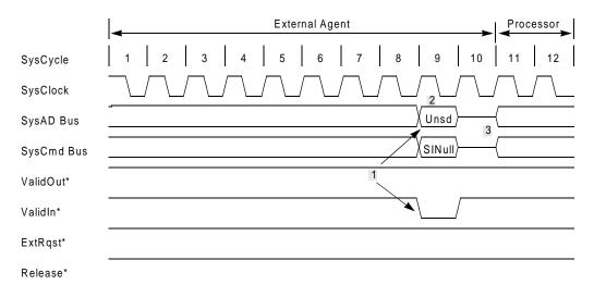
Figure 11-20 System Interface Release External Null Request
