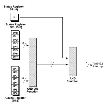
Figure 6-28 Masking of VR5432 Interrupts
