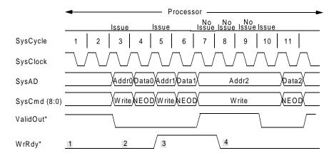
Figure 11-13 Pipelined Write Cycles
