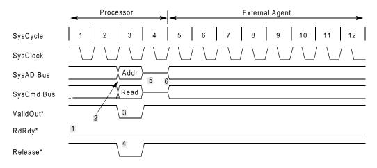
Figure 11-5 Processor Read Request Protocol
