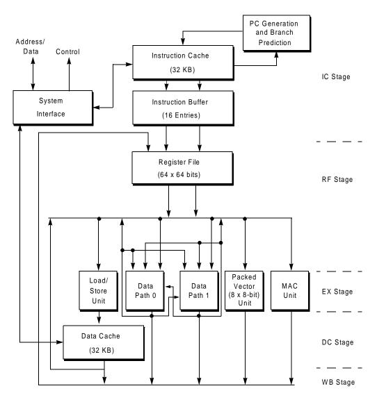
Figure 3-2 Dual-Issue Mechanism
