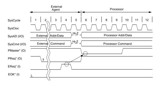
Figure 13-17 Bus Arbitration by the Processor
