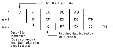
Figure 3-4 CPU Pipeline Load Delay
