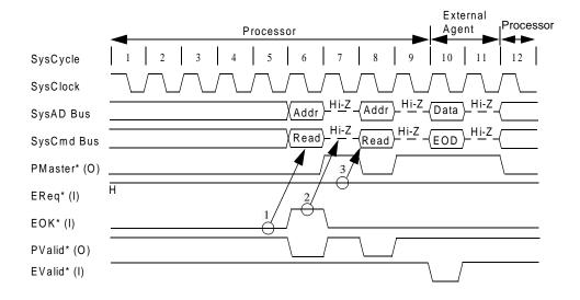
Figure 13-24 Discarding and Re-Executing a Processor Single Read Request
