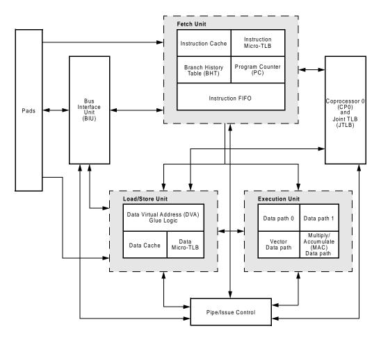
Figure 1-1 Block Diagram
