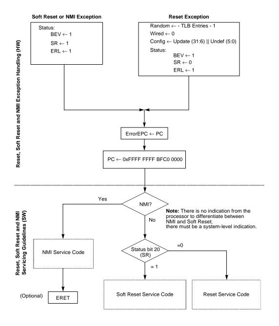
Figure 6-24 Reset, Soft Reset, and NMI Exception Handling
