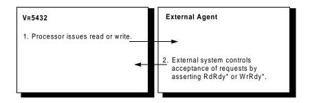
Figure 10-3 Processor Request Flow Control
