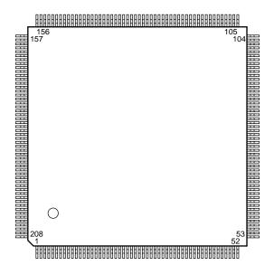
Figure 2-2 208-Pin PQFP Orientation (Top View)
