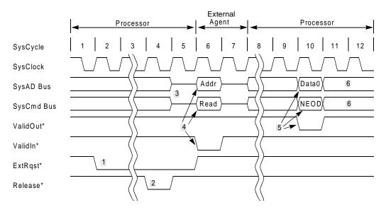
Figure 11-19 External Read Request, System Interface in Master State
