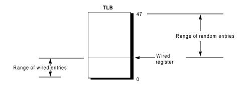
Figure 4-16 Wired Register Boundary
