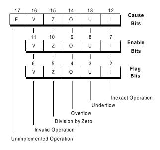
Figure 7-4 Control/Status Register Cause, Flag, and Enable Fields
