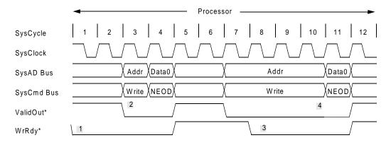
Figure 11-9 Two Processor Write Requests with Second Write Delayed
