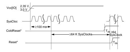
Figure 14-1 Power-On Reset Timing Diagram
