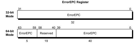
Figure 6-14 ErrorEPC Register Format
