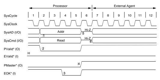
Figure 13-6 Delayed Processor Read Request
