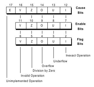
Figure 8-1 Control/Status Register Exception/Flag/Trap/Enable Bits
