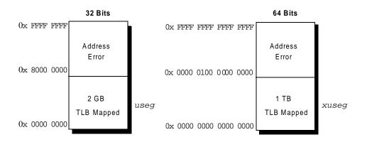
Figure 4-6 Virtual Address Space in User Mode
