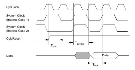
Figure 15-4 Bypass PLL Reset Timing
