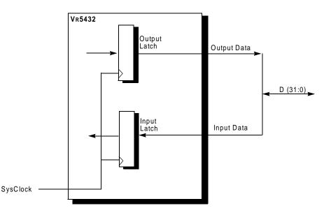
Figure 11-3 System Interface Register-to-Register Operation
