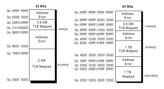
Figure 4-7 User and Supervisor Address Spaces in Supervisor Mode
