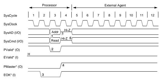
Figure 13-5 Uncompelled Transition Following Processor Read Request
