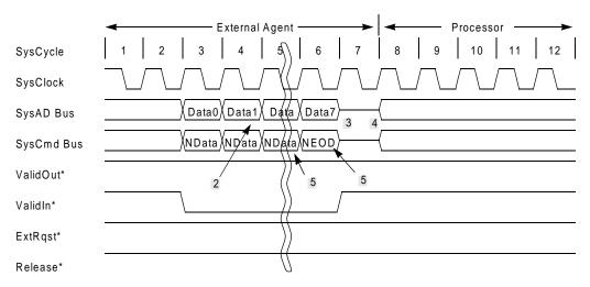
Figure 11-23 Block Read Response, System Interface Already in Slave State
