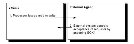
Figure 12-3 Processor Request Flow Control
