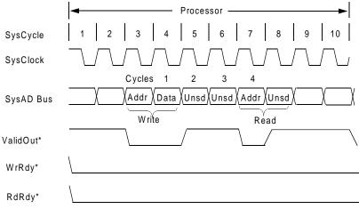
Figure 11-11 Read Cycle Following a Nonblock Write Cycle
