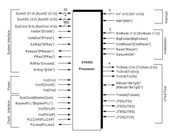
Figure 2-1 VR5432 Processor Signals
