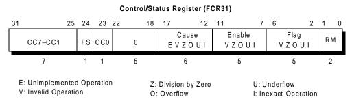
Figure 7-3 FP Control/Status Register Bit Assignments
