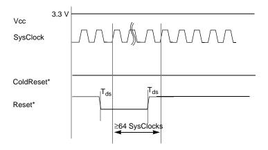
Figure 14-3 Warm Reset Timing Diagram
