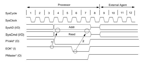
Figure 13-9 Delayed Processor Read Request
