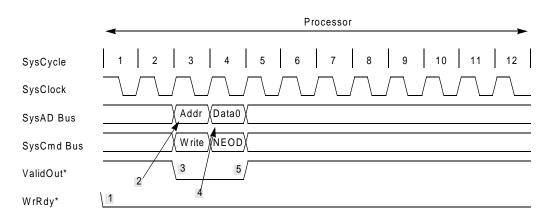
Figure 11-6 Processor Nonblock Write Request Protocol
