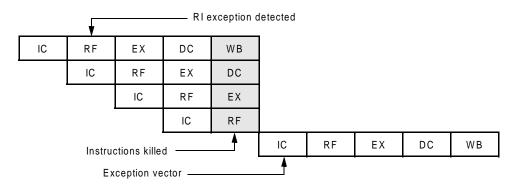
Figure 3-5 Exception Detection Mechanism
