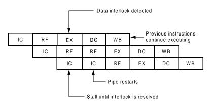
Figure 3-6 Servicing a Data Interlock Stall
