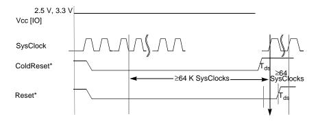
Figure 14-2 Cold Reset Timing Diagram
