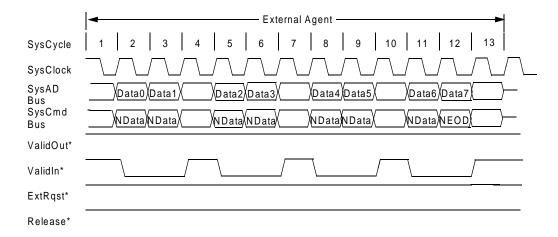
Figure 11-25 Read Response, Reduced Data Rate, System Interface in Slave State
