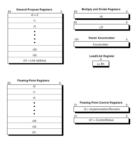
Figure 1-2 VR5432 Processor Registers
