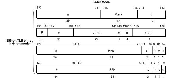
Figure 4-10 Format of a TLB Entry
