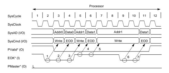
Figure 13-23 Discarding and Re-Executing a Processor Single Write Request
