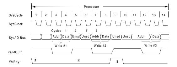
Figure 11-10 R4000-Compatible Back-to-Back Write Cycle Timing
