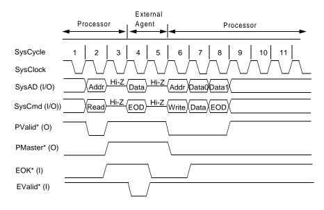
Figure 13-14 Processor Single Read Request Followed by Block Write Request
