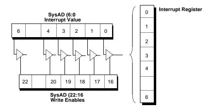
Figure 6-25 Interrupt Register Bits and Enables
