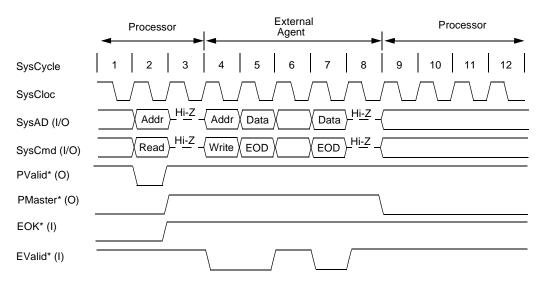
Figure 13-22 External Write Request Interrupts Processor Read Request
