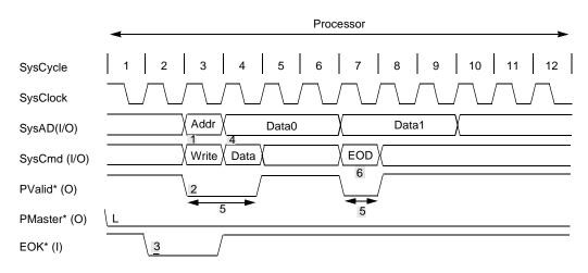
Figure 13-8 Processor Block Write Request (Write Data Pattern: Wxx)
