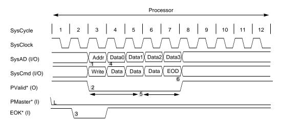
Figure 13-7 Processor Block Write Request (Write Data Pattern: W)
