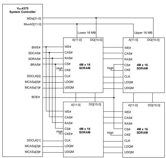
Figure 6. SDRAM Connections for Base Memory (Example)
