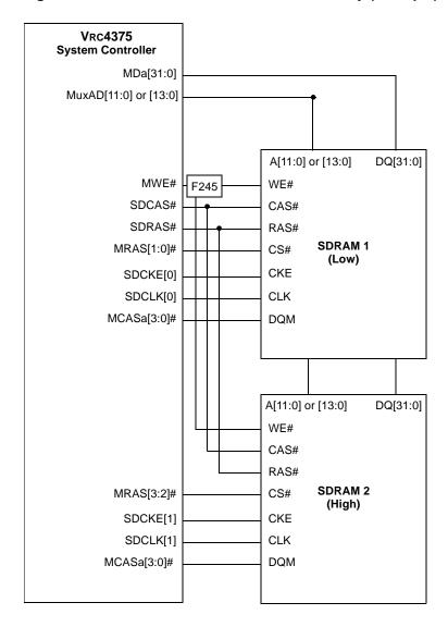
Figure 8. SDRAM Connections for SIMM Memory (Example)
