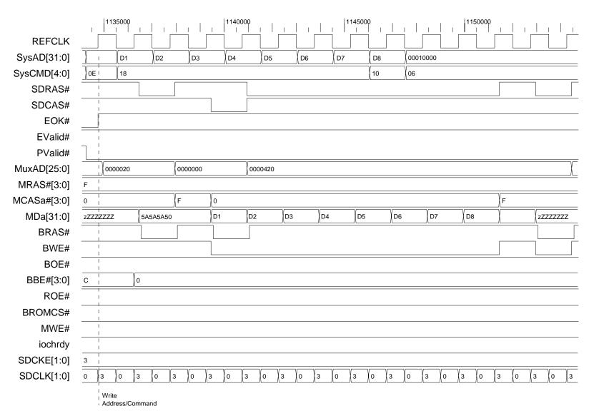
Figure 22. CPU Octet Write to SDRAM Base Memory
