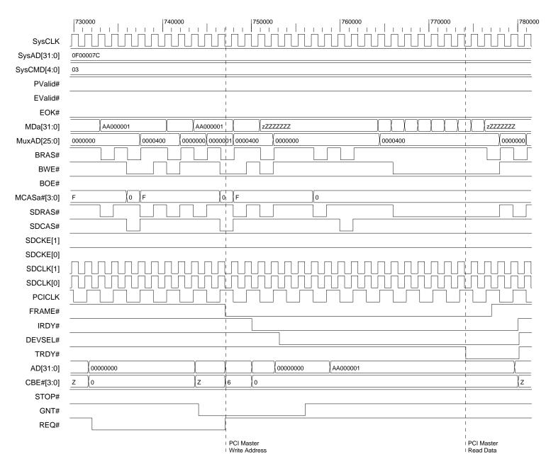
Figure 46. PCI Burst Write: 32 Words
