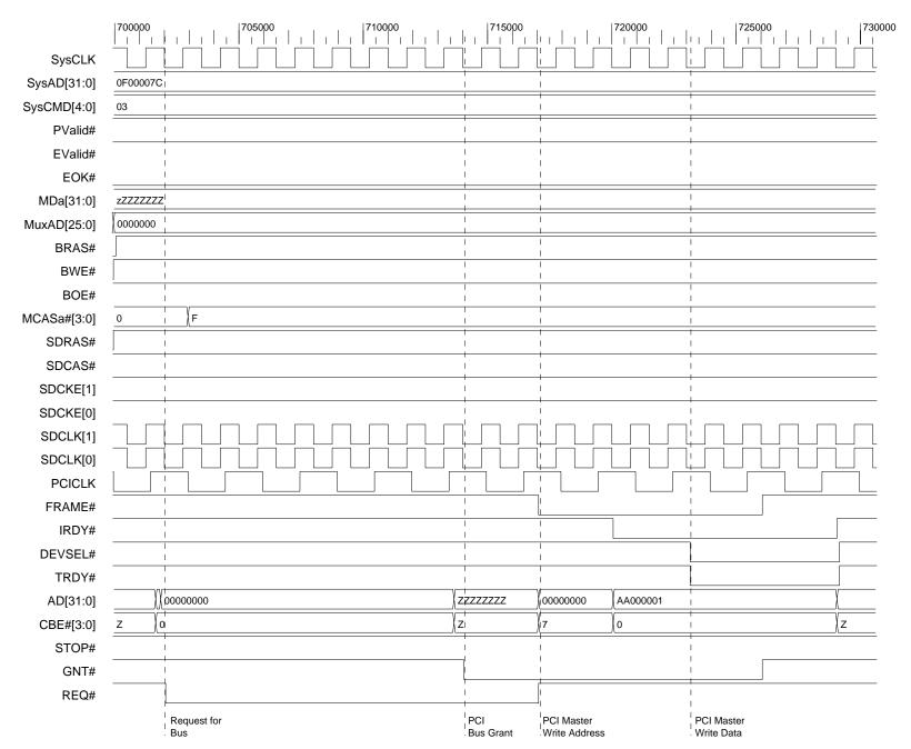
Figure 52. PCI to Controller Single 8-Byte Write
