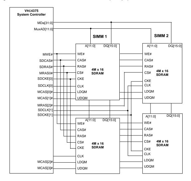
Figure 7. SDRAM Connections for SIMM 1 and SIMM 2 (Example)
