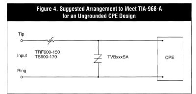
device with the appropriately rated SiBar device can provide a fully resettable solution for ungrounded and grounded systems as shown in Figures 4 and 5.
