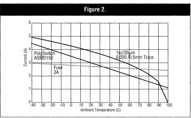
surface-mount ASMD150. Note how the trip current of the PolySwitch device tracks the trace current-to-damage over the temperature range. Even if a fuse could be used here, the nearest size fails to protect above a useful and standard automotive temperature in either case.
