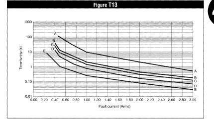
Figures T12–T17. Typical Time-to-trip Curves at 20°C for Telecommunications and Networking Devices continued
