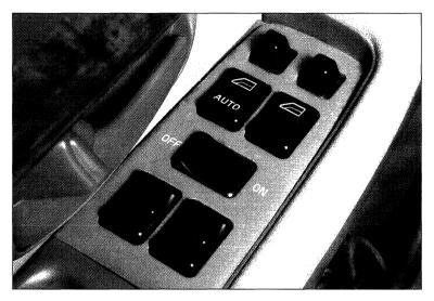
is reached. This de-activates the latched relay. Additional electronic functions are required to reject inrush current and transient voltages, and a fail-safe time-out feature is often added as a back-up for the event the primary system
