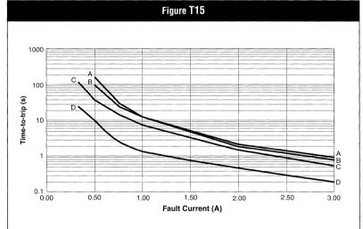
Figures T12–T17. Typical Time-to-trip Curves at 20°C for Telecommunications and Networking Devices continued
