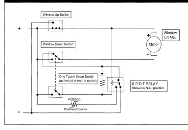
manual down (opening the window) switch, an auto-down initiate switch, a low current blocking diode, a resistor, and a singlepole-double-throw (SPDT) relay. The manual up and down switch is mechanically interconnected to provide a mutually exclusive operation. The auto down switch is mechanically interconnected to the manual down switch, and is activated at the end of travel in a mutually inclusive operation with the manual down switch.
