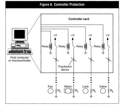
A long-standing tradition that contributes to miswiring is that both power (less than  $100 V_{DC}$ ) and signal lines are often run in the same conduit. At the remote end, which can be thousands of feet away from the host, it is not difficult to connect the wires incorrectly, wire the hot lines to ground, or superimpose powered lines on low-voltage data lines.
