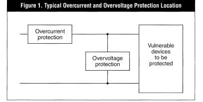
circuit) under normal operating conditions. When an overvoltage event occurs, however, the overvoltage device changes its impedance to divert current around the protected circuit to ground.
