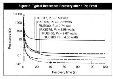
user with a sense of the thermal environment the device was placed in for the measurement. As with other electrical properties, the resistance recovery time will depend upon both the design of the device and the thermal environment. Since resistance recovery is related to the cooling of the device, the greater the heat transfer, the more rapid the recovery (see Figure 6 for miniSMD075 devices on boards with traces of 0.010 inch and 0.060 inch).
