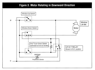
the relay coil drops below its "drop-out" level, the relay will be de-energized, and the relay contacts will open interrupting the current flow to the motor.
