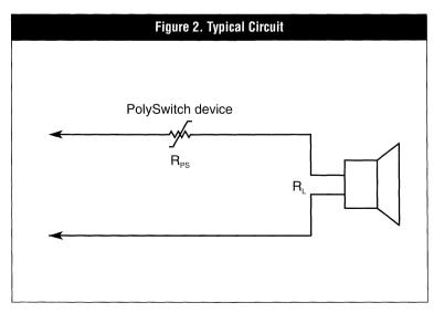
power attenuation in the tripped state is:
