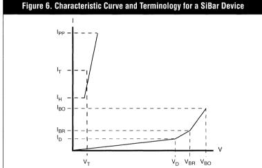
state condition. The leakage current should be as low as possible to minimize loss in the circuit. The leakage current is measured at 50V and at  $V_{DM}$ , which is approximately 90% of the breakdown voltage. The measurement is made at 50V because this is the typical voltage present on a standard telephone line. The upper voltage,  $V_{DM}$ , is defined at an acceptable current of 5µA.
