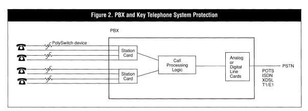
Telcordia GR-1089 requirements in North America or the ITU recommendations for other regions of the world. Reference diagrams for protection against UL60950, TIA-968-A, Telcordia GR-1089 Intrabuilding and Extrabuilding, and ITU recommendations can be found as separate application notes in this Databook.
