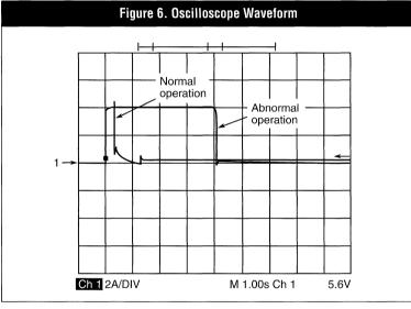
In the automotive market, a designer may use an intermittentduty solenoid in a trunk-release application. In most cases, the lock will only be energized once or twice within a couple of seconds. However, if the lock is continuously operated, the solenoid will eventually exceed its thermal rating and fail. A PolySwitch device in series with the coil can help eliminate this problem.
