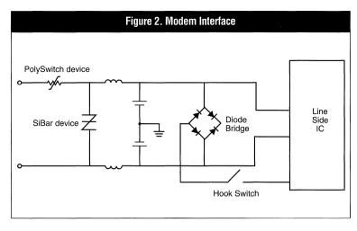
devices with off-state voltage  $V_{\rm DM}$  ratings of 270V are applicable for CPE equipment with maximum peak voltages up to 270V<sub>DM</sub>. For systems with lower expected volt-
