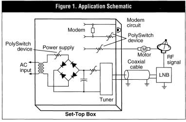
the antenna from the receiver. Thus, the LNB circuit should be protected.
