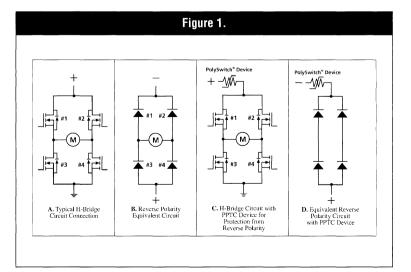
For the same reasons as stated earlier, the use of a series blocking diode, may not be economically feasible. However, the use of a series PPTC device helps provide reverse-polarity protection economically while minimizing the voltage loss in the system (Figure 1C). The equivalent circuit in a reverse-polarity condition is shown in Figure 1D. Generally, the FETs intrinsic diode will easily provide the momentary surge current necessary to cause the PPTC device to trip within milliseconds.
