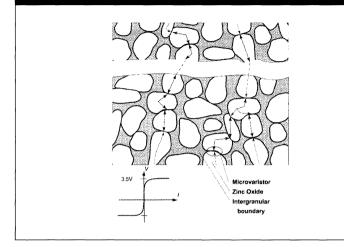
ZnO grains, separated by other metal oxide ceramics. This polycrystalline structure is depicted in Figure 2.
