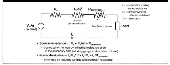
Figure 3. PolySwitch devices can limit transformer winding temperatures to well below UL/IEC specifications
