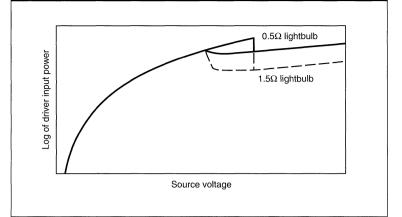
current just below the maximum safe steady-state current for the driver. In either case, the designer should conduct an empirical investigation to verify performance.
