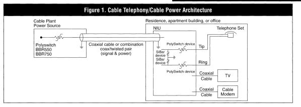
Overvoltage protection requirements depend upon the exact powering and ringing configuration used; however, for most applications, standard POTS voltage and current levels are expected.
