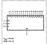
Parallel load : data present on  $D_0$ -  $D_{15}$  are entered into the register on the falling edge of CP. The SO output represents the  $Q_{15}$  register output.
