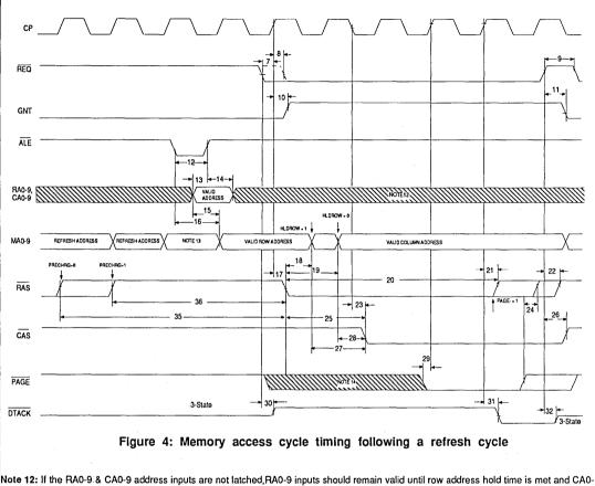
9 inputs should remain valid until column address hold time is met. Note 13: MA0-9 outputs will contain the present row address on the RA0-RA9 inputs or the last row address latched into the device. Note 14: PAGE input may be asserted anytime before this rising clock edge inorder to hold RAS Low.
