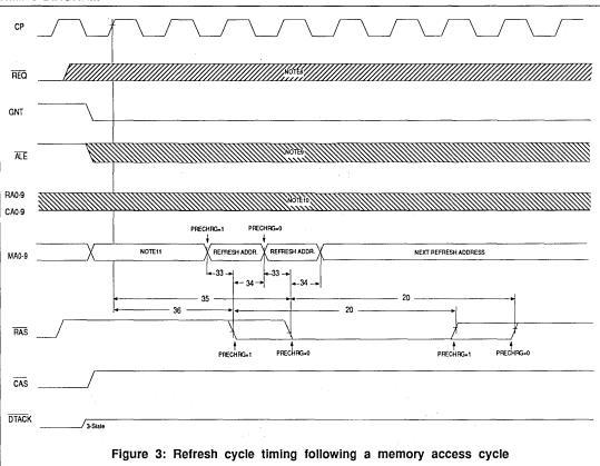
Note 8: REQ input is a don't care during a memory refresh cycle. If REQ is asserted during a refresh cycle, it will be recognized at the first rising CP clock edge, following the refresh cycle and it's associated RAS precharge time (see Figure 4). Note 9: RA0-9 & CA0-9 address inputs may be latched at anytime during a memory refresh cycle. However, a memory access cycle will not begin until after the completion of the refresh cycle.
