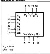
$(\overline{CE})$  is High. The outputs are active only in the READ mode (WE = High) and the output data is the complement of the stored data.
