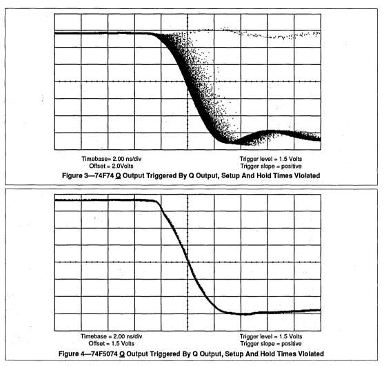
10.02 MHz data) the device-under-test operates continuously in the region where metastability can occur. If the Q output is then used to trigger a digital scope set to infinite persistence the  $\underline{Q}$  output will build a waveform.
