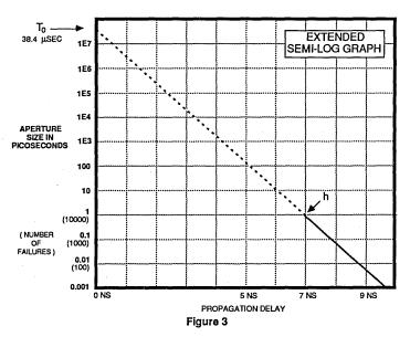
transitions were uniformly and randomly distributed over a clock period of 100 ns: you would expect 65 of these transitions to cause the outputs to go into a metastable state and remain there for at least 9 ns.
