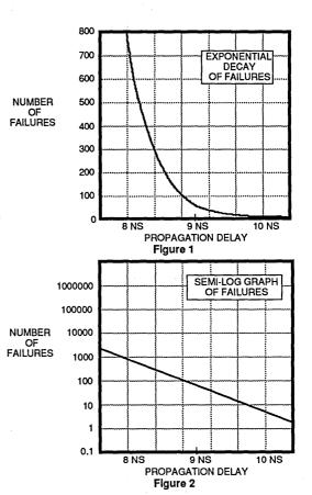
ponential time constant of the decay rate of the metastability. It is sometimes called the metastability time constant. The final parameter is the measured propagation delay of the device. Commonly, the typical propagation delays found in the data book are used for this and it is designated 'h' in the equations (although most designers are familiar with this value as Tpd). Now let's see how tau and  $T_0$  are determined by measurements.
