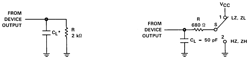
FIGURE 10. CAPACITIVE LOAD SWITCHING
