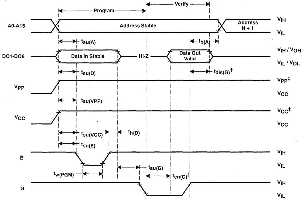
$^\dagger t_{dis}(G)$  and  $t_{en}(G)$  are characteristics of the device but must be accommodated by the programmer.
