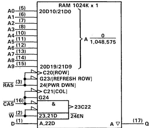
†This symbol is in accordance with ANSI/IEEE Std 91-1984 and IEC Publication 617-12. The pin numbers shown are for the 18-pin dual-in-line package.
