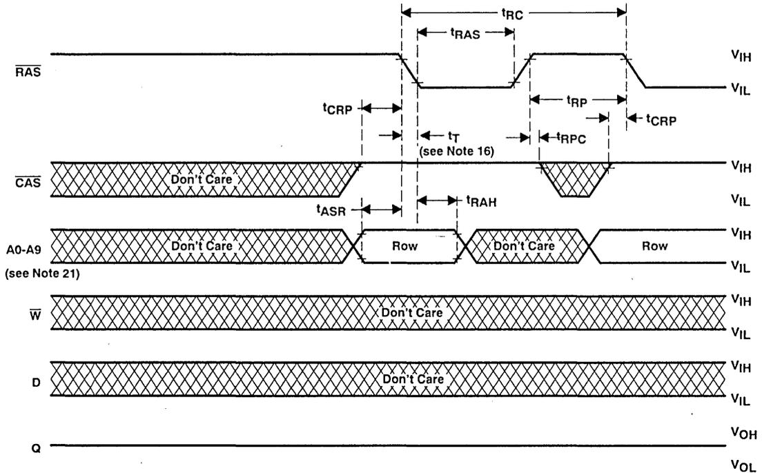
NOTES: 16. Transition times (rise and fall) for  $\overline{RAS}$  and  $\overline{CAS}$  are to be minimum of 3 ns and maximum of 50 ns.
