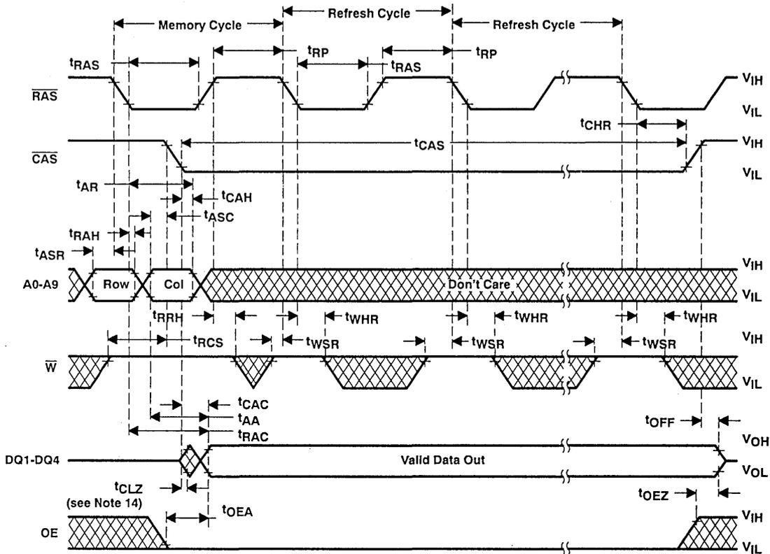
NOTE 14: Valid data is presented at the outputs after all access times are satisfied but may go from three-state to an invalid data state prior to the specified access times as the outputs are driven when  $\overline{CAS}$  goes low.
