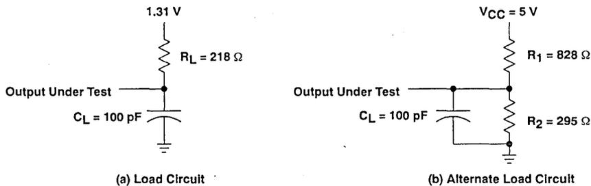
Figure 2. Load Circuits for Timing Parameters
