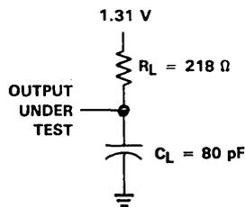
(b) ALTERNATE LOAD CIRCUIT
