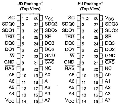
†The packages shown here are for pinout reference only and are not drawn to scale.
