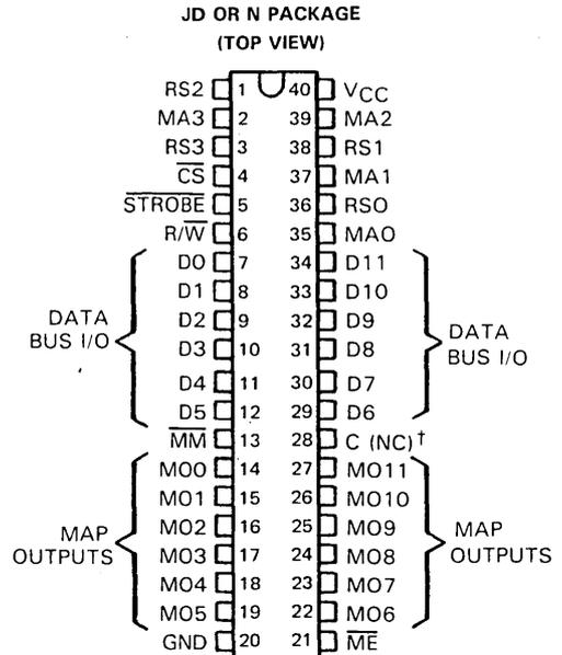
†This pin has no internal connection on the 'LS612.
