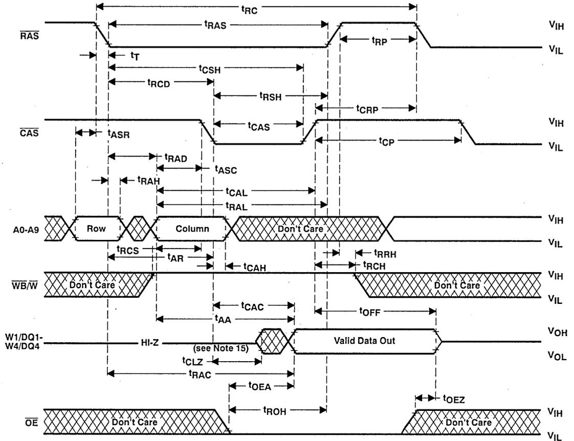
NOTE 34: Output may go from three-state to an invalid data state prior to the specified access time.
