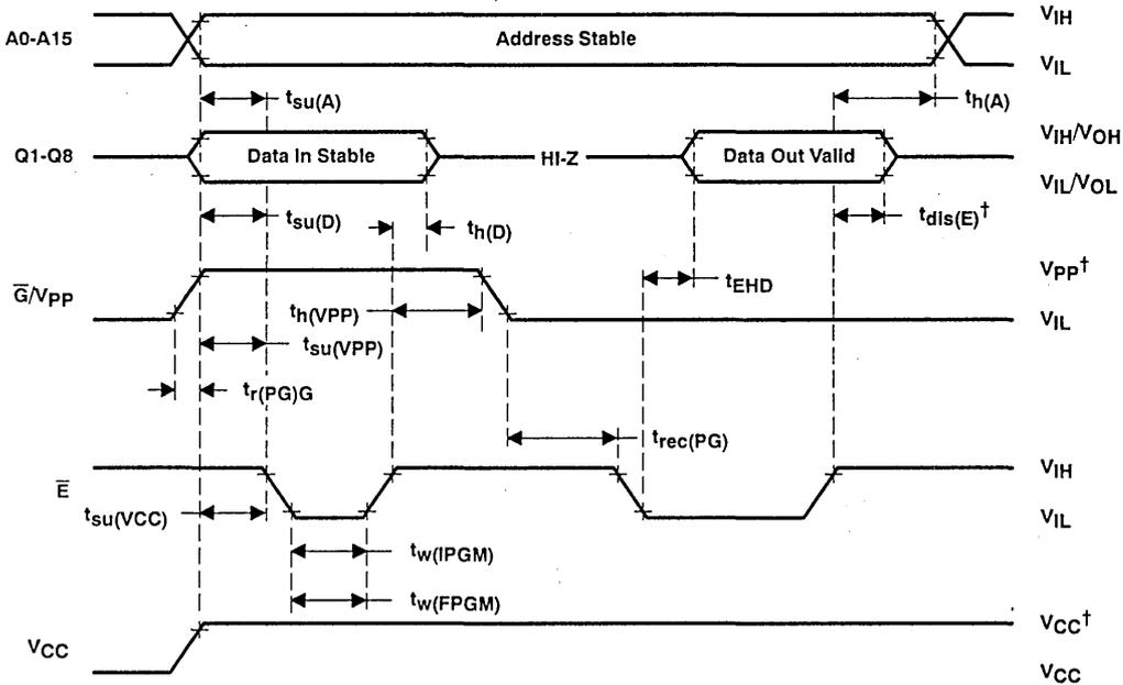
$^\dagger$  12.5-V  $V_{pp}$  and 6-V  $V_{CC}$  for Fast programming, 13-V  $V_{pp}$  and 6.5-V  $V_{CC}$  for SNAP! Pulse programming.
