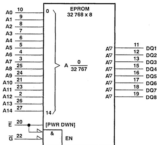
The address inputs are arranged in order of their assigned binary weights and the range of addresses are shown as  $A_m^n$  where  $m$  is the decimal equivalent of the lowest address and  $n$  is the highest. The outputs affected by these addresses are indicated by the letter  $A$ , as data inputs would also be if the device were a RAM.
