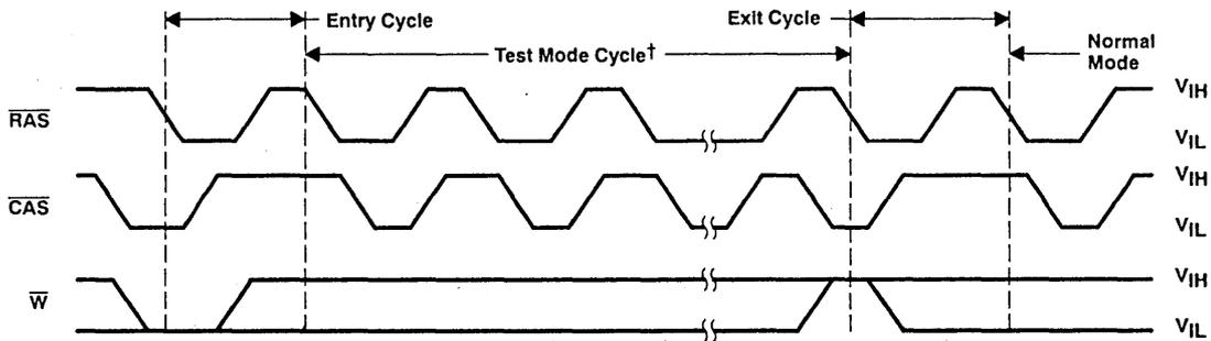
† The states of  $\overline{\text{W}}$ , Data-in, and Address are defined by the type of cycle used during test mode.
