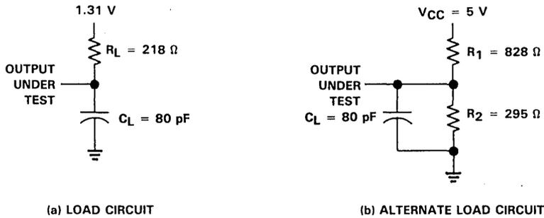
**FIGURE 1. LOAD CIRCUITS FOR TIMING PARAMETERS**
