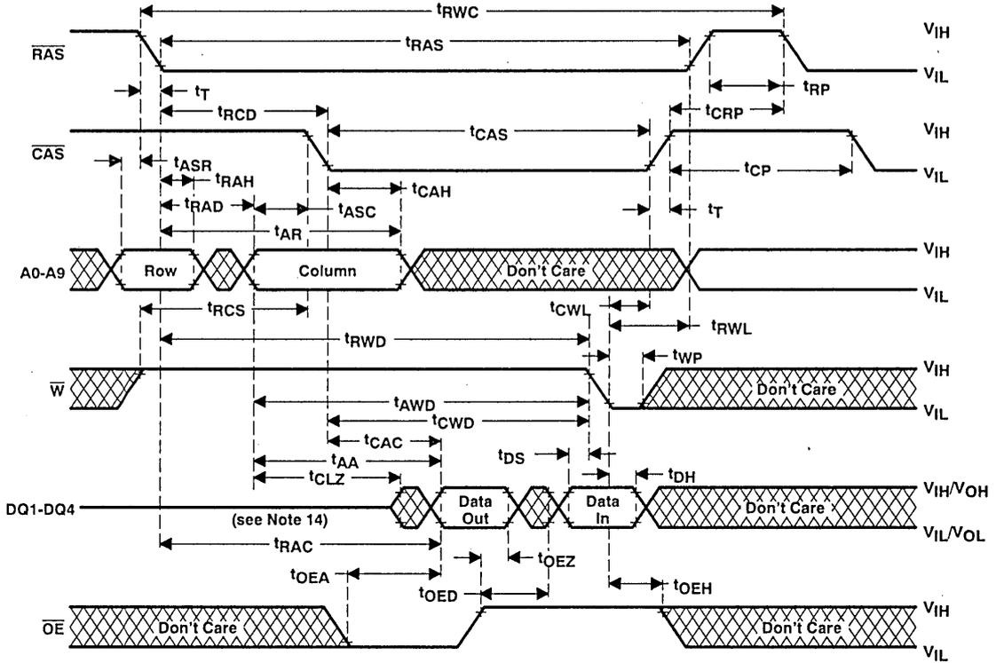
NOTE 14: Valid data is presented at the outputs after all access times are satisfied but may go from three-state to an invalid data state prior to the specified access times as the outputs are driven when  $\overline{\text{CAS}}$  goes low.
