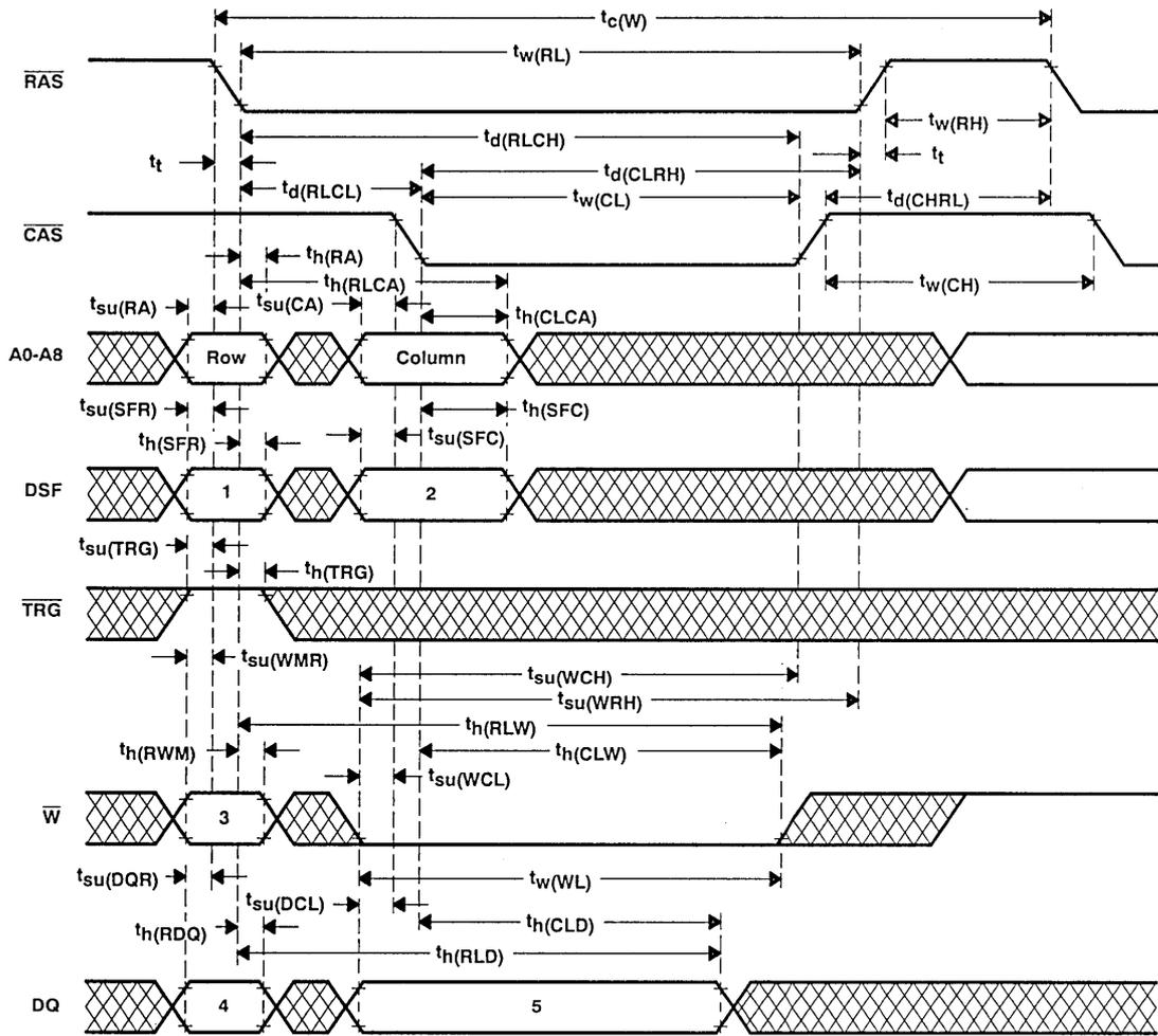
NOTE 24: See "Write Cycle State Table" for the logic state of "1", "2", "3", "4", and "5".
