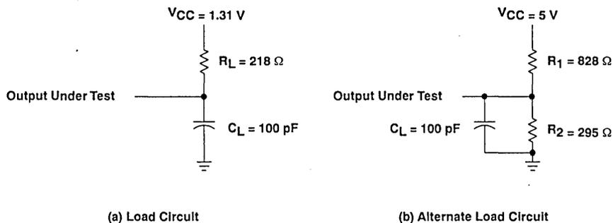
Figure 1. Load Circuits for Timing Parameters
