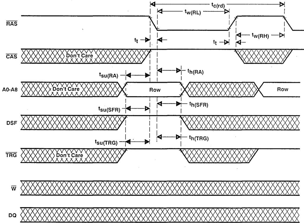
NOTE 30: In persistent write-per-bit function,  $\overline{W}$  must be high during the refresh cycle.
