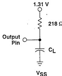
Figure 3. Load Circuit
