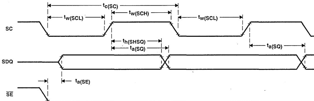
NOTES: 7. When the odd tap is used (tap addresses can be 0-511, and odd taps are 1,3,5 ... etc.), the cycle time for SC in serial data out cycle needs to be 50 ns minimum.
