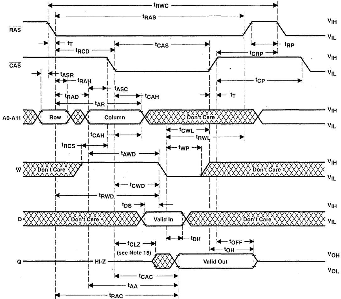
NOTE 15: Output may go from three-state to an invalid data state prior to the specified access time.
