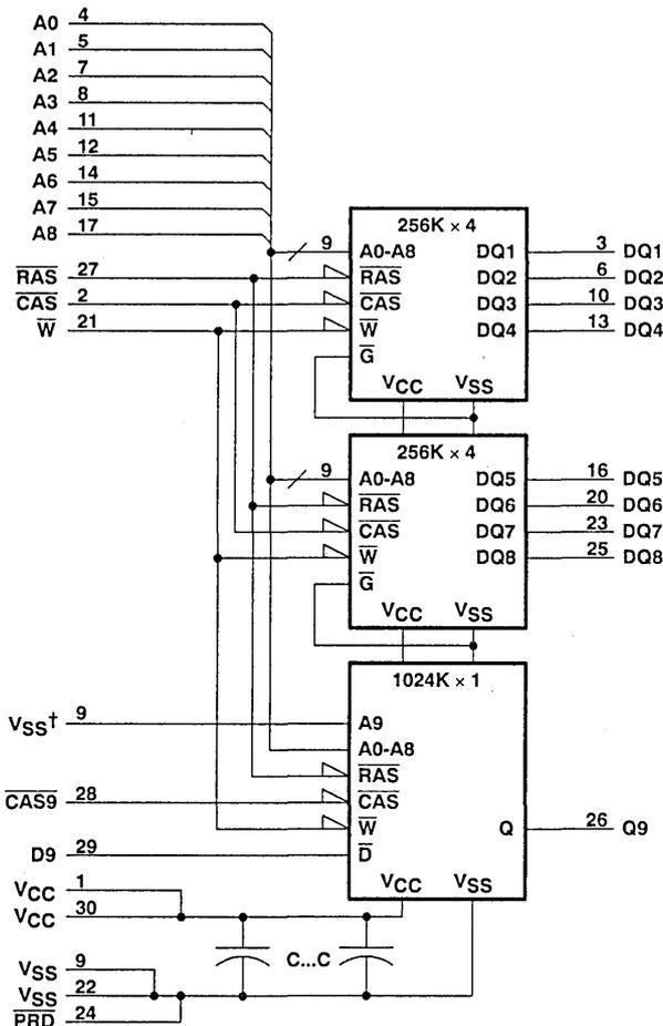
† Address pin A9 is connected to VSS.
