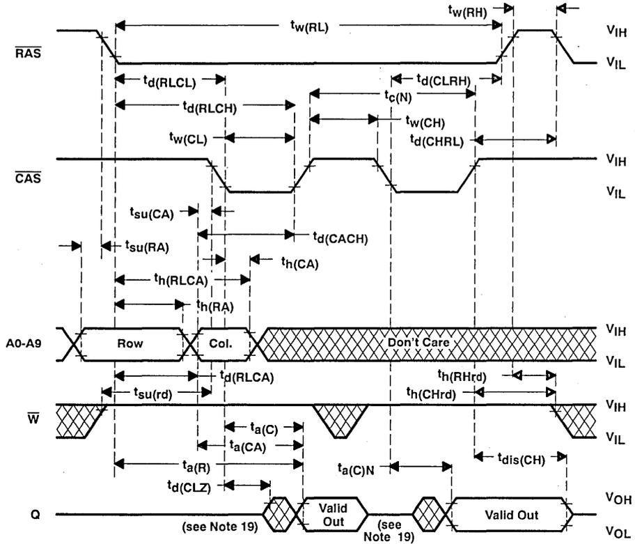
NOTE 19: Output may go from high-impedance to an invalid state prior to the specified access time.
