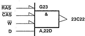
By virtue of the AND relationship between  $\overline{CAS}$  and  $\overline{W}$  (explicitly shown), when either one of these inputs goes low with the other one and  $\overline{RAS}$  is already low ( $\overline{RAS}$  is ANDed by G23), the D input is momentarily enabled (through C22). In an "early-write" cycle it is  $\overline{W}$  that goes low first; this causes the output to remain off as explained below.
