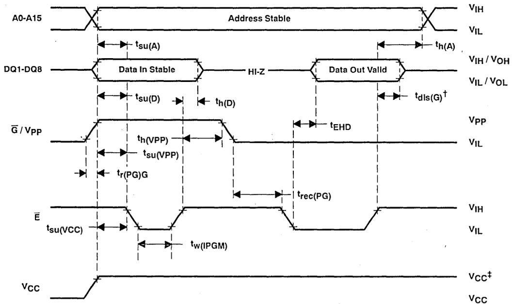
$^\dagger t_{dis}(G)$  is a characteristic of the device but must be accommodated by the programmer.
