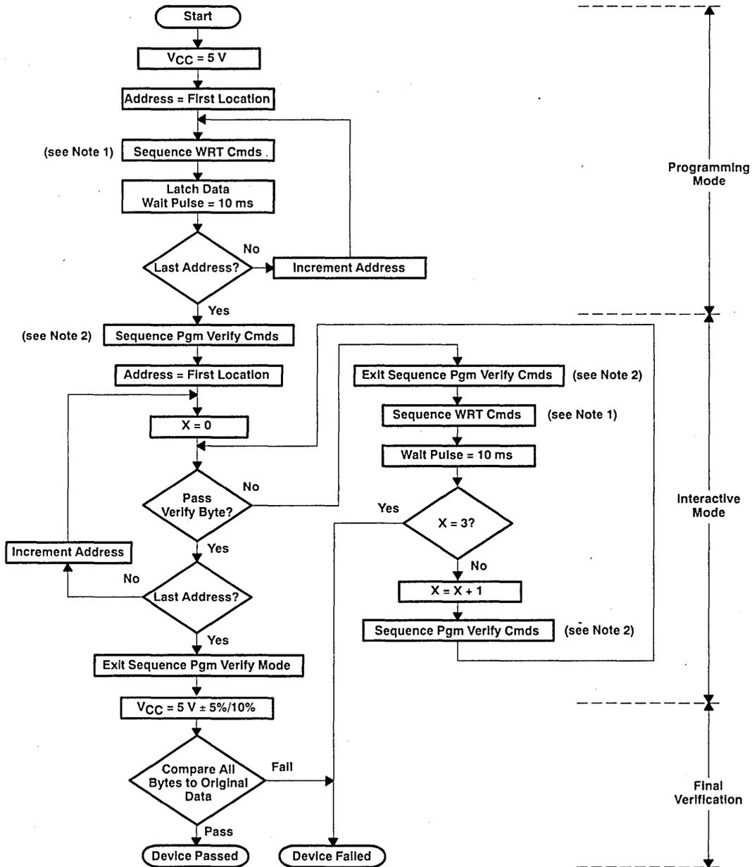
NOTES: 1. Upon the three-step sequence completion, the device is latched into the programming mode. The byte is latched and the byte programming operation starts if a subsequent rising edge of  $\bar{W}$  is not detected within 100  $\mu$ s.
