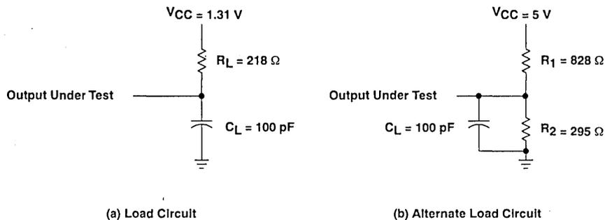
Figure 1. Load Circuits for Timing Parameters
