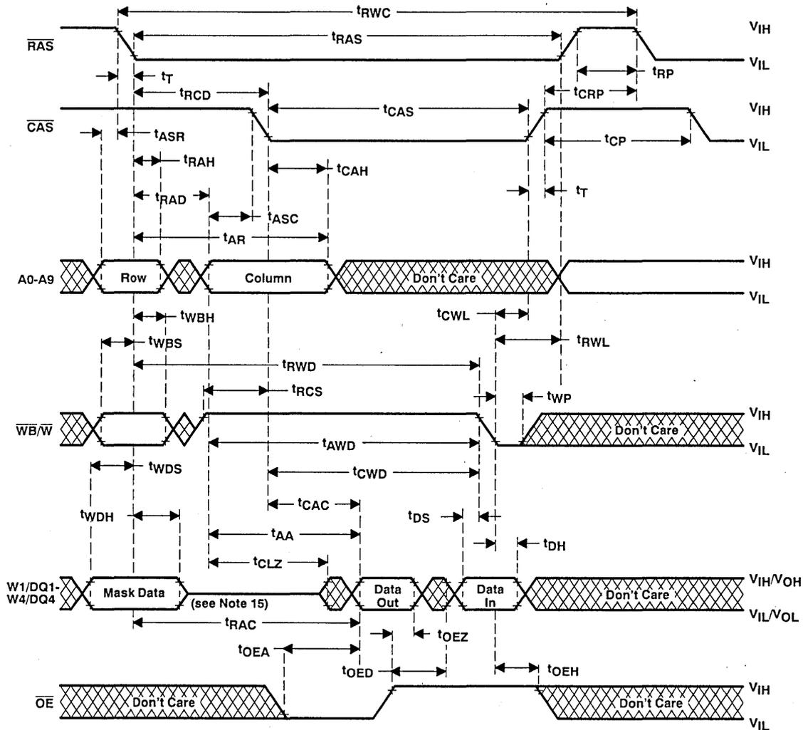
NOTE 15: Output may go from three-state to an invalid data state prior to the specified access time.
