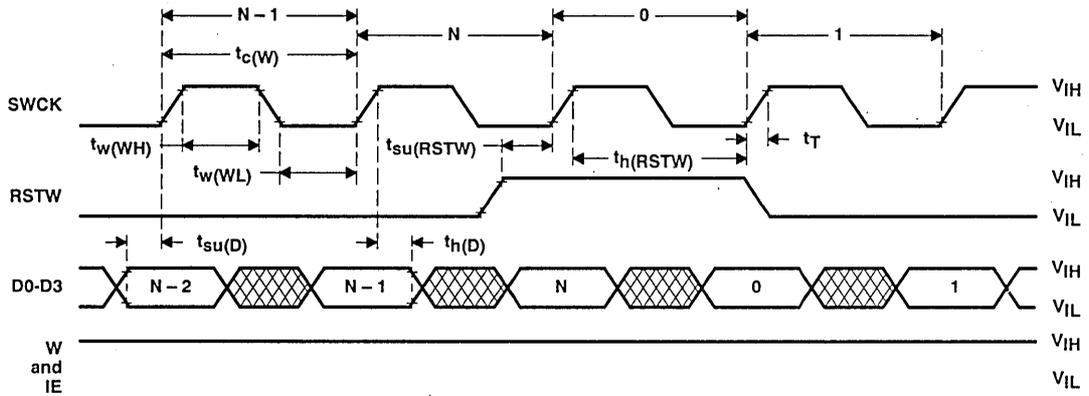
write cycle timing (write enable)
