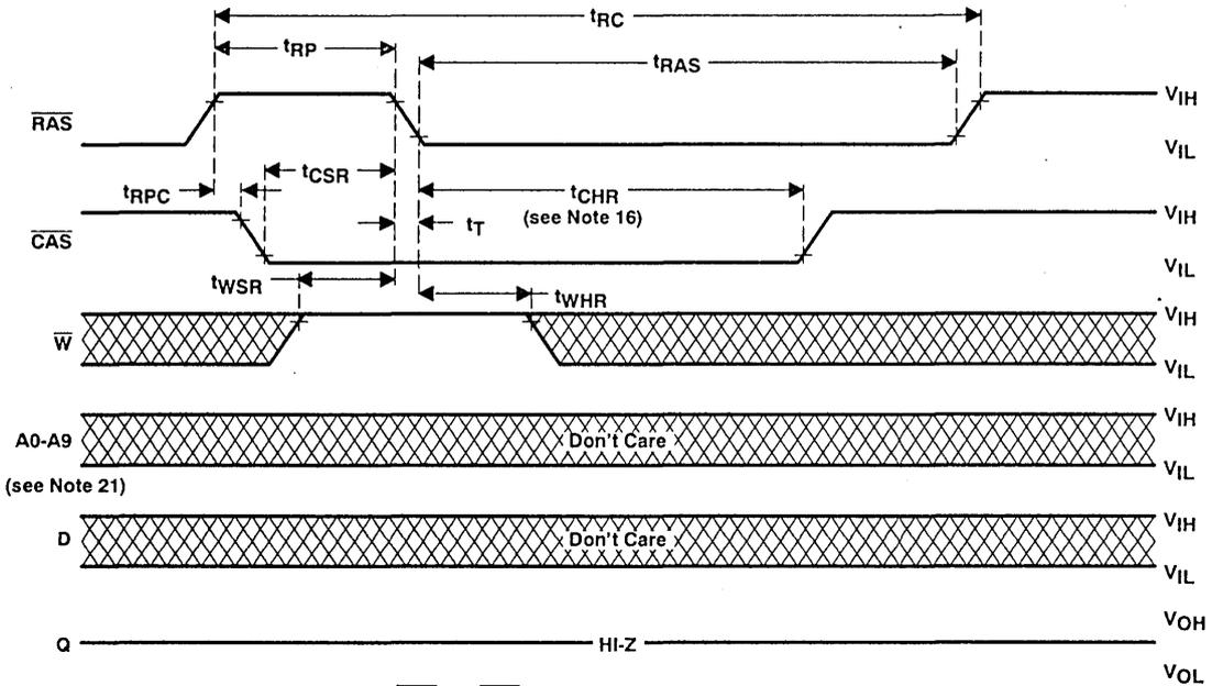
NOTES: 16. Transition times (rise and fall) for  $\overline{\text{RAS}}$  and  $\overline{\text{CAS}}$  are to be minimum of 3 ns and maximum of 50 ns.
