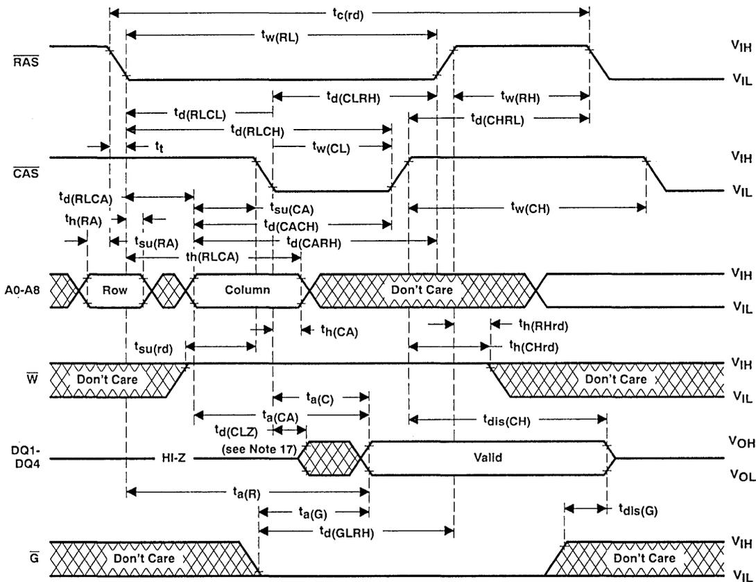
NOTE 17: Output may go from high-impedance to an invalid data state prior to the specified access time.
