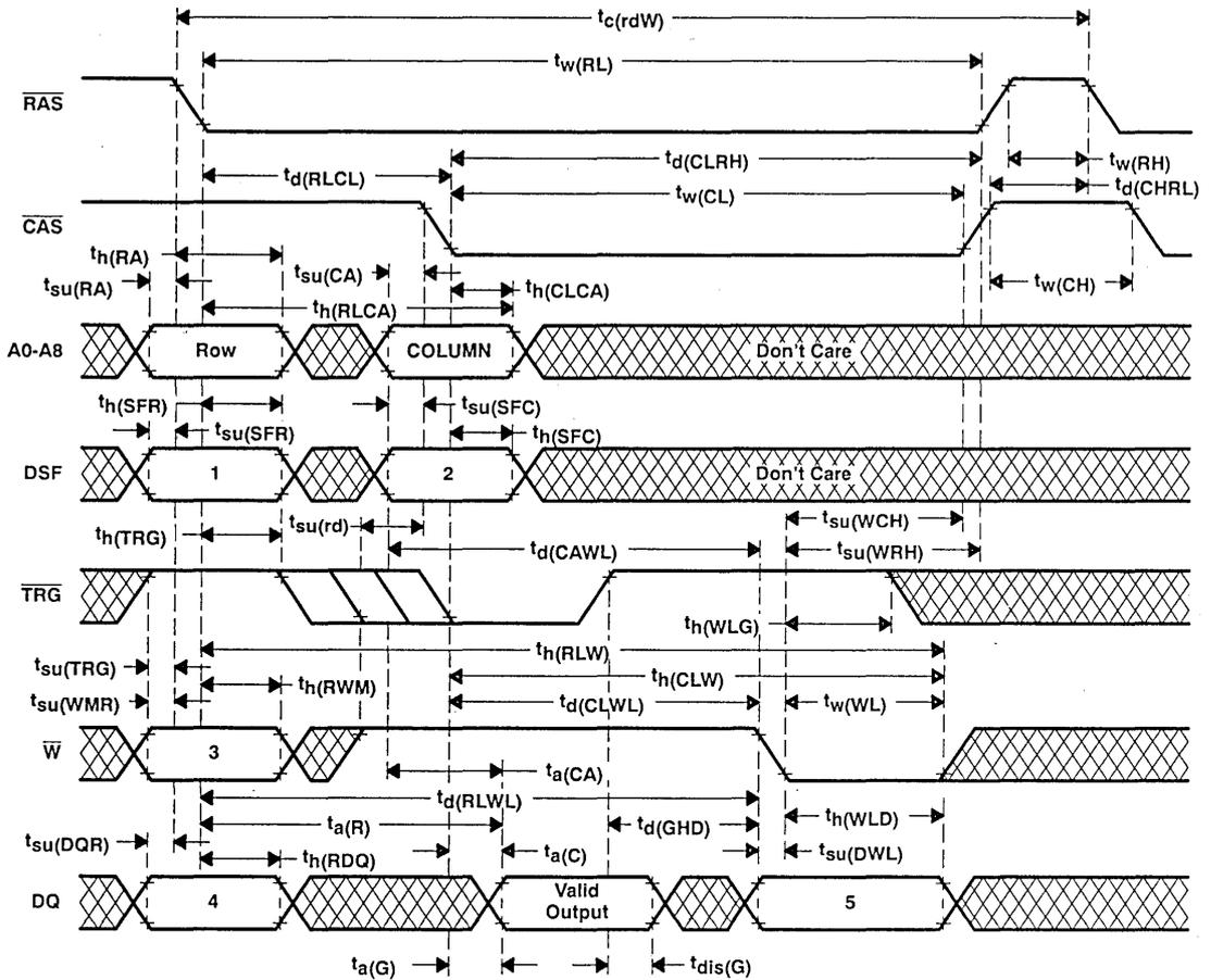
NOTE 27: See "Write Cycle State Table" for the logic state of "1", "2", "3", "4", and "5". Same logic as delayed write cycle.
