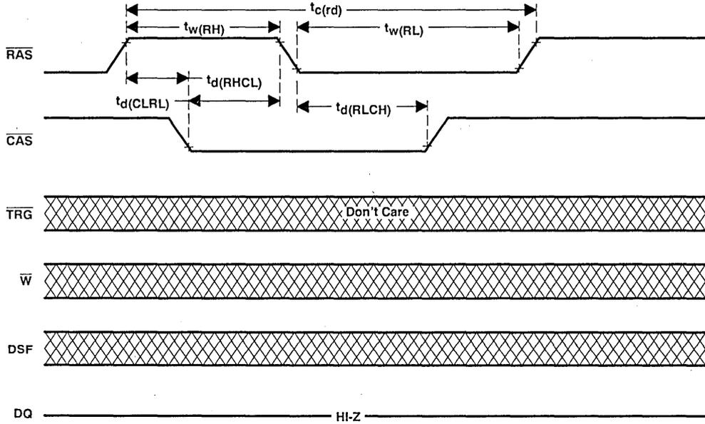
NOTE 30: In persistent write-per-bit function,  $\overline{W}$  must be high during the refresh cycle.
