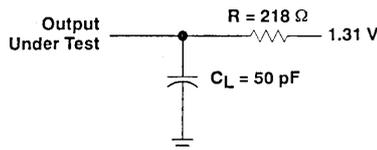
Figure 1. Output Load Circuit
