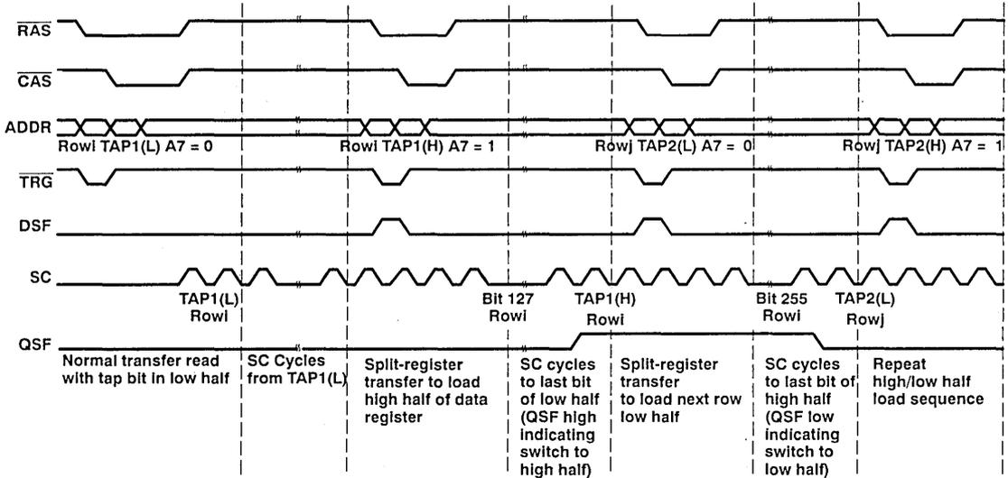
NOTES: 36. In split register mode, data can be transferred from different rows to the low and high halves of the data register.
