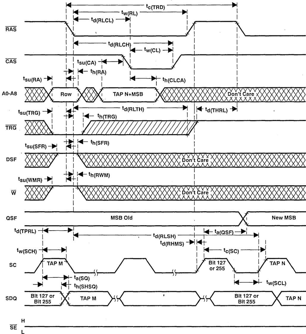
NOTE 35: There must be a minimum of two SC clock cycle between any two split-register reload cycles, and between a transfer read cycle and a split-register cycle.
