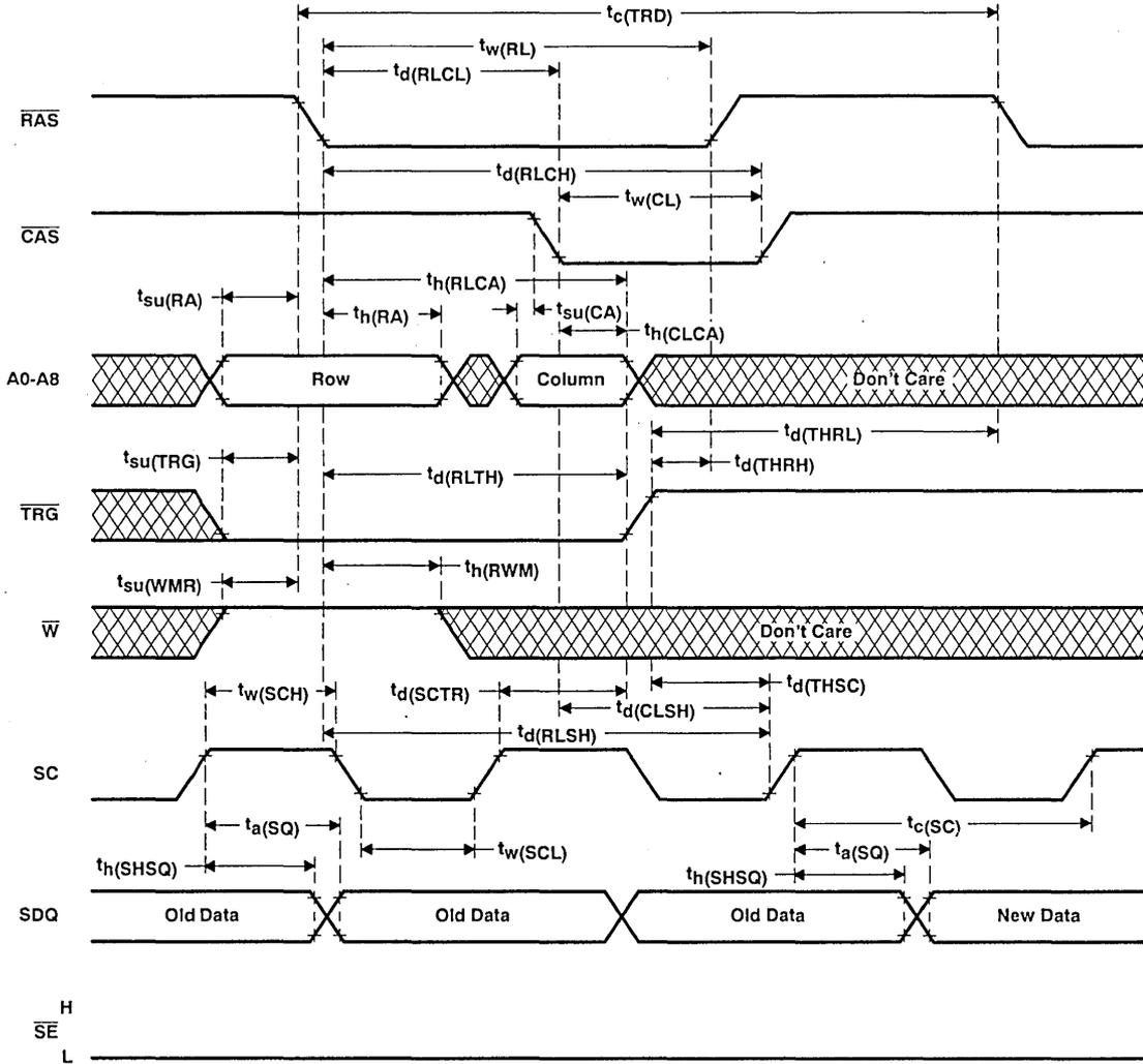
NOTES: 37. Random mode (Q outputs) remain in the high-impedance state for the entire memory to data register transfer cycle. The memory to data register transfer cycle is used to load the data registers in parallel from the memory array. The 512 locations in each data register are written into from the 512 corresponding columns of the selected row. The data that is transferred into the data registers may be either shifted out or transferred back into another row.
