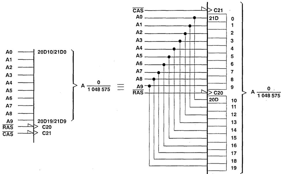
When  $\overline{\text{RAS}}$  goes low, it momentarily enables (through C20,  $\triangleright$  indicates a dynamic input) the D inputs of the ten address registers 10 through 19. When  $\overline{\text{CAS}}$  goes low, it momentarily enables (through C21) the D inputs of the ten address registers 0 through 9. The outputs of the address registers are in 20 internal address lines that select 1 of 1 048 576 cells.
