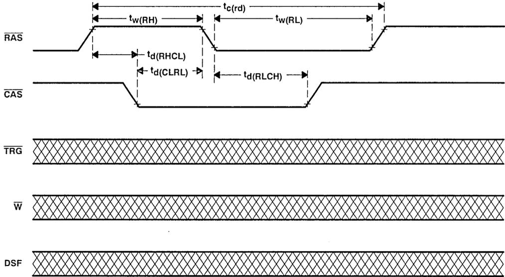
NOTE 29: In persistent write-per-bit function,  $\overline{\text{W}}$  must be high during the refresh cycles.
