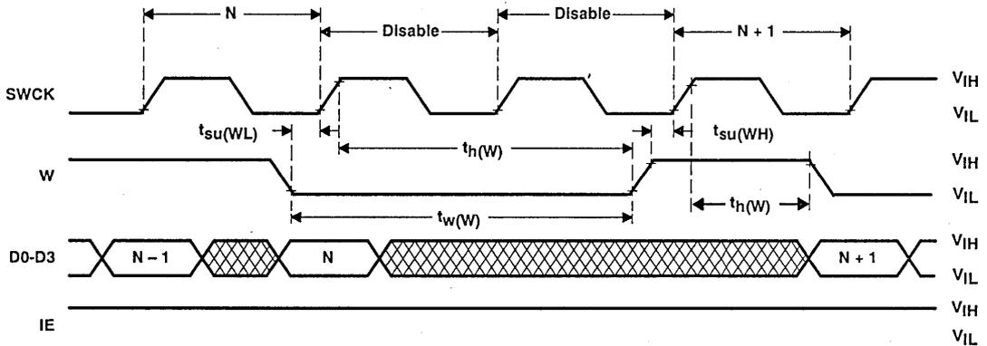
write cycle timing (input enable = write mask operation)
