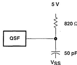
Figure 3. QSF Load Circuit (Revision "H" only)
