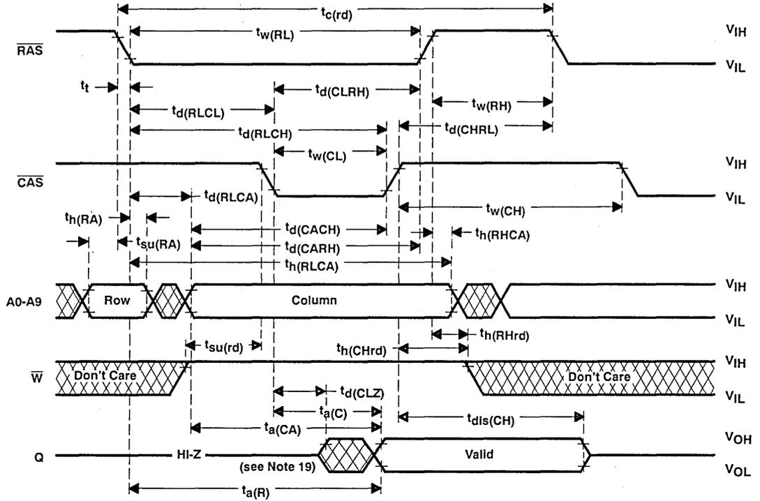
NOTE 19: Output may go from high-impedance to an invalid state prior to the specified access time.
