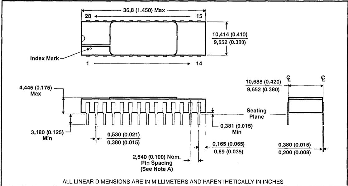
NOTE A: Each pin centerline is located within 0,250(0.010) of its true longitudinal position.
