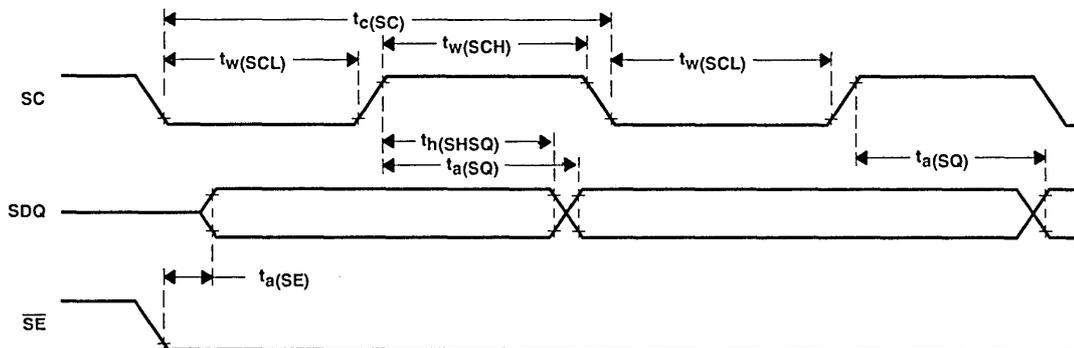
NOTES: 8. For mid-line load,  $t_c(SC) = 50$  ns for Revision I and subsequent revisions;  $t_c(SC) = 55$  ns for Revision H only. For split-register,  $t_c(SC) = 40$  ns for Revision H only.
