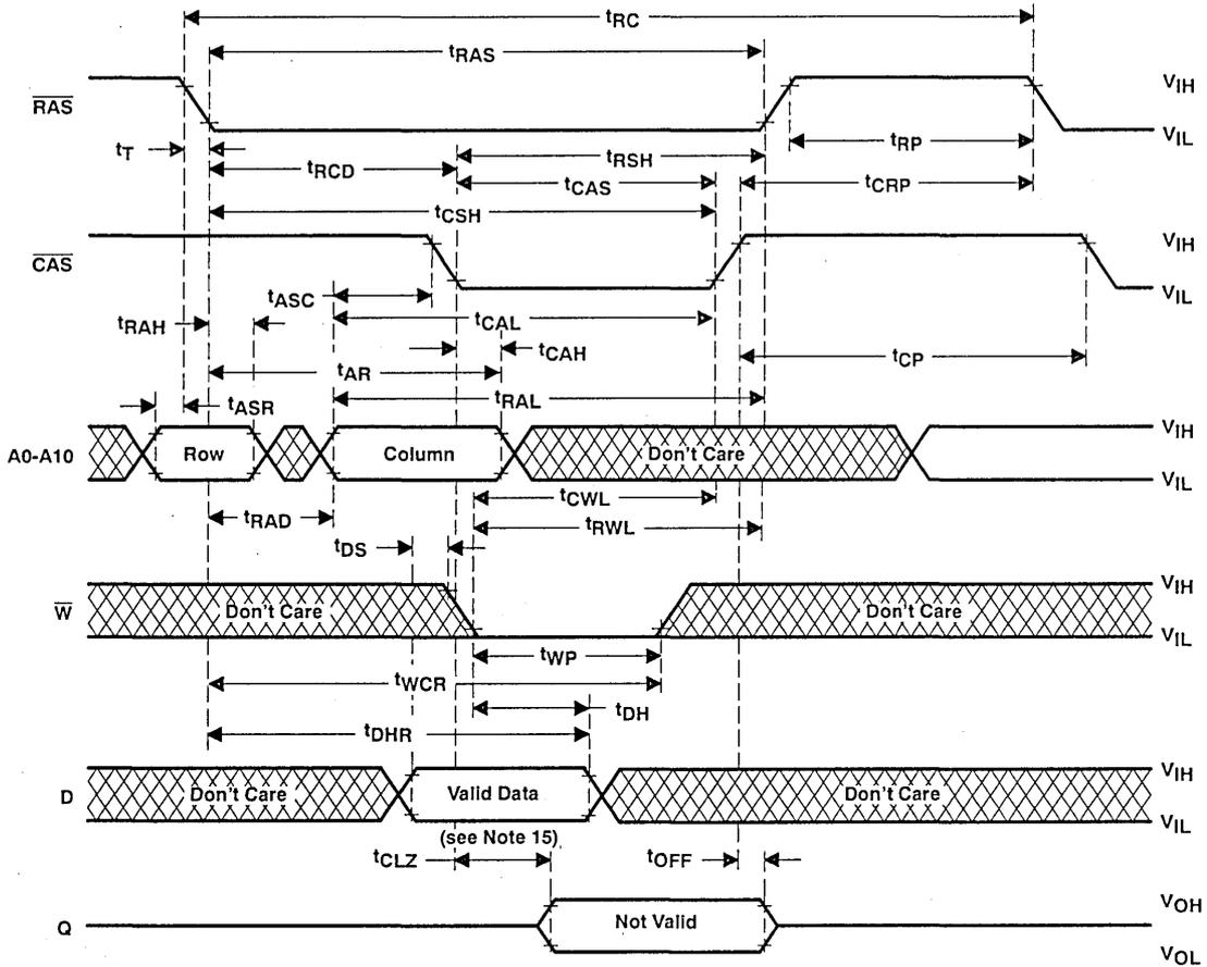
NOTE 15: Valid data is presented at the output after all access times are satisfied. The output may go from three-state to an invalid data state prior to the specified access times as the output is driven when  $\overline{\text{CAS}}$  goes low.
