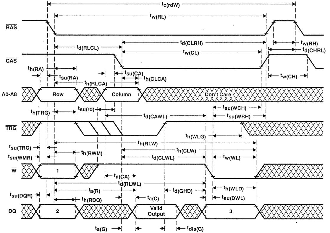
NOTE 27: See "Write Cycle State Table" for the logic state of "1", "2", and "3". Same logic as delayed write cycle.
