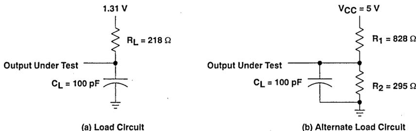
Figure 1. Load Circuits for Timing Parameters
