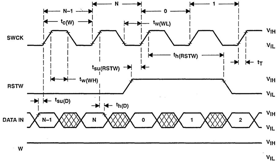
write cycle timing (write enable)
