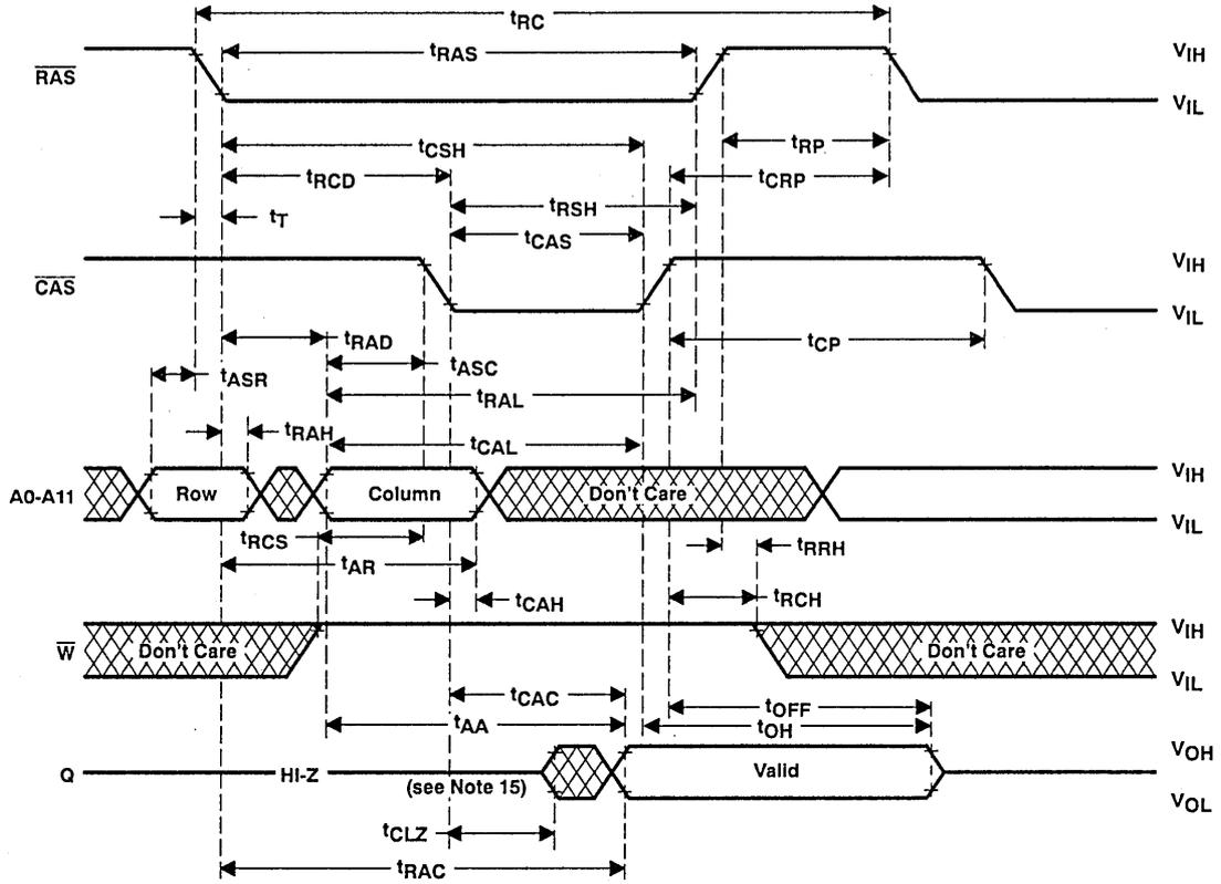
NOTE 15: Output may go from three-state to an invalid data state prior to the specified access time.
