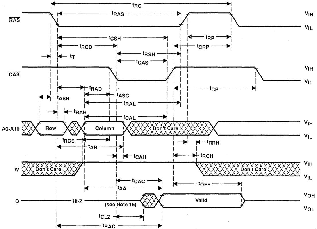
NOTE 15: Valid data is presented at the output after all access times are satisfied. The output may go from three-state to an invalid data state prior to the specified access times as the output is driven when CAS goes low.
