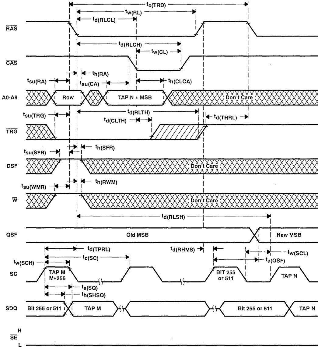
NOTE 37: There must be a minimum of two SC clocks cycle between any two split-register reload cycles, and a minimum of one SC clock cycle between a transfer read cycle and a split-register cycle.
