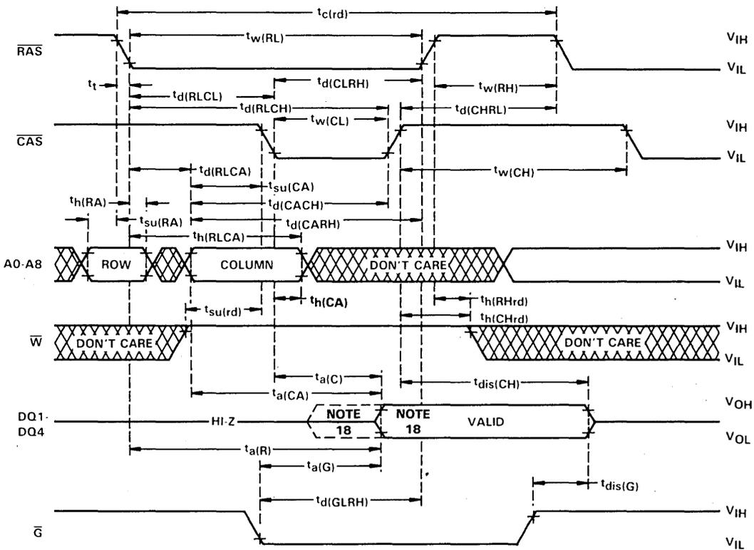
**NOTE 18:** Output may go from high impedance to an invalid data state prior to the specified access time.
