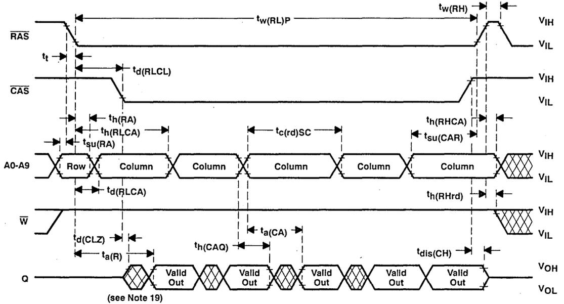
NOTE 19: Output may go from high-impedance to an invalid state prior to the specified access time.
