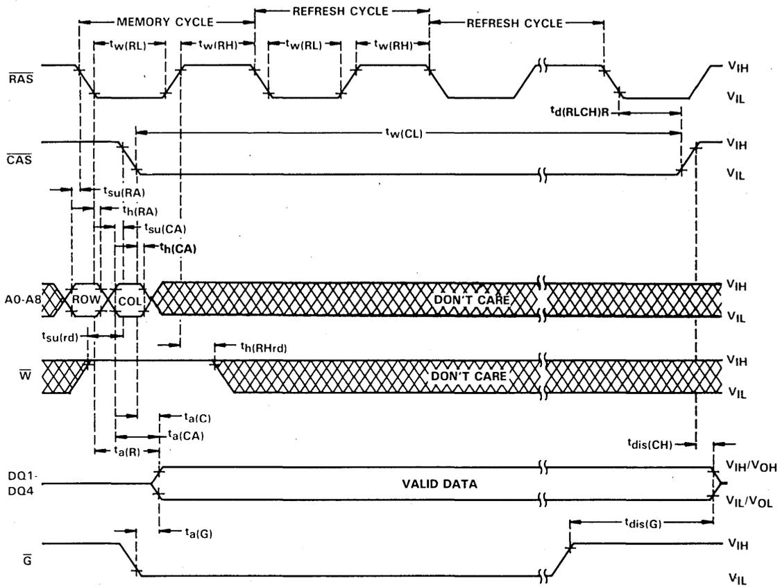
**automatic ( $\overline{\text{CAS}}$ -before- $\overline{\text{RAS}}$ ) refresh cycle timing**
