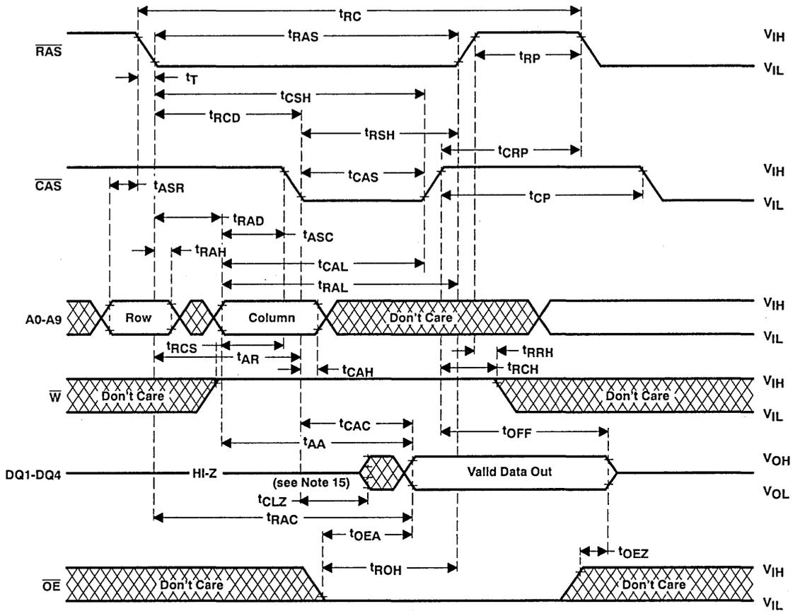
NOTE 15: Output may go from three-state to an invalid data state prior to the specified access time.
