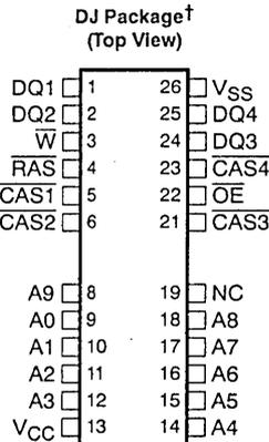
†The package shown here is for pinout reference only and is not drawn to scale.
