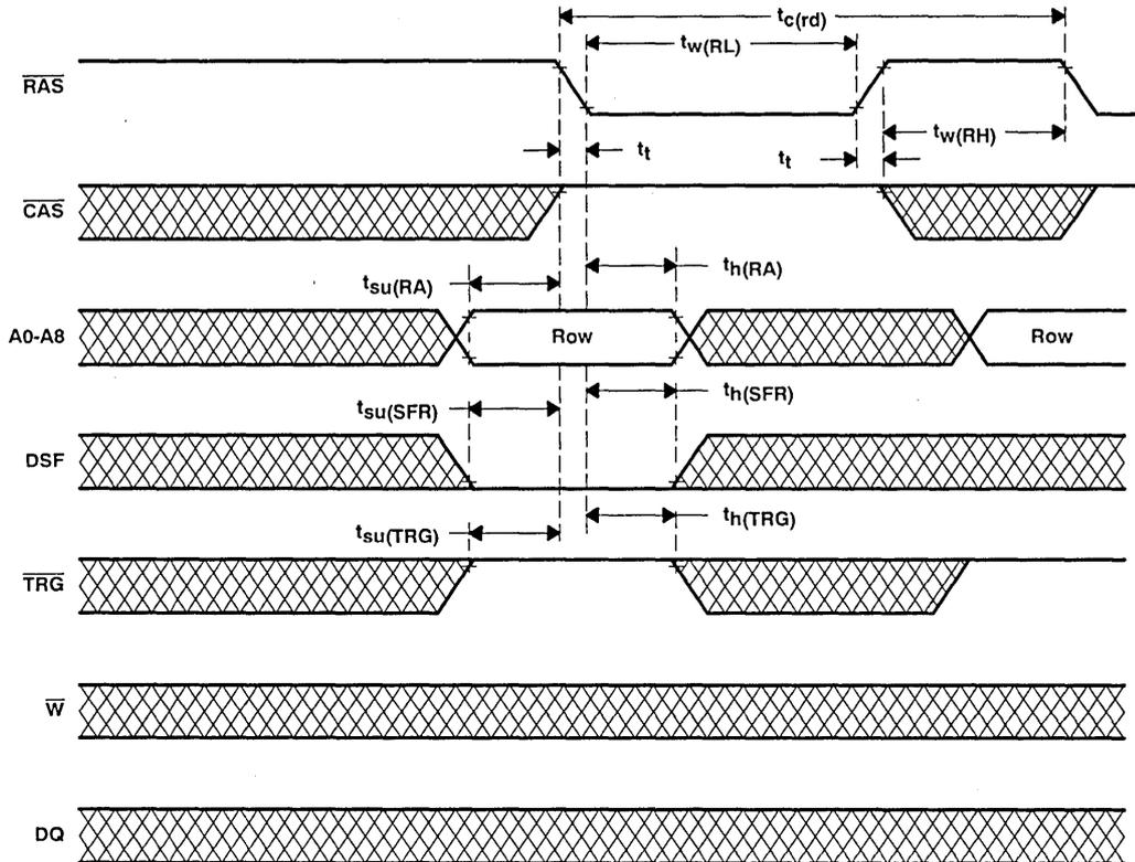
NOTE 29: In persistent write-per-bit function,  $\overline{W}$  must be high during the refresh cycles.
