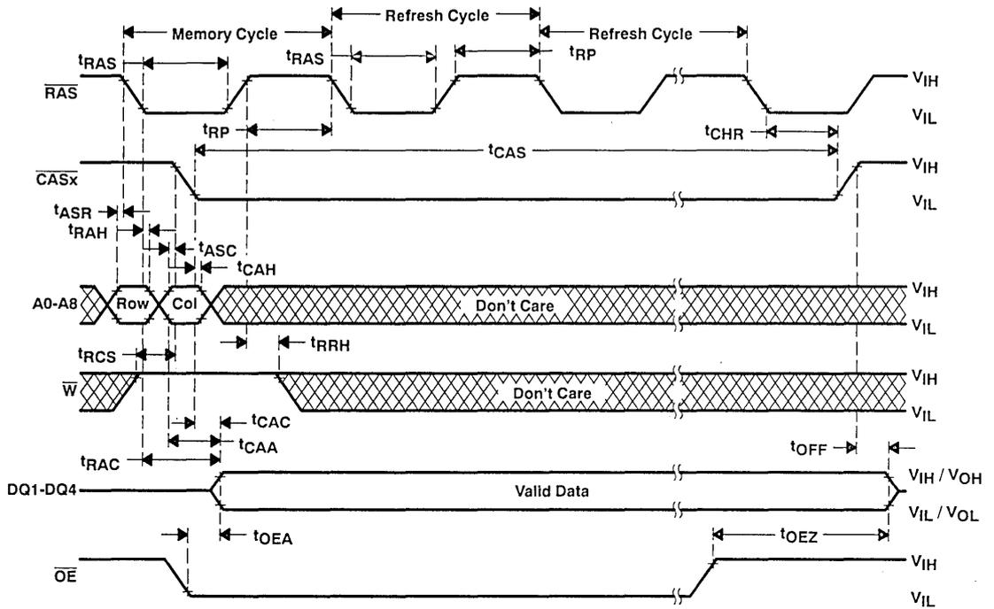
**automatic ( $\overline{\text{CAS}}$ -before- $\overline{\text{RAS}}$ ) refresh cycle timing**
