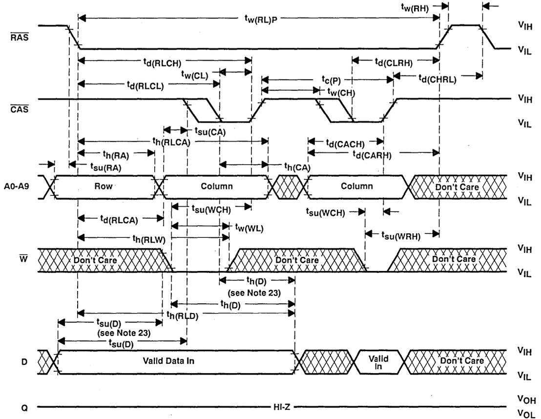
NOTES: 22. A read cycle or a read-modify-write cycle can be intermixed with write cycles as long as read and read-modify-write timing specifications are not violated.
