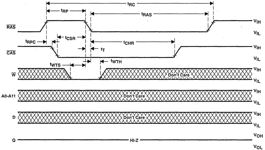
test mode exit cycle ( $\overline{\text{CAS}}$ -before- $\overline{\text{RAS}}$  refresh cycle)
