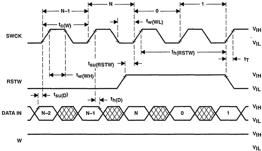
**write cycle timing (write enable)**
