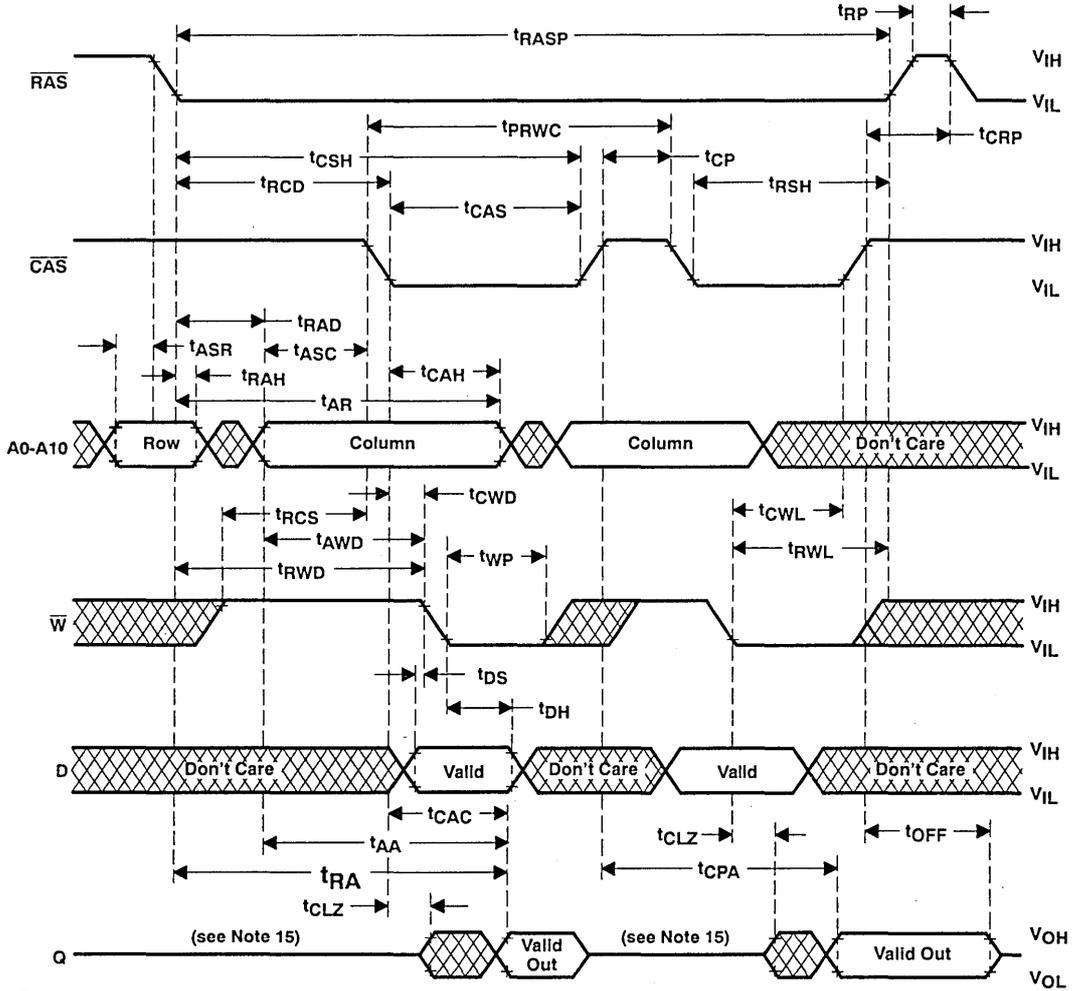
NOTES: 15. Output may go from three-state to an invalid data state prior to the specified access time.
