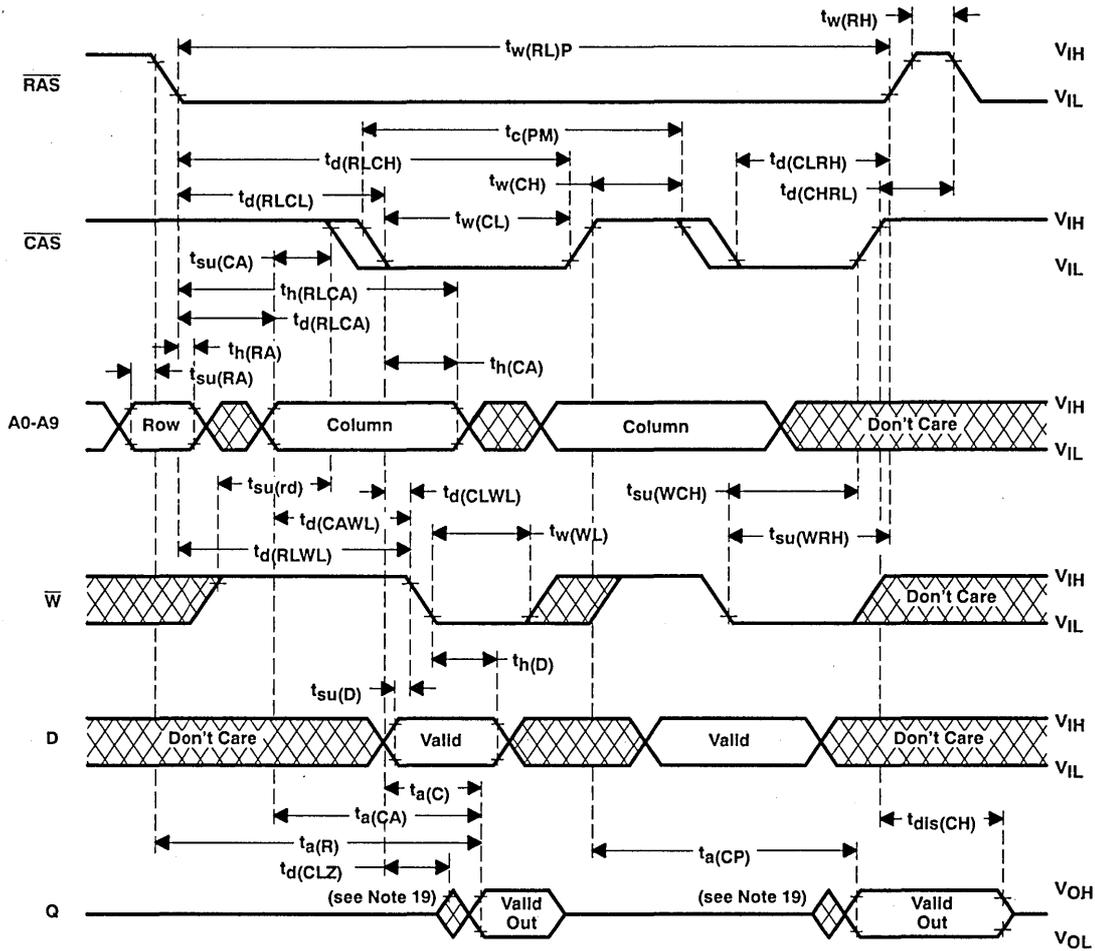
NOTES: 19. Output may go from high-impedance to an invalid state prior to the specified access time.
