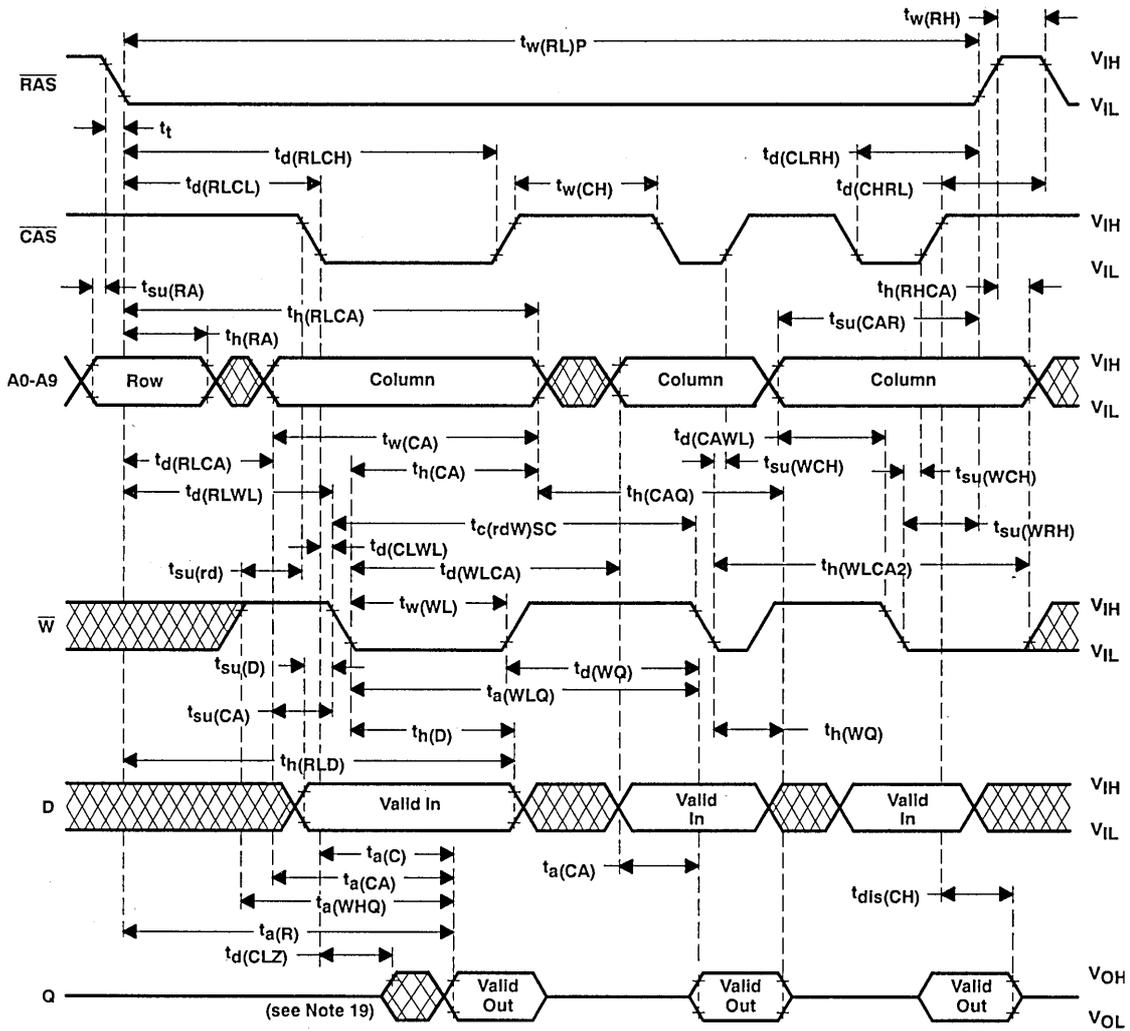
NOTE 19: Output may go from high-impedance to an invalid data state prior to the specified access time.
