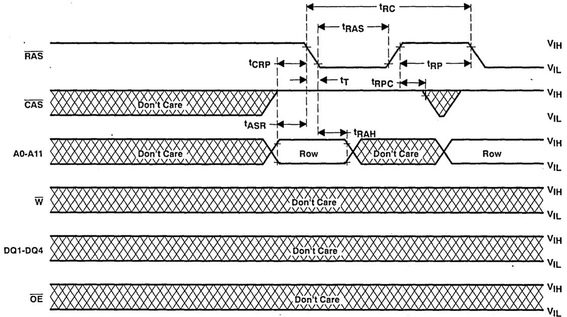
automatic ( $\overline{\text{CAS}}$ -before- $\overline{\text{RAS}}$ ) refresh cycle timing
