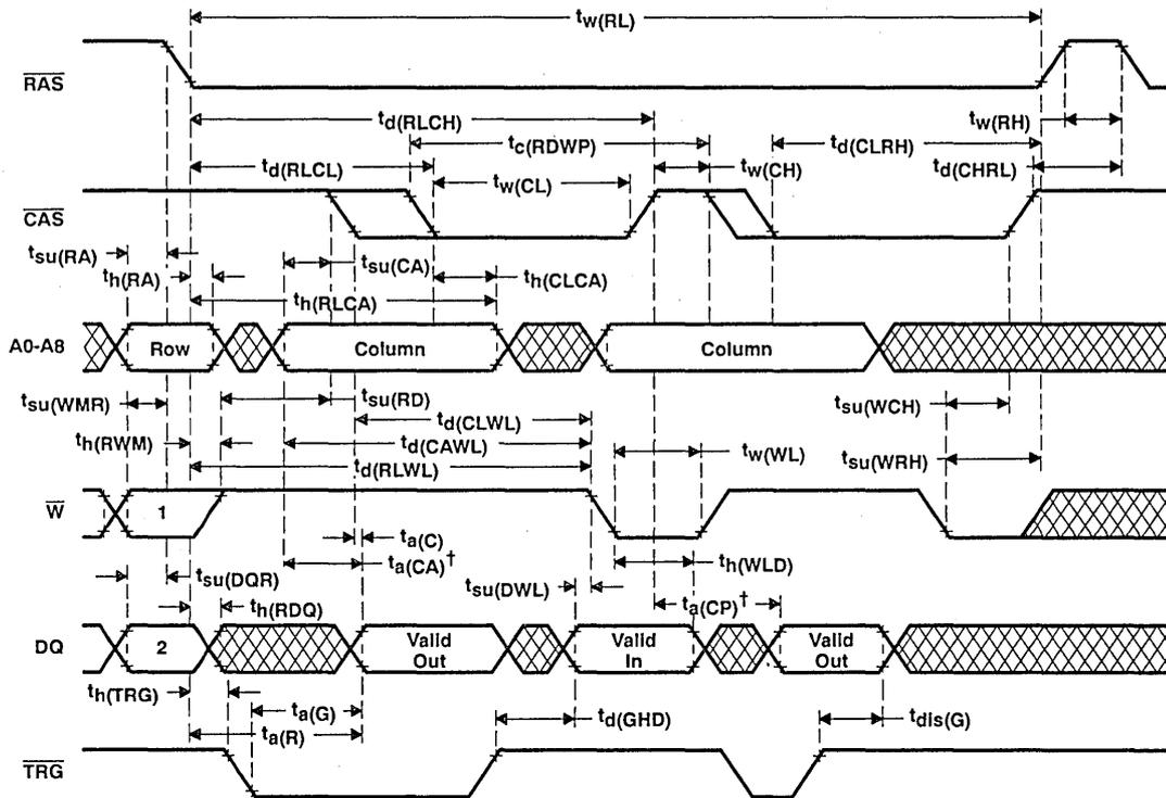
† Output may go from the high-impedance state to an invalid data state prior to the specified access time.
