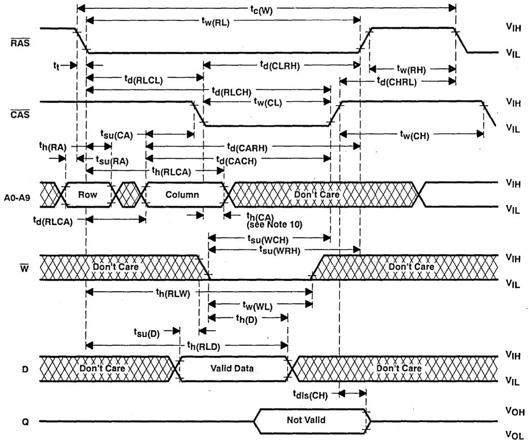
NOTE 10: Referenced to the later of  $\overline{CAS}$  or  $\overline{W}$  in the write operation.
