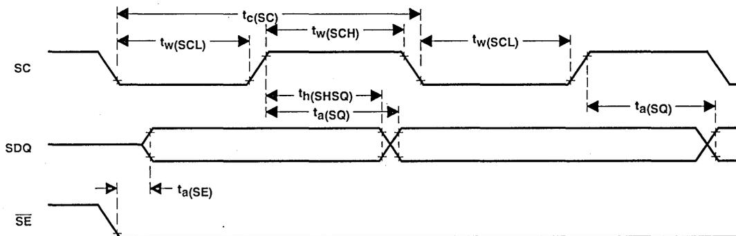
NOTE 38: While reading data through the serial data register, the state of  $\overline{TRG}$  is a Don't Care as long as  $\overline{TRG}$  is held high when  $\overline{RAS}$  goes low. This is to avoid the initiation of a register to memory to register data transfer operation.
