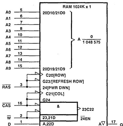
The TMS4C1024 symbol will be explained in detail for each operating function. The assumption is made that the previous sections have been read and understood. While this symbol is complex, so is the device it represents and the symbol shows how the part will perform depending on the sequence in which signals are applied.
