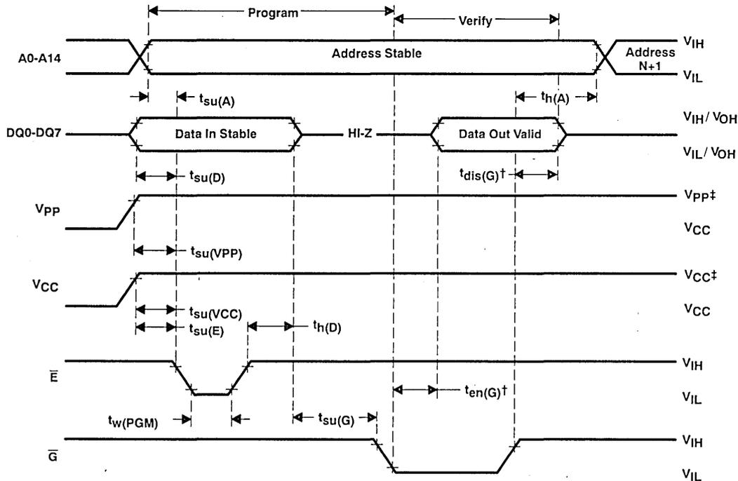
$^\dagger t_{dis}(G)$  and  $t_{en}(G)$  are characteristics of the device but must be accommodated by the programmer.
