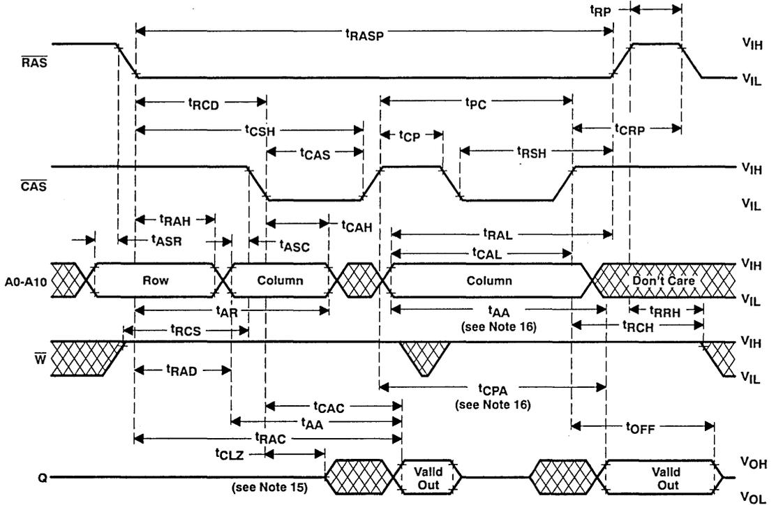
NOTES: 15. Output may go from three-state to an invalid data state prior to the specified access time.
