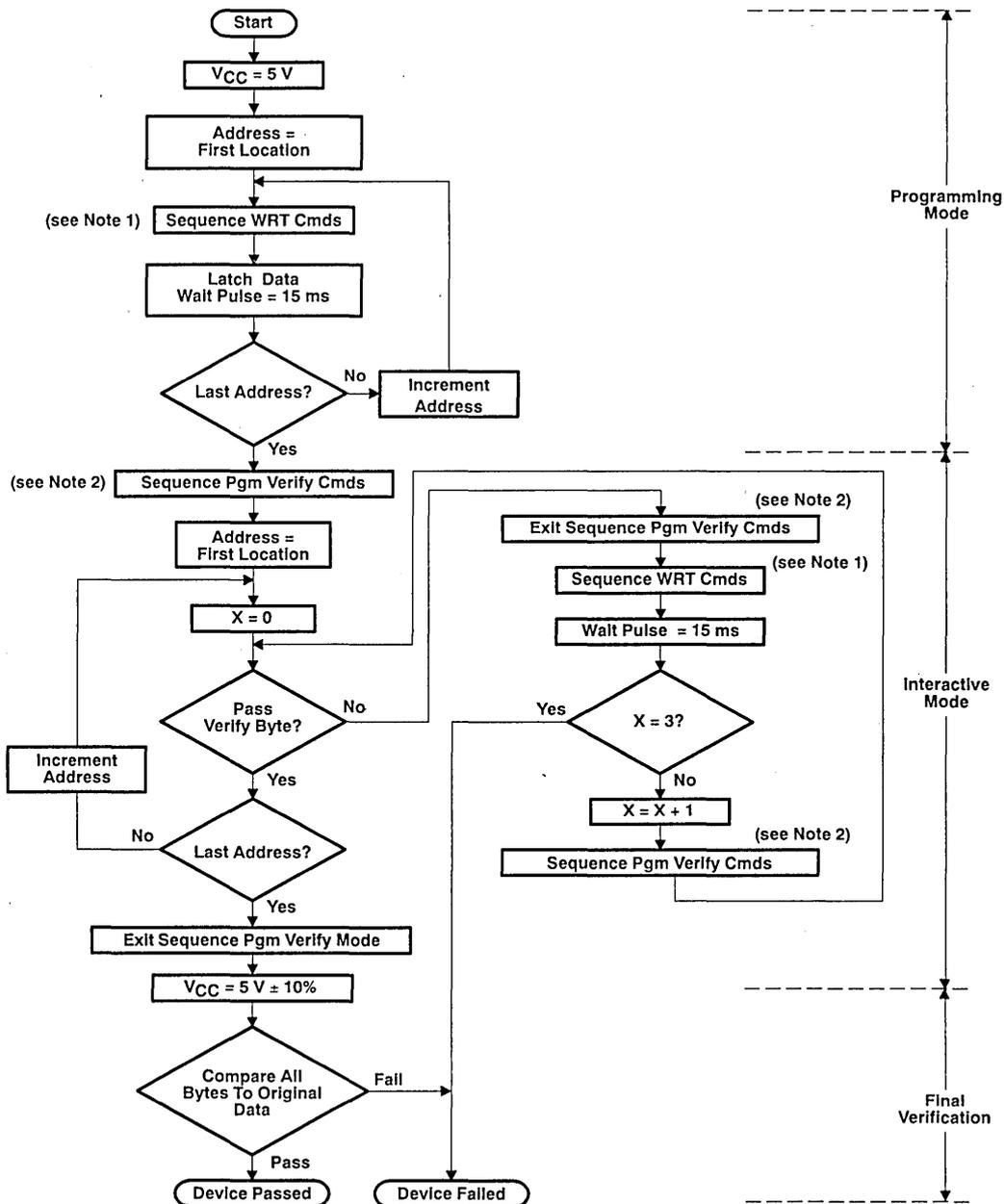
NOTES: 1. Upon the three-step sequence completion, the device is latched into programming mode. The byte is latched and the byte programming operation starts if a subsequent rising edge of  $\bar{W}$  is not detected within 100  $\mu$ s.
