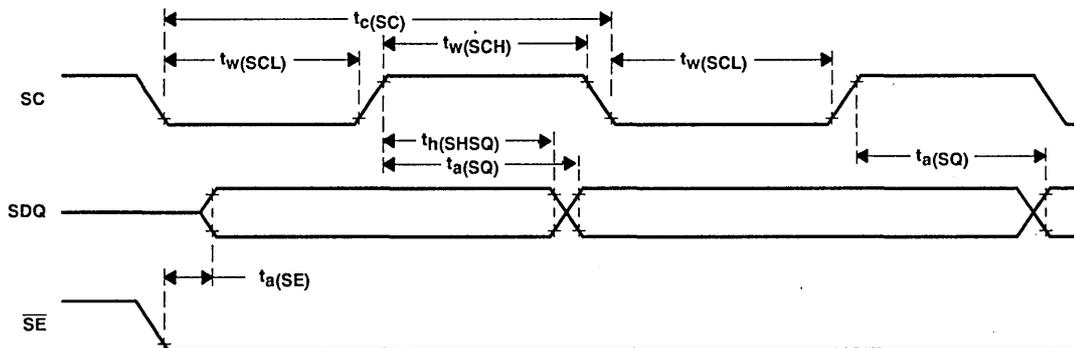
NOTE: 10. When the odd tap is used (tap addresses can be 0-511, and odd taps are 1,3,5 ... etc.), the cycle time for SC in the first serial data out cycle needs to be 40 ns minimum.
