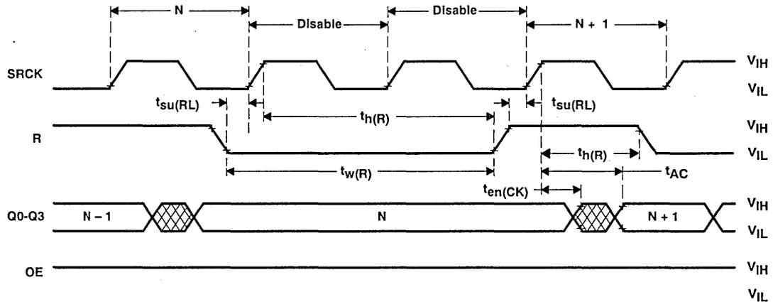
**read cycle timing (output enable)**
