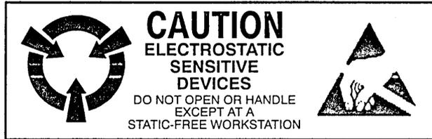
The warning label shall be legible and easily readable to normal vision at a distance of 3 feet.
