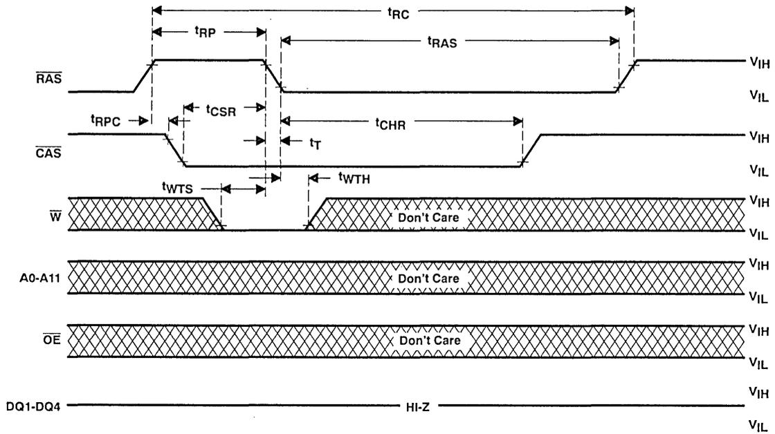
test mode exit cycle ( $\overline{\text{CAS}}$ -before- $\overline{\text{RAS}}$  refresh cycle)
