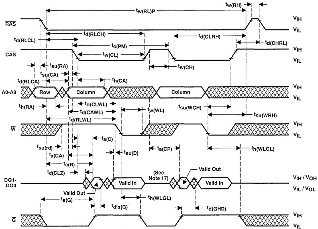
NOTES: 17. Output may go from high-impedance to an invalid data state prior to the specified access time.
