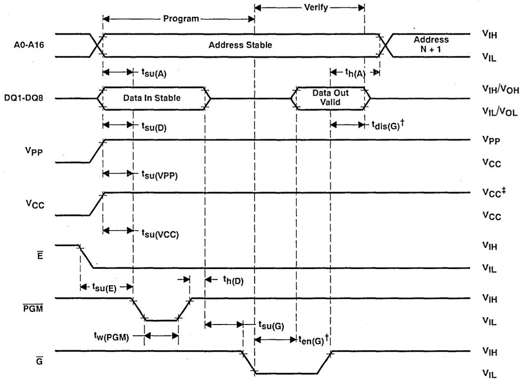
$^\dagger t_{dis}(G)$  and  $t_{en}(G)$  are characteristics of the device but must be accommodated by the programmer.
