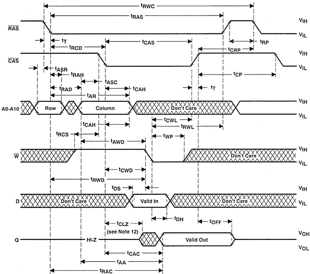
NOTE 12: Output may go from three-state to an invalid data state prior to the specified access time.
