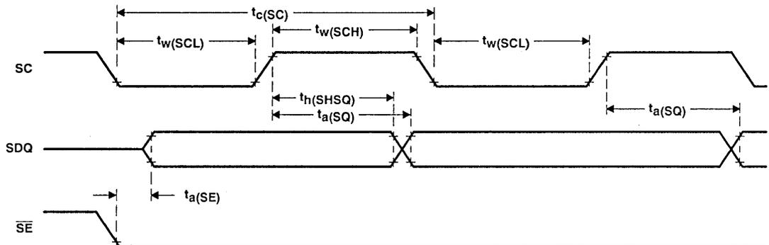
NOTE 10: When the odd tap is used (tap addresses can be 0-511, and odd taps are 1,3,5 ... etc.), the cycle time for SC in the first serial data out cycle needs to be 70 ns minimum.
