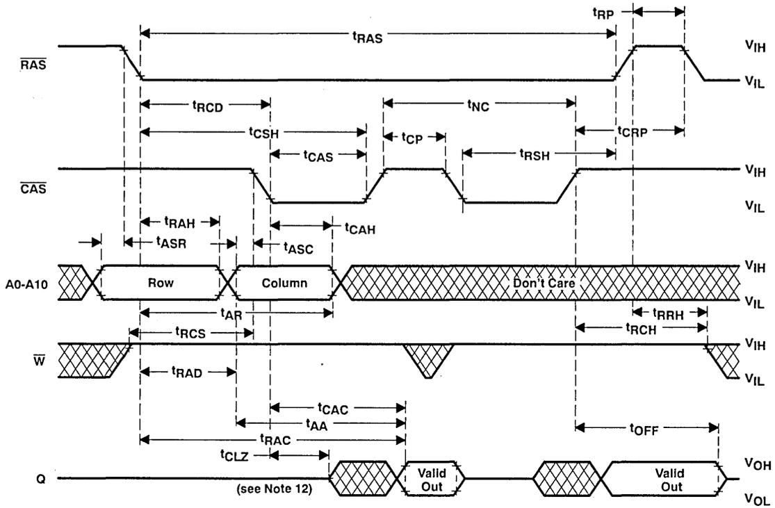
NOTE 12: Output may go from three-state to an invalid data state prior to the specified access time.
