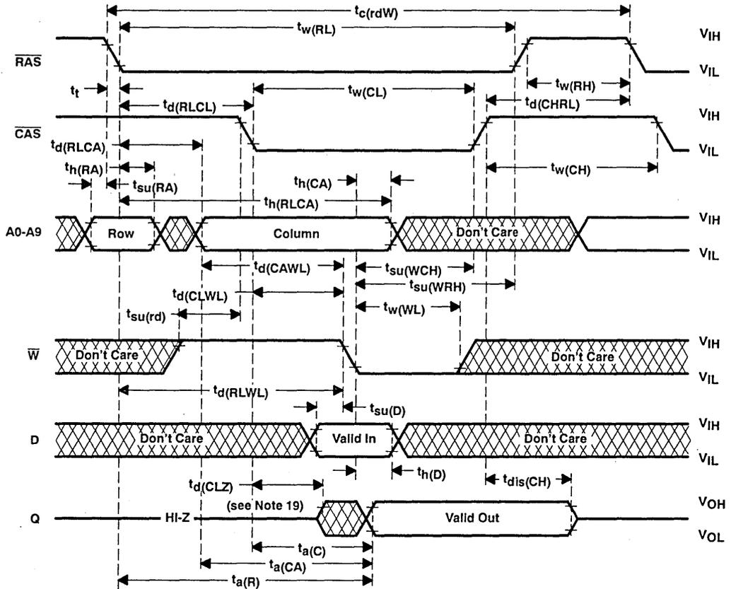
NOTE 19: Output may go from high-impedance to an invalid state prior to the specified access time.
