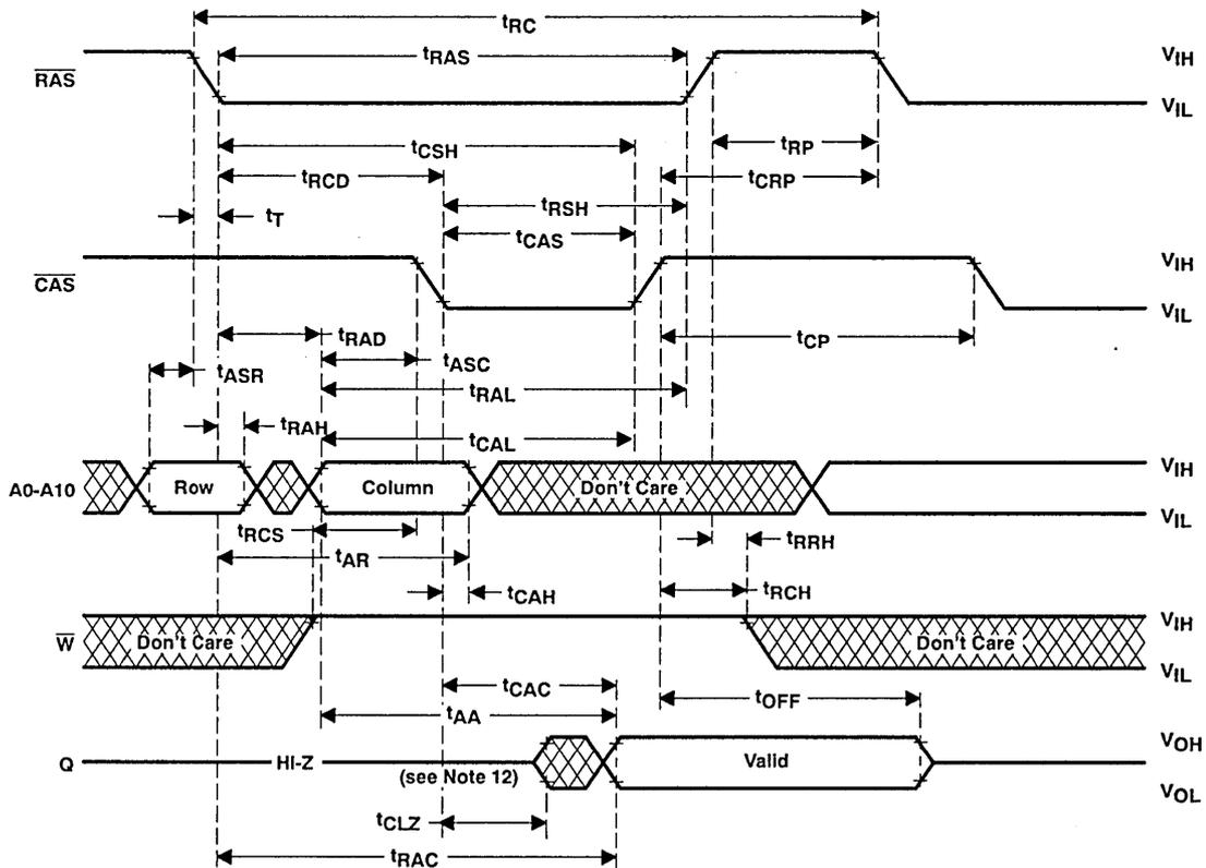
NOTE 12: Output may go from three-state to an invalid data state prior to the specified access time.
