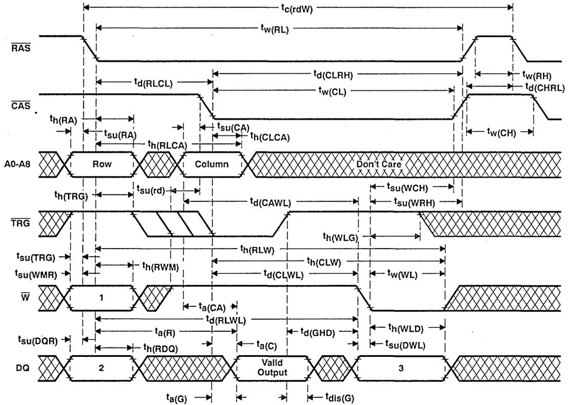
NOTE 24: See "Write Cycle State Table" for the logic state of "1", "2", and "3". Same logic as delayed write cycle.
