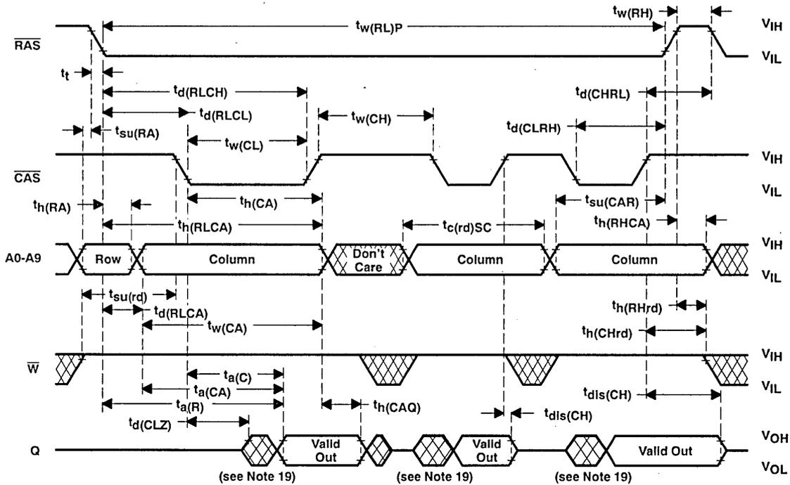
NOTE 19: Output may go from high-impedance to an invalid state prior to the specified access time.
