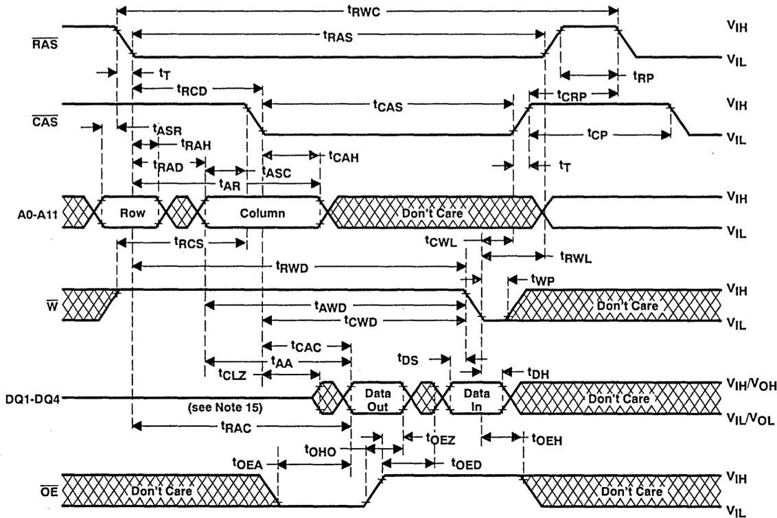
NOTE 15: Output may go from three-state to an invalid data state prior to the specified access time.
