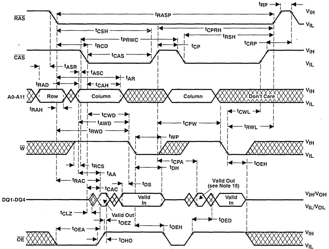
NOTES: 15. Output may go from three-state to an invalid data state prior to the specified access time.
