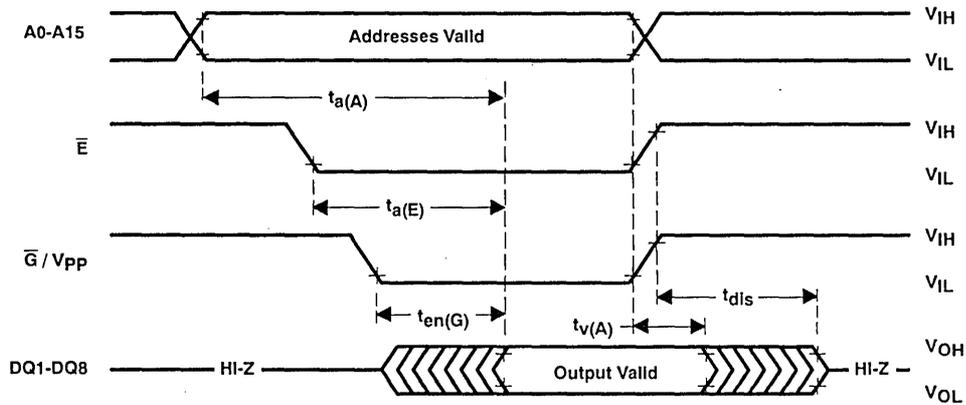
**program cycle timing (SNAP! Pulse programming)**
