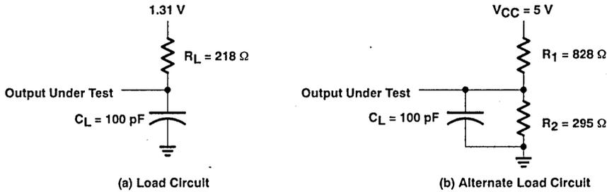
Figure 1. Load Circuits for Timing Parameters
