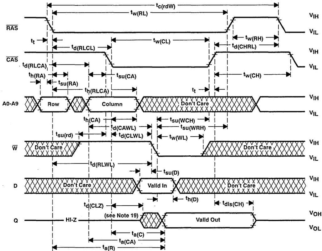
NOTE 19: Output may go from high-impedance to an invalid state prior to the specified access time.
