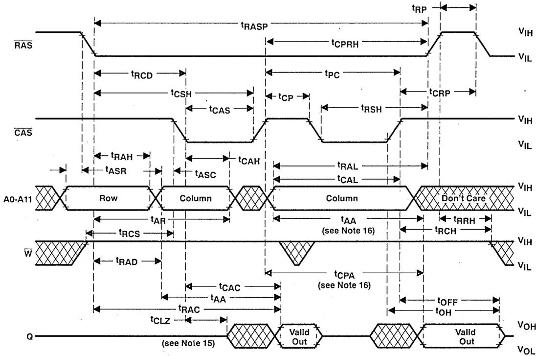
NOTES: 15. Output may go from three-state to an invalid data state prior to the specified access time.
