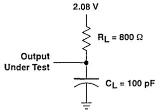
**Figure 5. Output Load Circuit**
