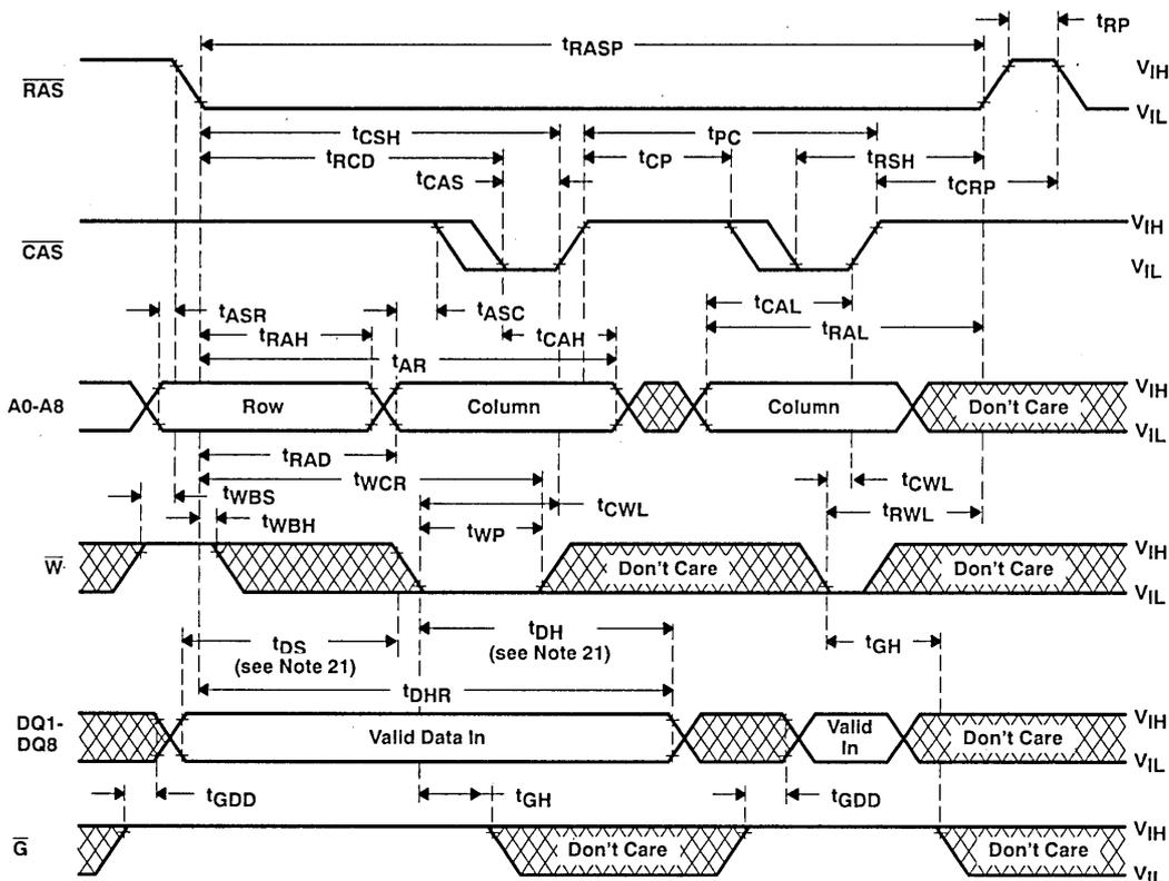
NOTES:20. A read cycle or a read-modify-write cycle can be intermixed with the write cycles as long as the read and read-modify-write timing specifications are not violated.
