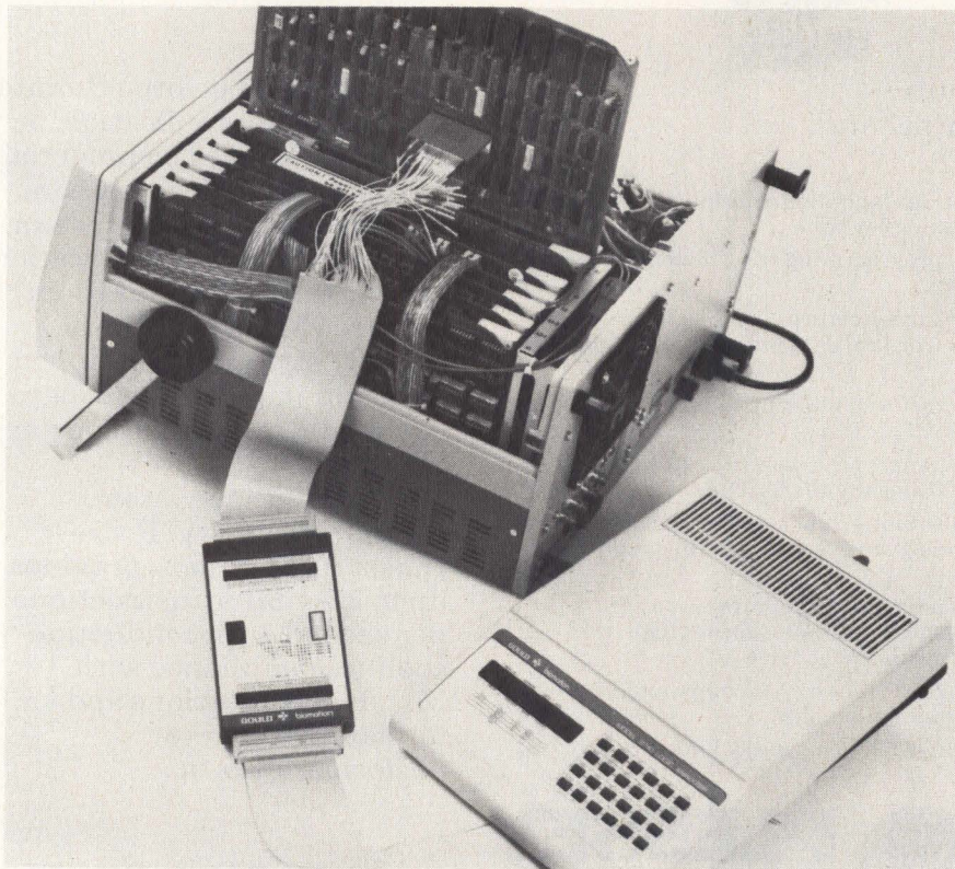
Universal microprocessor adapter (left) connects to Biomation's 2710 Data Domain Analyzer (right) to analyze 8-bit microprocessors, using added features of AND/OR clocking and common address/data bus demultiplexing
