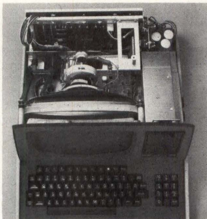
Integrated 8-bit microcomputer. Heath WH89 (with cover removed) contains keyboard, numeric keypad, floppy disc system (right front area), WH19 video terminal, 16k of RAM, and two Z80 microprocessors, all of which combine to handle high speed data processing tasks
