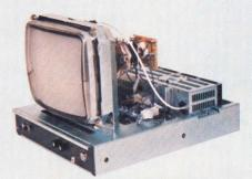
choice of screens to meet your specific application needs: Normal phosphor; long persistence phosphor to virtually eliminate flickering, or medium resolution versions for most ambient light situations.
