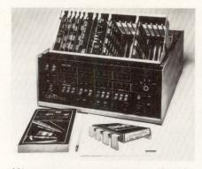
Microcomputer system. Pacific Cyber/Metrix's PCM-12 Omega runs DEC PDP-8 software without modification, and provides tilt-up card cage with 18-card capacity, heavy duty power supply, and full function front panel
