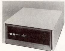
A series of STD-Bus based computers can be configured by the user to tailor a system using multisourced hardware and software components based on the STD-Bus. This integrated system allows users to select packaging and disc storage components that most closely fulfill select requirements. The Matrix OEM series is Z80 based and comes with or without 8" (20-cm) floppy disc drives.
