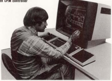
Incorporated in the IMI-500 advanced graphics display system, is a multiprocessor scheme designed to increase speed and flexibility and allow realtime 3-D viewing of complex objects. The system includes a 24-bit bipolar bit slice display processor, which incorporates a 24-bit floating point processor, a bipolar LSI display driver, and a Z80 based display controller. The display itself is a 21" (53-cm) calligraphic stroke type with a resolution of 4096 x 4096 points.
