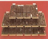
(2048 bytes) data buffer makes "data-late" errors a thing of the past. The advanced technology "micro-engine" allows a complete track to be written on a single drive revolution. A measurable performance advantage for your PDP-11.
