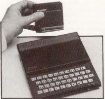
cuitry. New features include the ability to operate in 2 software selectable modes, fast and normal; fast is four times the speed of normal. In the normal mode, the computer will both compute and display simultaneously, allowing continously moving, flicker-free graphics.
