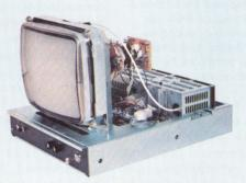
choice of screens to meet your specific application needs: Normal phosphor; long persistence phosphor to virtually eliminate flickering, or medium resolution versions for most ambient light situations.
