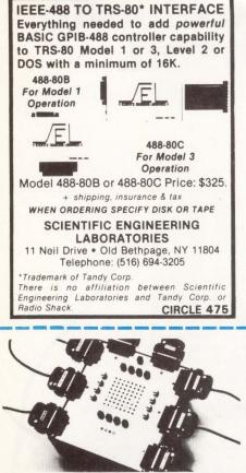
**RS232 DATA SWITCHING MATRIX** Implements every possible connection between Tx Data and Rcvd Data for eight I/O ports.
