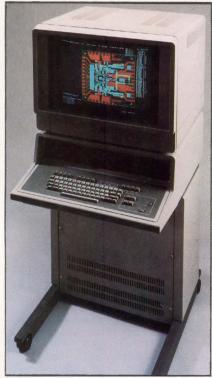
A 19" (48-cm) raster scan color display terminal that supports local picture segments, 2-D transforms, zoom and pan, and up to 4 bit planes of display memory has been added to the Tektronix 4110 series. The 4113 uses a 60-Hz noninterlaced scan to eliminate flicker, even for displays with large areas of a single color. In addition, the 3 standard bit planes allow use of 8 colors simultaneously. An optional 4th plane increases this number to 16.
