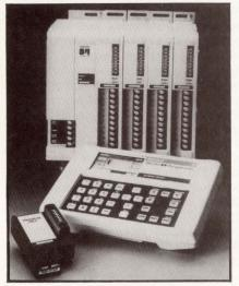
Solid state Micro-84 allows users to control small machine operations requiring 4 to 60 relays. The device has a free formatted multinode programming format, with programming in relay symbology. In addition to relay functions, it provides internal timers; counters; and arithmetic, drum, and sequencer functions. The controller can be programmed using the P190 multifamily CRT programming panel or the company's handheld/tabletop LCD programming panel.
