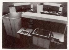
227x circuit board test system family. 2272 (foreground), 2271 (background right), and 2270 (background left) share same basic system architecture and can use same test programs. Fixtures are upward compatible between systems (continued on page 106)
