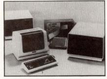
Modular 9516 microsystem integration station offers realtime in-circuit emulation, software and hardware analysis, and softkey and menu-driven human interface to ease debugging of microprocessor based systems. System features totally transparent realtime operation implemented in a dual bus structure for realtime control and monitoring. Dual bus allows access to the logic trace analyzer for setup and display without stopping emulation. The
