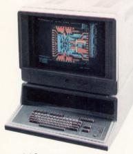
**112** A raster scan color graphics display terminal supports 2-D transforms and up to four bit planes of display memory
