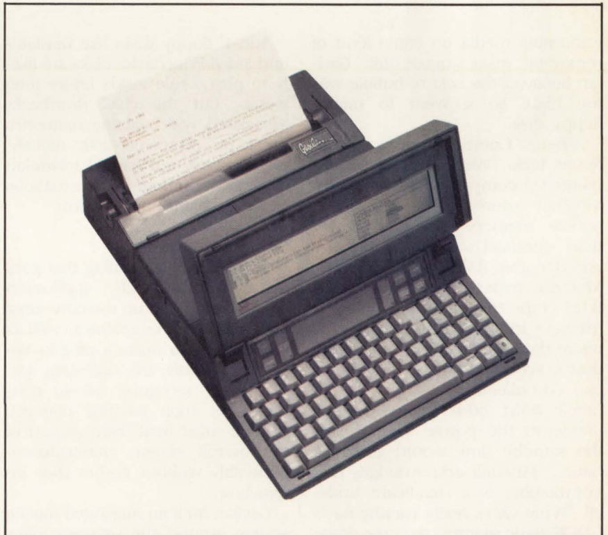
Gavilan's mobile computer was built around human interface software and a solid state "mouse" control panel. Plug-in CMOS RAMs with onboard battery retain data for about a year.
