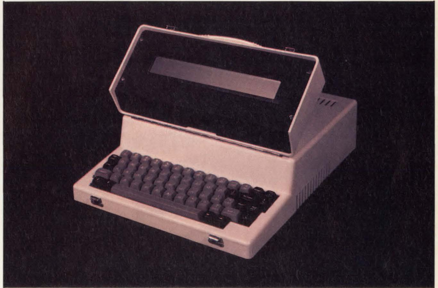
Athena Computer's 16-bit upgrade to the Athena I is first to market with the 80C86 CMOS processor. The dynamic RAM pseudodisk, however, presently limits standby data retention to six hours.
