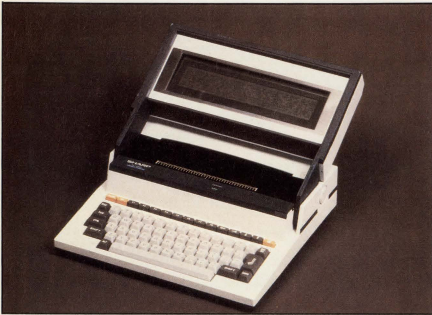
Sharp Electronics' PC-5000 features pop-in bubble memory cartridges for 128K bytes of nonvolatile storage. A high resolution LCD generates 640- x 80-dot bit-mapped graphics.
