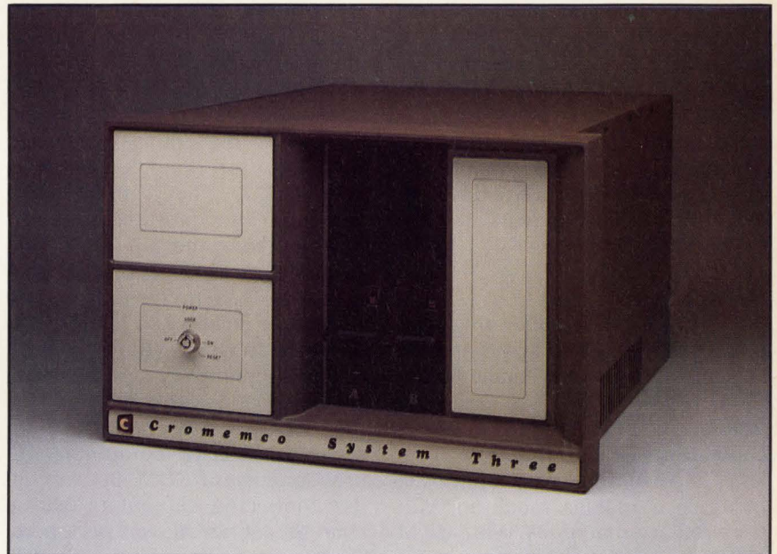
Cromemco's dual-processor System Three, like other members of the company's multi-user D-series computer systems, contains both a 16/32-bit 68000 and an 8-bit Z80A microprocessor. Therefore, the system can run software written for either microprocessor.
