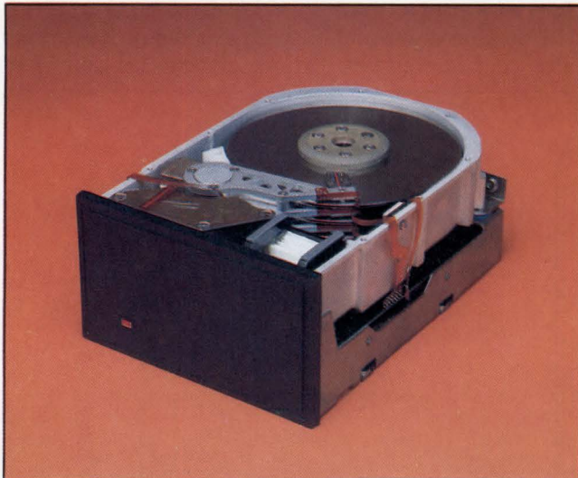
Tandon's TM705 uses standard Winchester heads with plated media to store 50 Mbytes on three platters. Track density of 1000 tracks/in. is achieved using a closed-loop servo system with rotary voice coil positioner.
