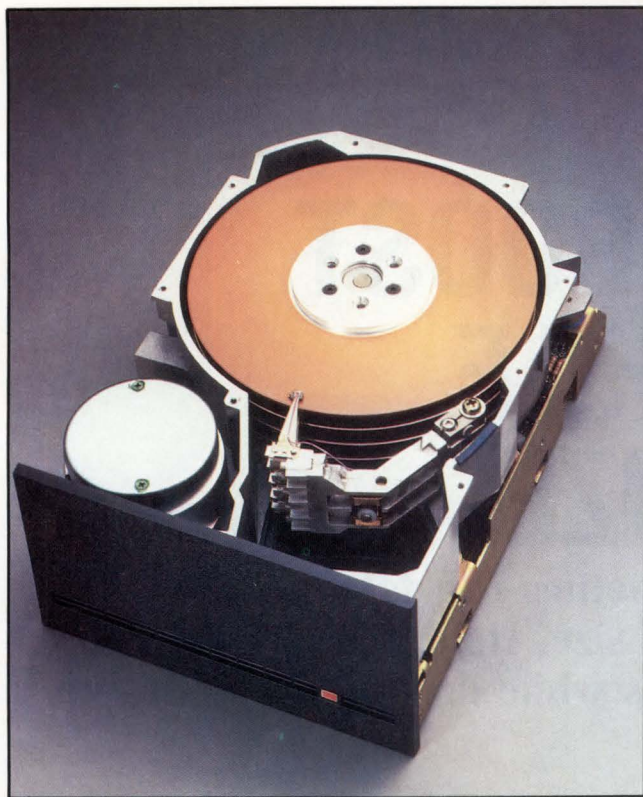
An 80-Mbyte capacity, 5¼-in. drive, Computer Memories' CM7880 writes data on four platters. The ability to pack platters into the compact unit results from mechanical design and use of 3370-type head flexures.
