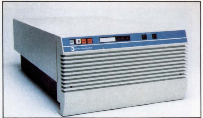
Using 19 thin-film heads to read/write on five 14-in. platters, Century Data's Advanced Marksman Series 571 meets high capacity, high performance needs. Multiple heads/platter cuts average access time to 19 ms.
