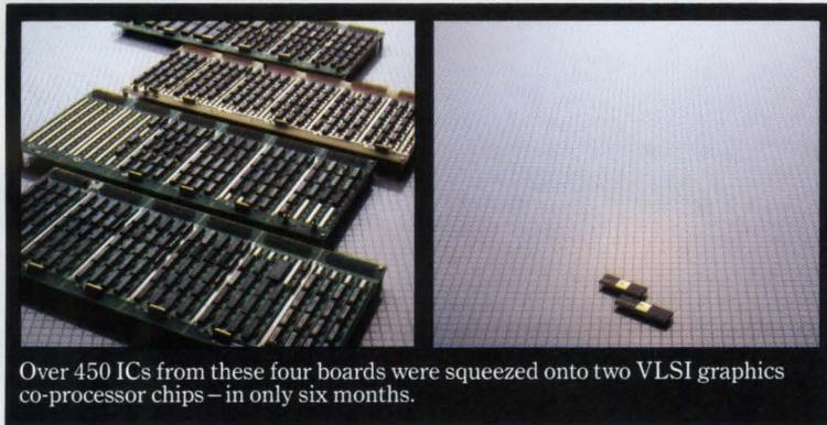
Over 450 ICs from these four boards were squeezed onto two VLSI graphics co-processor chips—in only six months.
