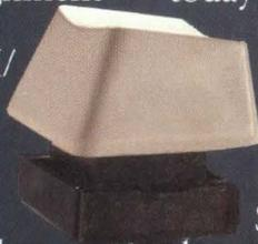
The ergonomically designed full travel switches have a total stroke of .140 (3.6 mm nominal), are rated at 50 million cycles, are wave solderable and field repairable. The switches contain Stackpole's patented twin bifurcated contacts, with four make-point redundancy, which assures you of switch closure. And today's sophisticated electronics make mechanical switch operation reliable and dependable...at lower cost.
