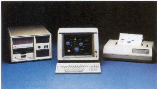
Techniques of structured analysis developed in data processing are used in a set of software tools tailored to meet the needs of software project specification. The tools are designed to define system and software problems at the beginning of the design cycle, before the actual code is written. These Structured Analysis (SA) tools cover four main areas: graphics diagram editing, internal consistency checking, error correcting, and format-
