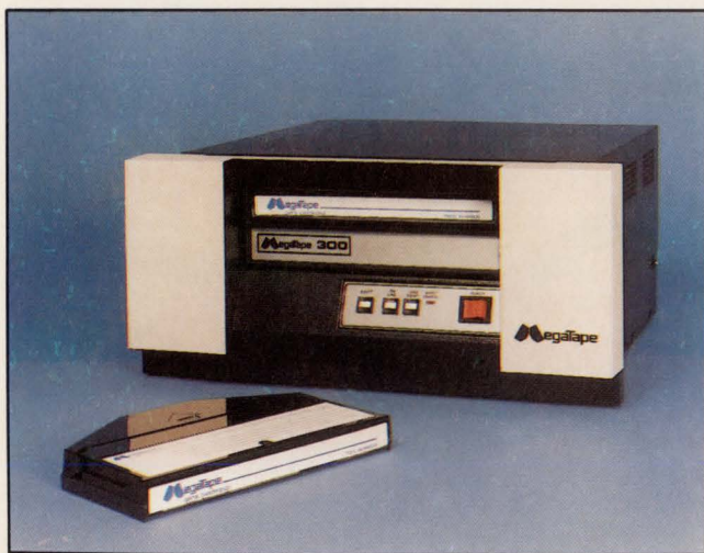
The MT-2210 cartridge tape drive from MegaTape can backup or restore 500 Mbytes in 36 min. Data are written on 1500 ft of half-inch tape using a 24-track serpentine format at a packing density of 9600 bits/in.
