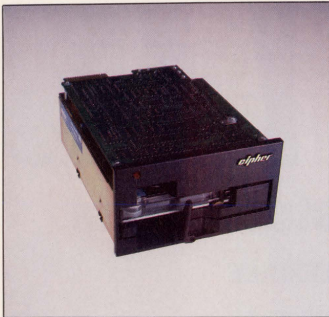
Fig 1 A floppy tape device can greatly increase the online secondary storage capacity of floppy-based systems, without any significant changes in system software or controller hardware.
