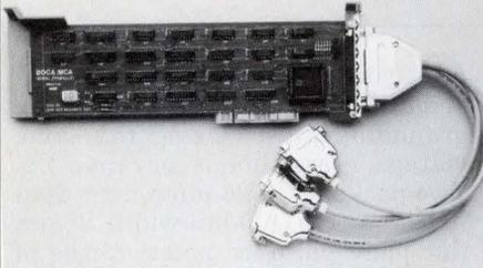
figured as COM1 through COM8. The parallel port can be configured as LPT1 through LPT3. Installation is conducted via the IBM set-up program. The .ADF file is supplied with the board. The price is \$210.
