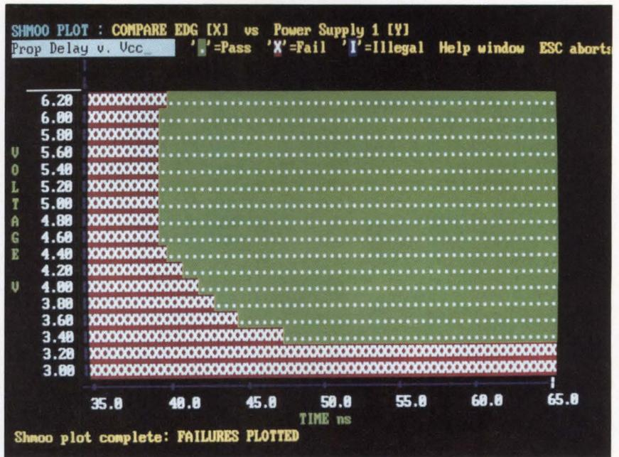
A Shmoo plot, an analysis tool included in prototype testers, lets users plot the interaction of any timing or voltage parameter against any other. A common application of a Shmoo plot is testing power-supply voltage ( $V_{cc}$ ) against propagation delay, as shown here on the Hilevel Topaz V system.
