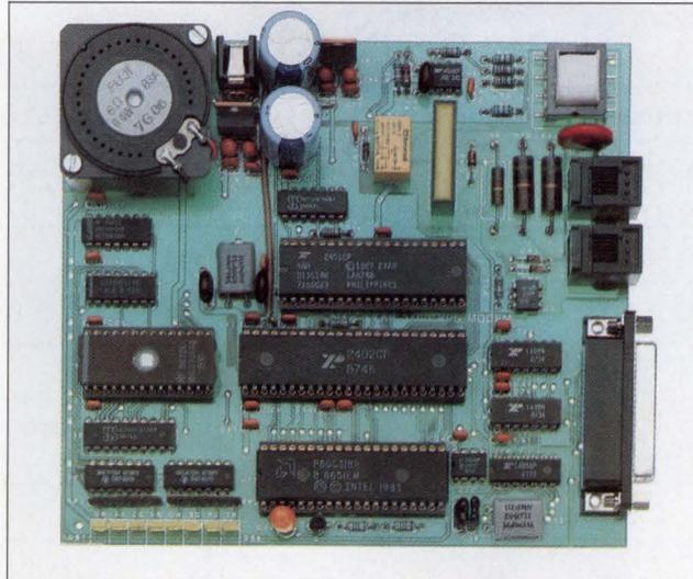
*V.22bis-compatible chip sets such as Exar's XR-2400 give designers maximum flexibility by supplying complete modem functionality in two compact packages. The set consists of the XR-2401, a general-purpose digital signal processor, and the XR-2402 analog front-end. Rather than use a dedicated controller, the chip set is designed to interface to popular off-the-shelf parts such as the 8051 and Z8.*
