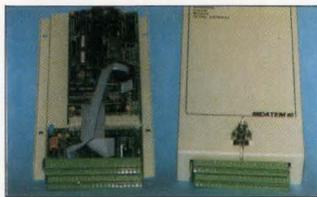
—The dDCN5000 family of intelligent communication gateways allow a range of equipment to be integrated into a DISTRIBUTED CONTROL NETWORK. Firmware drivers support interfaces to RS232, RS422, RS485, IEEE-488, and CENTRONICS; multitiered BITBUS networks are also supported. DATEM Ltd., 148 Colonnade Rd., Nepean, Ontario, Canada, K2E-7R4 — (613) 225-5919.
