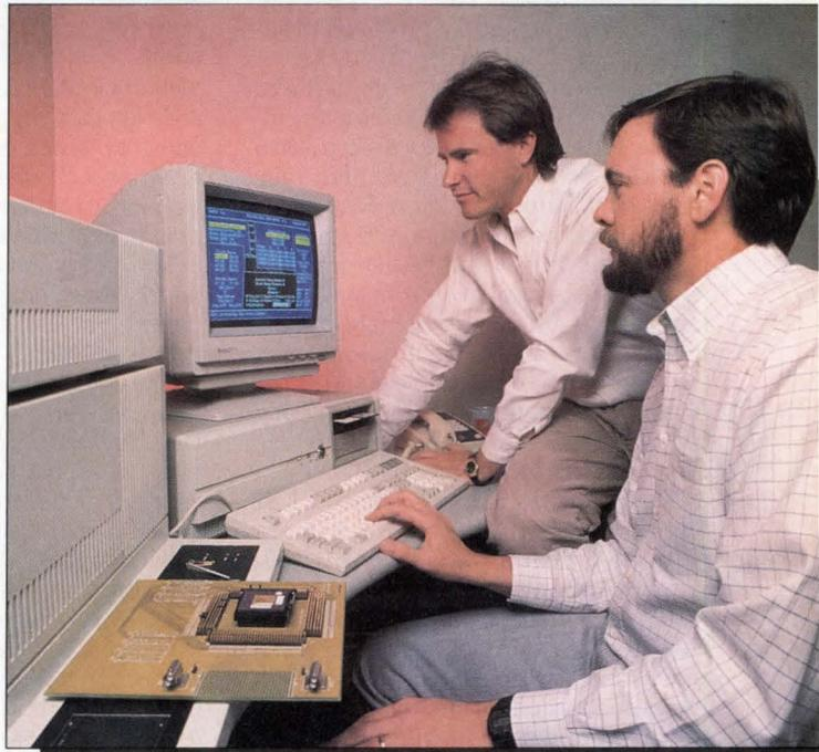
*Paul Gifford (right), manager of systems engineering at Sequent Computer, and Steve Shovoly, engineer responsible for application-specific IC verification and procurement, use a Cadic STM5200 digital VLSI test system for ASIC design verification and characterization. Sequent, like many designers of complex ASICs, has turned to prototype testers because, according to Gifford, a foundry won't tell you how close you are to your operating margins.*
