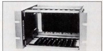
Full line with a .75" card spacing, extruded aluminum frames, aluminum endplates and non-conductive card guides. Open frame design excellent for convection cooling. Variety of mounting styles with 5, 8, 16 and 21 slots in stock.
