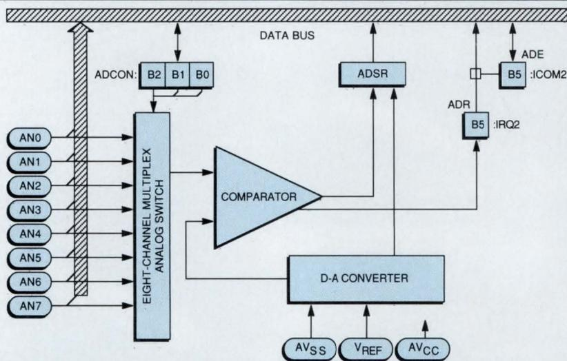
Nearly all analog-to-digital converters on microcontrollers are of the 8-bit successive-approximation type, as shown in the M37450M2 device from Mitsubishi Electronics America. The converter selects each successive bit of the digital output based on the difference between the current output and the input.
