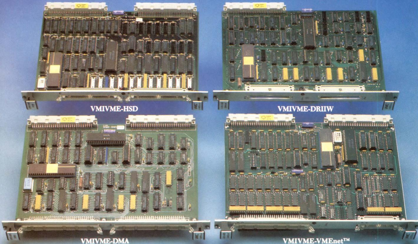
**VMIC manufactures a wide range of parallel DMA interfaces that allow VMEbus connection to a wide range of Host computers.**
