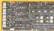
**Quadmodem** Four 2400 bps Full Duplex Modems on One Board
