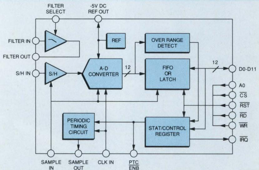
*Highly integrated analog-to-digital subsystems, such as Analog Devices' AD1332, can pack all the necessary stages of an ac data-conversion system into a single chip not much bigger than an external sample-and-hold (S/H) unit. Such packages provide an important alternative to on-chip A-D converters for non-dc applications.*
