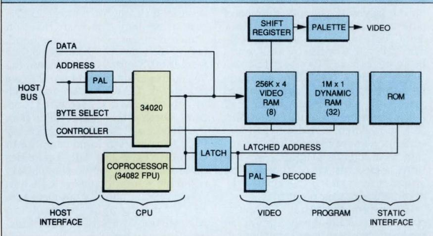
*This is one example of a graphics subsystem architecture using the TMS34020 graphics system processor and the TMS34082 floating-point coprocessor from Texas Instruments. The 34020 has equally direct access to the video RAM frame buffer and to dynamic RAM program memory, thus enabling the host to transfer large sections of code in a single operation, reducing bus overhead. In addition to its internal functions, the 34082 has access to user-designed microcode stored in ROM.*
