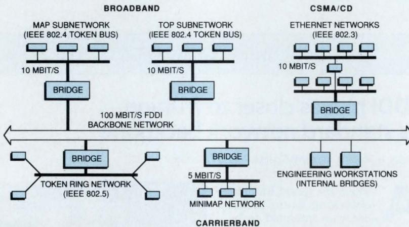
*Its 100-Mbit/s throughput will enable the Fiber Distributed Data Interface (FDDI) to serve as the backbone support for many slower speed LANs, such as IEEE-802.3 twisted-pair or coax Ethernet, IEEE-802.5 token ring and IEEE-802.4 broadband coax MAP. Bridges between the slower LANs and the fiberoptic backbone will be external for most applications, but will be built into devices such as larger computer systems.*
