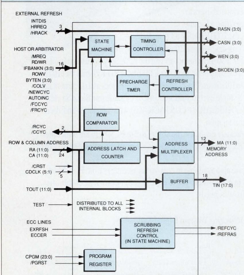
The controller macro of the TI toolkit offers multiple row-address strobe (RAS) and column-address strobe (CAS) outputs for bank selection and byte or word access. It operates with a 50-MHz clock, and RAS-to-CAS low time is programmable in 20-ns intervals. Via a test mode pin, the address bus may be used to transmit test data onto a test bus, allowing completely independent testing of the memory system.
