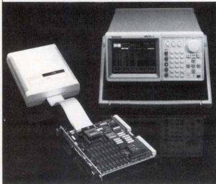
**Logic analyzer supports 68030 microprocessor**
