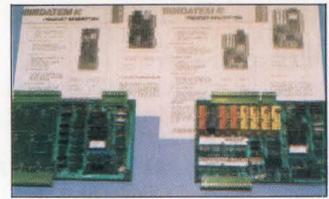
—The dDCM53x family of intelligent BITBUS compatible analog/digital industrial controllers allow OPTO-22 compatible termination modules to be integrated within a DISTRIBUTED CONTROL NETWORK that supports up to 250 nodes over 8 miles. Programmable in C, BASIC and Ladder, modules are supported by a comprehensive set of network development tools for DOS, QNX, XENIX, VMS. DATEM Ltd., 148 Colonnade Road, Nepean, Ontario, Canada K2E-7R4 — (613) 225-5919.
