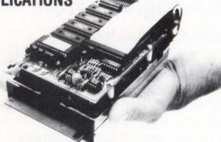
**TINY188** is a low cost "PC somewhat compatible" engine for OEM controller applications. A selection of high level languages is available in ROM.
