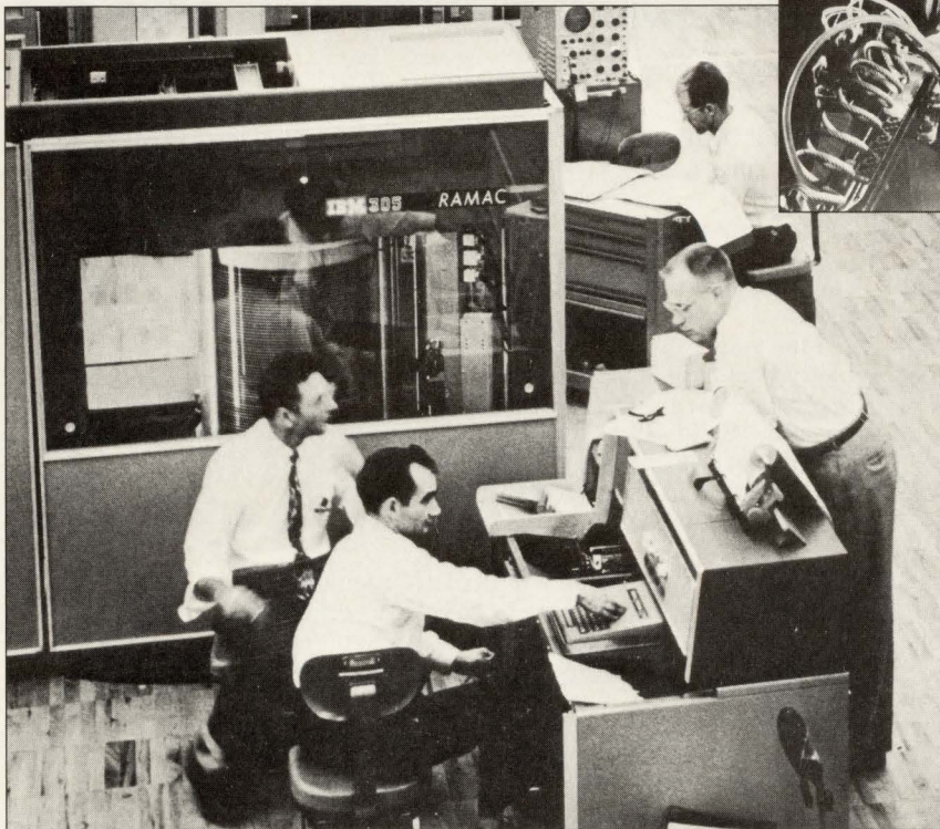
The first hard disk storage unit was the RAMAC 350, a refrigerator-sized unit introduced in 1956 by IBM's San Jose Research Center. The RAMAC, which stood for random access method of accounting, replaced sequential access tapes with random access methods, and set the stage for interactive computing. The machine stored 5 Mbytes of data on 50 24-in. platters.
