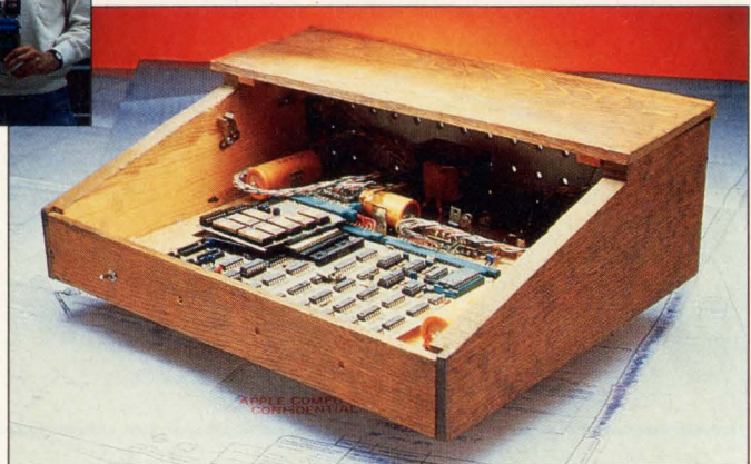
The board-level Apple I required hobbyists to add a keyboard, power supply and case. The second product designed by Apple Computer's Wozniak and Jobs was the Apple II, the first personal computer for the mass market.
