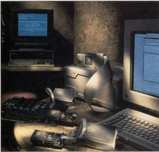
The CodeTap 960 CA rounds out Applied's development environment for Intel's i960 CA superscalar RISC processor, providing an alternative to expensive emulators. Able to run transparent to the target system at up to the full clock speed of the i960 CA, CodeTap can do everything an emulator can do except locate complex time-related errors.
