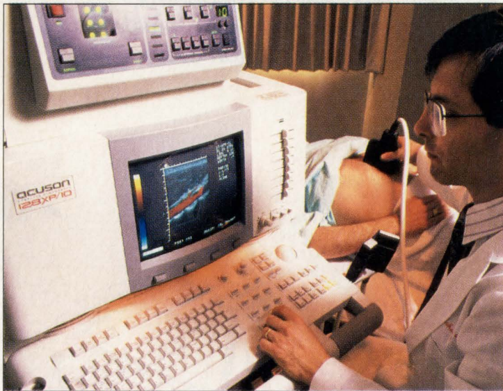
Medical imaging, such as computer-aided sonography, is one of the few high-performance applications in which much of the signal processing must be performed with precision analog circuitry. State-of-the-art sonography machines, like this one from Acuson, can image cancer cells on the surface of a body organ several inches beneath the surface of the skin. While sonographic scanners operate at frequencies of 2 to 10 MHz, the resolution required is typically greater than 16 bits—a sampling resolution requirement stretching the capabilities of commercially available data converters. Shown on the screen in this photograph are red blood cells in an artery.
