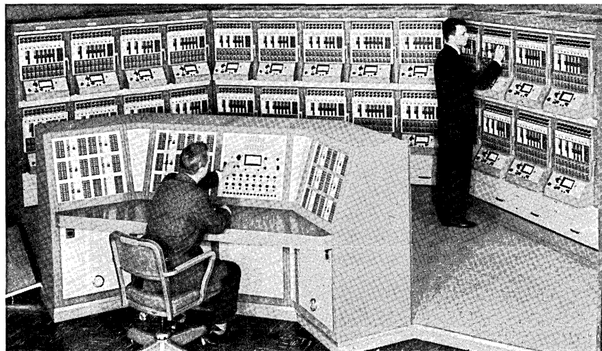
A large, transistorized analog computer system is shown undergoing final inspection and check out at EAI. The system was built under a contract from the U.S. Signal Corps.
