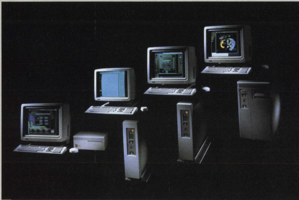
DEC's family of VAX-based workstations. (L-R) The new VAXstation 2000, the monochrome VAXstation II system, the 4-plane and the 8-plane VAXstation II/GPX systems.
