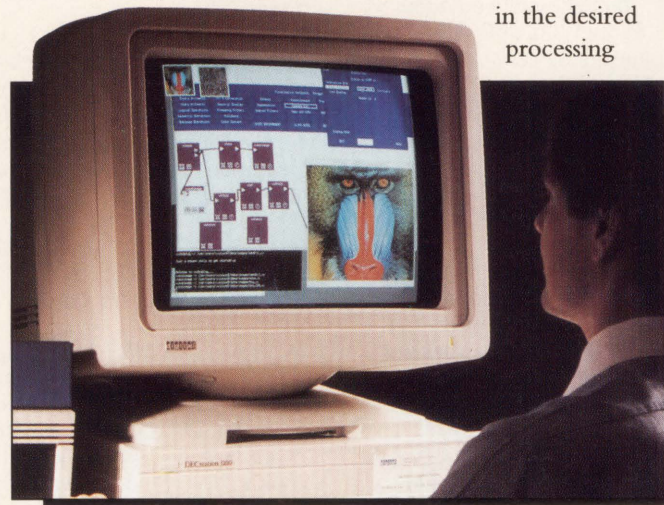
Paragon Imaging's Visualization Workbench incorporates a visual programming system and automatic program generators that let nonprogrammers develop imaging applications.
