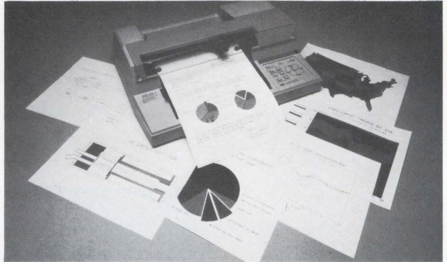
Figure 1: The HP7470 pen plotter can be connected to a variety of computers to produce high-quality business and technical graphics on overhead transparency film and paper.
