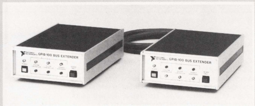
Bus extenders allow the bus to be used in a network configuration.
